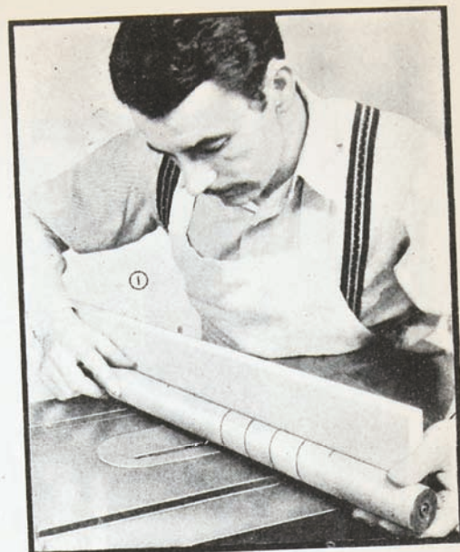
Perfect Spirals on Round Stock are Easily Cut with the Circular Saw Method.
