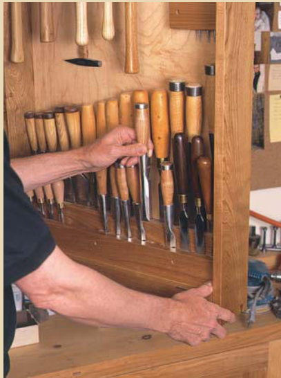
TIERED CHISELS. Inside the door, chisels are stored in dadoed strips to protect their cutting edges.
