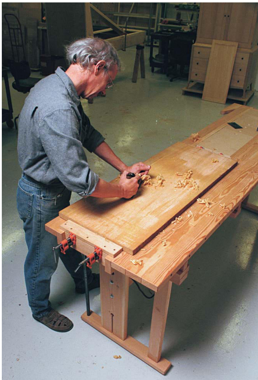
HORIZONTAL CLAMPS RUN FULL LENGTH. A pair of pipe clamps, running under the benchtop, hold work in the same way that a traditional tail vise does.
