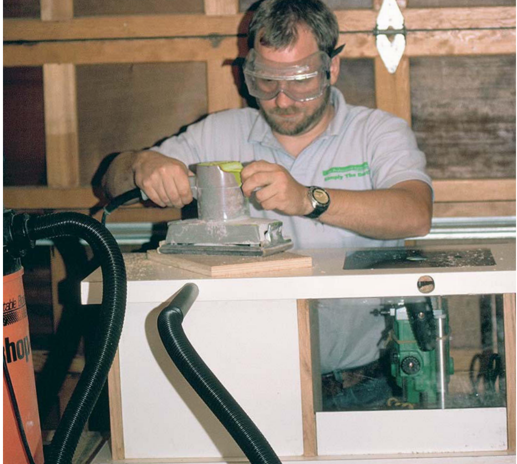
VACUUM SIDE HAS PLENTY OF CLAMPING POWER. The vacuum surface (left) clamps a drawer front as the author sands its face. An open hole on the edge of the table (right) shows where he connects his shop vacuum when he's routing.
