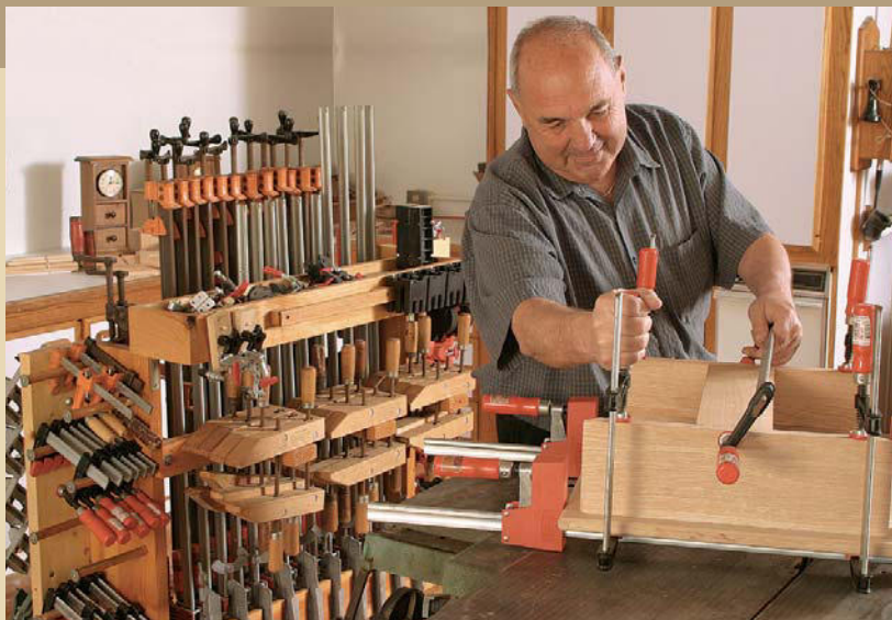
HAVE CLAMPS, WILL TRAVEL. Blessed with plenty of floor space, DiRanna chose to put all of his many clamps on a rolling cart.
