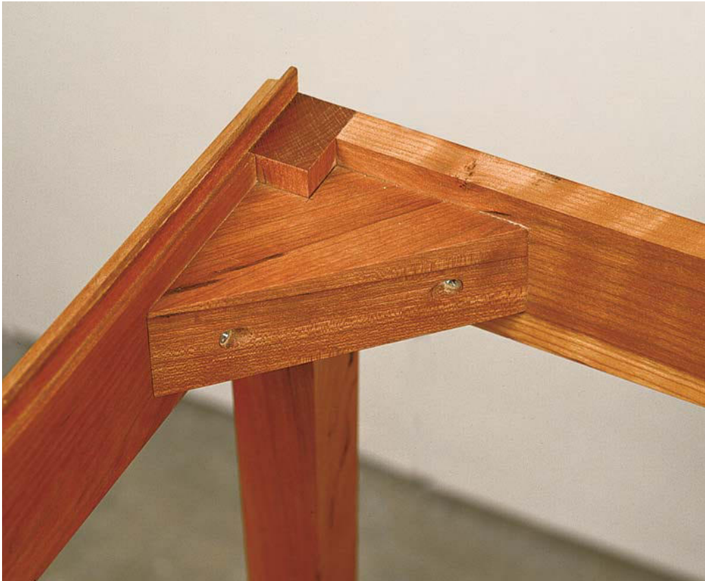
SUPPORTING HEAVY LOADS. Corner braces reinforce the mortised-and-tenoned rail-to-leg joint and enable this elegant base to support the heavy tool chest.
