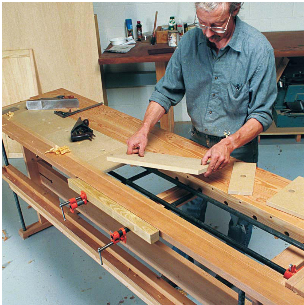
LIFT-OUT MDF PANELS. The panels, cut in different lengths from MDF scraps, make a durable yet disposable center surface for the bench. The panels get removed when the tail-vise pipe clamps are in use.
