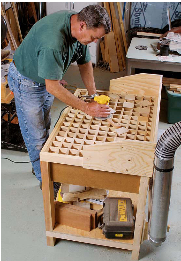
THIS SHOPMADE UNIT CONQUERS dust without breaking the bank.
