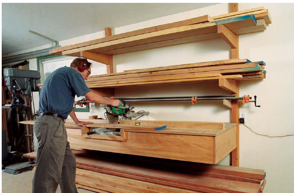
CANTILEVERED ARMS AND A BUILT-IN CHOPSAW TABLE provide plenty of storage, easy access, and efficient cross-cutting in a small space.
