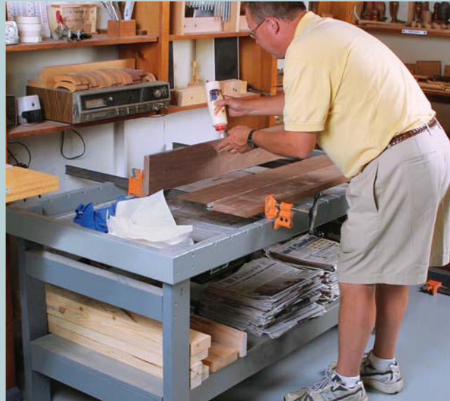
LESS STRESS AND LESS MESS. The slotted table frame holds clamps in position while you're gluing up boards. Any glue squeeze-out drips into the newspaper-lined tray.
