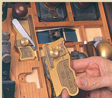
FITTING A TOOL. Odd-shaped tools, such as this side rabbet plane, fit into french cutouts in the shelf.
