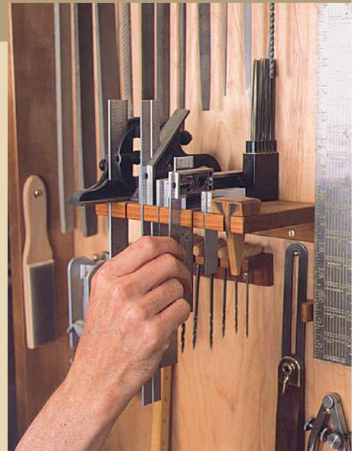
SHELVED SQUARES. Becksvoort's squares slide into sawkerfs cut on a small shelf, which takes up much less space than laying them out flat.
