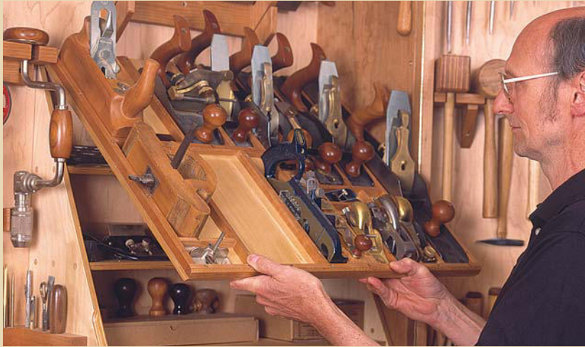
PLANES WITHIN EASY REACH. Ledger strips locate planes on the shelf, and small pieces of leather are used to protect the blades.
