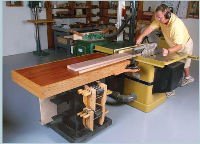
A MULTIPURPOSE SUPPORT TABLE. This table can be wheeled to support operations at the tablesaw or the jointer, while the base stores clamps and jigs.
