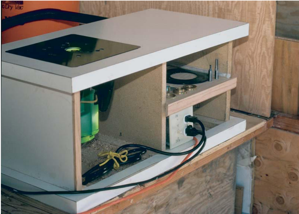
TO WIRE HIS TABLE , the author fed a 4-in. work box for a pair of switched receptacles: one for the vacuum, one for a router or sander. A shelf at the back of the table holds tools and accessories. He drew outlines of the items and routed recesses to hold each shape, which reminds him when something's missing.
