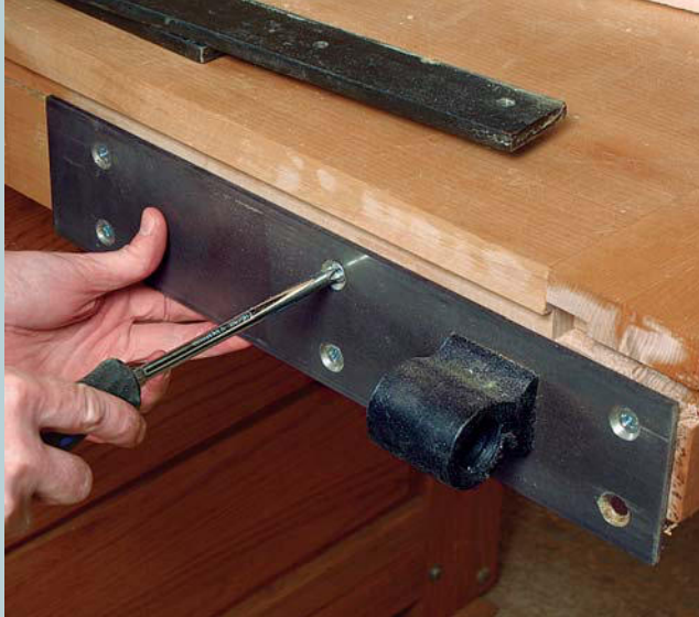
SECURE THE MAIN PLATE. Position the top edge of the plate slightly above the bottom edge of the groove in the top.
