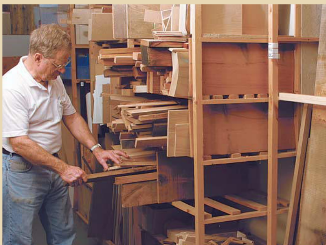
ADJUSTABLE WOOD STORAGE RACK. The rack is converted from horizontal storage to vertical storage by simply removing the crosspieces.
