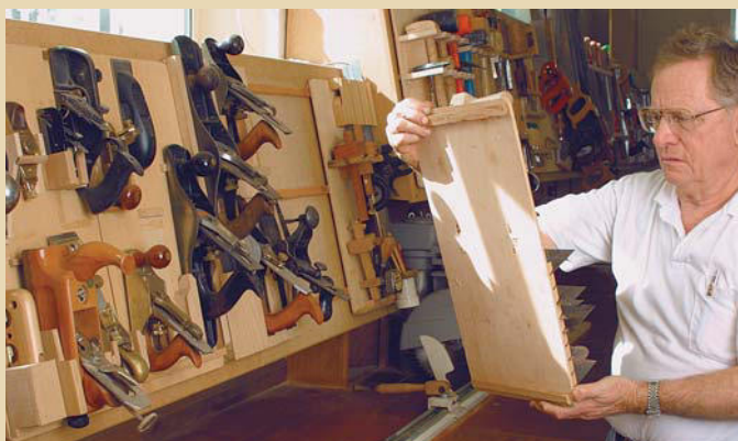
ANGLED TOOL RACKS ARE PLACED ABOVE THE BENCH. Individual tool holders are attached to the rack with French cleats.
