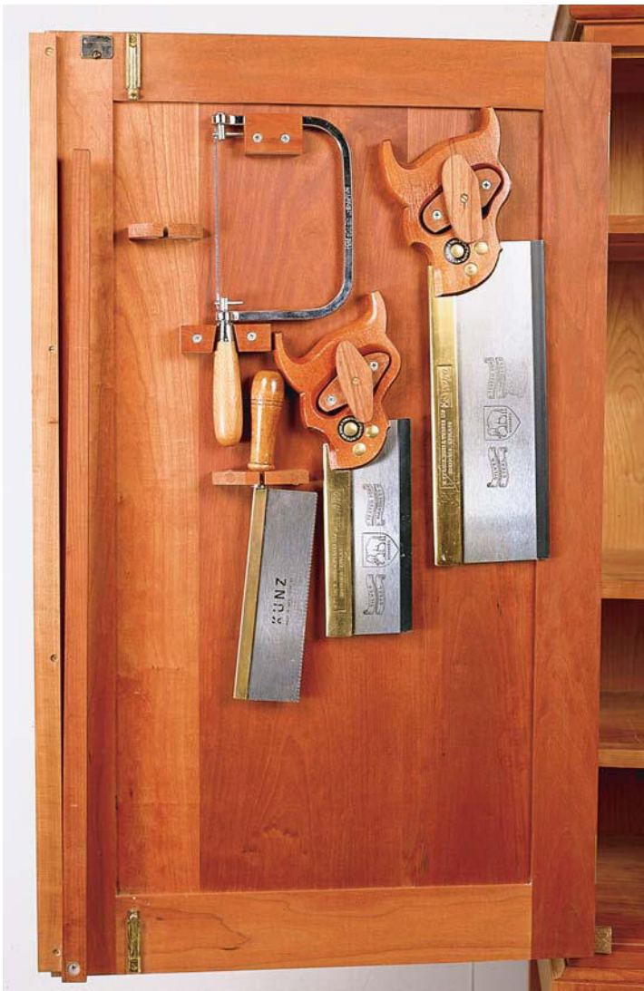
PREVENTING DOOR SAG. Legs screwed to the doors' lock stiles help support the heavy tools hung on the doors and prevent the hinge screws from pulling out.
