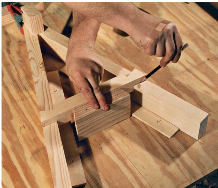
A SIMPLE, NAILED-TOGETHER JIG SPEEDS LAYOUT and ensures consistency from horse to horse. Here, the author scribes around the end stretcher dovetail to cut out its mortise in the leg.
