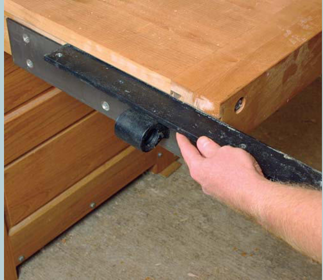
SLIDE THE TOP PLATE ONTO THE MAIN PLATE. When properly located, the top guide plate should slide smoothly along the main plate without interference.
