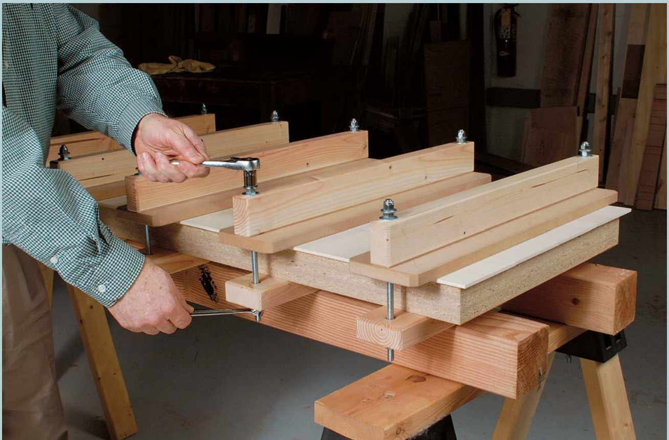
CLAMP THE VENEER TO THE PARTICLEBOARD WITH CLAMPING CAULS. No need to have a small fortune in clamps to do this glue-up. Shopmade clamping cauls get the job done for pennies.
