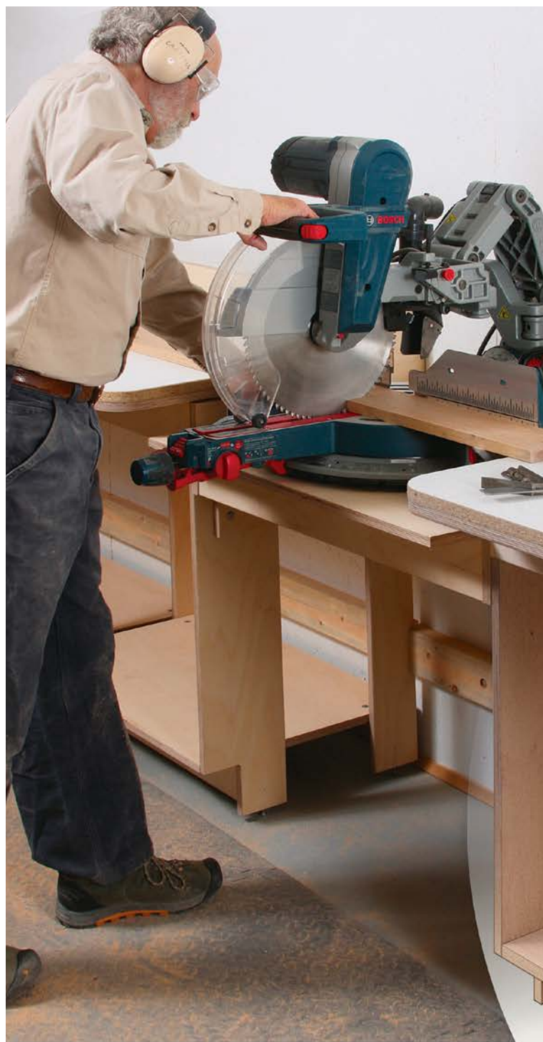
Smart use of plywood. Beneath a spacious top, a clever leg design maximizes the yield from a sheet of plywood and minimizes how much muscle it takes to install the countertop.
