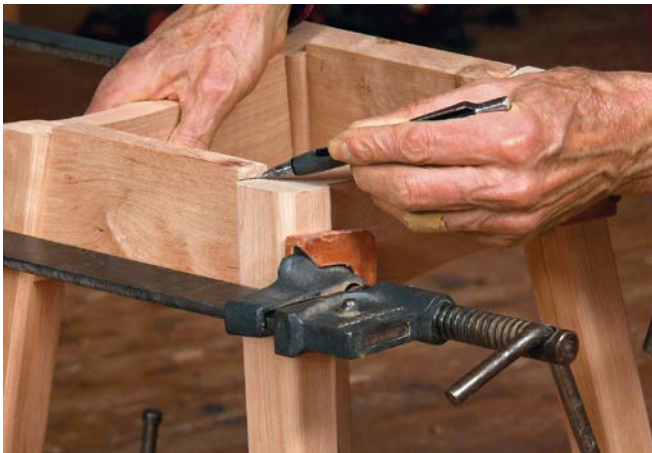
Dry-fit and draw a line. With the side rails and rungs dry-assembled, mark the side rails where they protrude above the leg. Then disassemble and trim to the line at the bandsaw or tablesaw.
