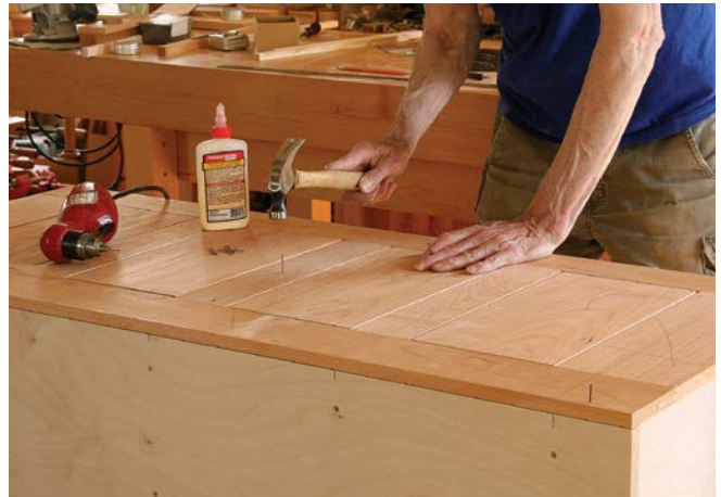
Beautify the back. With the drawer fitting finished, Becksvoort glues the solid cherry frame-and-panel back to the cabinet.
