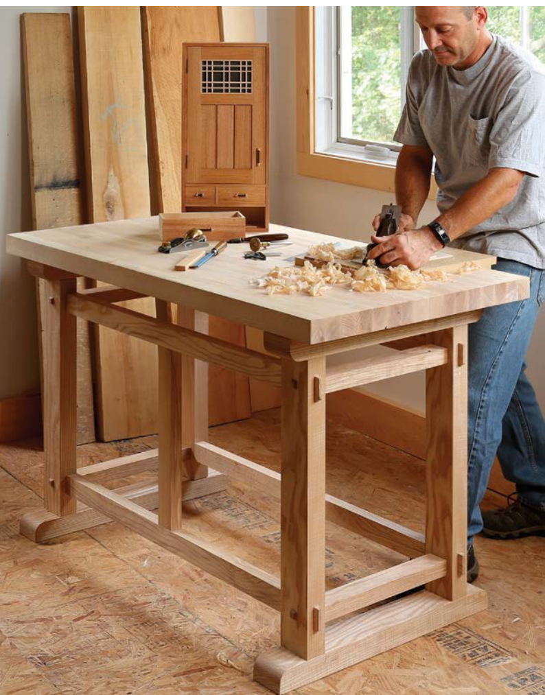
All in the joints. Compact design gets its strength and rigidity from clever interlocking joinery.
