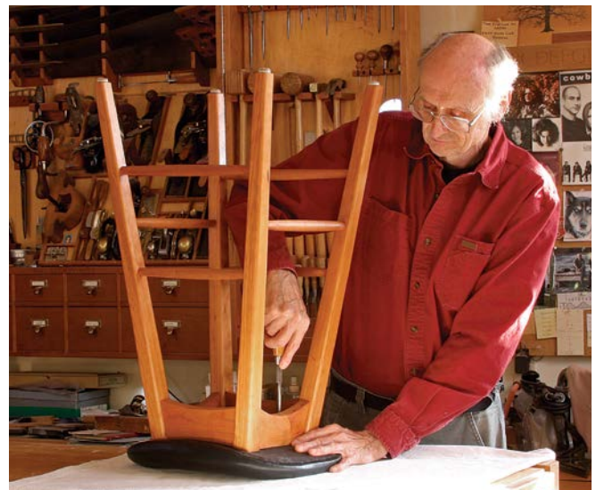
Done. When the seat is upholstered, drive screws through the screw blocks to attach it to the stool's base.
