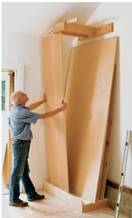
Take your pick. The restraining bars let you leaf through the stack to find a sheet and remove it easily without removing others.
