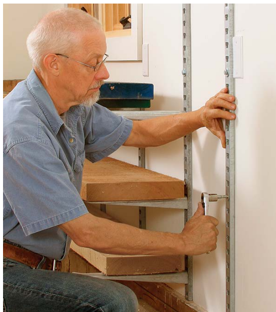
Rock-solid lumber rack. A heavy-gauge steel rack, mounted to the wall studs with lag screws, can hold several hundred pounds of lumber. These brackets and standards are sold individually at leevalley.com .
