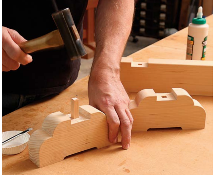
Pare the pegs. Using a knife, Cullum chamfers the ends of the floating tenons (above) to be sure they enter their mortises cleanly. He begins the assembly by gluing the pegs into the feet (right).
