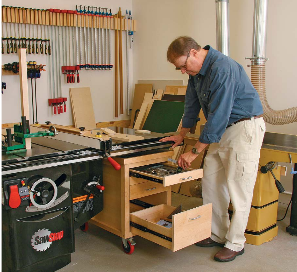
Storage tailored to the tablesaw. O'Brien's tablesaw cart, which holds measuring tools, jigs, and saw accessories, slips beneath the side extension table and keeps saw supplies within easy reach.
