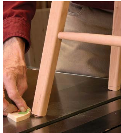
Wobble check. To eliminate rocking, trim all four legs in the same plane. Holding the stool steady on a flat surface, trace around each foot with a pencil held on its side and elevated on a scrap. Cut to the lines on the bandsaw, and follow up with rasps and files.
