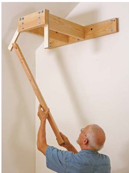
Safe storage for sheet goods. The restraining bars lift out of the way for loading. A lipped platform secures the sheets at the bottom.
