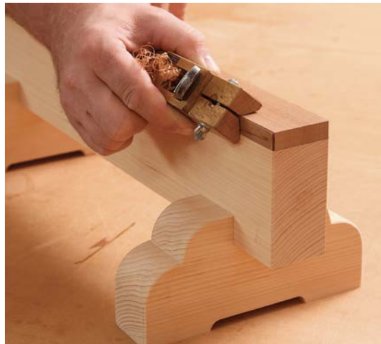
No clamps. After he drives the joints home with a hammer (left), Cullum will place weights on the beam while the glue sets. To protect the beam—and his workpieces—Cullum adds a sacrificial cap piece to the beam, adhering it with double-sided tape. He uses a Japanese chamfer plane to produce just the right finishing touch on the edges (above).
