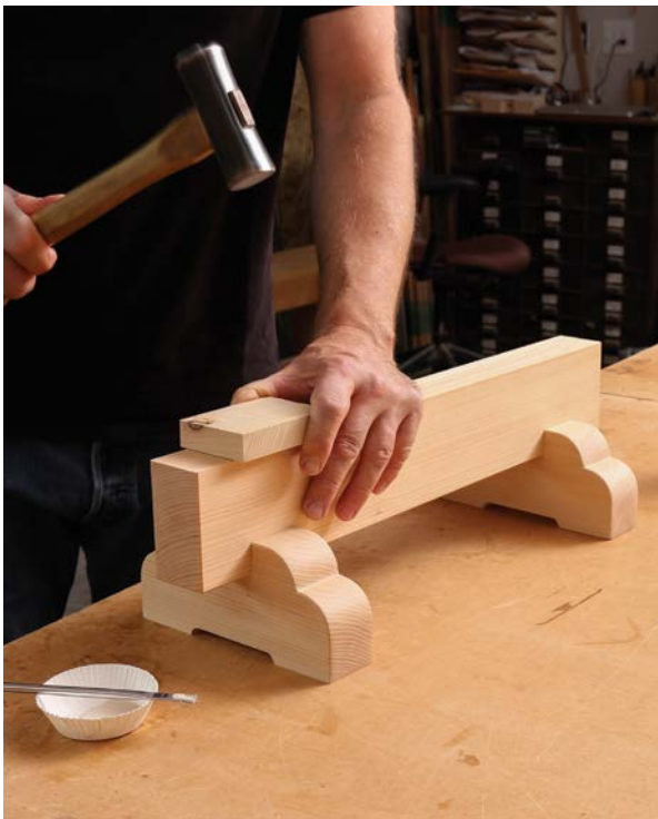
No clamps. After he drives the joints home with a hammer (left), Cullum will place weights on the beam while the glue sets. To protect the beam—and his workpieces—Cullum adds a sacrificial cap piece to the beam, adhering it with double-sided tape. He uses a Japanese chamfer plane to produce just the right finishing touch on the edges (above).
