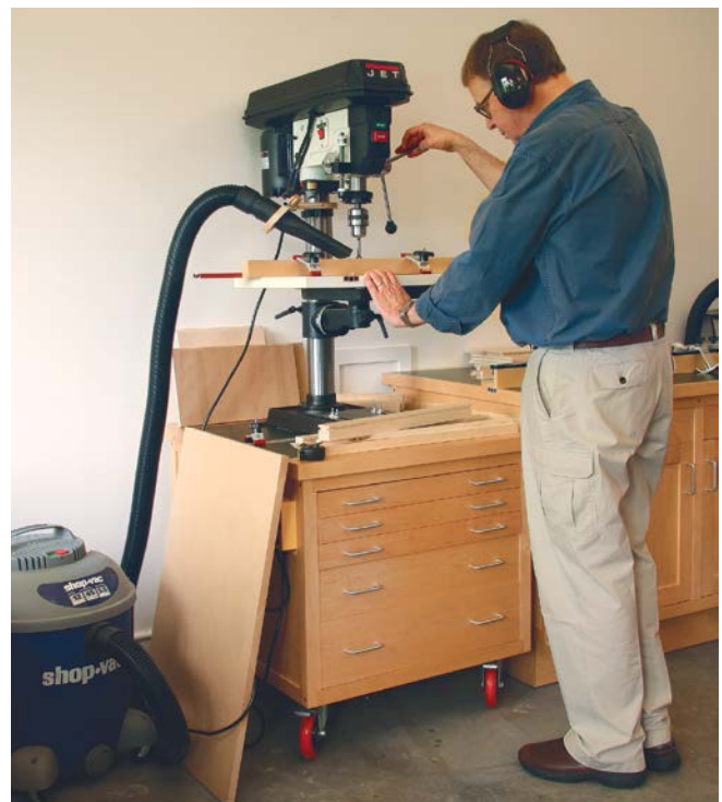
Drill-press cart. The cabinet height is low enough to keep the drill press's base from interfering with long boards being cut on the adjacent miter saw table.
