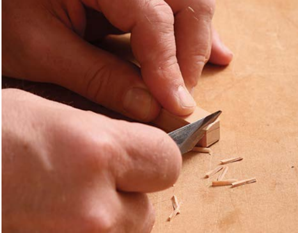
Pare the pegs. Using a knife, Cullum chamfers the ends of the floating tenons (above) to be sure they enter their mortises cleanly. He begins the assembly by gluing the pegs into the feet (right).
