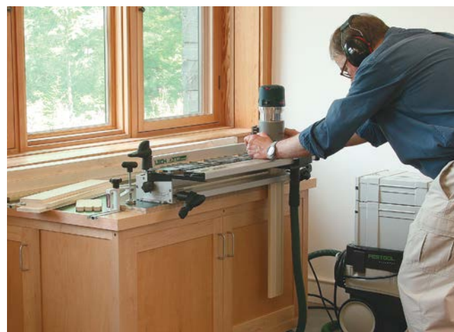
Custom cart for a dovetail jig. O'Brien sized the lower drawer in this cart to fit his Leigh dovetail jig (top), which clamps into the T-tracks on top (bottom). The other drawers contain routers, clamps, bits, and wrenches.
