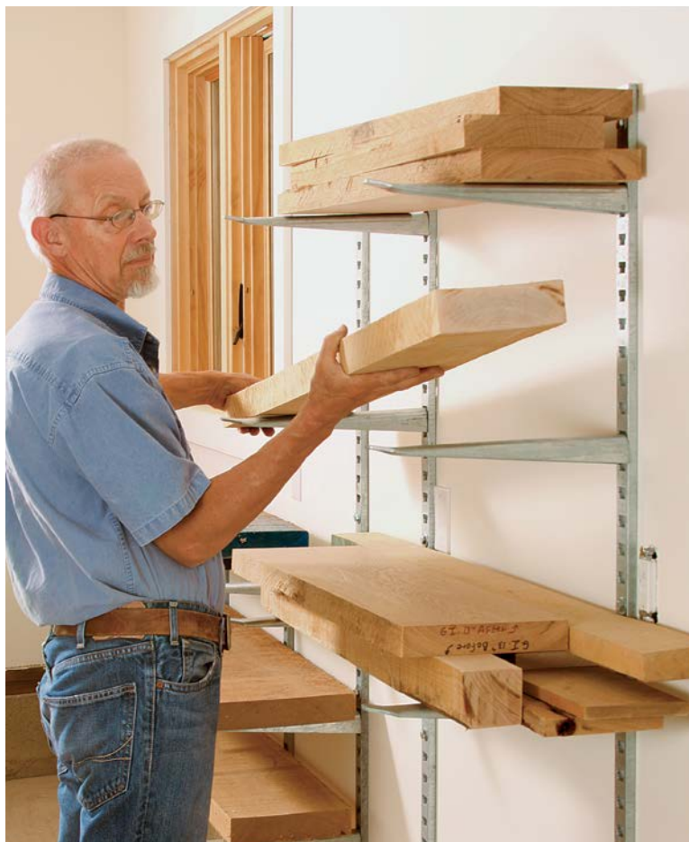
Take your pick. The restraining bars let you leaf through the stack to find a sheet and remove it easily without removing others.
