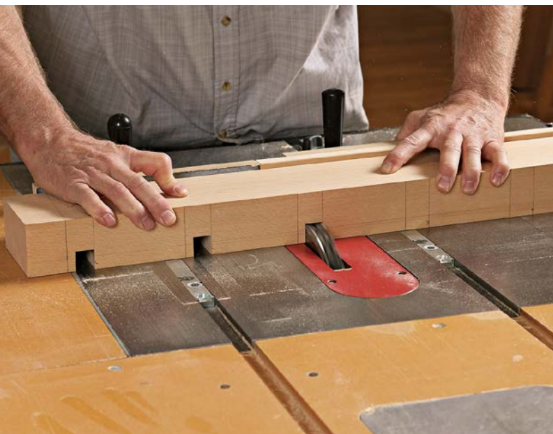
Cut angled dados for the benchdog holes. Use a dado head and a miter gauge to remove most of the waste from the dog holes.
