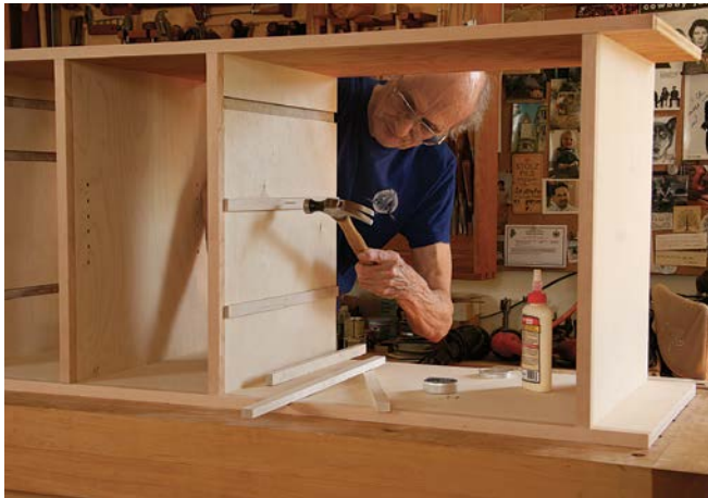
Fix the runners. Becksvoort glues in the maple runners, using brads instead of clamps to hold them in place.
