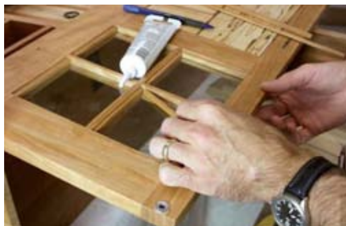
Once everything is finished, install the glass using small strips of cherry ( \frac{1}{8} " and \frac{1}{4} " thick). A few dabs of clear silicone and a couple small pins do the trick.
