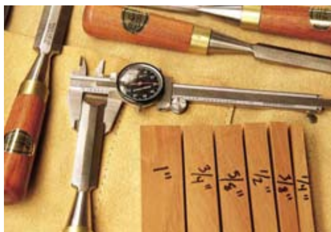
A dial caliper is handy for checking your chisels' dimensions. Measure the width of each blade, add \frac{1}{16} " to each measurement, then rip a scrap piece to that width, which will come in handy during assembly.
