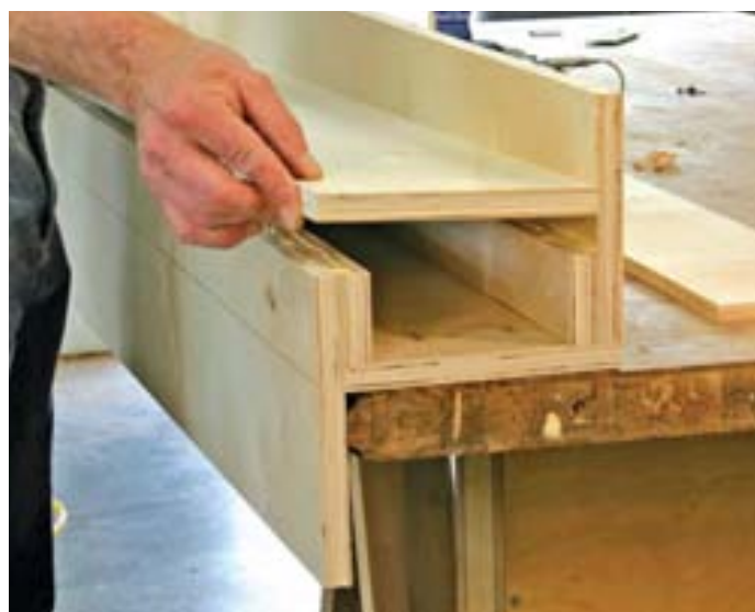
Quick and strong. The box beam construction keeps the fence assembly straight, and the narrow strips of plywood make it easy to put together.
