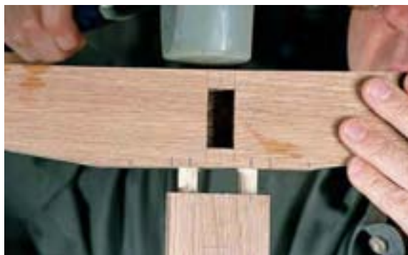
Joining the top stretcher to the top rail and the leg to the top rail on Table 1 requires the dowel placement to straddle the mortise.
