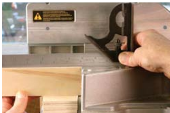
Double check. Checking the width of the strips with a straightedge will help keep the fence beam at the same height as the saw table.
