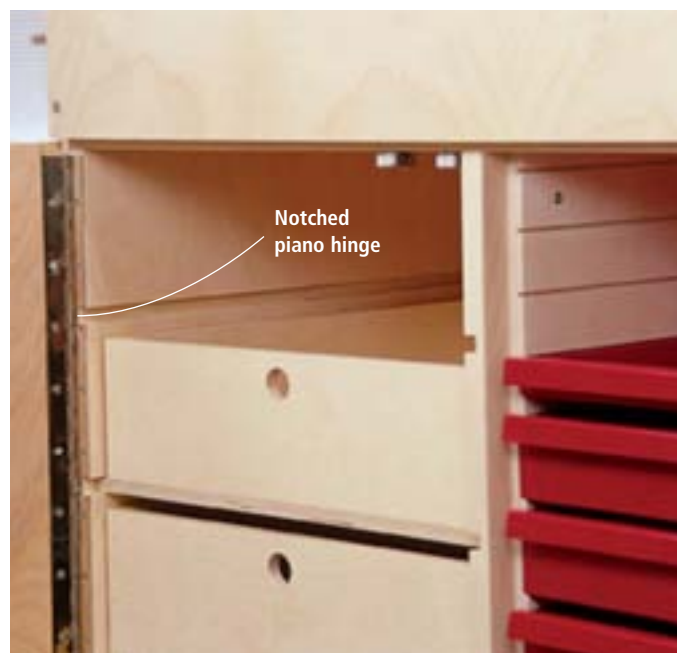
You can see the two sets of dados for the drawers with a few drawers removed. Also, notice the notched piano hinge to allow the drawers to slide in and out.
