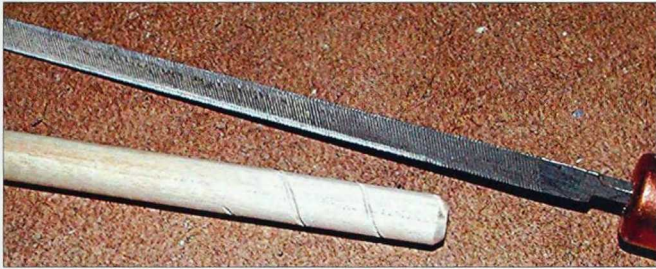
2-150. Save money and custom-cut your own dowels for dowel glue joints.
