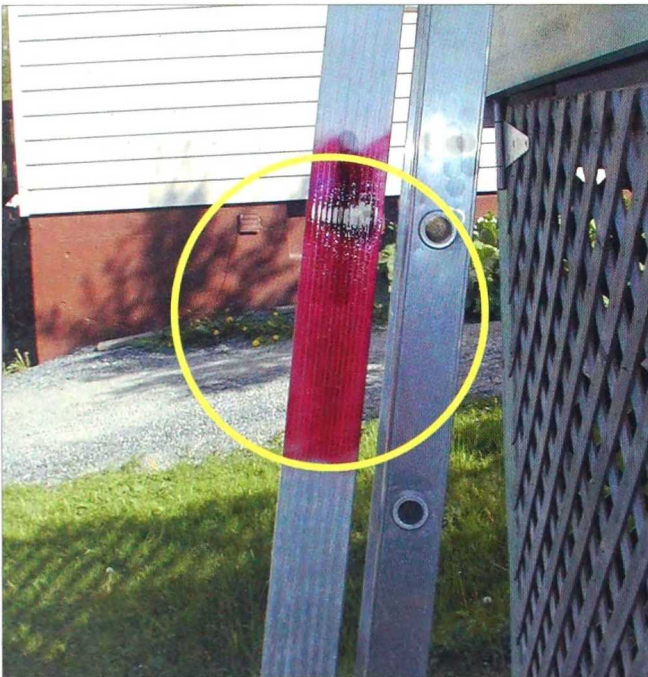
2-194. Paint the balance point of your extension ladder to make carrying it easier.
