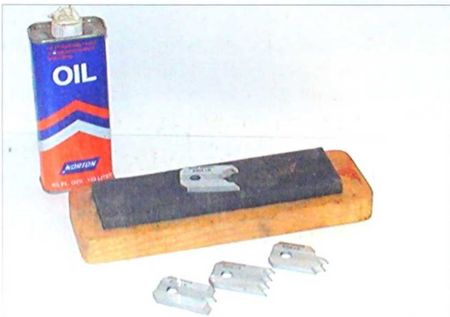
2-417. Always hone only the flat side of shaper blades and be sure that your oilstone is flat.
