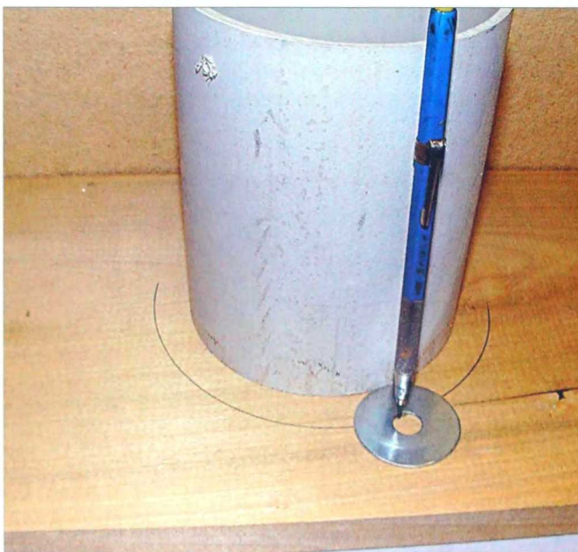
2-306. Enlarging a pattern with a fender washer.
