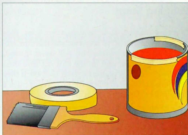
2-290. A bit of masking tape around the rim of a paint can will stop the splatter when closing it.
