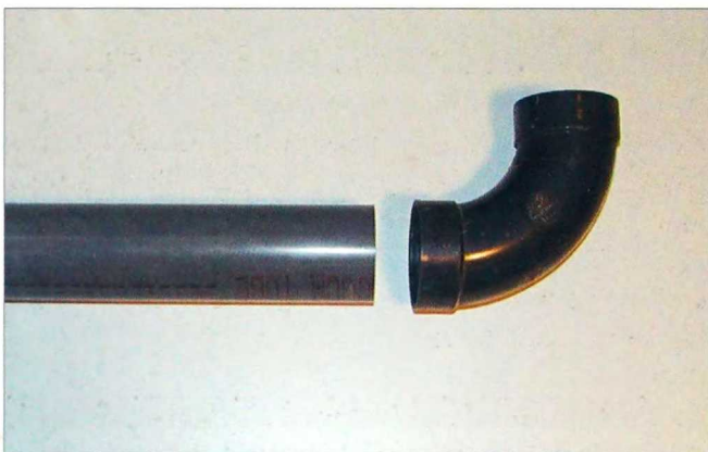
2-371. Do not use glue with these types of dust collector fittings. They will fit tightly and then may be opened to remove any blockages.
