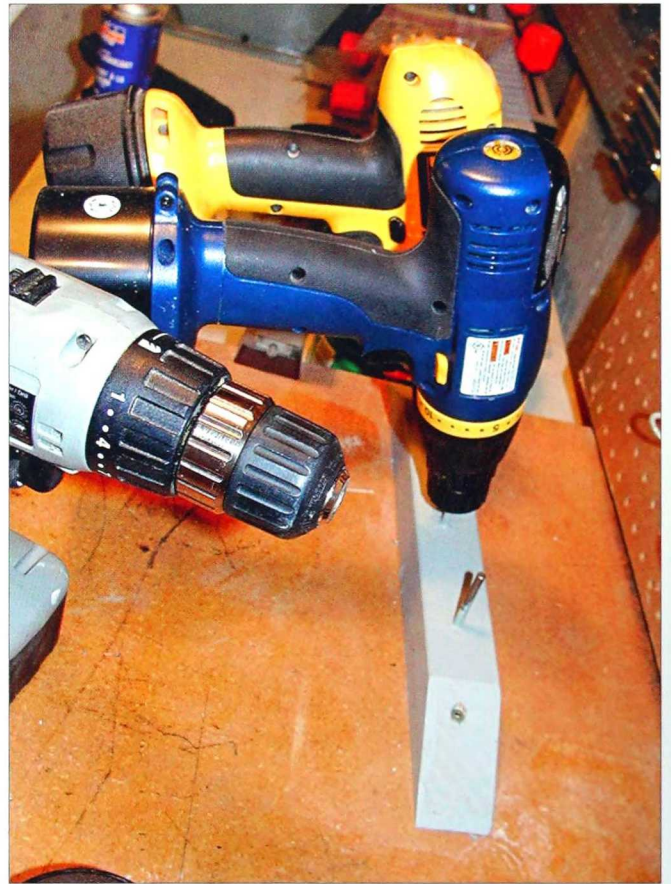
2-173. This shop-made drill "parking" station will keep your portable drills handy.
