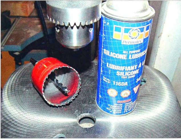
2-232. To facilitate easy release of the wheel from a hole saw, spray the inside with silicone or cooking spray.
