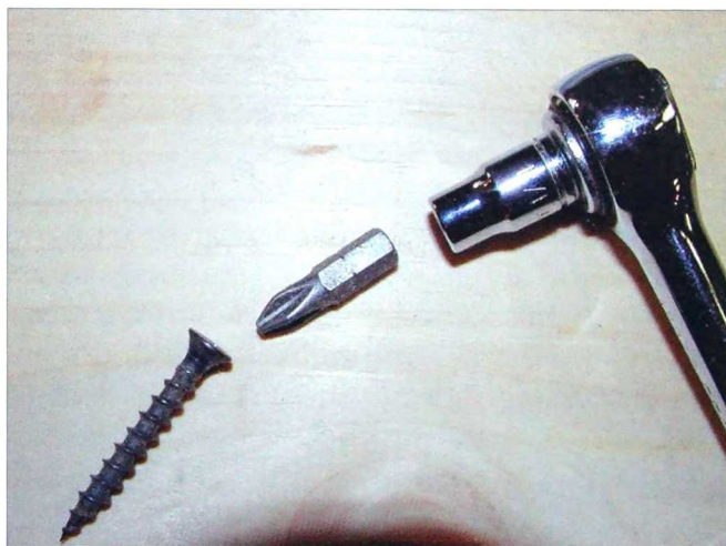
2-395. A socket wrench with a 1/4-inch socket will hold a screwdriver bit for placing screws in a restricted area.
