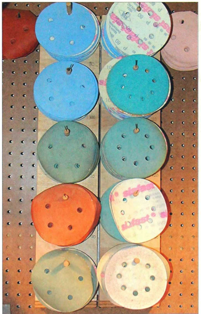
2-9. Storing perforated sanding discs on dowels keeps them in order and makes it easier to find the right grit for the job at hand.
