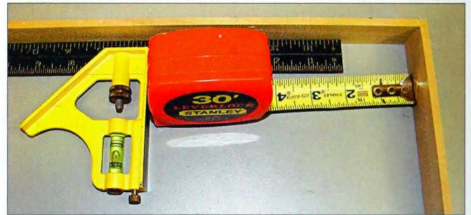
2-458. Using a combination square and a tape measure will give you more accurate inside measurements. The measurement shown is 14 inches.
