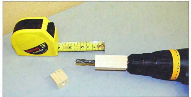
2-170. Cut the 1 x 1 to the required length and put it on your drill bit to use as a depth gauge for repeated holes.
