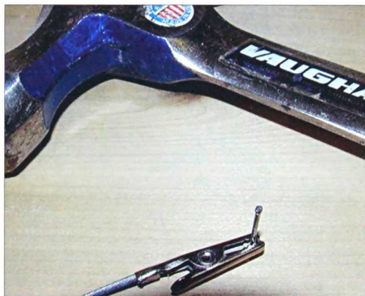
2-274. Alligator clips to hold small nails will save your thumbs.
