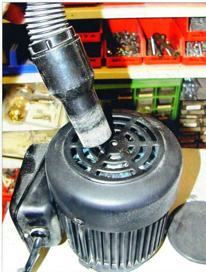
2-516. A regular vacuuming of your shop is a safety factor. Regular vacuuming of your tools and their motors will prolong their lives.
