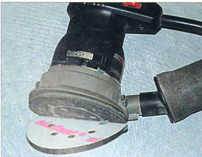
2-5. Hook-and-loop sanding discs can be reused more readily than adhesive-backed discs.
