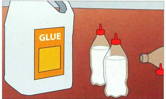
2-32. A soda bottle is just the right size for small glue-up jobs if you put a caulking tube tip through the bottle cap.
