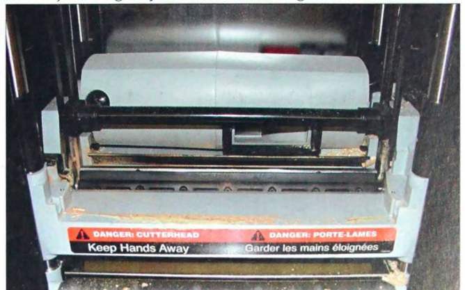
2-462. Moving only one knife slightly on a thickness planer will correct a nick in a knife.
