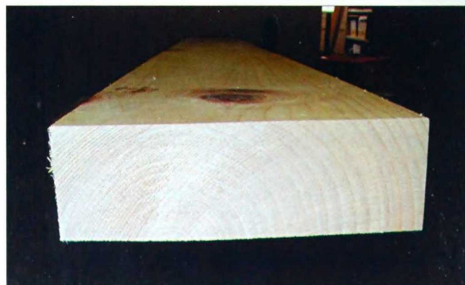
Lumber that is being air-dried. Notice that its annual rings arch upward, to prevent cupping and warping.
