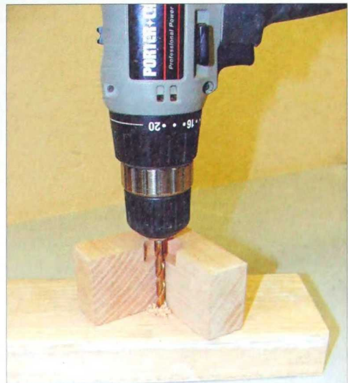
2-170. Cut the 1 x 1 to the required length and put it on your drill bit to use as a depth gauge for repeated holes.
