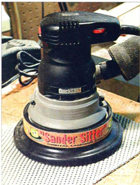
2-339. This Sander Sitter allows you to set your sander down while it is still running and cleans the sanding disc at the same time.
