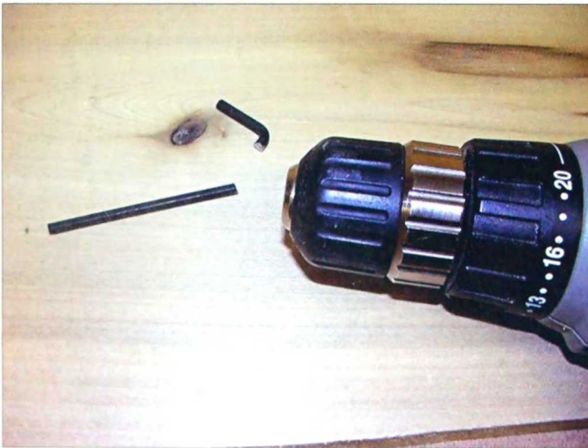
2-41. A straight Allen key can be chucked into a drill for more torque.
