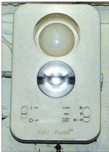
1-13. This strobe light flasher will alert you in a noisy workshop.
