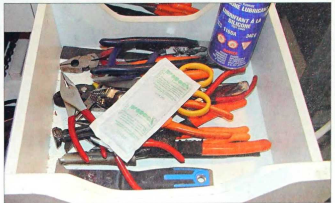
2-359. Silica gel packs placed in your tool drawers will absorb moisture and help prevent rust. Spraying your tool drawers with silicone will also prevent the tools from rusting.
