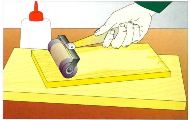
2-212. A printer's brayer can be used to spread white glue on larger surfaces.
