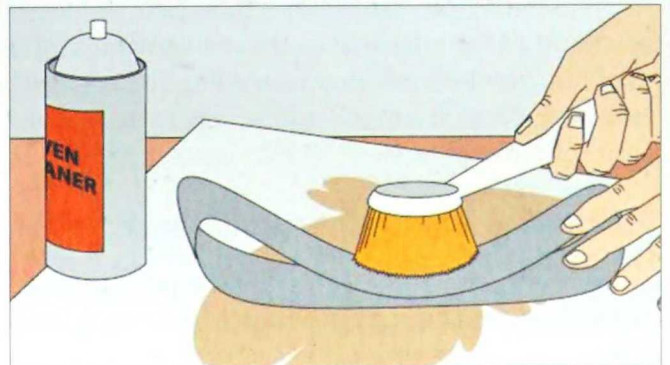
2-12. Oven cleaner will dress up an old sanding belt.
