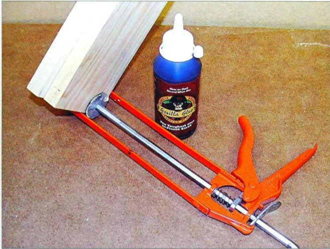
2-124. A caulking gun can be used in an emergency as a makeshift clamp.
