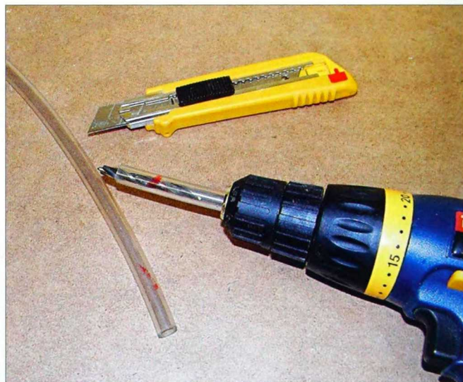
2-167. Neoprene tubing makes an efficient depth stop for your drill.
