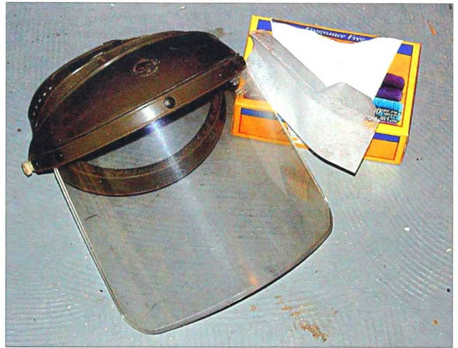
2-382. One way to control sawdust buildup on safety glasses is to wipe them occasionally with a used sheet of fabric softener.
