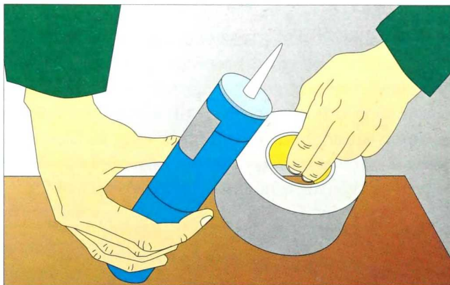
2-99. Wrapping duct tape around the caulk tube.
