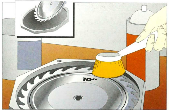
2-112. One method of cleaning circular saw blades is to spray on oven cleaner and to brush the blades clean. The inset shows one of many types of circular saw containers.
