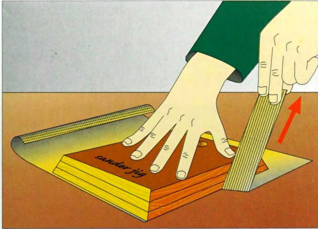
2-11. Using these jigs will simplify the cutting of sandpaper for your one-quarter-, one-third-, or one-half-sheet orbital power sanders.
