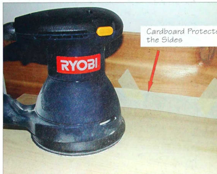
2-364. Cardboard taped to the vertical sides of the workpiece will prevent the sander from marking it.
