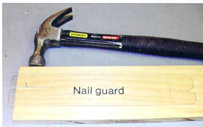
2-272. A shop-made Plexiglas nail guard will protect the surface of the workpiece from hammer marks.
