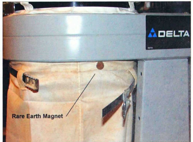
2-376. Rare earth magnets help in replacing the dust-collection bag.
