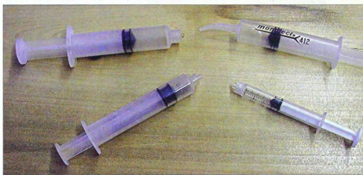
2-26. Syringes of various types are excellent tools for applying glue in tight spaces.
