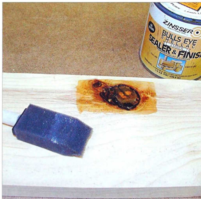
2-501. A coat or two of shellac will prevent knots from bleeding through the finish.
