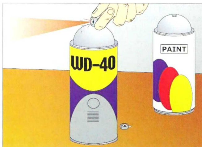
2-285. WD-40 lubricant will clean your paint-can nozzle. Replace it on the paint can for later use.
