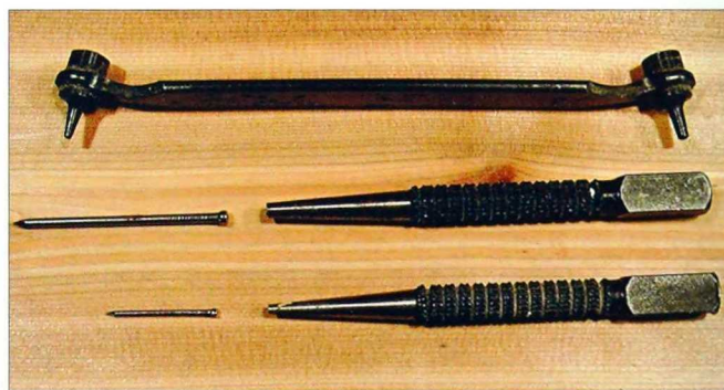
2-273. The nail set at the top of the photo is for setting nails in cramped quarters. The middle tool is for finishing nails of 2 inches or larger. The lower nail set is used for 1 1/2-inch nails or smaller.
