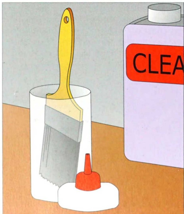
2-282. An old plastic glue bottle with its top cut off makes an ideal paintbrush-cleaning container.
