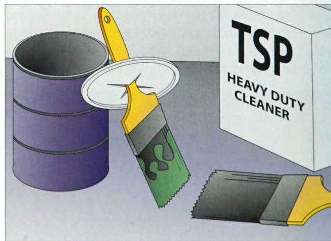
2-283. Trisodium phosphate (TSP) mixed with water is a less-expensive way of cleaning old paintbrushes.
