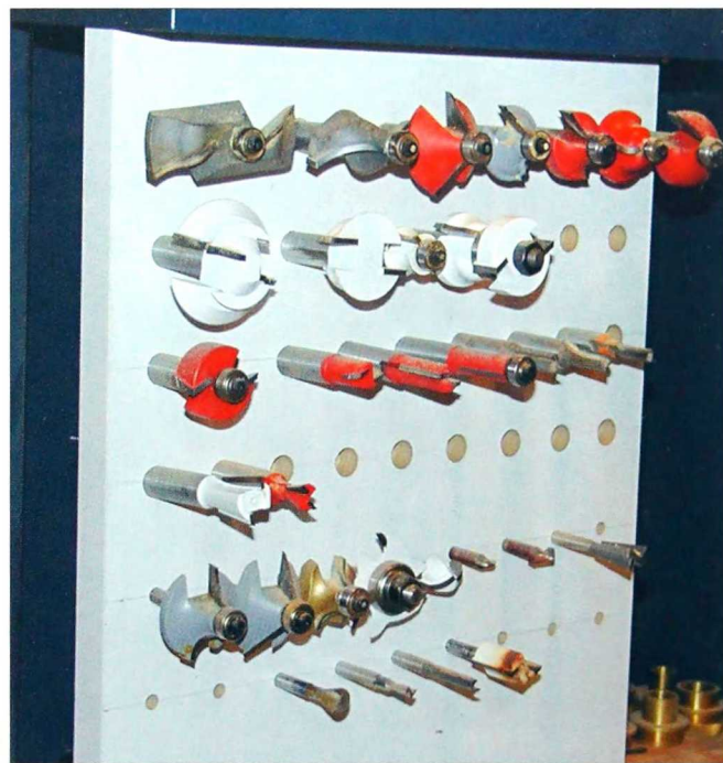
2-355. Router bit edges are quite fragile. This storage panel keeps the bits apart and safe from damage.
