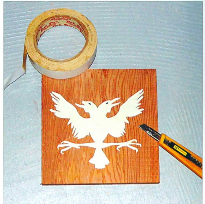
2-307. Cut your pattern with a utility knife or scissors and then trace the pattern on your workpiece with a sharp pencil.
