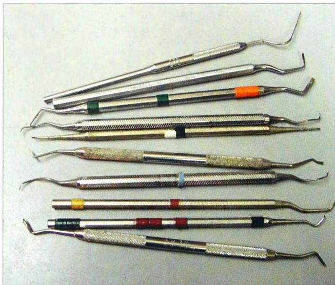
2-27. These various-shaped dental picks can remove dried glue squeeze-out and even apply wood filler in some spaces.
