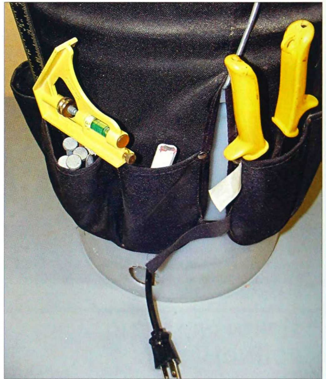
2-464. An extension cord coiled in the bottom of a bucket tool kit will add to the convenience.
