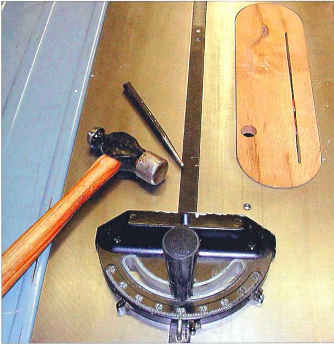
2-447. Peening dimples in a miter gauge will take out any play in it.
