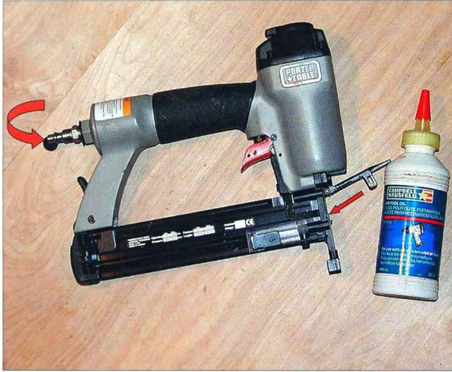
2-40. Check the jamb release for excessive wear and add some oil to the moving parts.
