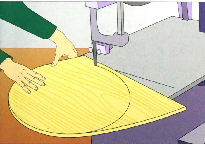
2-54. This way of cutting rounded corners on a band saw is difficult.
