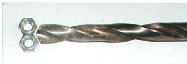
2-166. You can use a couple of hex nuts to determine whether the tip of a high-speed-steel drill bit is at the correct angle.
