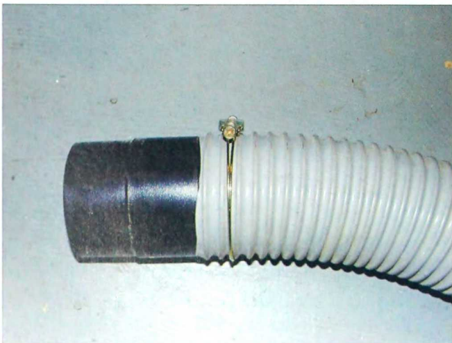
2-372. Flexible hoses allow easy access for the removal of sawdust blockages.
