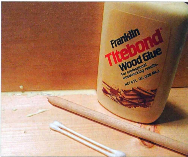
2-211. A sharpened dowel and some moistened Q-Tips will remove excess glue.
