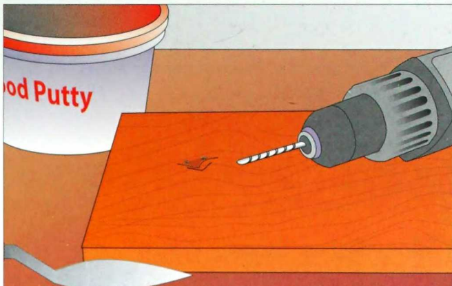
2-495. Drilling a couple of shallow holes in the dents will allow the wood filler to grab hold.
