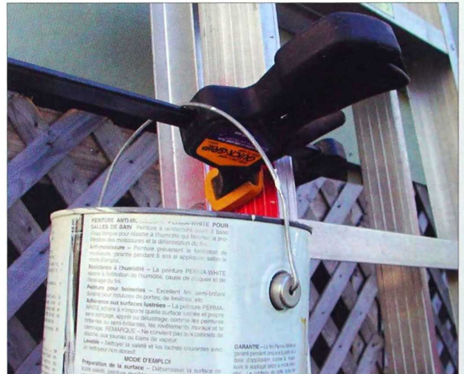
2-196. Squeeze-type bar clamps will hold that gallon can of paint on your ladder.
