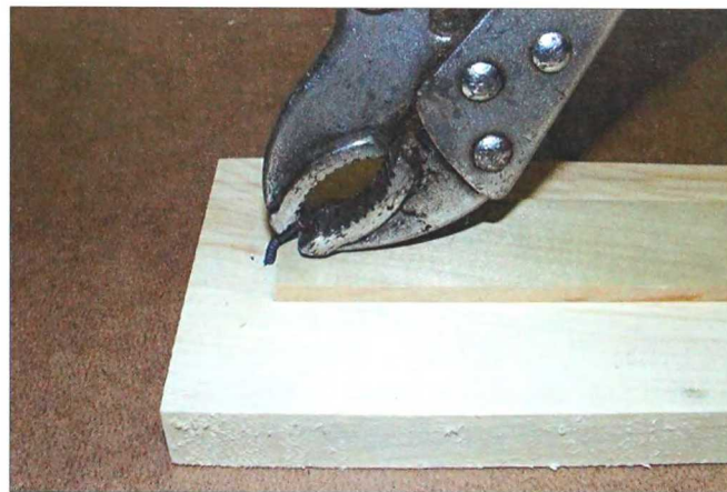
2-276. Vise-Grips will make pulling ring or spiral nails easier.
