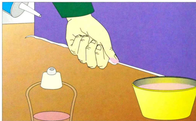
2-95. Dip your thumb frequently into a dish of detergent liquid when applying caulk in corners.
