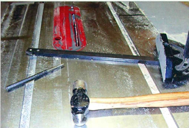
2-263. Peening the bar of a miter gauge makes it fit tighter in the saw table slot.
