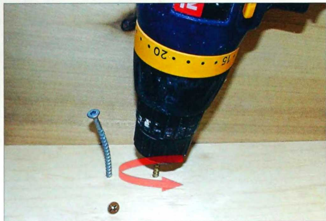
2-401. Damaged screws can be removed by putting your drill chuck on them, tightening them up, and then putting your drill in reverse.
