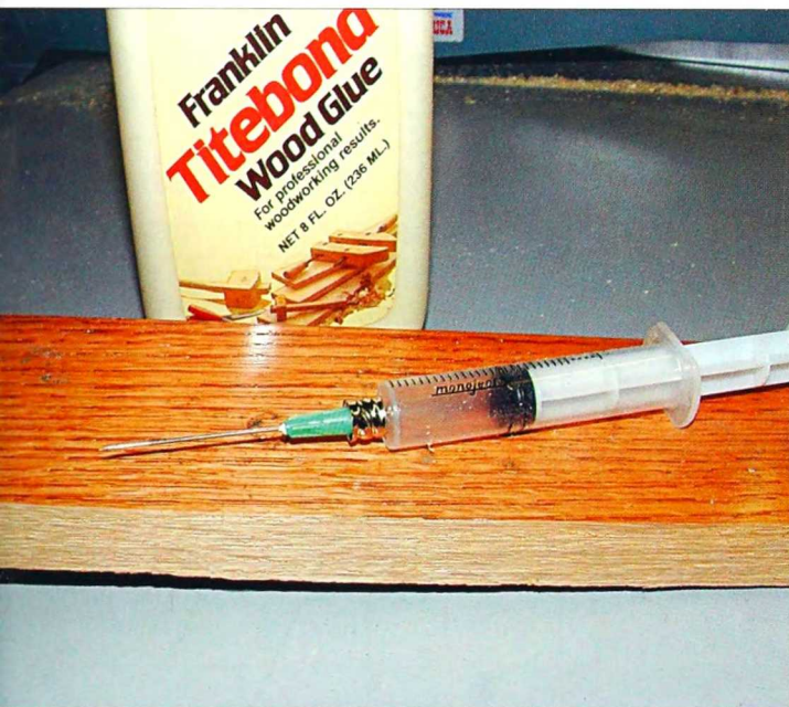
2-484. To eliminate a bubble on veneer, inject a few drops of carpenter's glue into the bubble.
