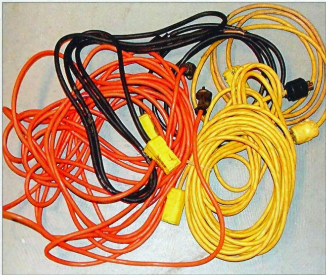
2-192. Make sure that you select an extension cord of the proper length of gauge.
