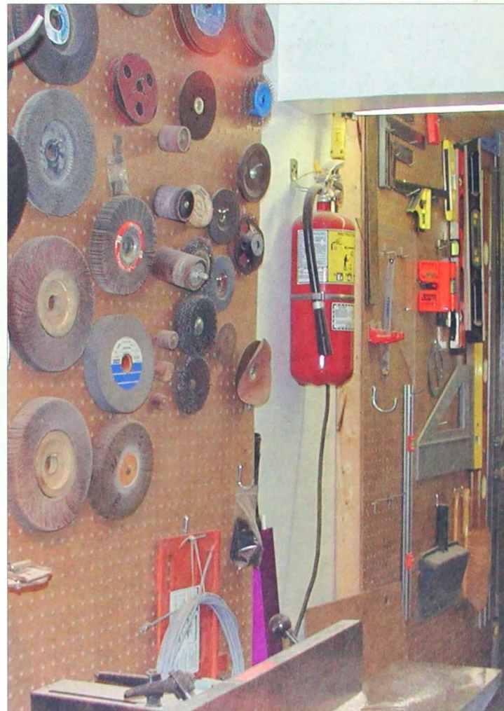
1-12. Pegboard walls are an effective way of storing tools.
