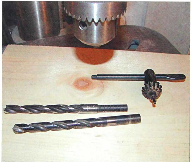
2-186. Tightening all three holes in the chuck will prevent scraping and slipping of the drill bit.
