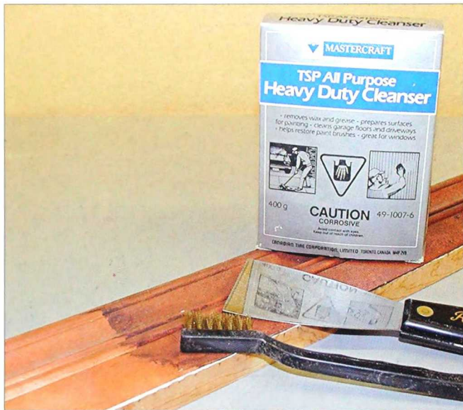
2-299. Trisodium phosphate (TSP) is an inexpensive substitute for commercial paint removers.
