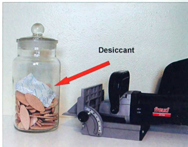
2-90. Keep a pack of desiccant in a sealed jar with your biscuits.
