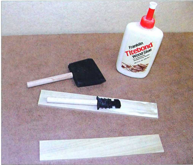
2-34. The flexible plastic insert in an old foam paintbrush makes an excellent glue spreader.
