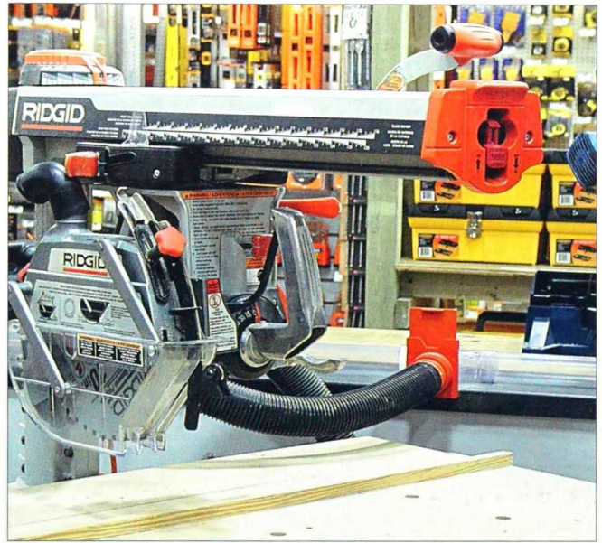
2-329. The radial arm saw is a very versatile power tool. It can be used to cut boards to length, make rip cuts, and for mitering and dadoing.
