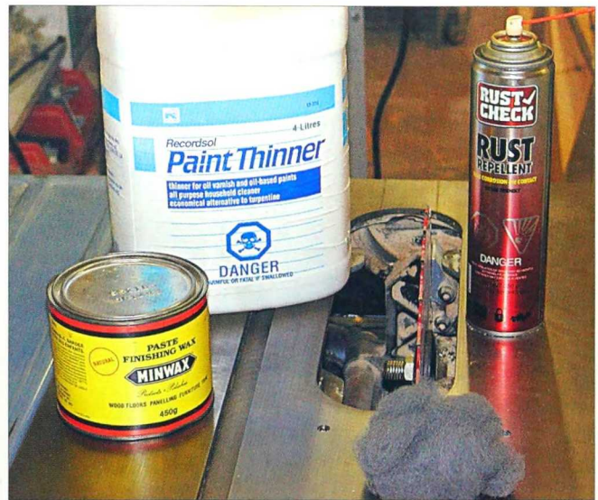
Paint thinner can be used to clean the top surface of a table-saw table every six months.
