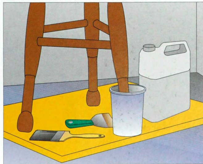
2-342. Placing plastic containers under the legs of your refinishing project will allow you to collect the stripper drippings and reuse them.
