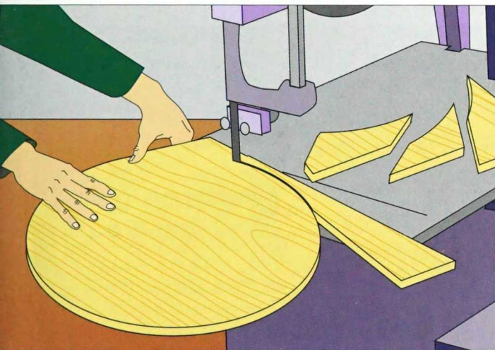
2-55. The easiest and best way to saw rounded corners is to nibble away at each curve.
