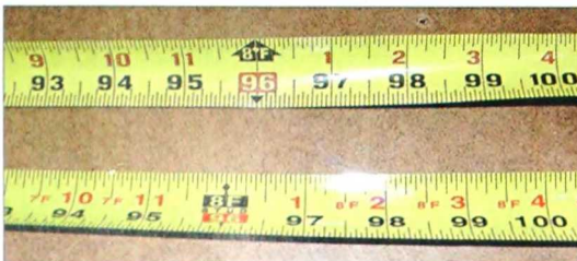
2-457. Use the same tape measure to transfer dimensions.
