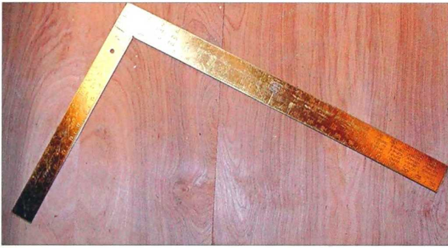
2-435. The builder's square has etched scales and data on it.
