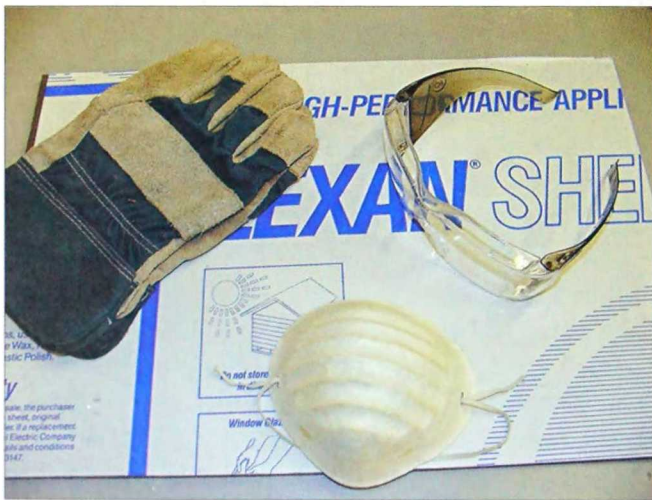
2-318. Some of the safety gear that should be used whenever plastics are being worked with.
