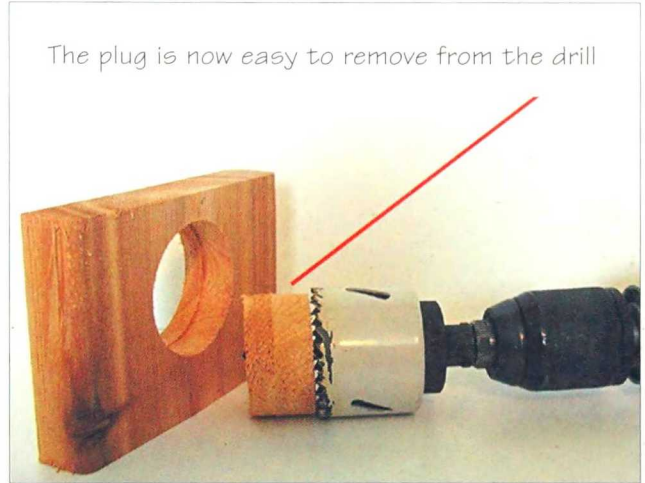
2-235. The plug will drop out of the hole saw quite easily.
