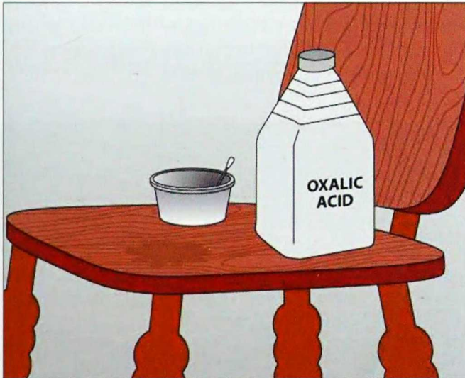
2-489. Oxalic acid will remove stains from finished wood.
