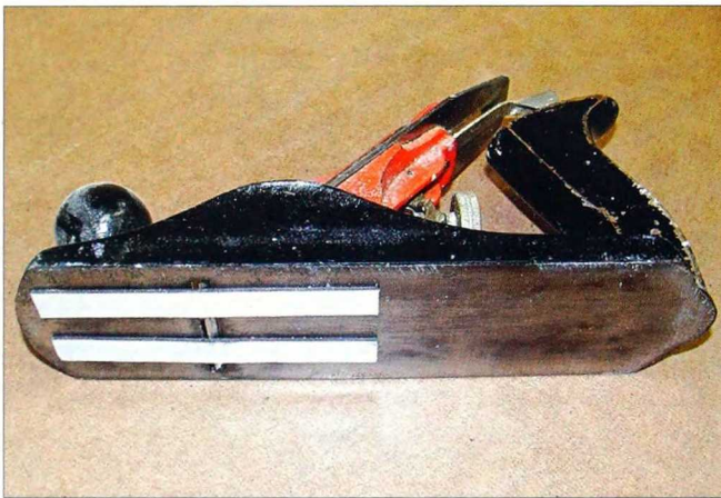
2-223. Plastic refrigerator magnets will protect hand-plane blades.
