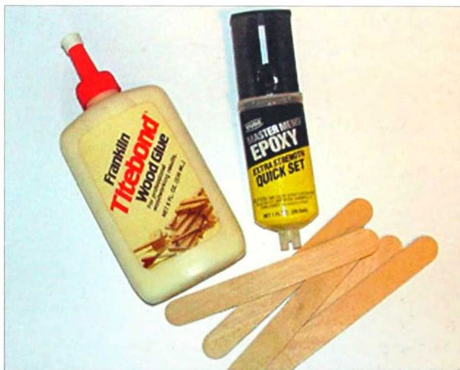
2-25. Tongue depressors are useful for mixing two-part epoxy and for spreading glue.
