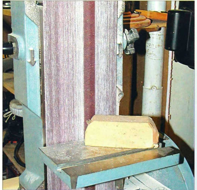
2-6. The crepe rubber block cleans this sanding belt and will more than double the life of abrasives on all types of sanders.
