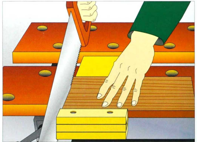
2-506. The bench hook is an extremely handy jig for square-cutting, planing, or carving.
