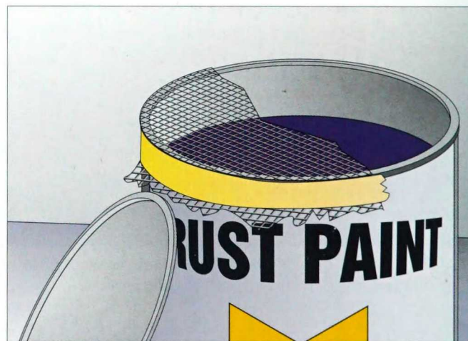
2-288. This piece of nylon window screening, taped to the can, can be used to filter paint.
