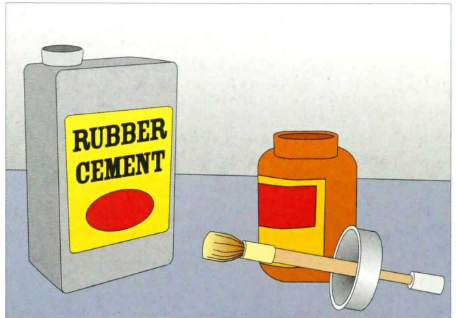
2-358. Rubber cement works well for sticking paper patterns on wood surfaces.
