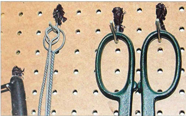
2-312. To keep the hooks on pegboard secure, apply a little dab of hot-melt glue.
