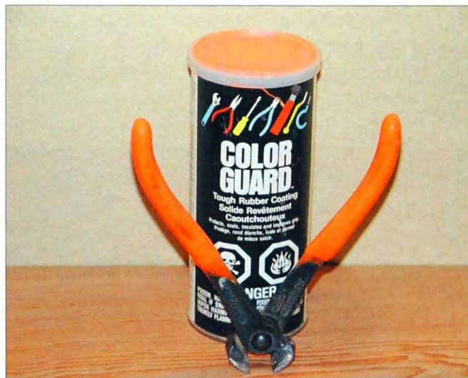
2-221. Color Guard can also be used to mend the handles of tools.
