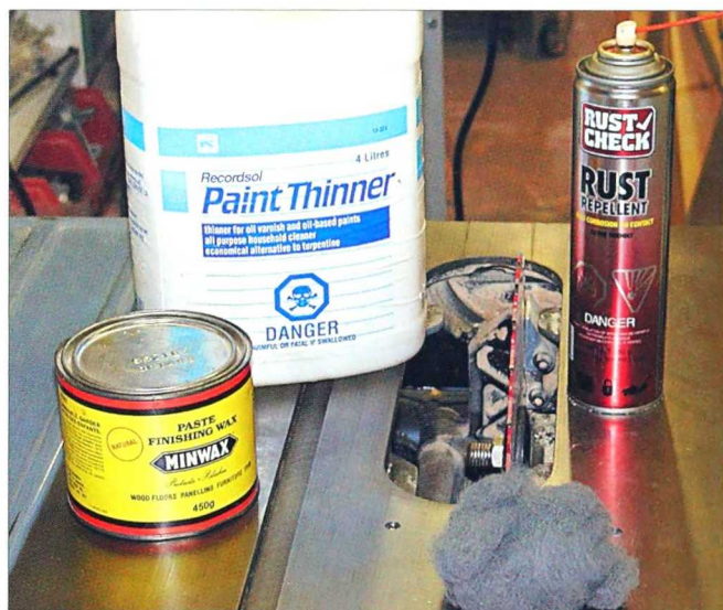
2-451. Clean the top surface of a saw table every six months with paint thinner or WD40 oil and very fine steel wool.
