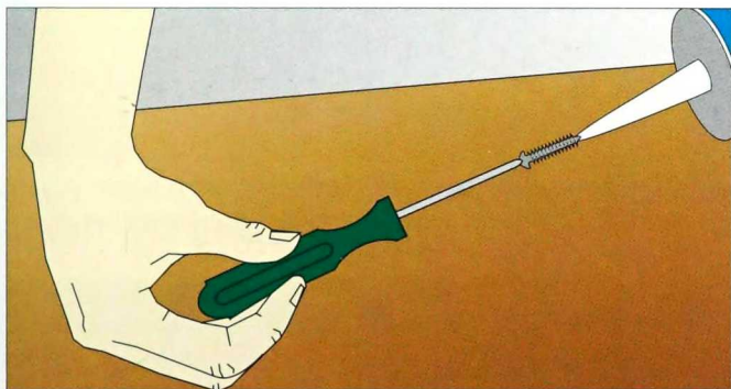
2-97. Screwing a pan-head wood screw into the nozzle of a tube of caulk.
