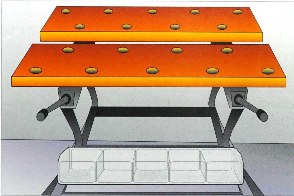
2-513. This nail-bin hanger bracket is riveted to the Workmate with a cross-brace. Storage containers can be hung on it.
