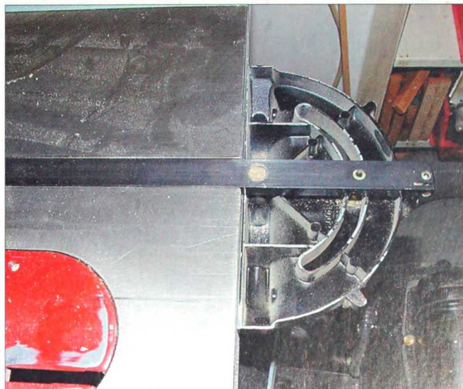
2-443. If you see light between the inverted miter gauge and the table saw edge, the gauge needs to be adjusted.
