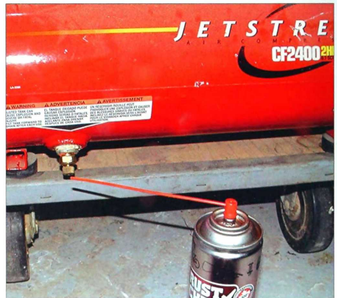
2-36. Adding a rust preventative to the compressor tank can extend its life. Allow it to sit for a day or two and then drain it completely before using the compressor.
