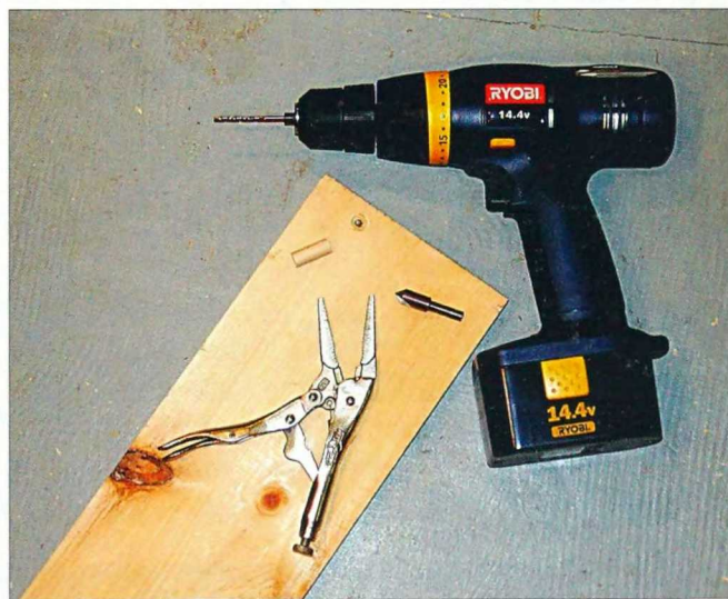
2-402. A broken screw can be repaired with little damage to the finished workpiece.
