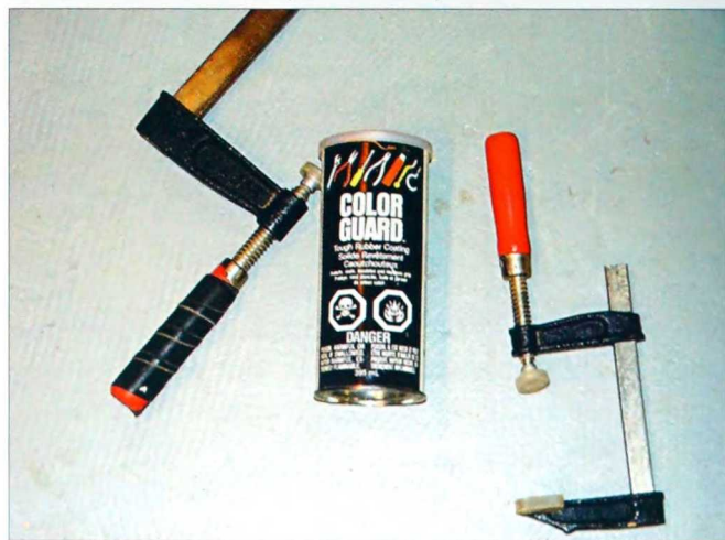
2-84. Color Guard by Locktite has been applied to the bar clamp handles.
