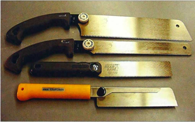
Dozuki saws are saws that cut on the pull stroke. They have thinner steel than traditional backsaws and disposable blades.
