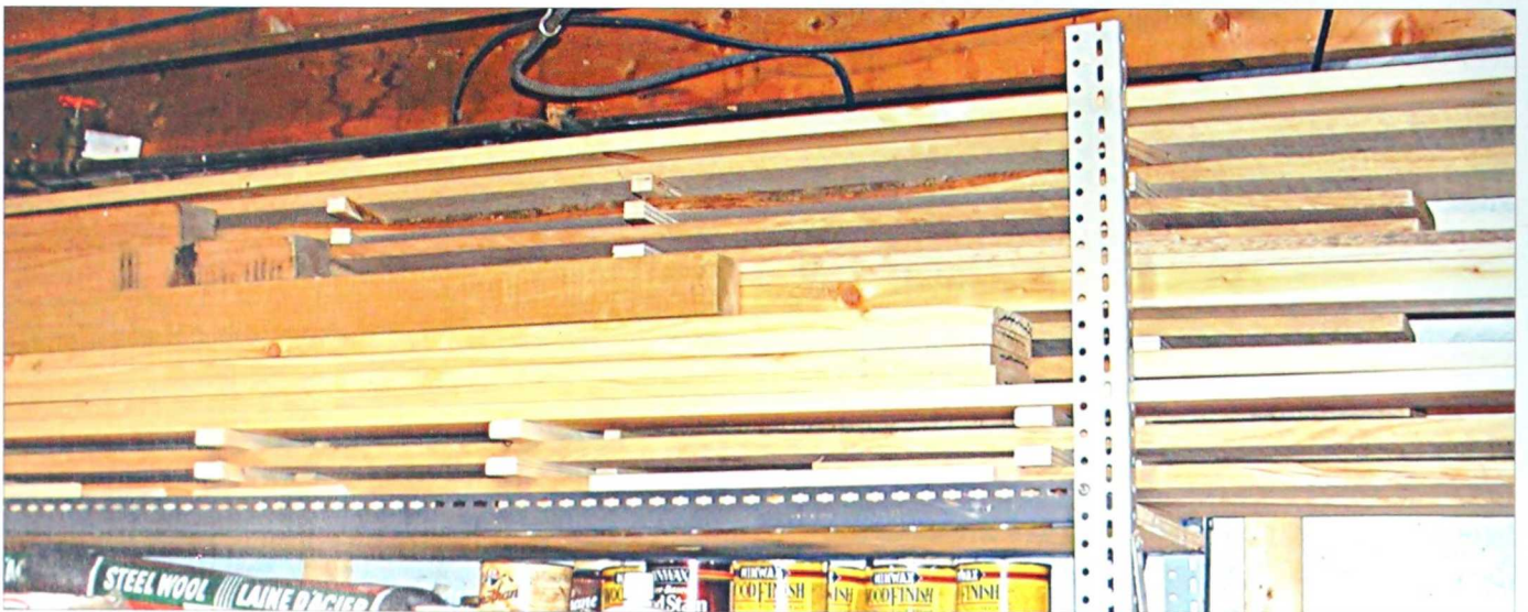
If lumber in the workshop has a moisture content of between 10 and 25 percent, the boards should be stickered; that is, strips of wood should be placed between the boards at two-foot intervals. This allows air to circulate through the boards to quicken the drying process.
