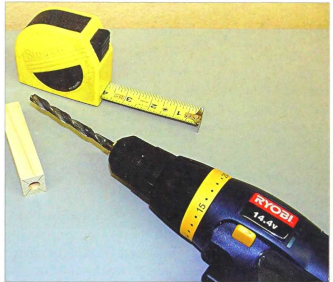
2-169. Bore down the center of a 1 x 1 to make a depth gauge for drilling.
