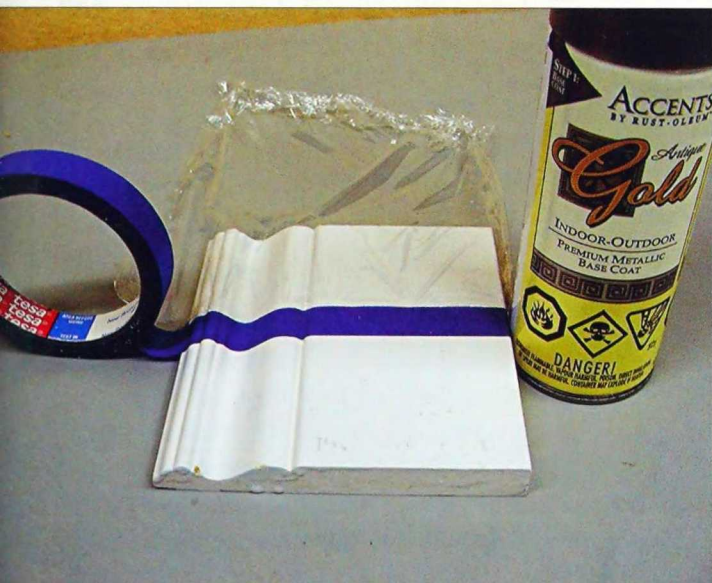
2-503. Plastic wrap makes better masking material than newspaper or brown paper; it molds to odd shapes more readily.
