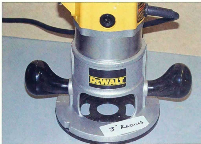
2-352. Write your router base radius on a sticky label.
