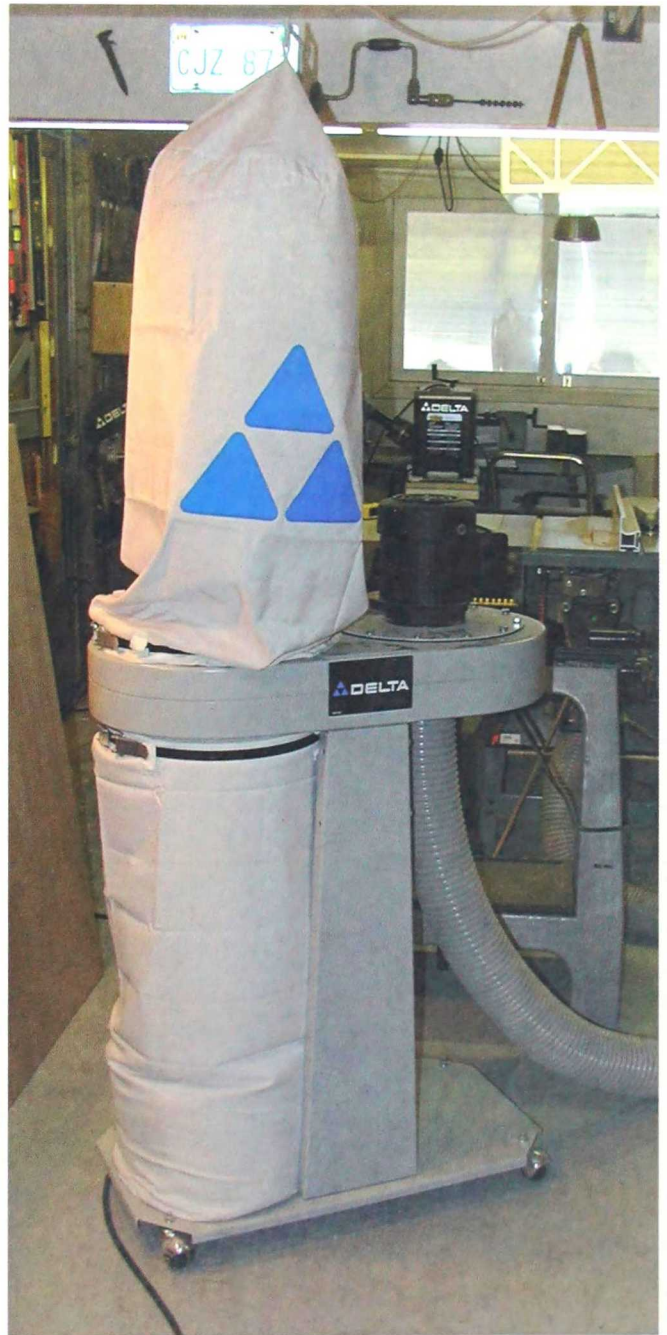
1-8. This two-stage dust collector will control sawdust in most small workshops.
