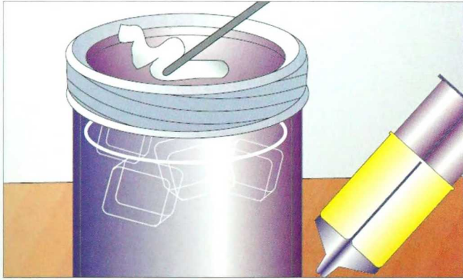
2-191. Mixing epoxy glue on the lid of a jar filled with ice water will help retard its setup time.
