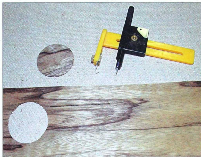
2-133. This circle cutter makes it easy to cut circles in veneer.
