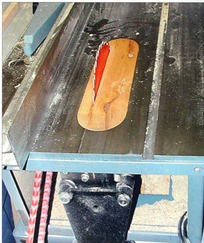
2-452. A piece of 1/4-inch plywood will serve as a temporary zero-clearance jig for your table saw.
