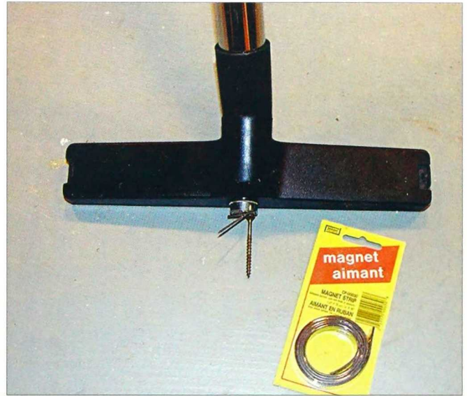
2-466. A strong magnet attached near the bottom of the shop vacuum will pick up nails, screws, etc.
