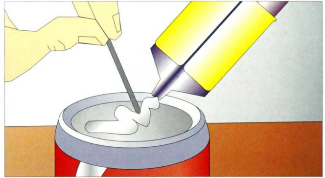
2-190. Use the bottom of an unopened can of soda to mix the hardener and resin for the epoxy glue.
