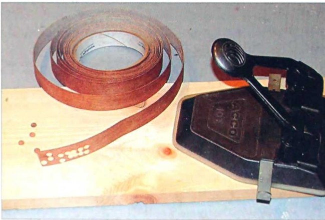
2-404. For smaller screws (#4 or #5), an office hole punch will make clean circles in edge-banding veneer.
