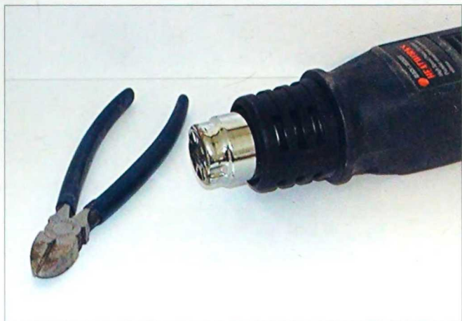
2-220. Mending the handles on cutters with heat-shrink tubing and a heat gun.
