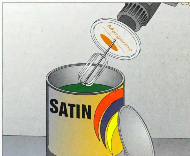
2-291. This old beater makes an effective means of mixing paint
