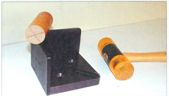
2-153. This Veritas center finder makes it easy to mark dowel centers.
