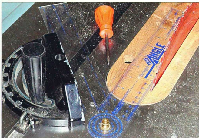
2-441. Use a protractor to align your miter gauge.
