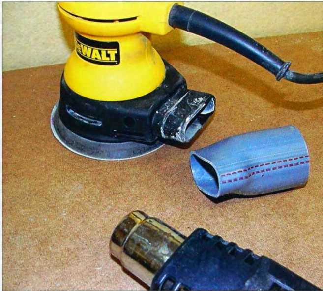
2-374. A heat gun will soften the dust-collection connectors found on most portable tools so that they can connect to a shop vacuum.
