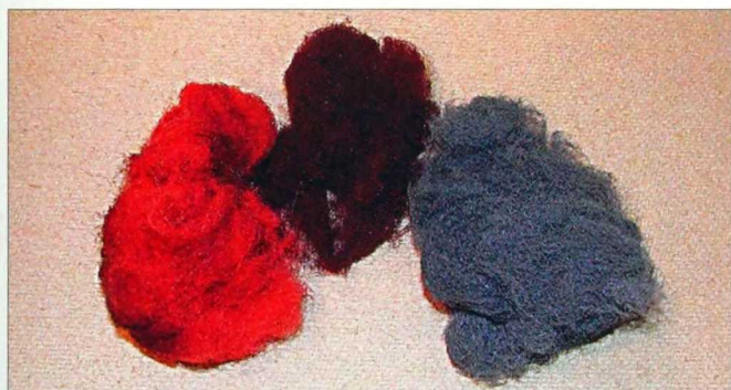
2-20. Steel wool is safe to use with solvent-based finishes. Synthetic wool and abrasives should be used with water-based finishes.
