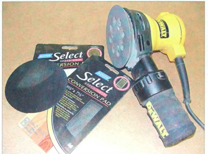
2-3. Replacement pads are available for hook-and-loop sanders.
