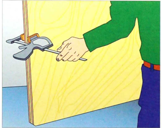
2-324. A squeeze-type clamp can help with toting sheet goods.
