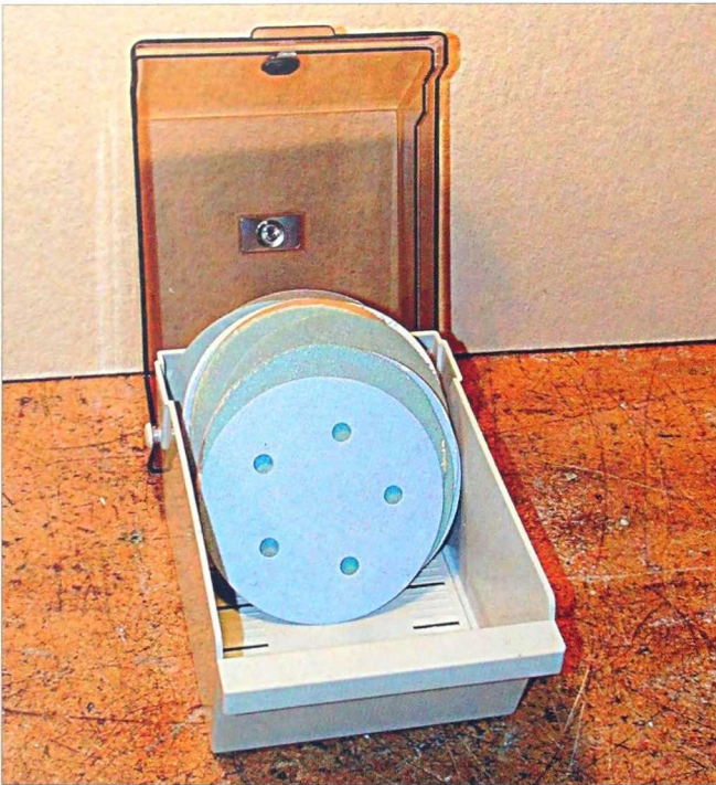
2–10. CD-ROM storage boxes are a convenient way of storing sanding discs.
