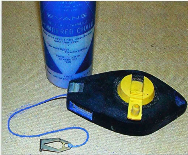
2-104. A typical chalk line and a bottle of powdered chalk.
