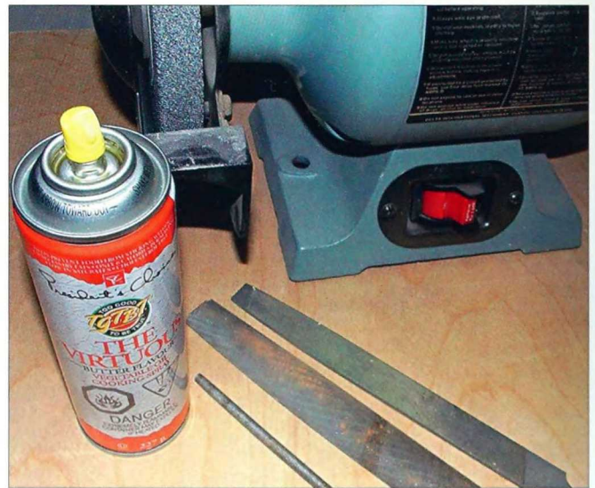
2-42. Spraying your files and grinding wheel with nonstick cooking oil before using them will help prevent the aluminum from sticking to the files and grinding wheel.
