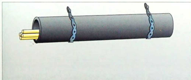
2-158. Keep your dowels in order. Put them in a plastic pipe and use steel strapping to mount the tube on a wall.
