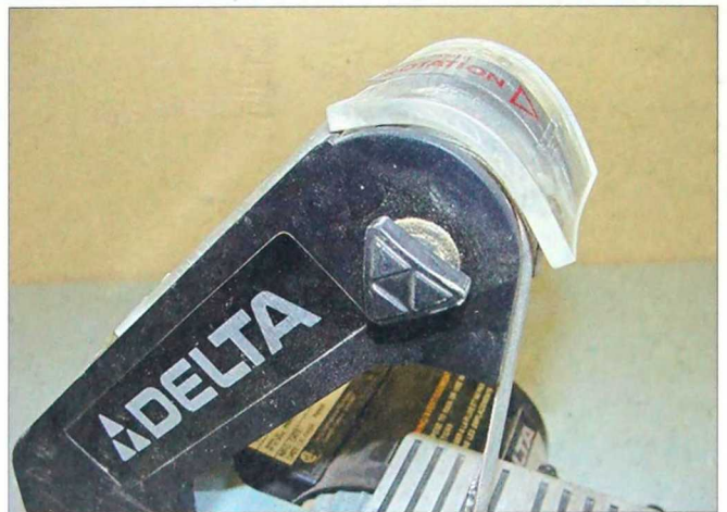
2-87. The shop-made Plexiglas guard will deflect sanding debris on this Delta 1-inch belt sander.
