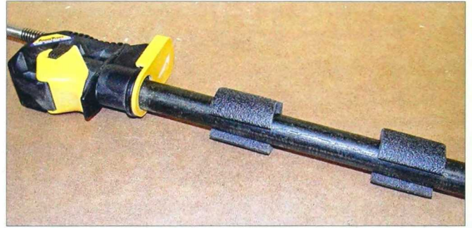
2-126. Foam pipe insulation will protect your workpiece.
