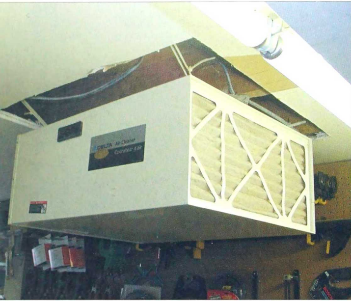
1-9. An air cleaner such as this will rid your home workshop of airborne sawdust.
