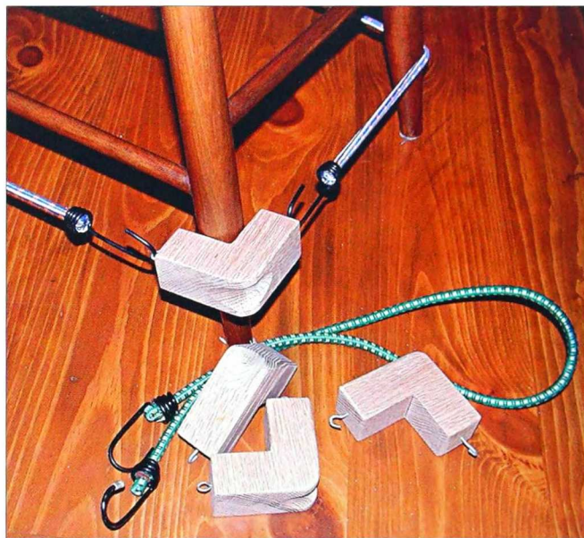
2-129. The bungee cords from your camping gear can be used to make these framing clamps.
