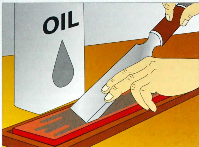
2-226. The correct way of holding a chisel blade for sharpening on a bench stone.
