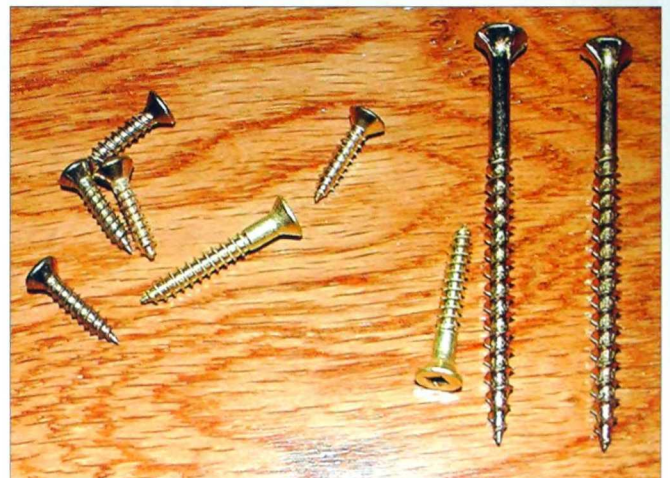
2-406. Use brass or stainless steel screws when working with oak.
