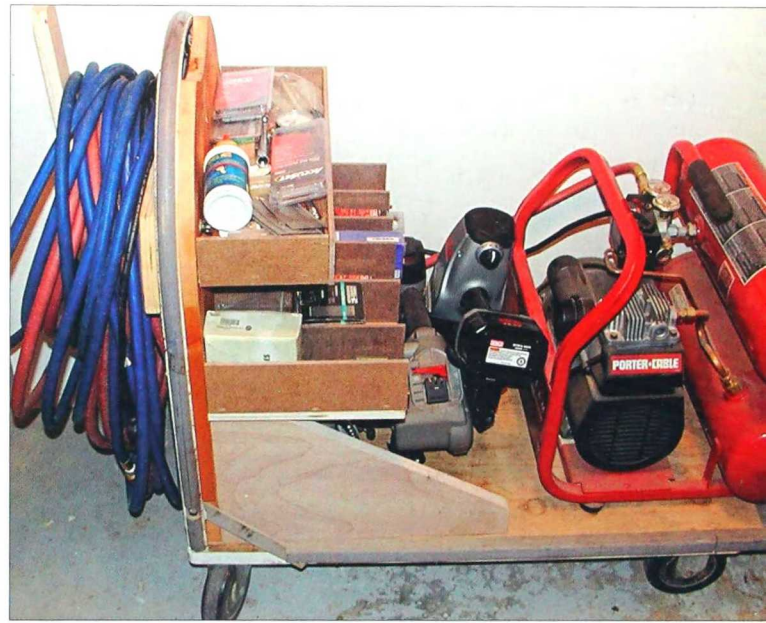
2-38. This compressor cart is mobile and contains all of the nailers, nails, and accessories.
