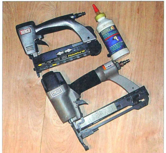
2-39. Adding oil regularly to the air nailer will help preserve its parts.
