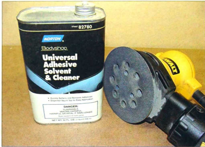
2-4. Either a utility knife or a solvent can remove the old pad.
