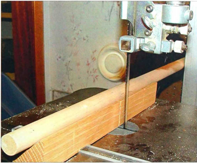
2-61. Using the V block to crosscut dowels.
