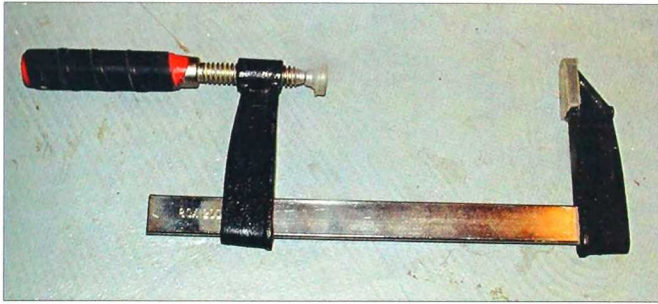
2-85. An old inner tube cut in strips will give you a better grip on your clamp handles.
