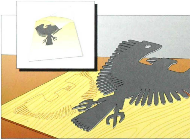
2-308. Cut out the pattern with a utility knife.
