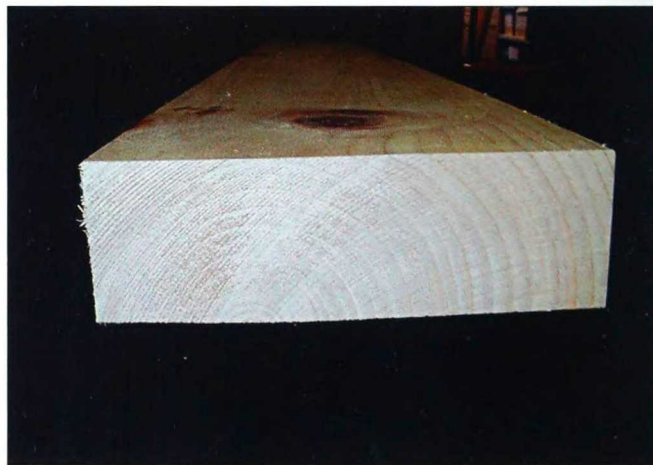
2-493. When air-drying lumber, the annual rings on the lumber should arch upward to prevent cupping and warping.
