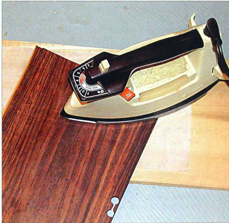
2-481. Use adhesive fabric to apply veneer to small, flat workpieces.
