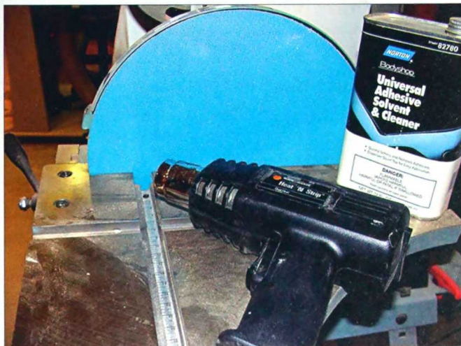
2-8. Adhesive-backed sanding discs can be removed more easily and cleanly when the adhesive is warm.
