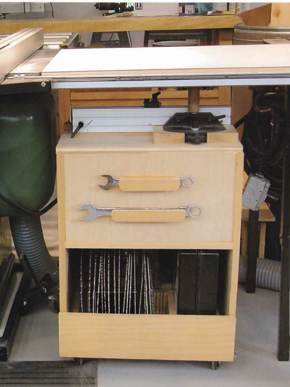
▲► IN-AND-OUTSIDE CABINET. A cabinet that fits all the blades and accessories for one tool is ideal. It's even better if it's portable so it rolls where you need it. Walt Segl's cabinet has a pull-out drawer that holds blades in kerfed blocks. When the hinged lid is lifted, a deep well for storing a tenoning jig and throat plates is revealed.
