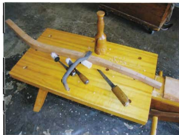
◀ ▲ CHOP WHILE YOU SIT. Topping a standard chairmaker's shaving horse with a wood slab allows you to cut joints and perform other pounding tasks without moving to your main bench. Russ Filbeck's maple top connects in seconds and is drilled with holes that engage holdfasts for secure clamping.
