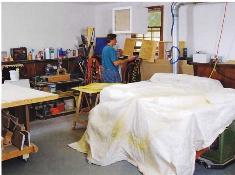
▼ USE WHAT YOU HAVE. You can spray in the shop with a little creativity. First, cover machine surfaces with dropcloths. Anatole Burkin then installs a plywood duct extension between his shopmade air cleaner and window frame to exhaust overspray and fits the cleaner with a coarse furnace filter.
