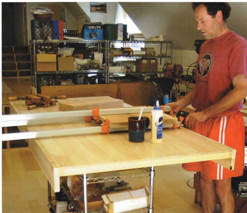
▲ BUILD DOWN LOW. A low setup table is a versatile companion to your main bench. The top on Frank Klausz's 27-in.-high assembly table measures 40 in. by 60 in. and provides a handy surface for assembling casework, while organizing hardware and tools in drawers, bins, and cubbies.
