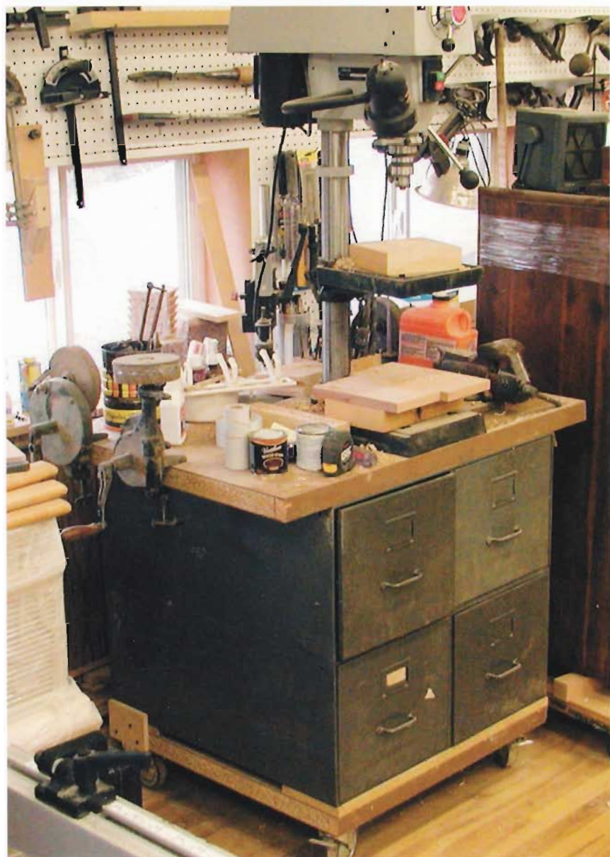
▶ BENCHTOP MADE BIGGER. A bank of old file drawers supports a benchtop-style press and provides plenty of storage to boot. Russ Marie added a heavy maple top to create a larger workstation and mounted the assembly on a shop-made dolly for easy transport.
