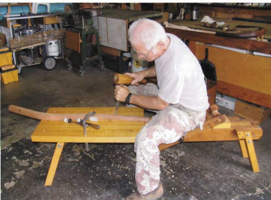
◀ ▲ CHOP WHILE YOU SIT. Topping a standard chairmaker's shaving horse with a wood slab allows you to cut joints and perform other pounding tasks without moving to your main bench. Russ Filbeck's maple top connects in seconds and is drilled with holes that engage holdfasts for secure clamping.
