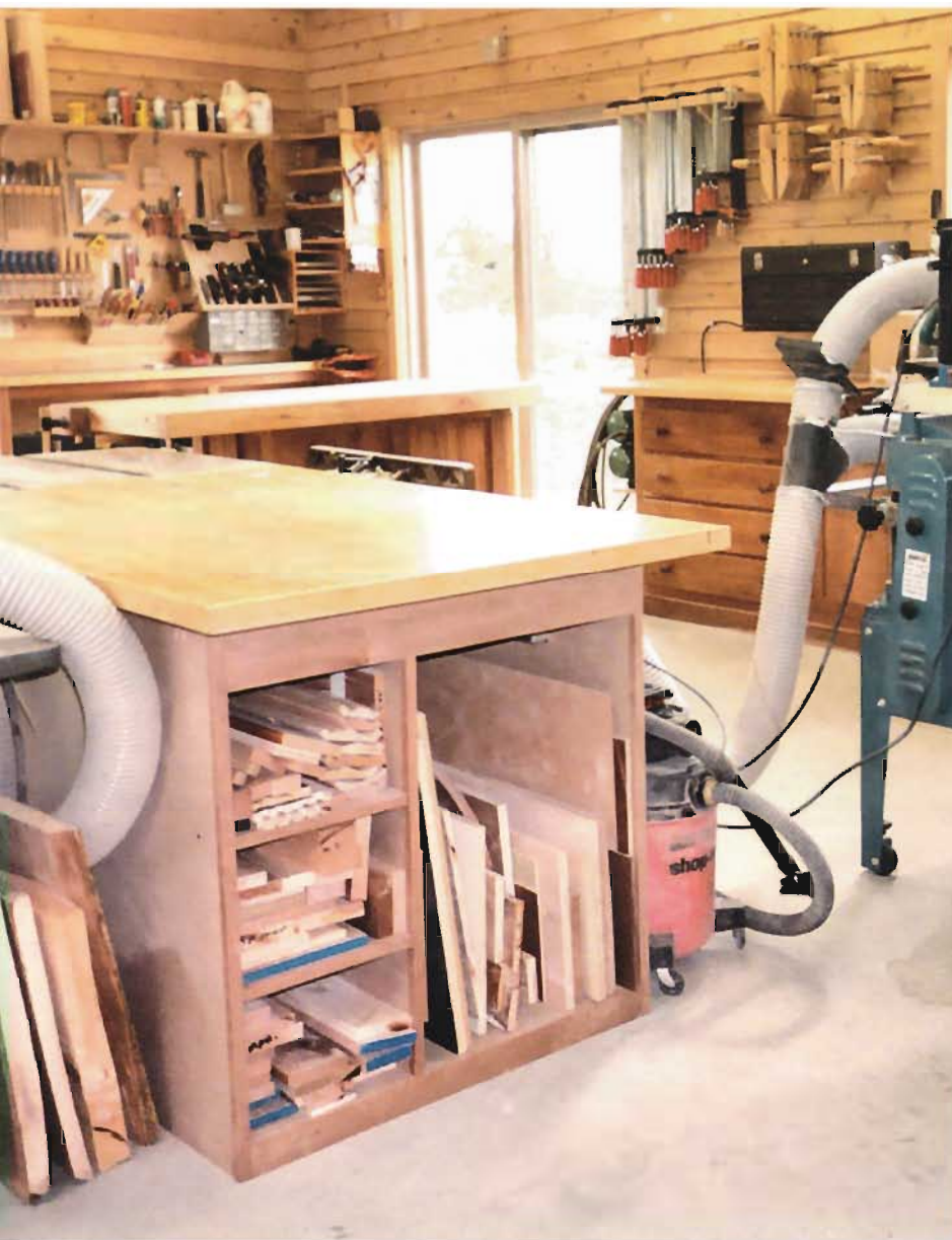
▲ LOAD AT THE END. A cabinet under an outfeed table serves double-duty as support for the table and as storage for plywood shorts and solid-wood rippings. Tom Dumke divided the cabinet and installed shelves, neatly compartmentalizing his offcuts.
