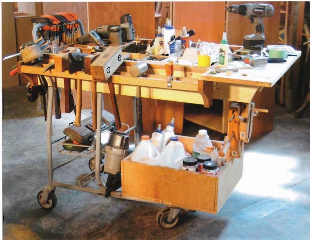
▲ ◀ SHOPPING IN THE SHOP. A converted shopping cart makes a convenient rolling hardware station. For his cart, dubbed the “piercing pagoda,” Gabe Aucott added a plywood top fitted with divided boxes to keep screws and other hardware neatly sorted and a staging platform at one end. Below, a large plywood box holds glue and other assembly tools.
