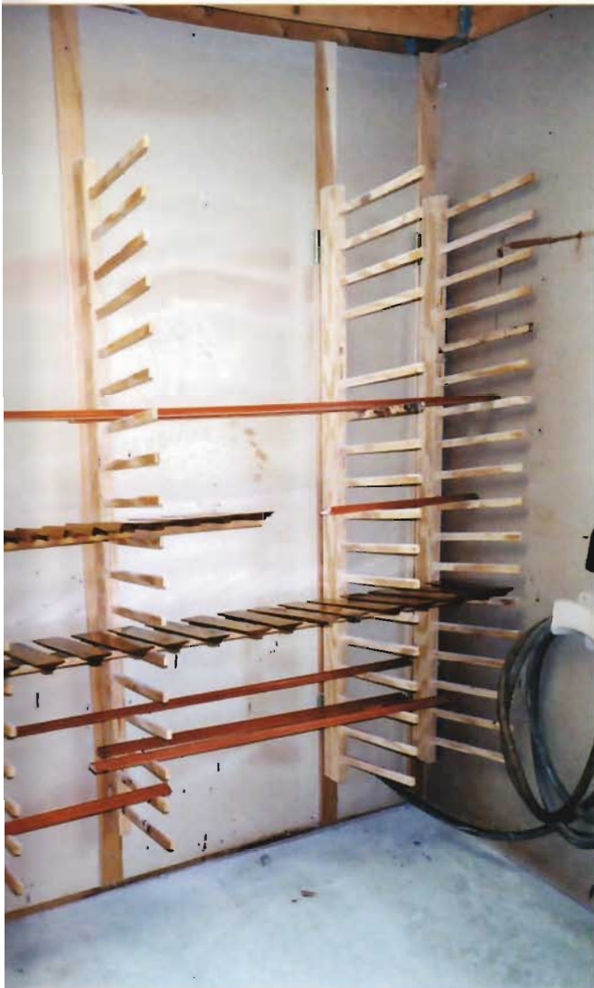
▲ RACKS THAT FOLD. If space is tight, a folding rack can provide some breathing room. The racks in Tom Dumke's finish room are made from 2x4s hinged to the studs in the wall, with removable sticks for supporting different-sized work. When drying is done, the racks fold conveniently onto the wall.
