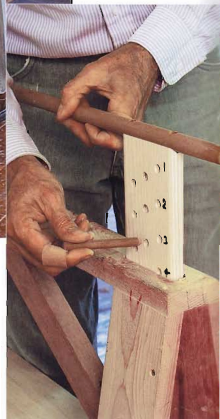
▲ ► UP AND DOWN HORSE. Built-in adjustability lets you work at any height. You can adjust the beam height on Chris Becksvoort's sawhorses by relocating dowels in the drilled uprights. A frame that slides into the horses is capped with a wood dowel wrapped in foam pipe insulation to cushion delicate work.
