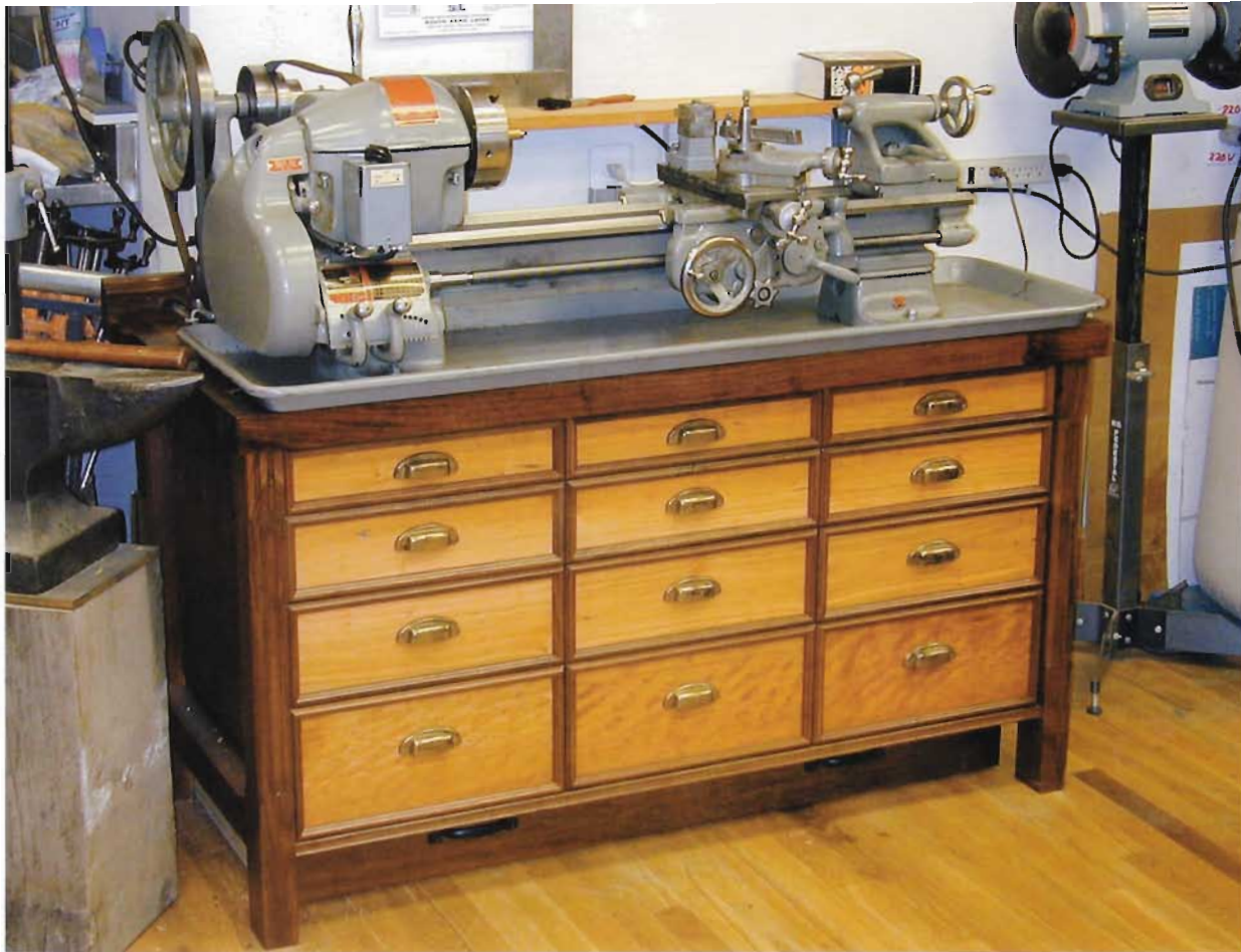
▲ WEIGHT IT OUT. Metal lathes, and even wood lathes, will benefit from a heavy mass supporting the work to reduce vibration. Jim Moon's lathe bench is stout and sturdy, and drawers filled with gear ensure smooth operation above while the works spins.
