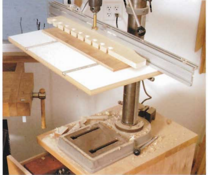
◀ ▲ DRILLING FROM A CORNER. A mobile benchtop drill press lets you park the tool out of the way, then pull it out for drilling long work or to facilitate cleanup. A bank of drawers stocks bits and accessories, adding necessary weight to keep the center of gravity low.
