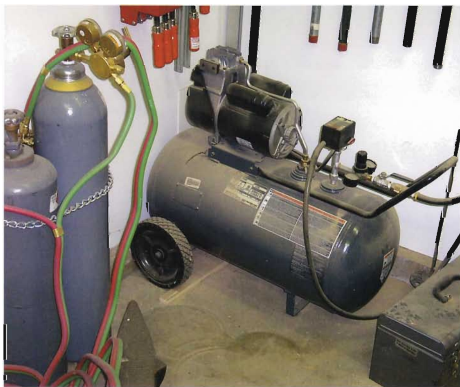
▲ MIDSIZED SPRAYER A midsized compressor like this 25-gal. unit can handle all sorts of jobs, including light sanding and spraying with a low-pressure gun. Wheels and a handle let you move it from spot to spot, but don't expect to get it up the stairs.
