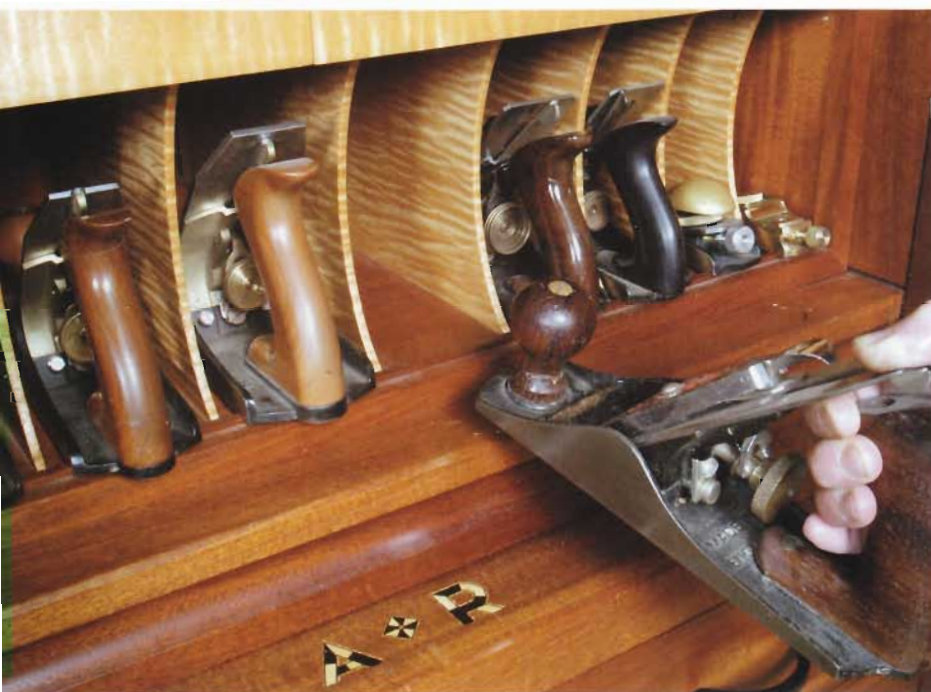
▲ DIVIDED BY SIZE. Dividers create cubbies and are spaced to the width of individual planes, saving space while devoting specific spots so tools won't get lost. The heel of each plane rests on a small strip of hardwood, raising the back of the plane to prevent the sharp iron from digging into the shelf.
