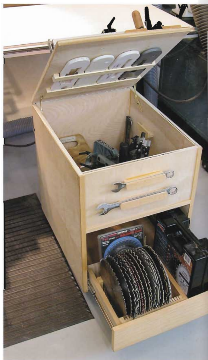
▲► IN-AND-OUTSIDE CABINET. A cabinet that fits all the blades and accessories for one tool is ideal. It's even better if it's portable so it rolls where you need it. Walt Segl's cabinet has a pull-out drawer that holds blades in kerfed blocks. When the hinged lid is lifted, a deep well for storing a tenoning jig and throat plates is revealed.
