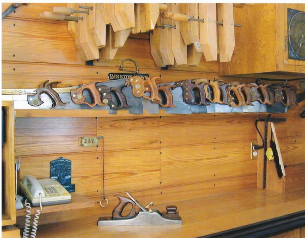
◀ ▲ SAWN SHELF Innovative saw storage means the saws are ready for use at a moment's notice and don't take up much room. In Jim Moon's shop, a series of angled saw kerfs (above) sawn into the shelf with a thin-kerf circular saw hold a collection of vintage saws upright and in a relatively compact space.
