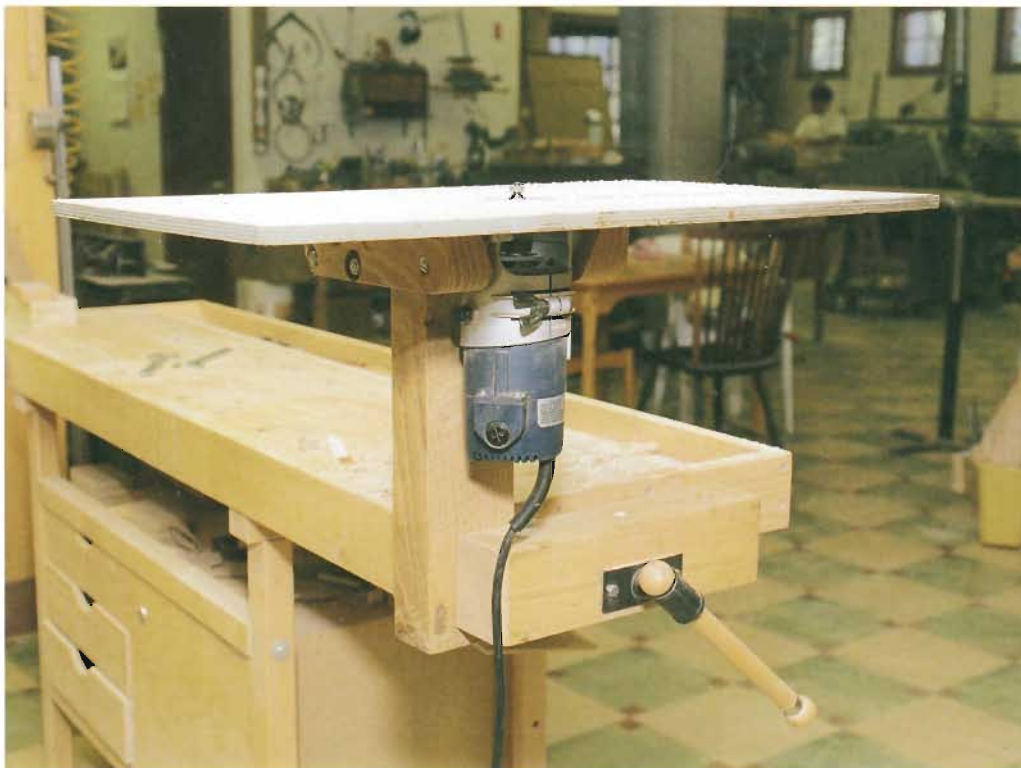
◀ A TABLE THAT DISAPPEARS. Router tables don't need to be fancy or take up precious shop space to work well. This bench-mounted version clamps quickly and securely in a vise and offers a more convenient routing height. Once routing is done, simply unclamp and store it on a shelf.
