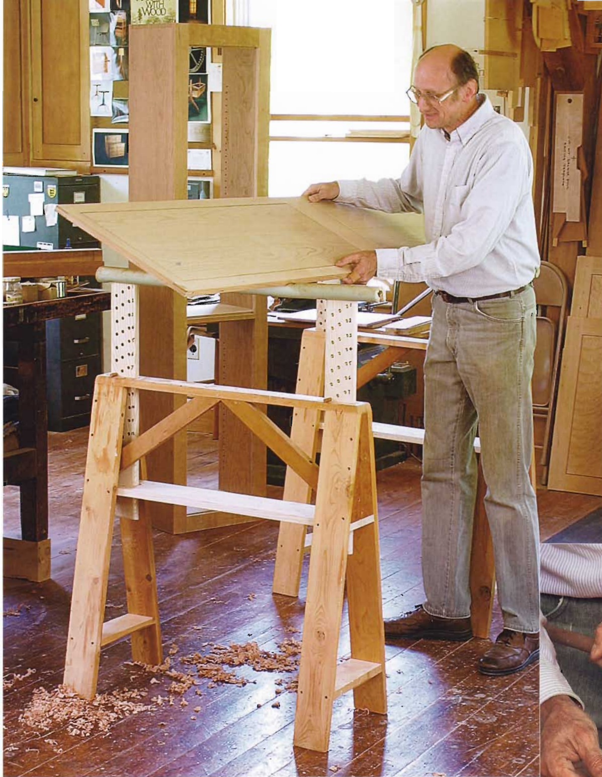
▲ ► UP AND DOWN HORSE. Built-in adjustability lets you work at any height. You can adjust the beam height on Chris Becksvoort's sawhorses by relocating dowels in the drilled uprights. A frame that slides into the horses is capped with a wood dowel wrapped in foam pipe insulation to cushion delicate work.
