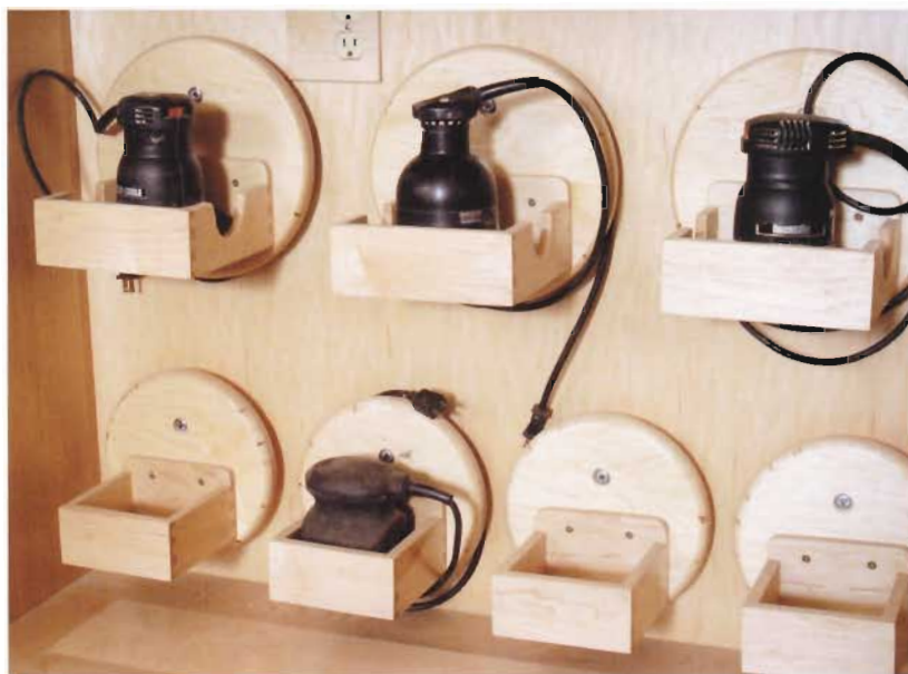
◀ SANDBOX UNDER CONTROL. Individual racks are the perfect size for palm and orbital sanders. The boxes in Palomar College's shop are mounted to wooden disks, with space behind so cords can be wrapped neatly out of the way. This setup works well in a classroom situation or wherever shop tools are shared.
