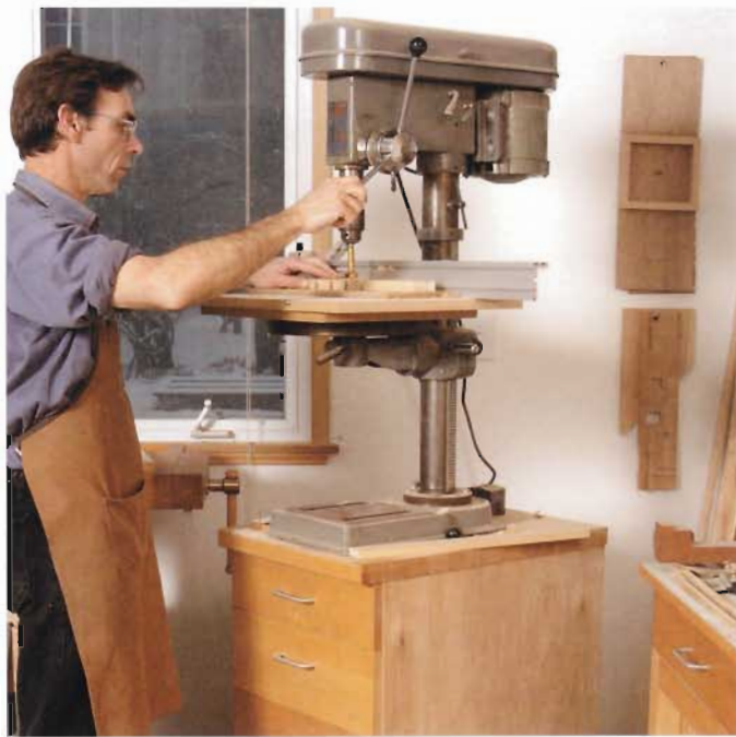
◀ ▲ DRILLING FROM A CORNER. A mobile benchtop drill press lets you park the tool out of the way, then pull it out for drilling long work or to facilitate cleanup. A bank of drawers stocks bits and accessories, adding necessary weight to keep the center of gravity low.
