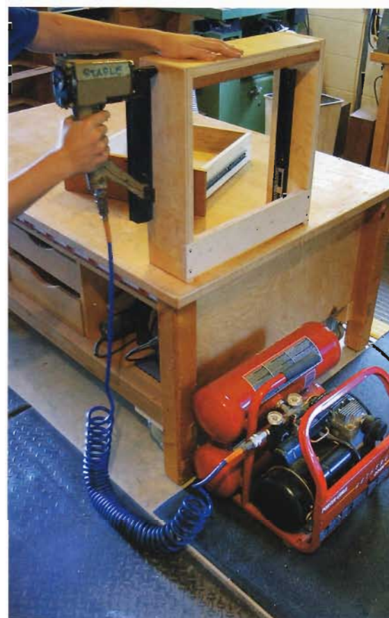
▲ PORTABLE NAILER A small compressor can power one or two nail guns all day long. Its relative light weight lets you use it in the workshop, or carry it around the house or to the job site for trimwork or installations.
