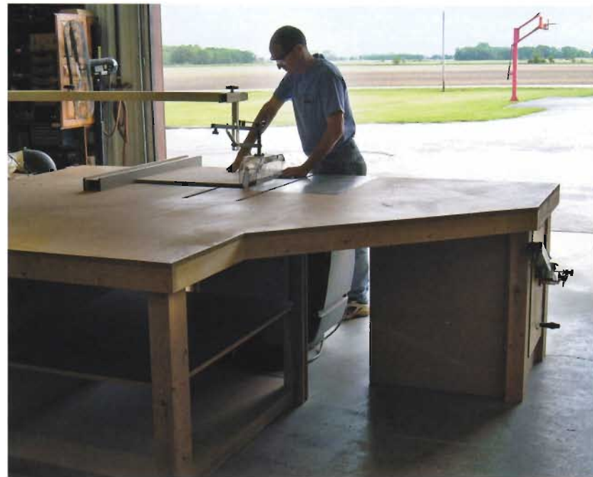
▲ WORK WHERE YOU'RE COMFORTABLE. Setting up a table saw in front of a garage door allows easy access, good light, and a cool breeze during hot weather. Building support tables around the saw increases its versatility and lets you saw and stack parts with less effort.
