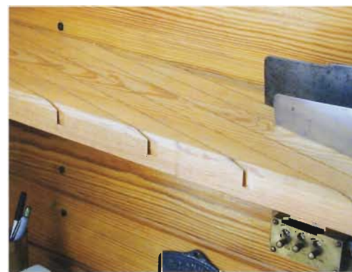
◀ ▲ SAWN SHELF Innovative saw storage means the saws are ready for use at a moment's notice and don't take up much room. In Jim Moon's shop, a series of angled saw kerfs (above) sawn into the shelf with a thin-kerf circular saw hold a collection of vintage saws upright and in a relatively compact space.
