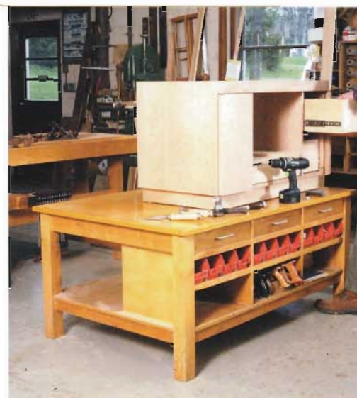
▲ BUILD DOWN LOW. A low setup table is a versatile companion to your main bench. The top on Frank Klausz's 27-in.-high assembly table measures 40 in. by 60 in. and provides a handy surface for assembling casework, while organizing hardware and tools in drawers, bins, and cubbies.
