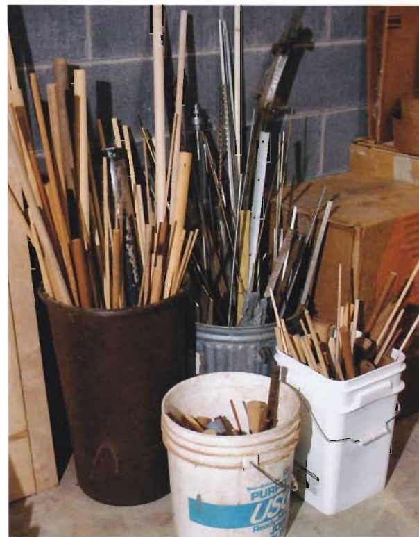
▲ BUCKET BRIGADE. Trash cans and buckets in varying sizes make great instant storage for dowel stock. Long dowels live in taller containers, while shorter offcuts go in short buckets, making small stuff more accessible. A heavy-duty metal trash can stores rod and other metal stock.
