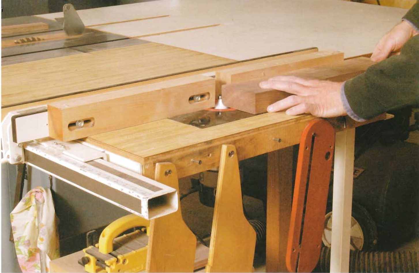
▲ TABLE SAW TURNED ROUTER. Take advantage of your table saw's sidefeed table by mounting a router underneath. You can use the saw's rip fence, too, by adding wood blocks that let you adjust the bit opening so you can tailor the setup for any routing procedure.
