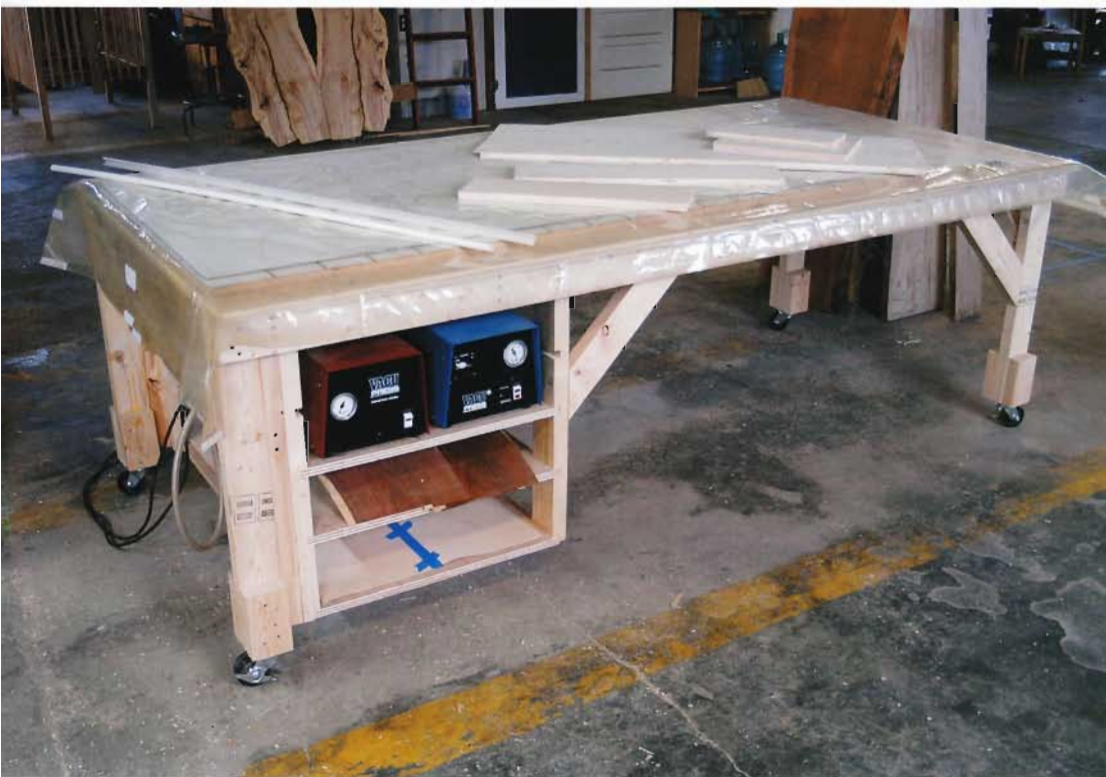
▲ BUILT LIKE A BRICK. Vacuum veneering requires a sturdy, flat table for successfully flat veneer jobs. Gabe Aucott's rolling table is made from 2x4 stock with a plywood top and is heavily braced to prevent sag. Veneer and vacuum pump storage is built in.
