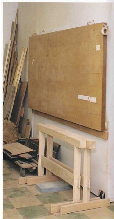
▲ VANISHING VENEERING. If veneering is a part-time activity, you'll appreciate a veneering table that moves out of the way. Joe Tracy's table folds down onto a pair of sawhorses for use, then stows against the wall when done. For even more space, the entire wall rolls out of the way with the setup in place.
