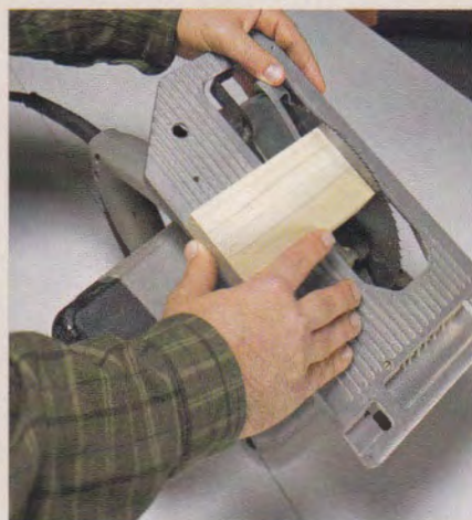
The setup block matches the distance from the blade to the edge of the base.
