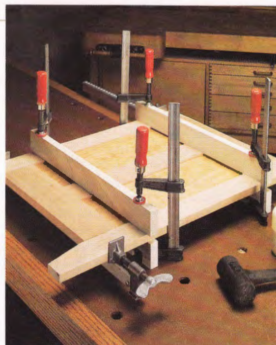
To ensure a perfectly flat side assembly, clamp it between two pairs of straight boards. The bottom board is notched for clamp clearance.
