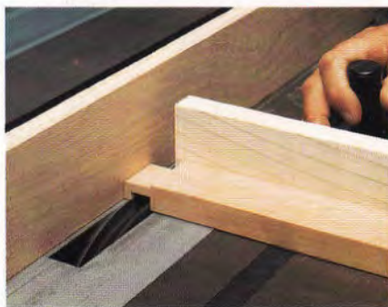
To make the tenons, use a table saw equipped with a dado blade.
