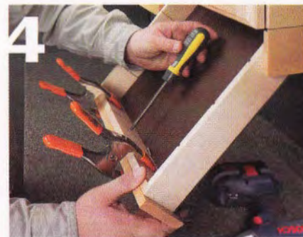
4] Pull out the tray, and attach the false front by running screws through the tray front and into the false front.
