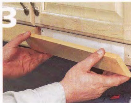
3] Temporarily “clamp” the false front in position on the front of the tray with a strip of double-sided tape.
