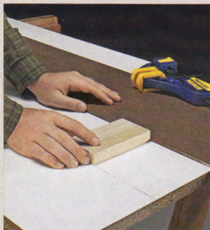
A setup block lets you easily position the straightedge in relation to the cutline.
