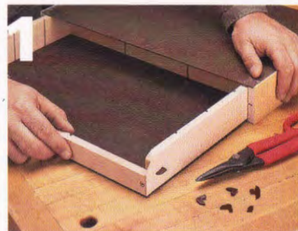
1] To install the trays, clip one “wing” off each shelf support ( left ). Install the supports, and slide the tray into the rails.
