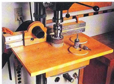
Here's the sanding drum lowered into the table; the vacuum hose is mounted on top of the table.
