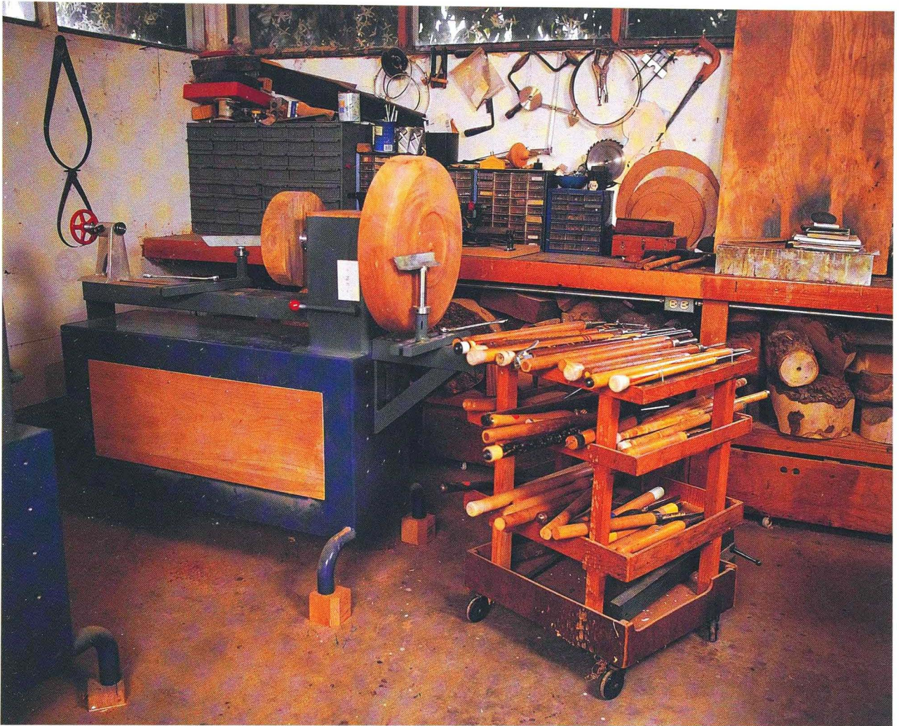
Ted Bartholomew's custom lathe is designed for working on either side of the machine. The portable tool storage cart is easily moved throughout the woodshop.
