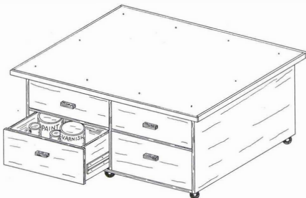
This low, mobile workstation features drawers on both sides of the unit and wheels. Lockable wheels are recommended. The unit is approximately 16" to 24" in height.
