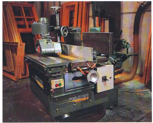
The Felder machine rotates upon a swivel base so that each function is easily accessible. Note that the planer tables are raised.
