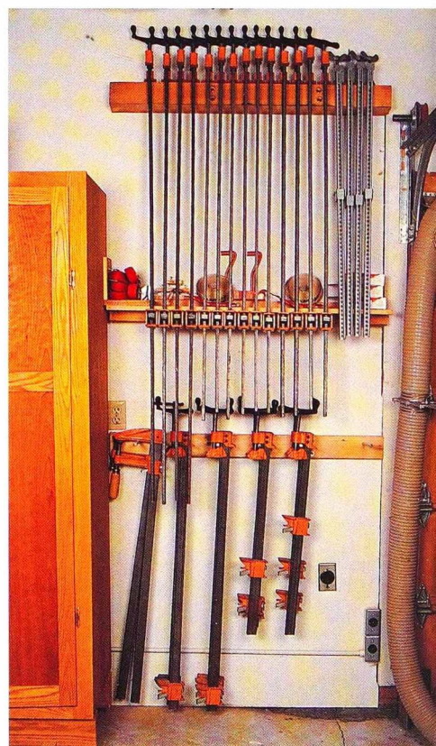
Here's a view of clamp storage in my woodshop. The upper 4" × 4" beam has an angled face so that clamps are suspended at an angle. Shorter bar clamps are suspended from \frac{1}{2} " metal dowels inserted into a secured 2" × 4" board.
