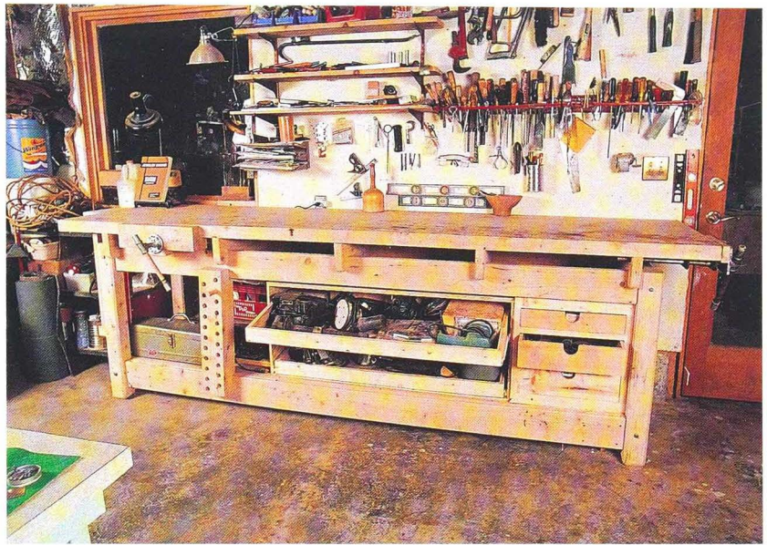
Harry Charowsky's workbench, made from 2" x 6" fir boards measures 29½"-wide by 114½"-long by 36¾"-high. It features drawer storage, movable workpiece support, shop-made hardware for vises, and it has a shop-made mobility system (underneath the bench) that makes it easy for one person to move the workbench.
