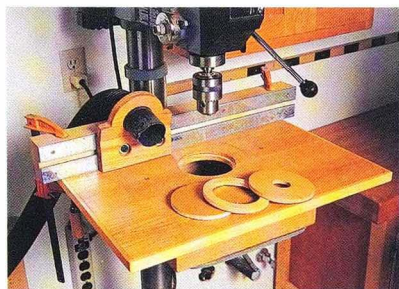
The drill press table in my woodshop features different table inserts for different-diameter sanding drums. The fence has a holder for a vacuum hose.
