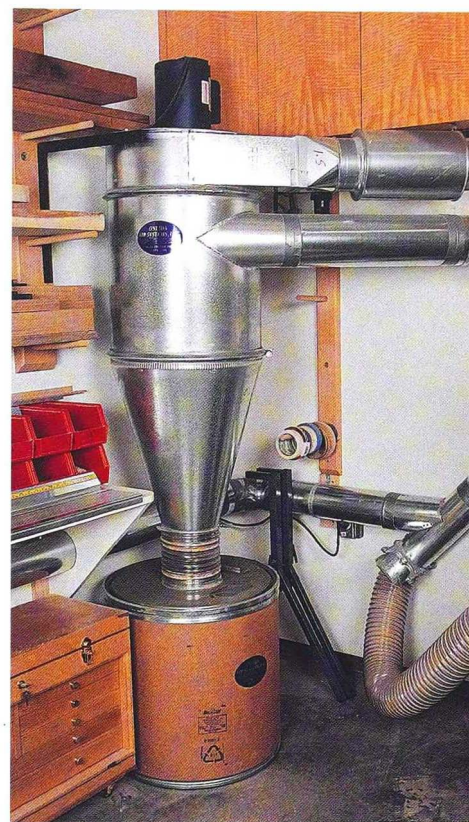
The Oneida cyclone dust collector, shown above in Charles Caswell's shop, has the air filter within the cyclone. It also features a muffler (protruding horizontally just below the motor), 5" ductwork, 35-gallon fiber barrel and a remote on/off switch located on the combination machine.
