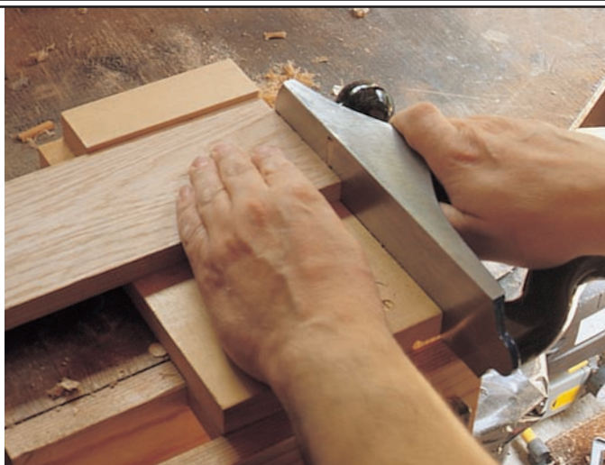
12 Final fit the drawer fronts using your handplane.
