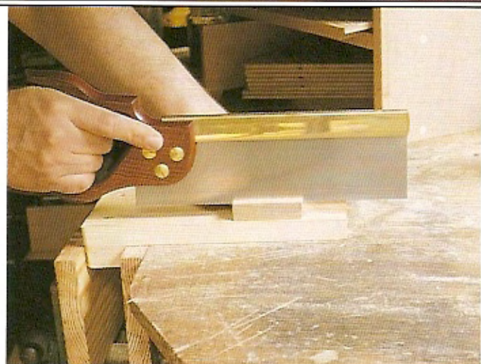
11 Cut the drawer faces to rough length.
