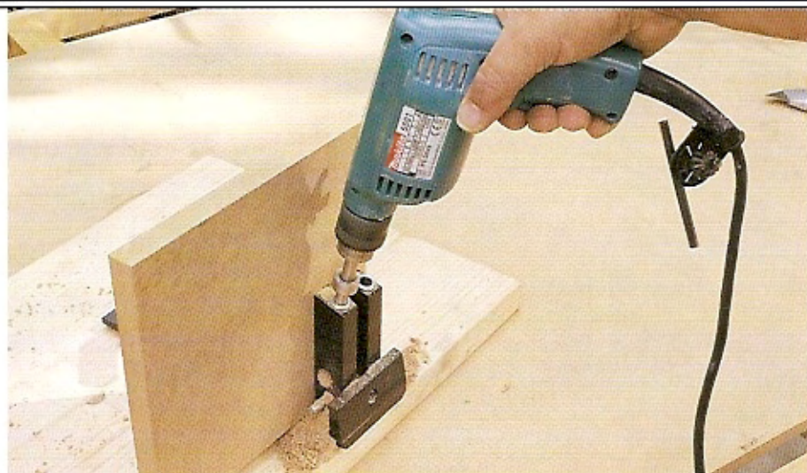
8 Drill pocket holes in the shelves.
