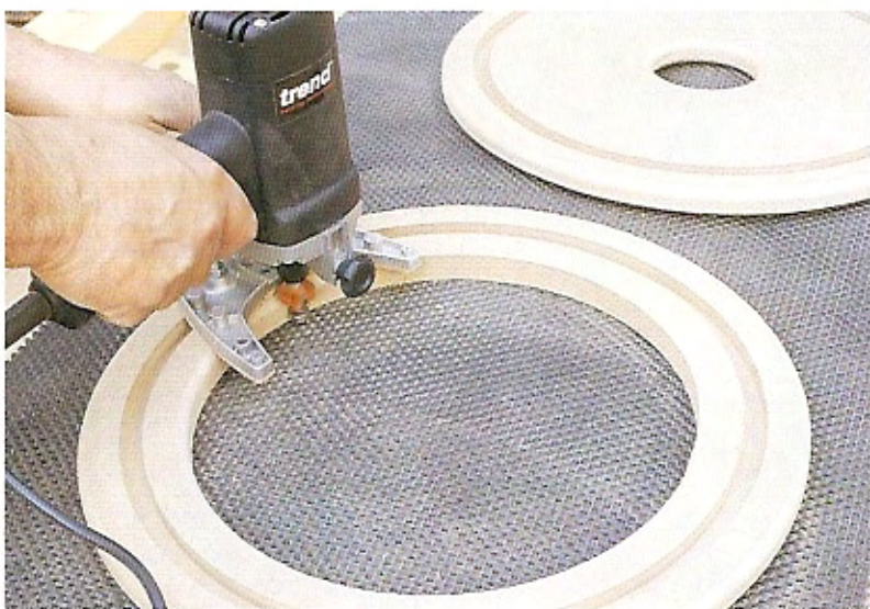
12 Round over all the exposed edges of the router park.
