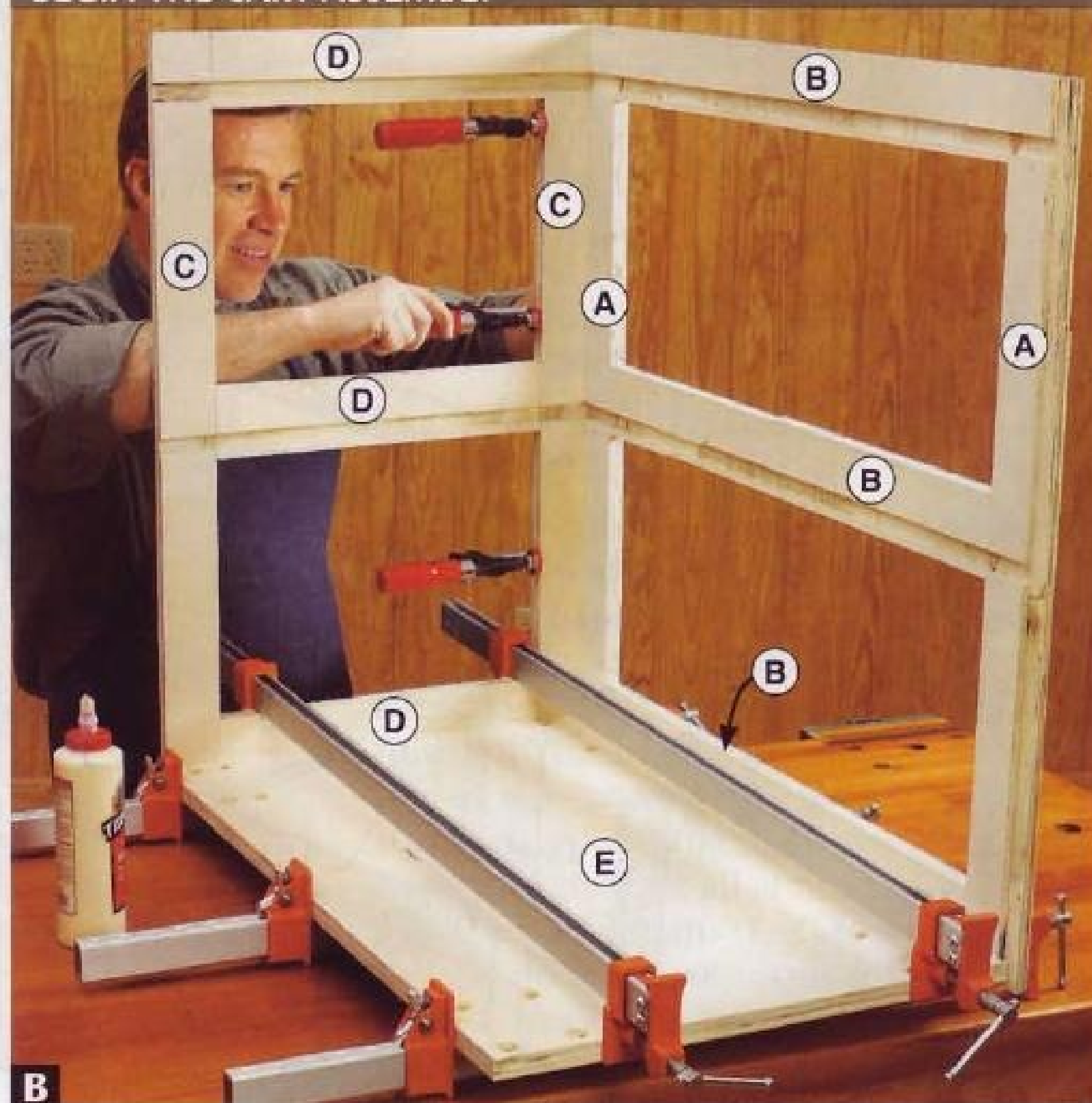
B Glue and clamp a side frame (A/B), end frame (C/D), and the bottom shelf (E) together, making sure you close the frame corner joint by drawing the end frame tightly into the rabbet in the side frame.
