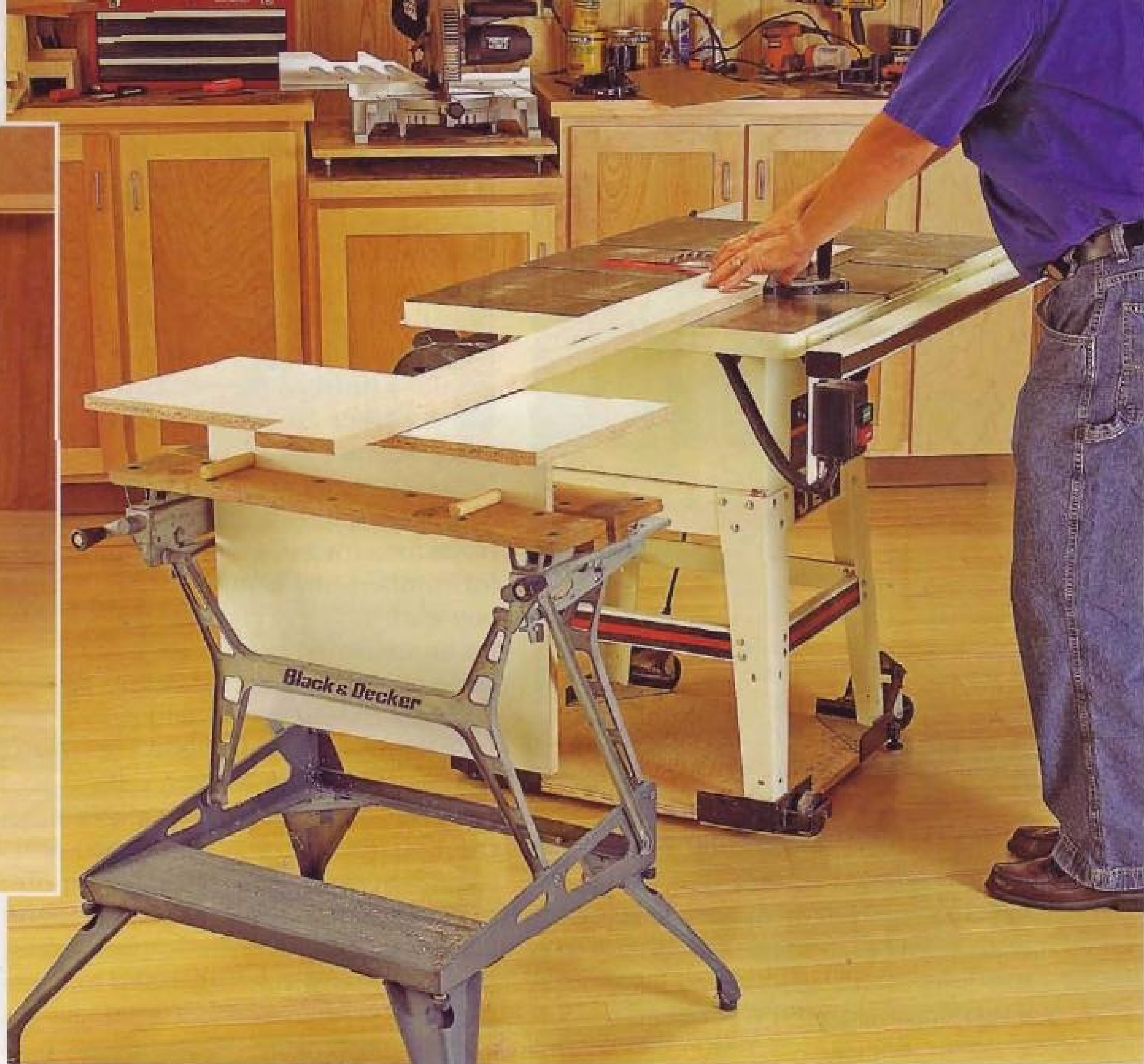
A Black & Decker Workmate manages clamping tasks ( above ) and proves equally handy as a workpiece support ( right ).
