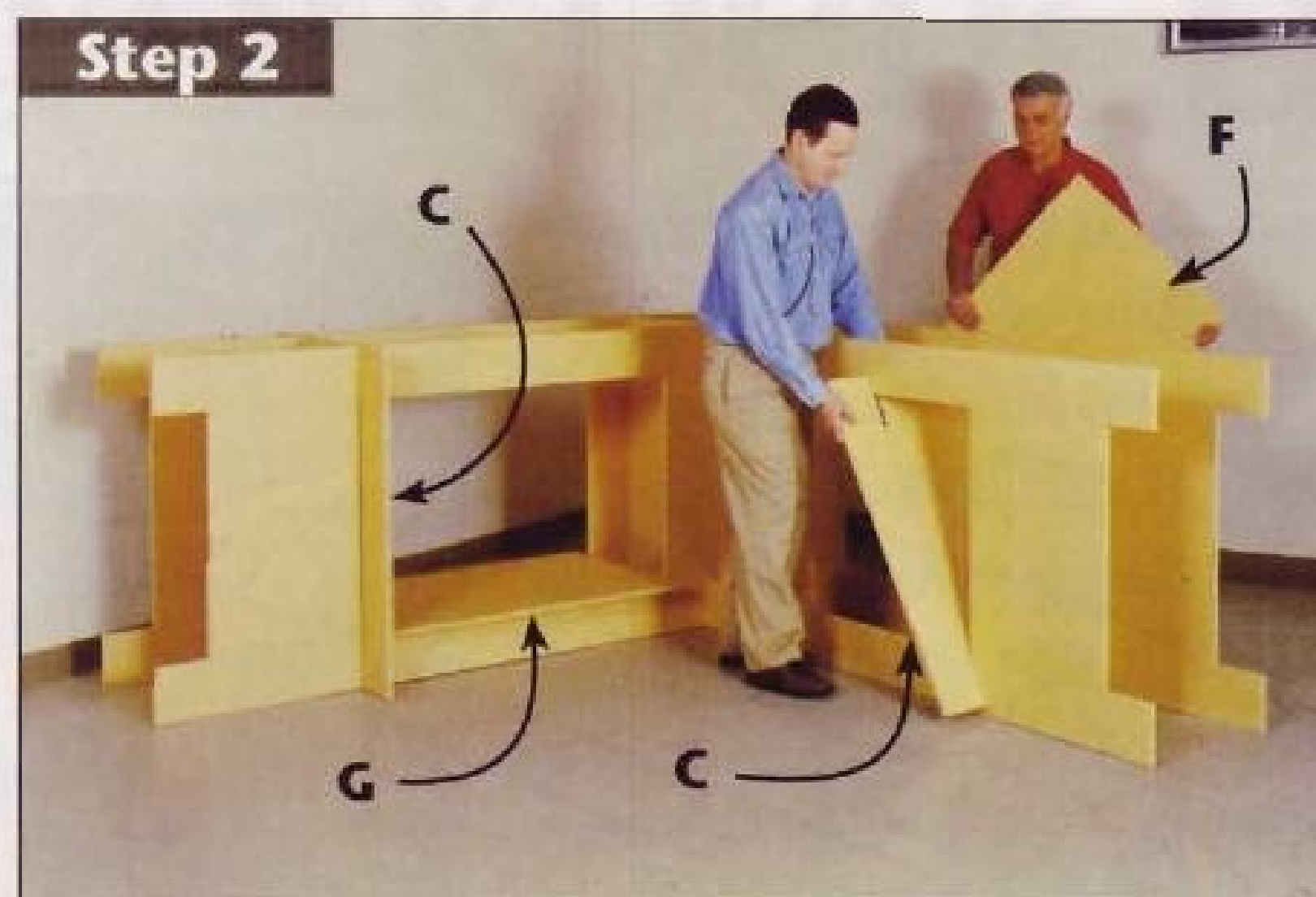
Interlock the slots in the ends (C) with the bases. Add the lower base shelves (F, G).
