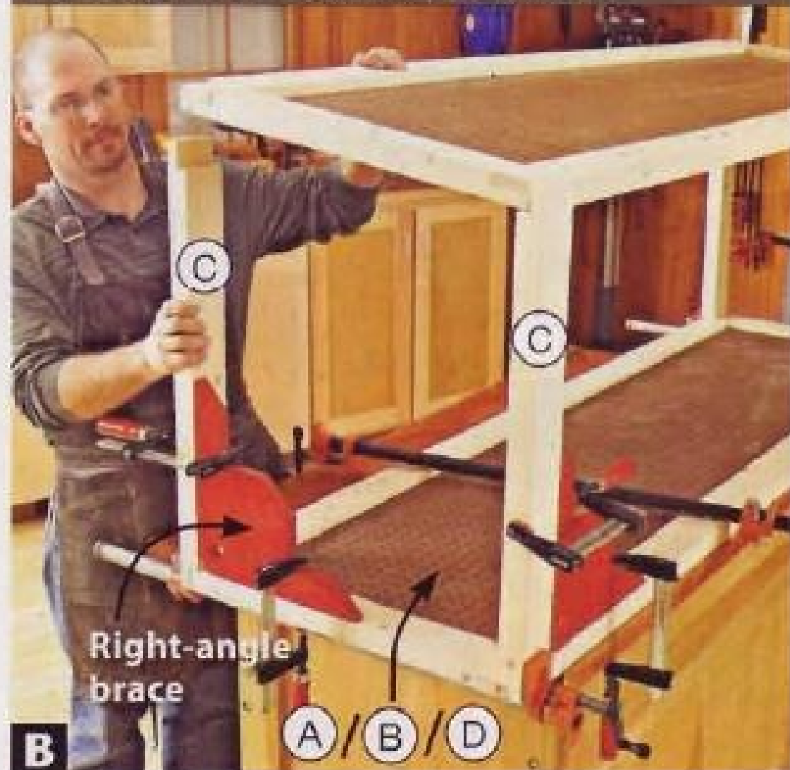
With the stretchers (C) attached to the first side (A/B/D), apply glue to the stretcher rabbets, and position the second side.
