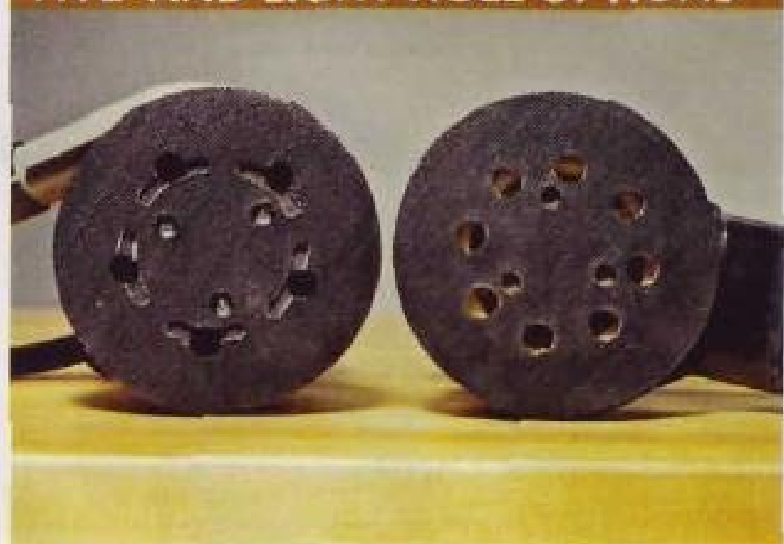
When the sander base has slots (left), you can use either five- or eight-hole paper.
