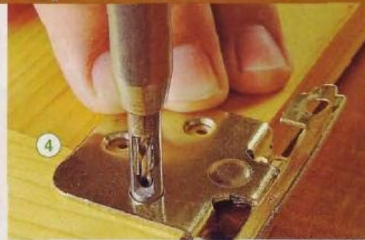
Four precision bits: ① Single-flute countersink (no. 145636, set of 4 for #4-#10 screws, about $40, Woodcraft, 800-225-1153 or woodcraft.com); ② brad-point; ③ Forstner for holes up to 1½"; and ④ Vix for self-centered holes in hinge-mounting holes (no. and price vary, McFeely's, 800-443-7937, or mcfelys.com).
