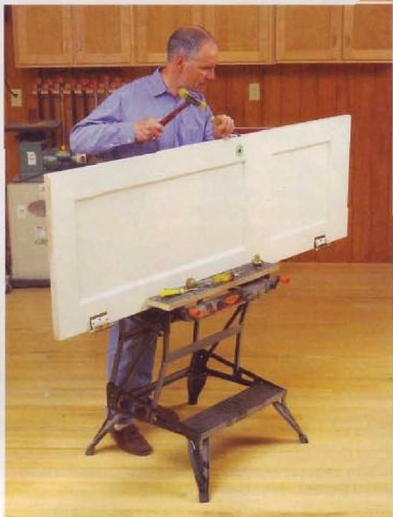
A Black & Decker Workmate manages clamping tasks ( above ) and proves equally handy as a workpiece support ( right ).
