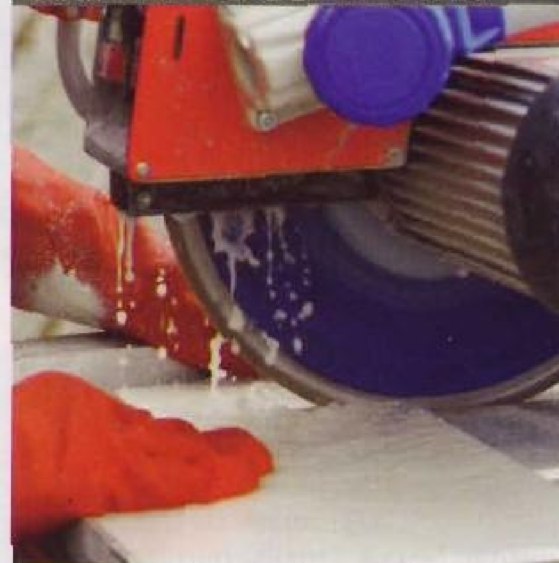
A tile wet saw is a must for smooth cuts in stone, porcelain, and many floor tiles.
