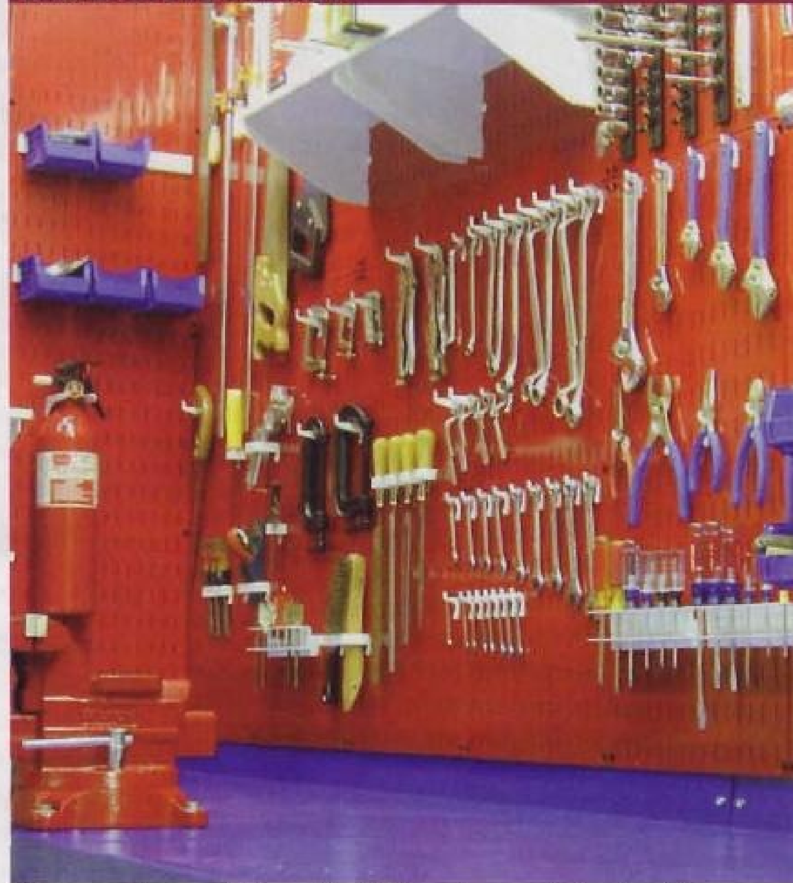
These steel panels from Wall Control are solid, colorful alternatives to perforated hardboard. Although the company offers a wide variety of hooks and accessories, the panels allow the use of any third-party magnet hooks or hangers.
