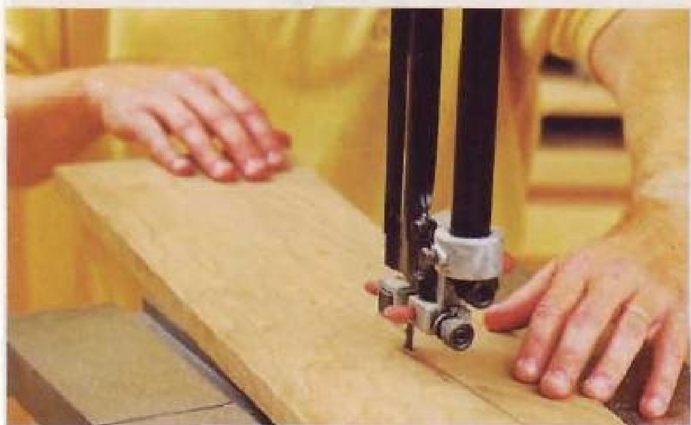
A bandsaw shines at cutting curves, and can also rip, resaw, cut circles, and even mill short, small-diameter logs into lumber.
