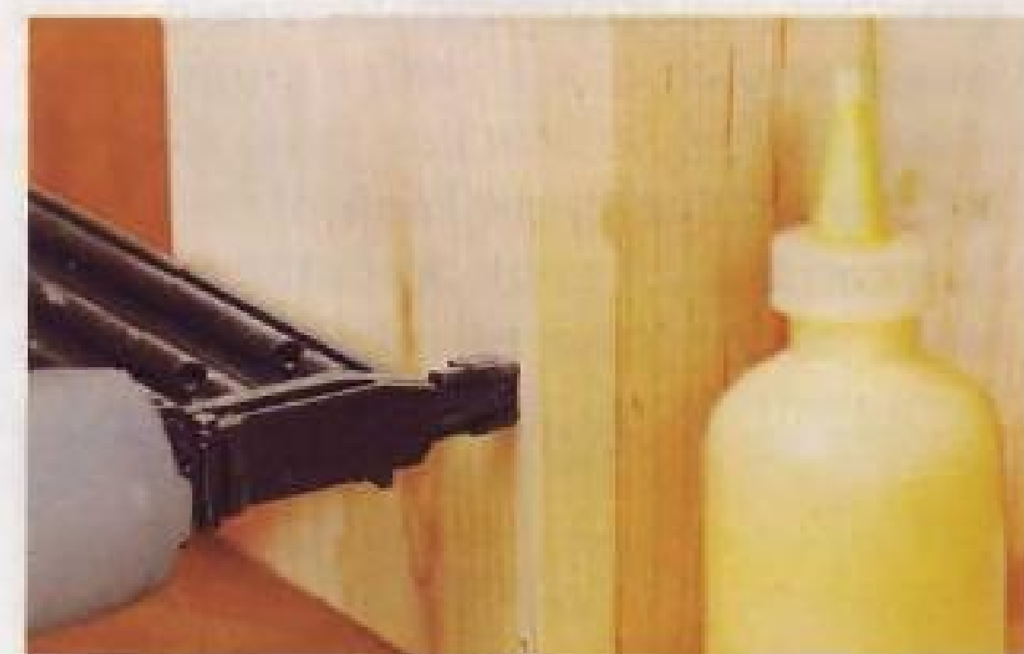
A pneumatic air nailer drives a brad into joints without splitting the wood, and holds the assembly while the glue sets.
