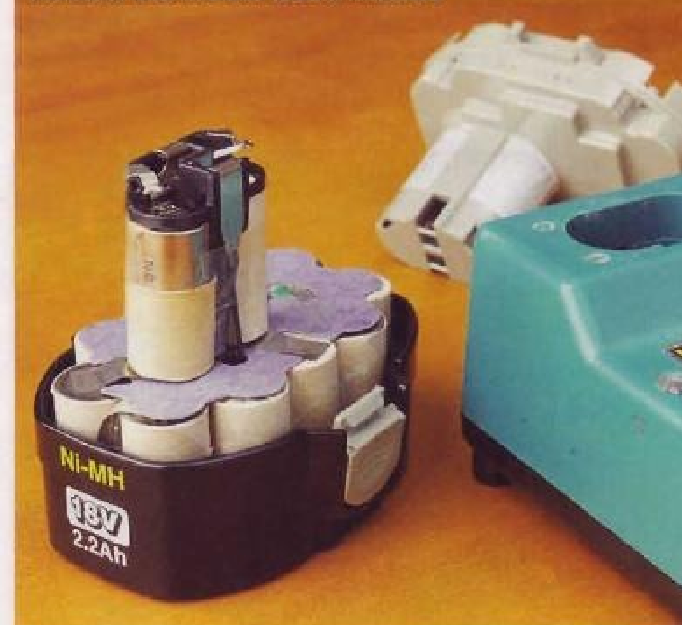
It takes 15 cells, each rated at 1.2 volts, to produce the long run times of this 18-volt nickel-metal-hydride battery pack.
