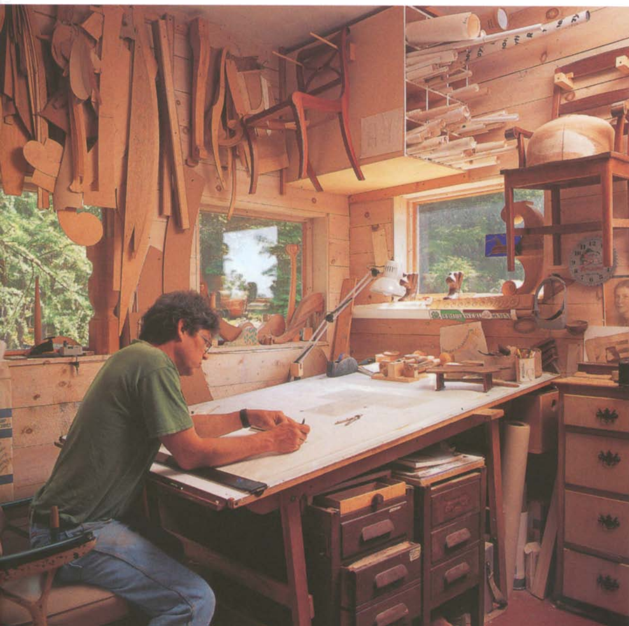
ASTRIDE A SALVAGED dentist's chair, Turner goes to work at a spacious drafting table. He typically produces full-scale drawings for furniture, a practice he learned at Boston's North Bennet Street School. Although time-consuming to produce, the drawings save time when Turner makes patterns for furniture parts.
