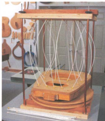
FIBERGLASS RODS that Abrams bought from a local fishing-supply dealer make ingenious go-sticks to clamp the tops of mandolins and guitars to their bodies. The height of the platen can be moved up or down to adjust tension.
