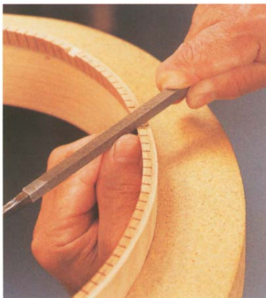
ABRAMS PREPS the curved side of an octave mandolin to receive the top. Although he once had to make the kerfed mahogany reinforcement on the inside edge of the case himself, the material is now available from specialty suppliers.
