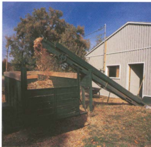
PRODUCTION TURNING makes shavings by the truck-load. Stinson adapted a conveyor typically used to clear manure from barns to ferry shavings into a 4-ft. by 12-ft. dump trailer, which can be hauled away.
