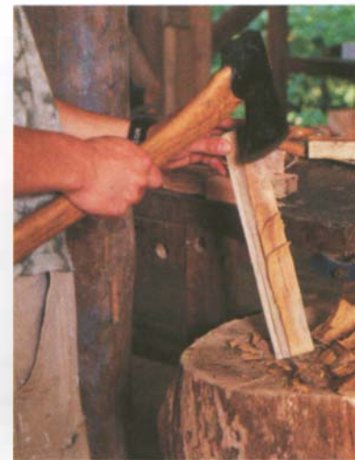
A HEWING AX cuts a leg blank down to size. Although students have access to motor-driven lathes, many of the school's classes emphasize the use of hand tools and skills practiced by country furniture makers.
