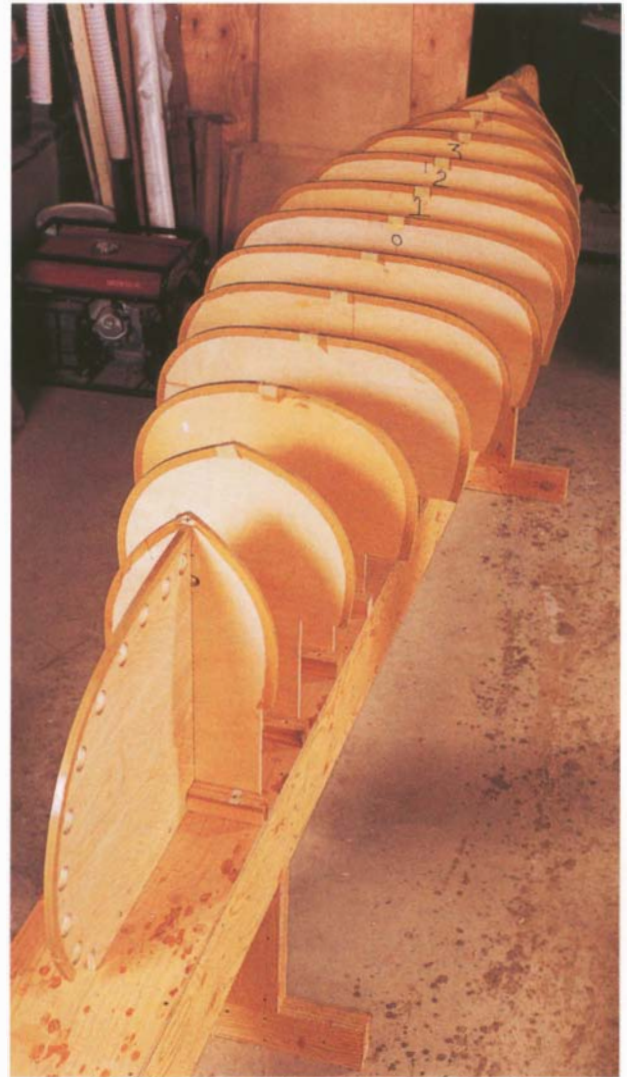
STATION MOLDS make a reusable plywood form for “The Leaf,” a solo canoe that Martin designed. Strips of cedar whose edges have been milled into a bead-and-cove pattern are laid over the molds to form the hull and then finished with epoxy.
