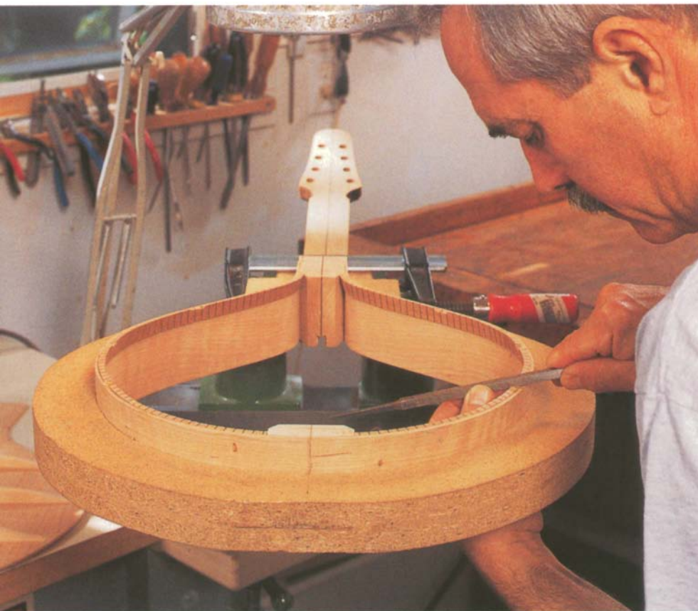
ABRAMS PREPS the curved side of an octave mandolin to receive the top. Although he once had to make the kerfed mahogany reinforcement on the inside edge of the case himself, the material is now available from specialty suppliers.
