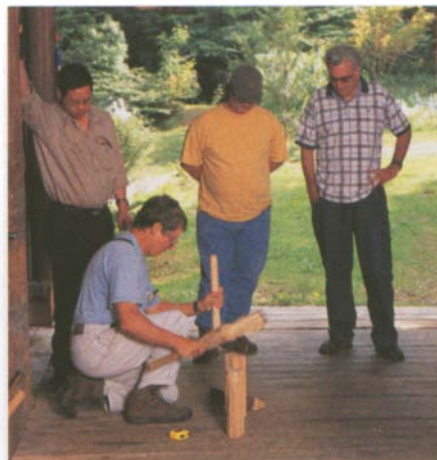
CLASSES MAY START with a log. Drew Langsner demonstrates the use of a froe for students in one of his chairmaking classes. Striking the tool with a rough mallet rives a section of wood, which can then be fashioned into a chair part.
