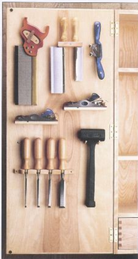
This back saw fits over a block that's cut to match the inside shape of the handle. Twisting a hardboard turn button locks the saw in place.
