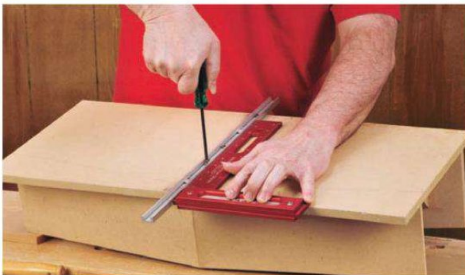
Figure 4: Attach an 18"-long miter bar to the bottom of the jig. Make sure it's square, relative to the base.
