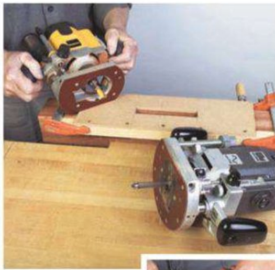
Clean up the mortise with jig-guided bits. The insert (right) lets you cut two sizes with the same jig.
