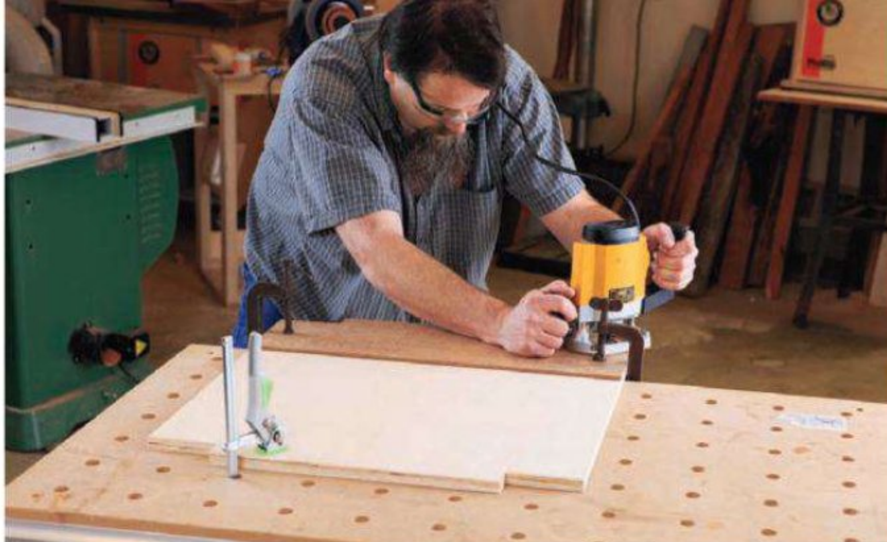
After roughing out the notches on the inner panels, the author pattern-routed the final shape with a 1/2"-diameter pattern routing bit. Its radius perfectly matched the 1/4" roundover bit used on the legs.
