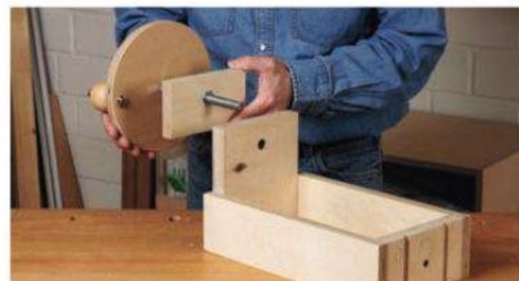
Thread the crank assembly through the captured nut in the lift bracket, fit the rod through the lift base hole, and screw these parts together.
