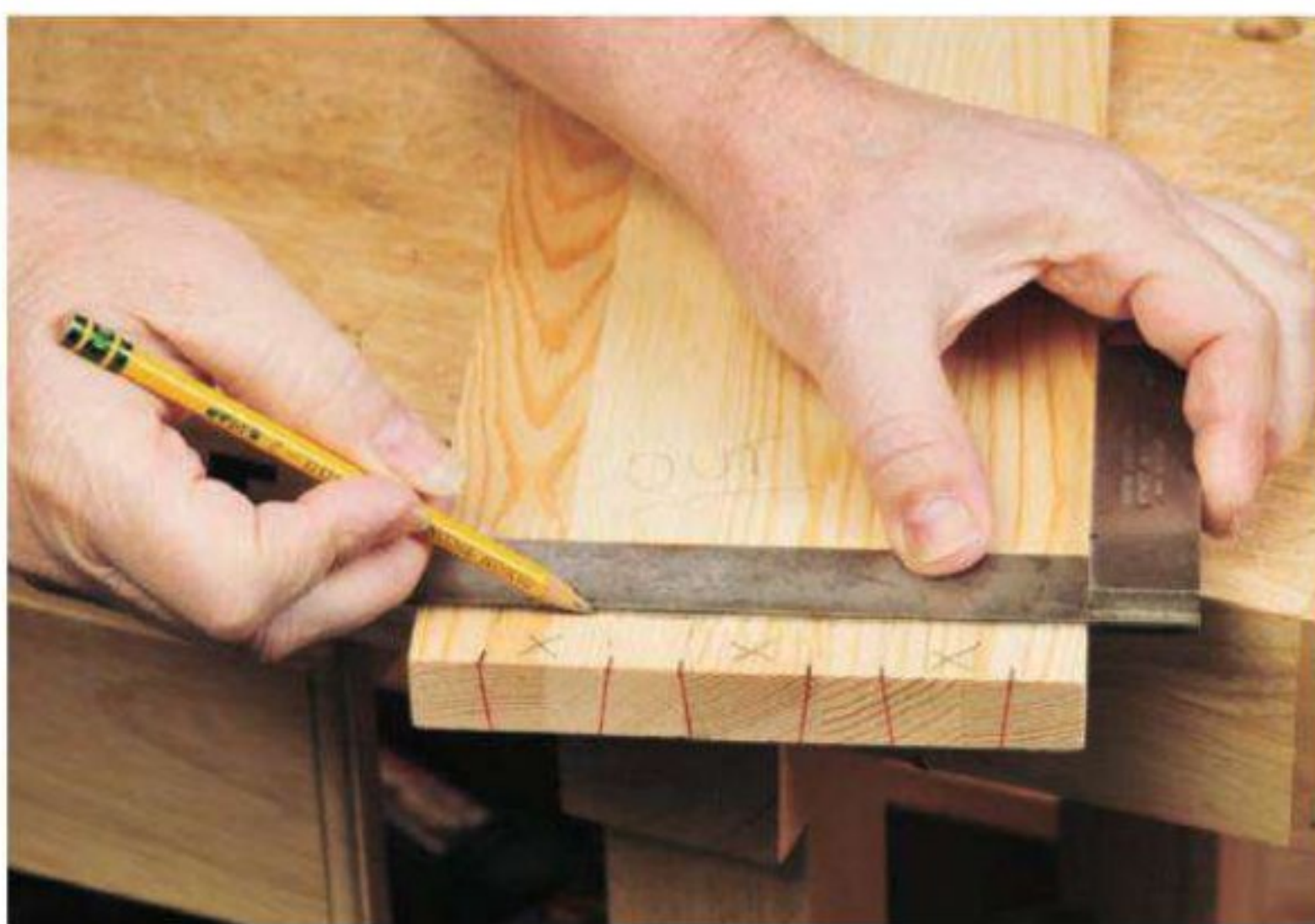
Figure 6: Here the angles of the pins are marked in red simply to illustrate the pin shape. Remember that you must mark out the "narrow" sides of the pins on the board's outside face. The "X"s indicate the waste areas.
