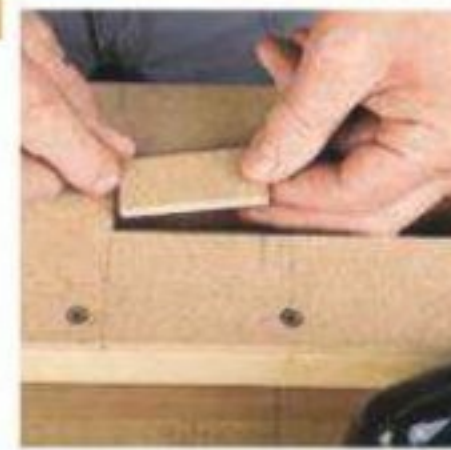
Clean up the mortise with jig-guided bits. The insert (right) lets you cut two sizes with the same jig.
