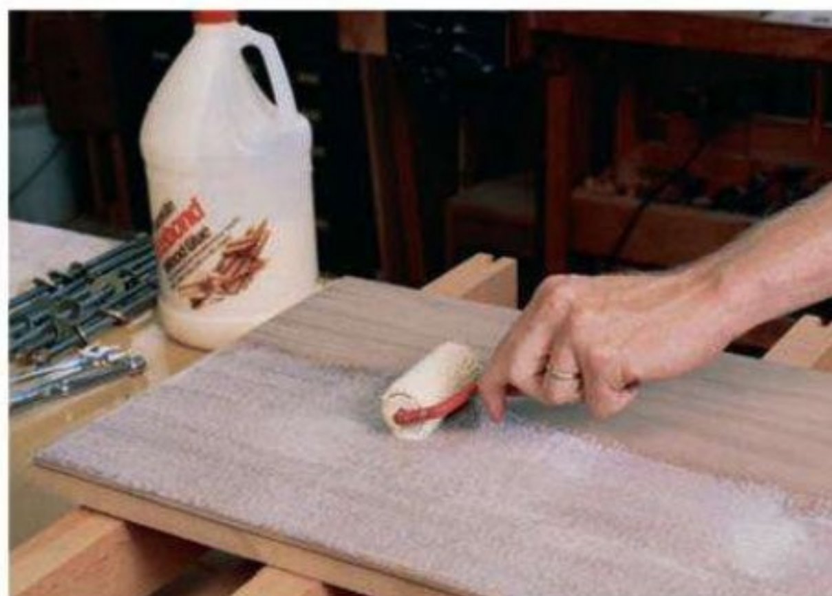
Use a small roller to spread glue evenly on the substrate. To avoid excessive curling, don't put glue directly on the veneer.
