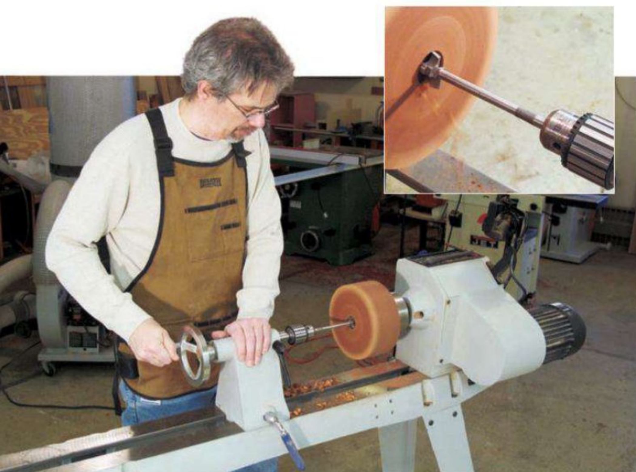
With the bowl blank spinning, the author bores a hole dead center in the wood. He sets the depth of the boring with the graduated scale on his tailstock.
