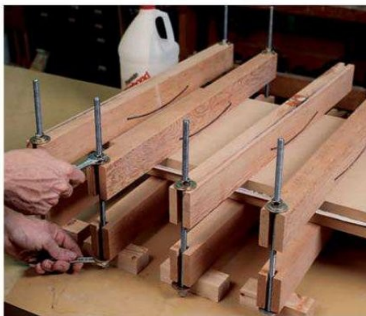
Tighten the nuts with a box wrench until you see a consistent bead of glue squeeze-out along the edges of the panel.
