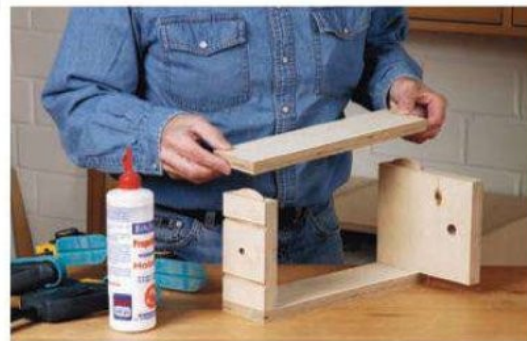
Use biscuits and glue to assemble the router lift frame. Notice that the top piece of the frame is actually the rear router mounting block.
