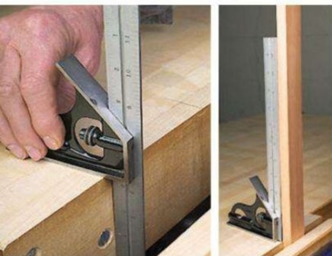
Make the fixed cheek square with the benchtop (top-left). A clamped workpiece should be square (top-right) with the top and vise cheeks parallel (right).
