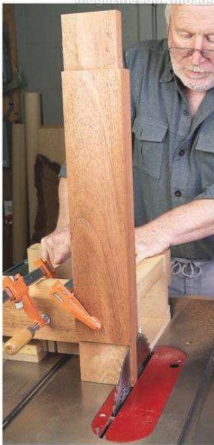
A block clamped in place on the front of the jig positions the rail to cut the cosmetic shoulder and avoids sawing into the jig.
