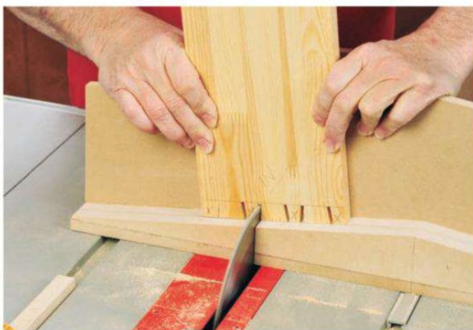
Figure 10: Spin the jig around front to back and cut the tails, using the ramps on each side of the jig to make the right- and left-hand cuts.
