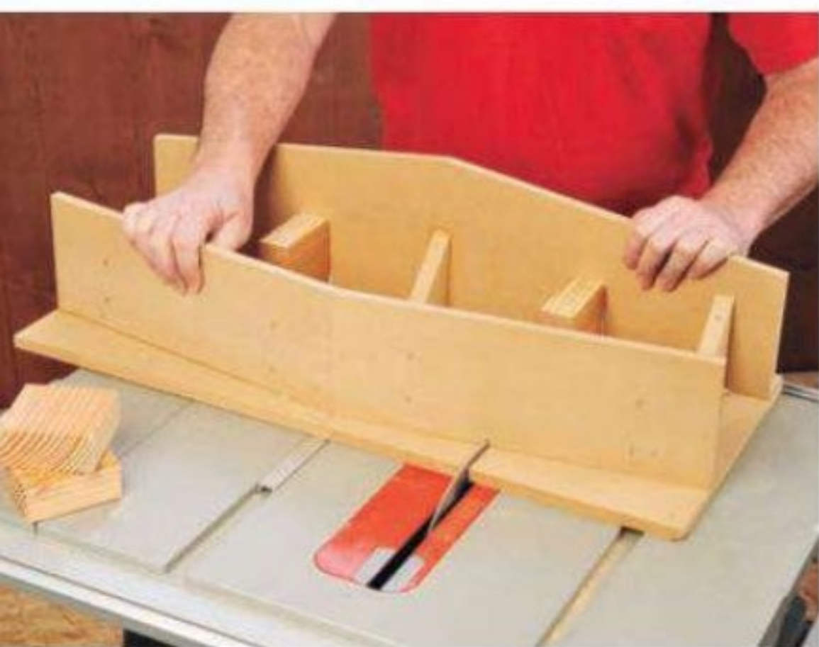
Figure 5: "Cutting in" a registration slot on all four of the jig's fences is essential for locating your dovetail cuts. Note the freshly glued-in blocks of wood: these cover the saw blade's exit points and protect your fingers.
