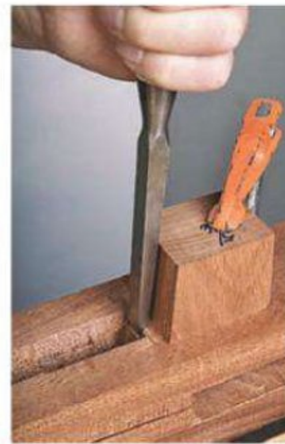
Put the leg in the vise on a support block and chop out the bulk of the waste using a mortise chisel (left). Complete the cut (right) by pressing a sharp bench chisel tight against the face of the angled guide block.
