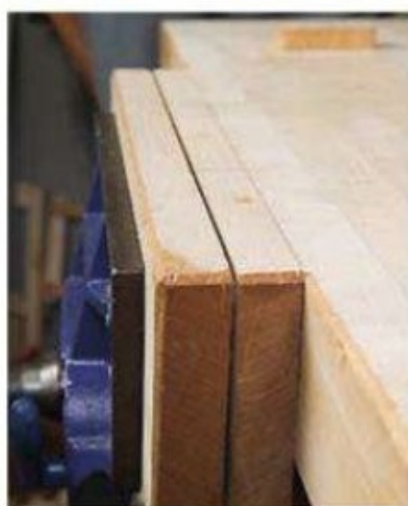
Make the fixed cheek square with the benchtop (top-left). A clamped workpiece should be square (top-right) with the top and vise cheeks parallel (right).
