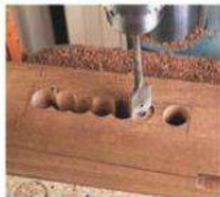
Use a 7/8" spade bit on center to leave 1/16" of waste on each mortise wall.
