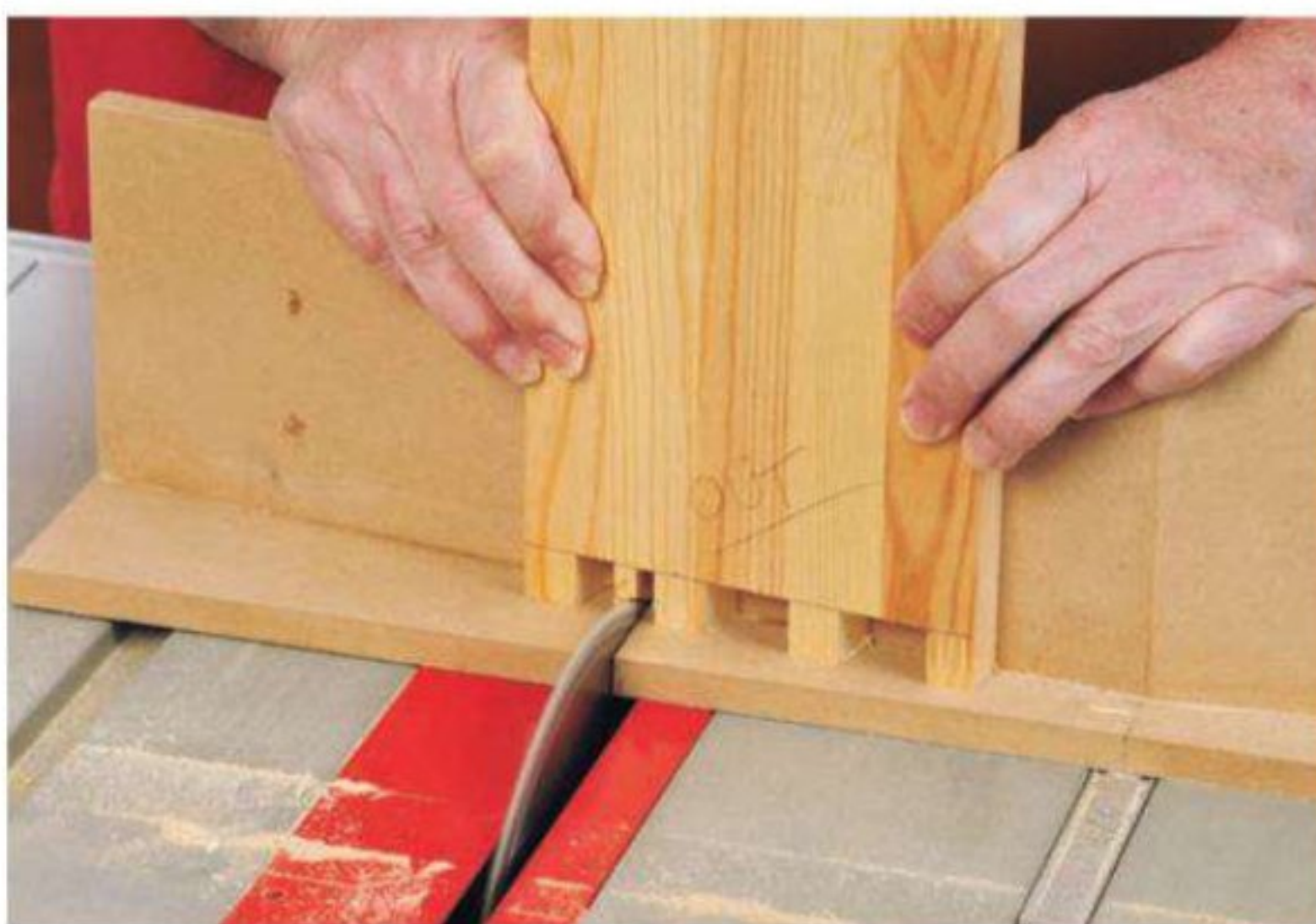
Figure 8: After establishing the left side of the pins, you can take multiple passes to remove the waste.
