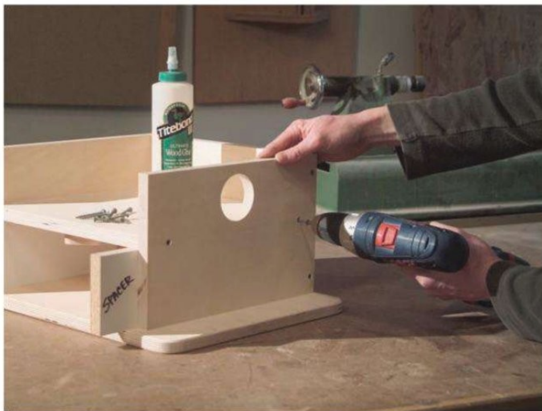
The author slips a pair of 4¼" -wide spacers inside the cabinet to position the divider while installing it. The spacers ensure that the 4" drawer sides will slide smoothly.
