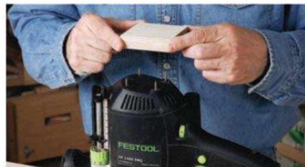
The author uses short wood screws, nested in the holes of his router's motor cap, to keep the router lift plate from spinning when cranking it up and down. Here, he's marking the screw positions on the lift plate.
