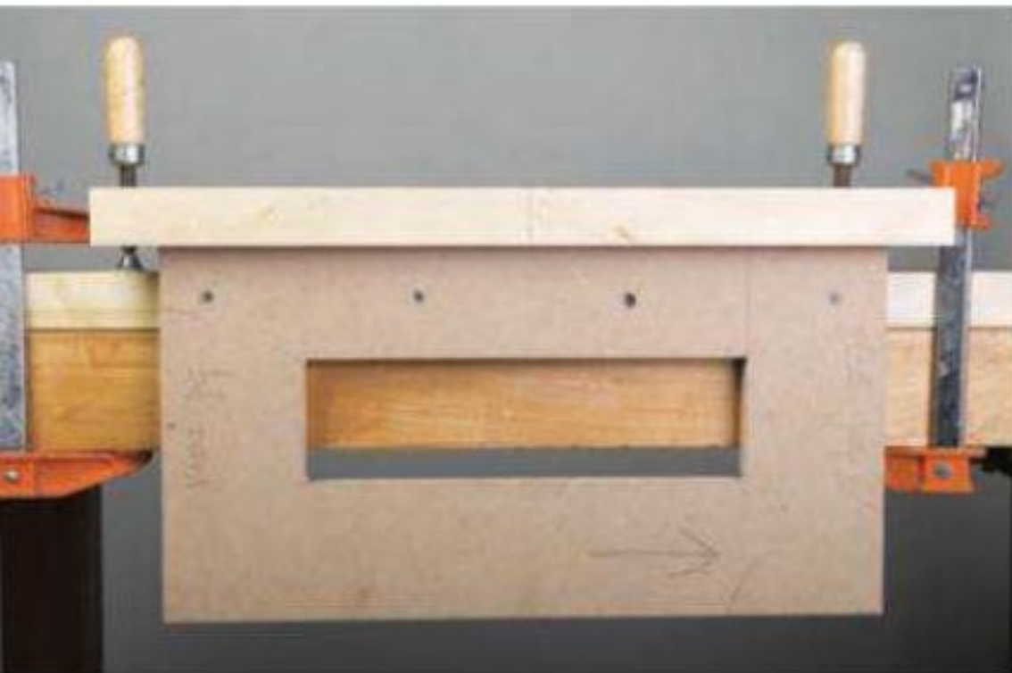
Begin the vise installation by clamping the pattern jig for routing the vise mortise in place to the benchtop.
