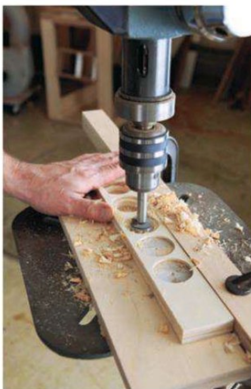
Drilling the two-step borings in the top pieces of the tool holders is most easily completed on a drill press. It can be done with a handheld drill, but it's just a bit trickier.
