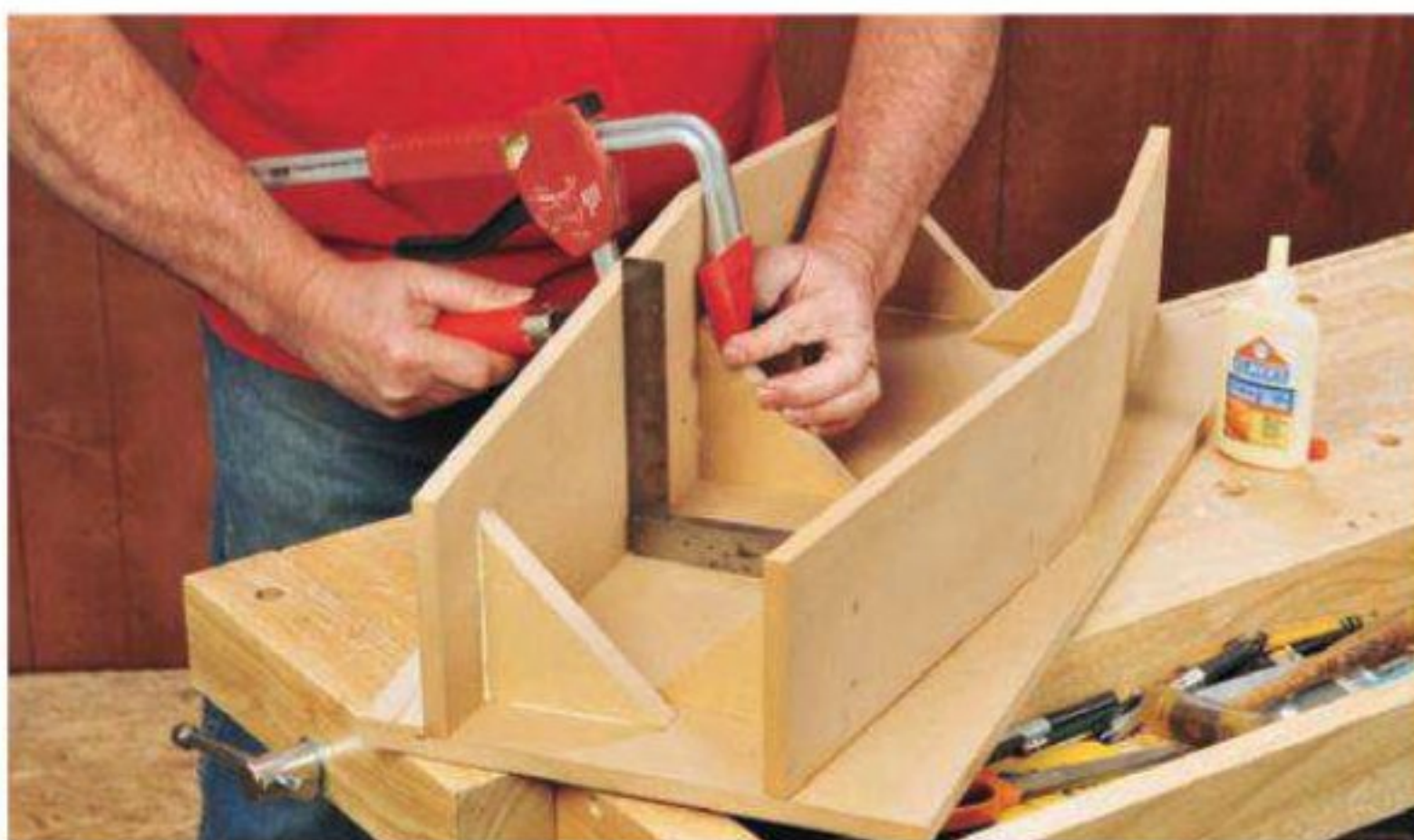
Figure 3: Braces keep the tail fence perpendicular to the base.
