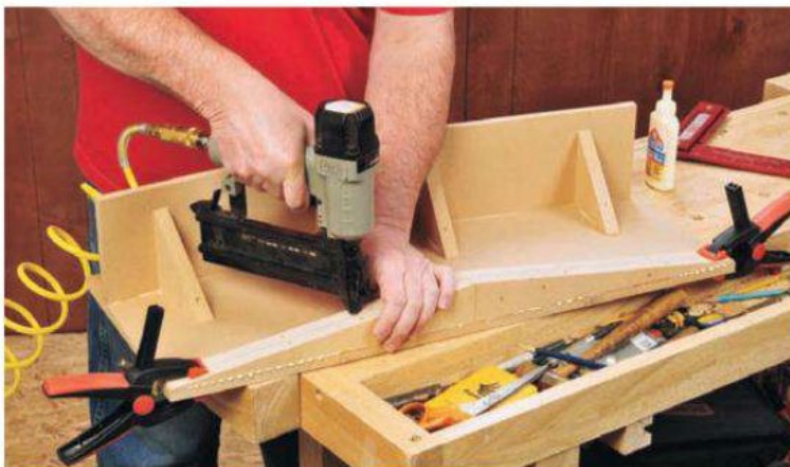
Figure 2: The 8° wedge ramp is formed from two 3/4" pieces.
