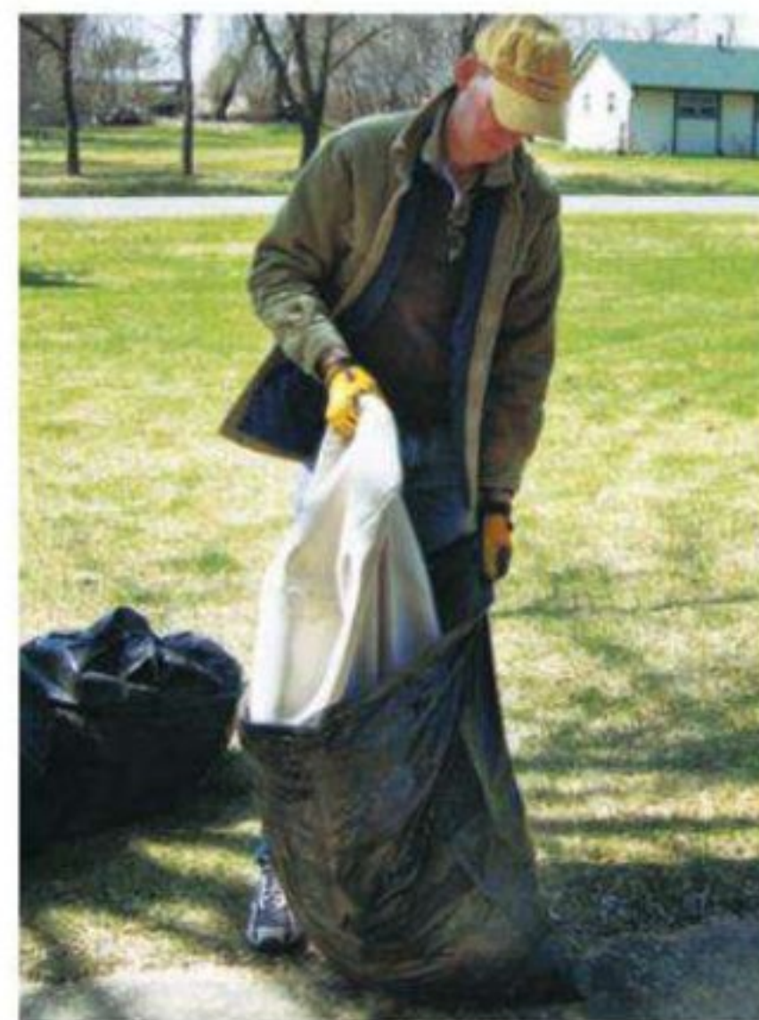
Left: Vigorously shaking out a dust collector bag might, our expert warns, eliminate its “healthy cake.” It’s best to gently empty and shake the bag into a trash bag (right) and call it a day.
