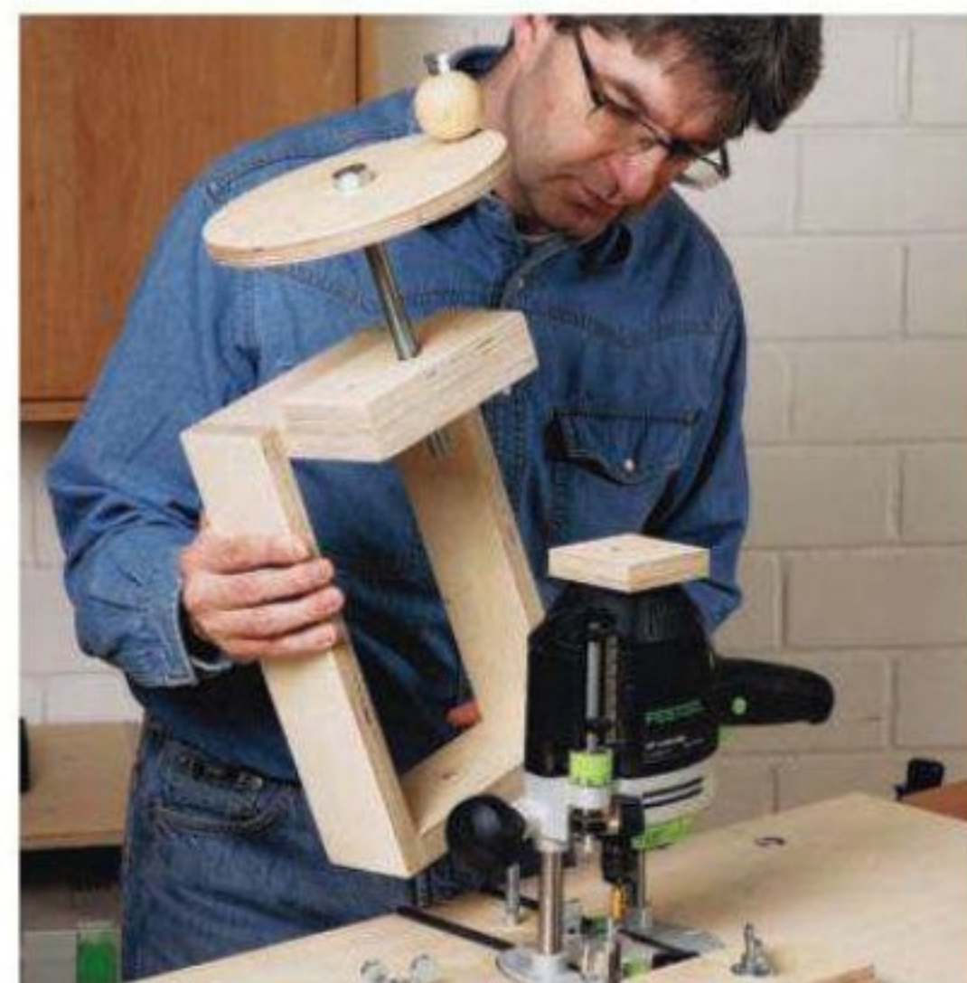
The router lift attaches to the table using the same carriage bolt as the rear mounting block. Tighten the wingnut to secure the lift, then crank the threaded rod until it seats against the router lift plate.
