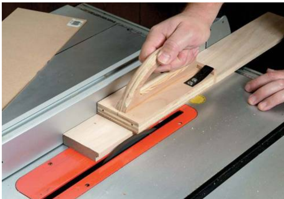
A rabbet can be cut on the edge of a workpiece in two passes on the tablesaw using a regular sawblade.
