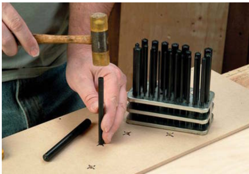
A transfer punch fits through a hole in a layout template to mark the precise location of the hole on the workpiece underneath.
