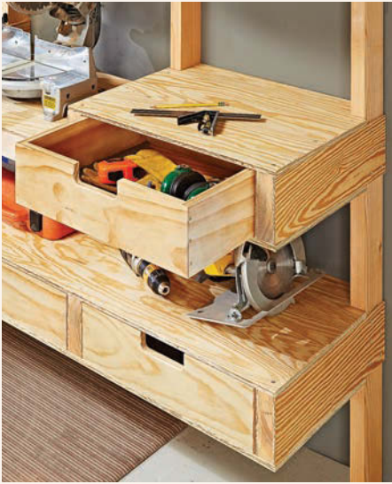
▲ Drawers. Simple to build rabbeted construction will give you solid drawers for storing tools and supplies.
