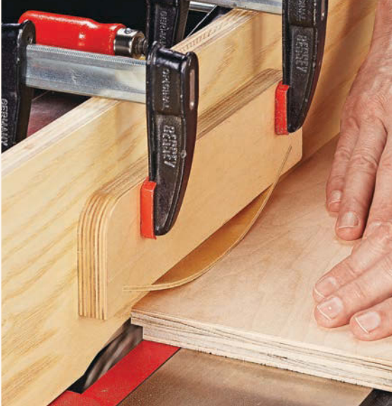
▲ Better Rabbets. A shop-made hold-down works just like a featherboard to ensure a consistent cutting depth when creating rabbets.
