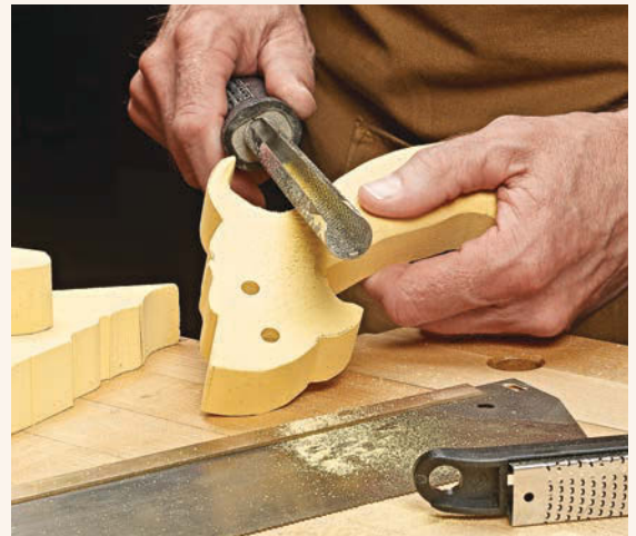
▲ Balsa-Foam. This lightweight foam cuts and shapes easily. Use a band saw or coping saw to cut it to rough shape, then smooth it with rasps.
