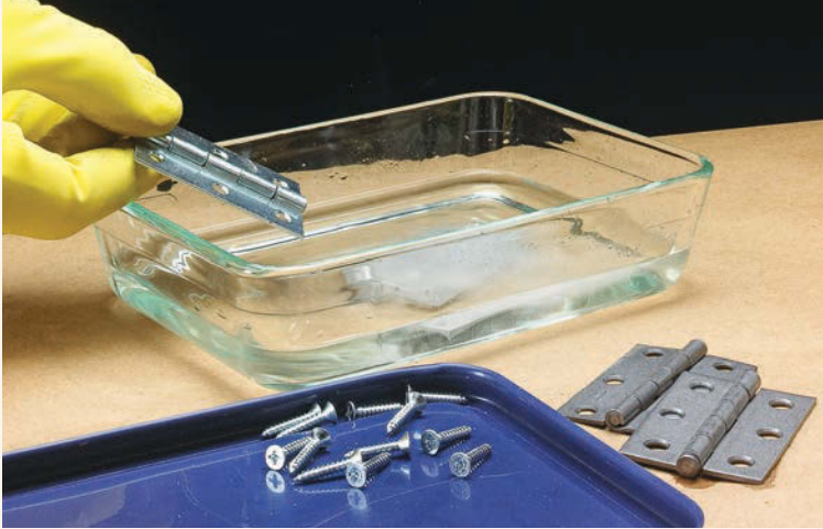
▲ Remove Zinc Plating. Diluted muriatic acid will remove the zinc plating from a hinge in just a few minutes. The result is a dull, bare steel surface with an old-time look.
