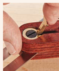
Cam secures blade position
