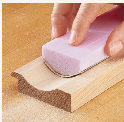
▲ Custom Blocks. Sanding curved profiles is hassle-free with a matching extruded polystyrene sanding block.
