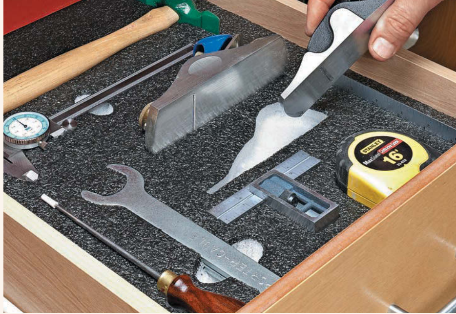
▲ Custom Drawer Liners. The density of polyethylene helps it to retain its shape, but it's also easy to cut. Here, I used a knife to cut out custom recesses for my tools to keep them organized and in place.
