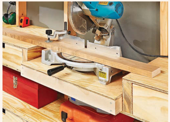
▲ Install the Miter Saw. A platform for the saw raises it so it's level with the shelf but still allows you to pick up the saw and move it to another location as necessary.
