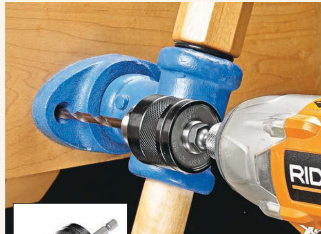
▲ Impact Driver Adapter. Rated for impact use, this adapter adds a 3-jaw chuck to your impact driver so you can use standard drill bits.
