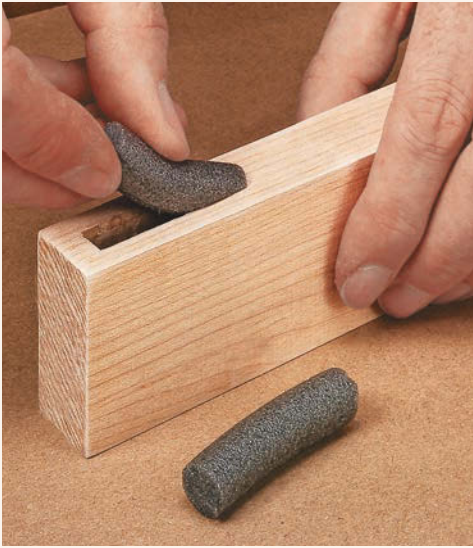
▲ Plugs. Prefinishing parts makes the finishing process easier. Plug openings with backer rod to keep out finish.
