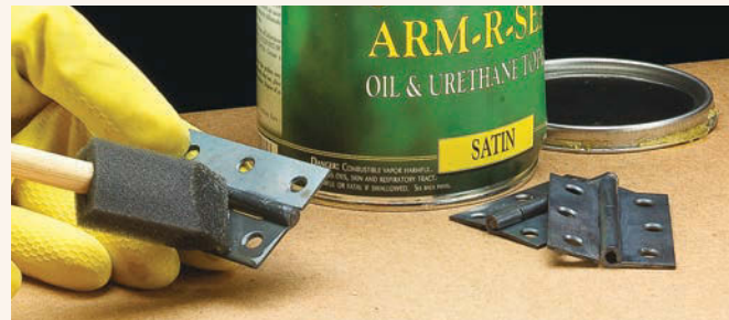
▲ Enhance It With Oil. After applying a coat of oil-based finish, use a torch again to burn it. Buff out the surface once it cools and dries.
