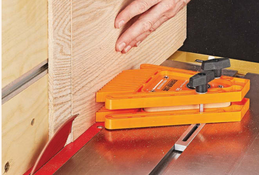
▲ Stack Them. Double up a pair of featherboards to create a taller support system when cutting wide workpieces that are held on edge. Position the featherboards ahead of the blade.
