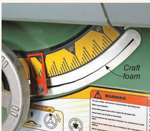
▲ Seal Off Openings. Craft foam is useful for sealing off openings, as on this table saw, for more efficient dust collection.
