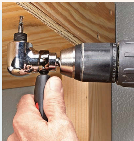
▲ Right Angles. This small attachment with a locking handle chucks into your drill or driver for driving screws in tight spots.
