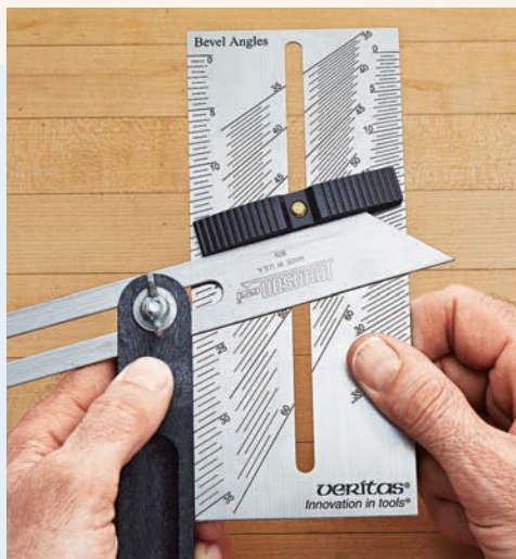
▲ Bevel Setter. Align the blade on the bevel gauge with the fence.
