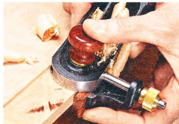
▲ Special Features. A rabbet plane cuts tight into a corner while the fence helps maintain the width of the bevel along the panel's edge.
