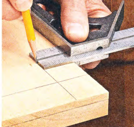
▲ Face Lines. Lines on the face of the panel act as the goal line to determine the overall width of the bevel.
