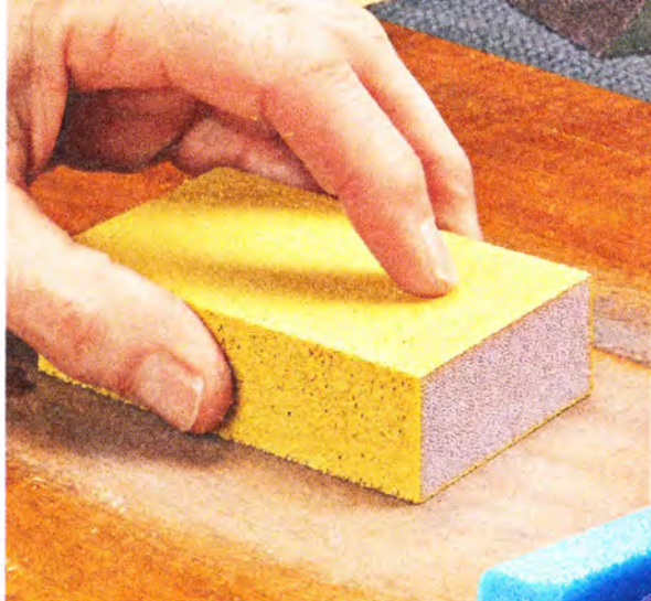
▲ Sanding Sponge. A 320-grit sanding sponge is ideal for leveling coats of finish.
