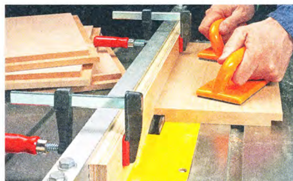
▲ Clamp. The simplest way to attach an auxiliary fence is to clamp it to the rip fence. But this only works if your workpiece will fit under the clamps.
