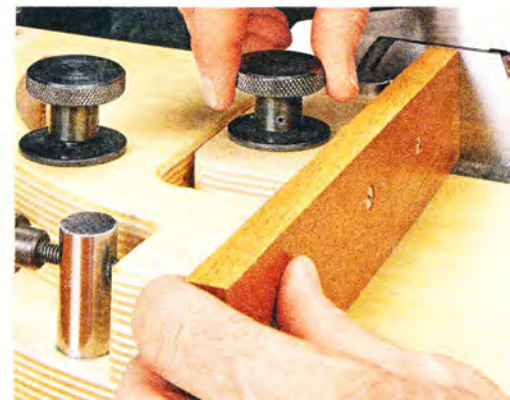
▲ Adjust the Fence. Loosen the knob to butt the adjustable fence up against the sole of the plane.
