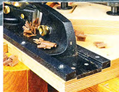
▲ UHMW. Soft UHMW is kind to bits and blades (main photo). Reprocessed UHMW is a less expensive alternative, as shown in the inset photo.
