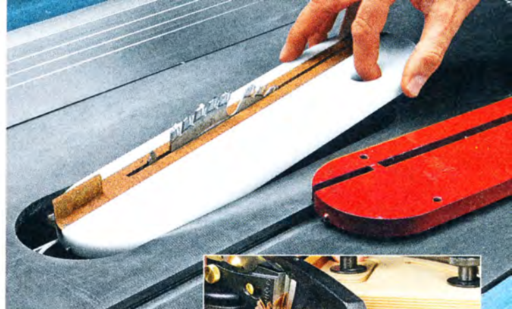
▲ UHMW. Soft UHMW is kind to bits and blades (main photo). Reprocessed UHMW is a less expensive alternative, as shown in the inset photo.
