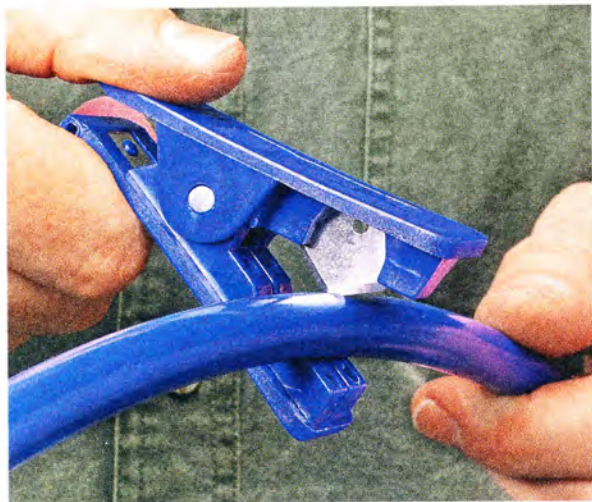
▲ Cutter. An included tool makes it easy to cut the tubing square for an air-tight fit.
