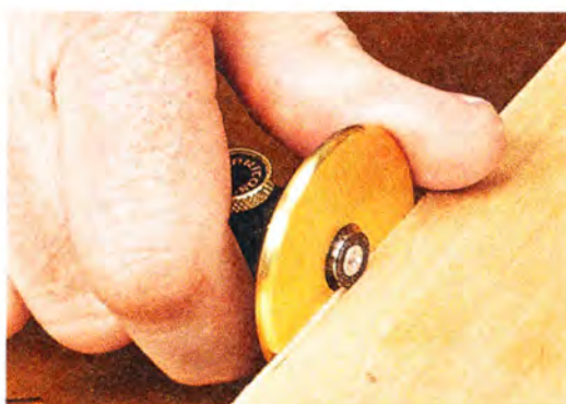
▲ Mark the Depth. I like to use a marking gauge to score the final depth of the hinge mortise before removing the waste.
