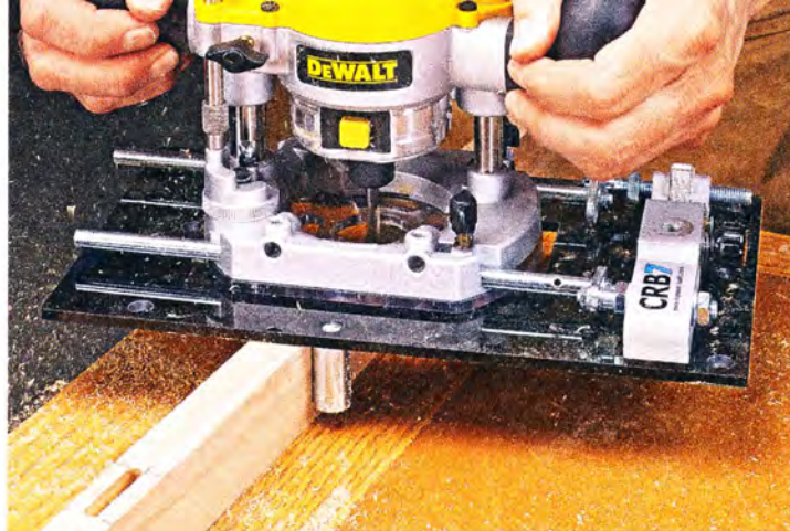
▲ Mortising. Two pins on the underside of the base ride against opposite faces of the workpiece to rout a mortise. The micro-adjuster lets you dial in the exact mortise location.
