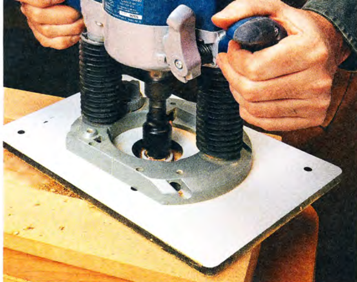
▲ Phenolic. Strong and stable, phenolic is a good choice for a number of shop accessories like router table insert plates. It's unaffected by humidity and stands up to heavy use.
