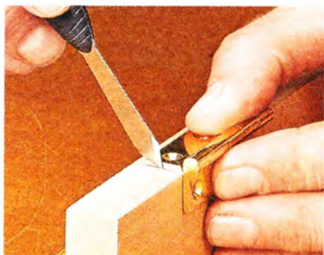
▲ Mark the Outline. A sharp knife makes quick work of scoring deep lines for crisp mortise edges.
