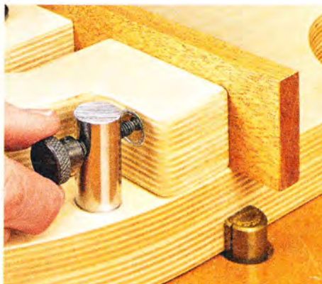
▲ Fine Adjustment. With the locking knob loosened, fine-tune the angle of the fence by turning the micro-adjuster.
