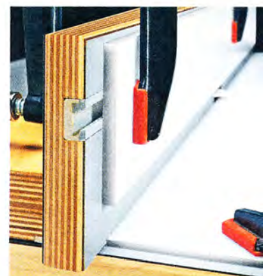
▲ HDPE. This material makes ideal spacers with its precise thickness.
