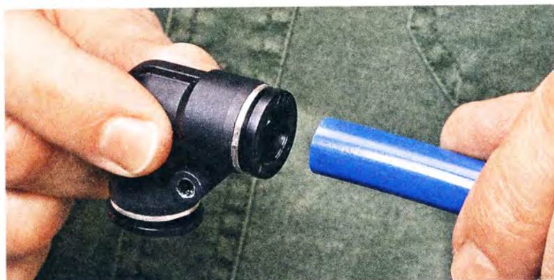
▲ Push to Connect. To install the tubing, simply push the squared-up end into the fitting until it's firmly seated.
