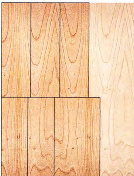
▲ Efficient. Cutting pieces for the most yield from a sheet sacrifices the appearance of the parts.
