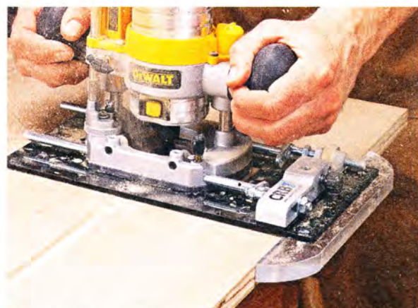
▲ Edge Guide. This optional attachment allows you to rout dados, grooves, and other profiles parallel to the edge of a workpiece with precision.
