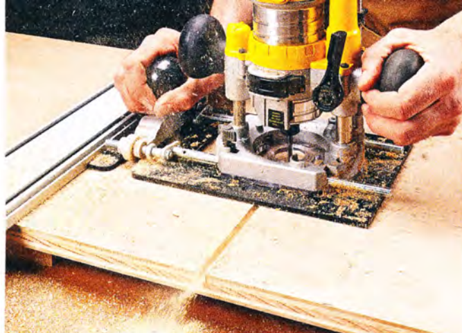
▲ Straightedge. The edges of the router base make it ideal for use with a straightedge guide. The router's position on the base can be fine-tuned for accuracy.
