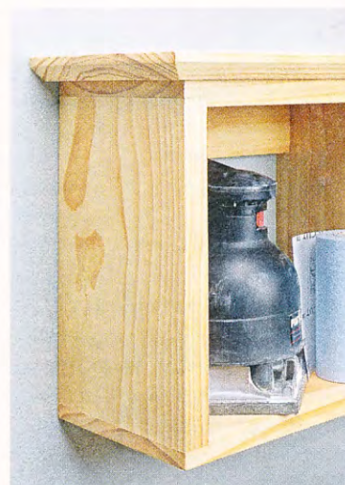
▲ Wall Shelf. Rabbets and dados make building this shelf a quick and easy task.
