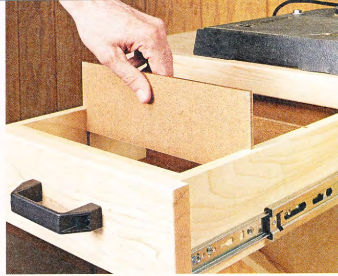
▲ Drawer Organizers. Slip hardboard dividers into dadoes in the drawer sides to organize the contents and make items easier to find.
