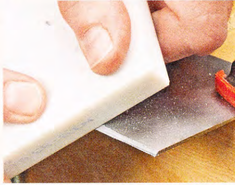
▲ Hone the Edge. An oilstone removes the mill marks left by the file and creates a razor-sharp edge.
