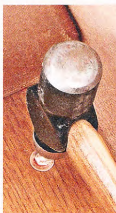
▲ Plywood Bottom. Cut the plywood to size before rounding over the long edges on the bottom and drilling the holes for the rivets. Finally, peen the rivets flat on the inside of the bag.
