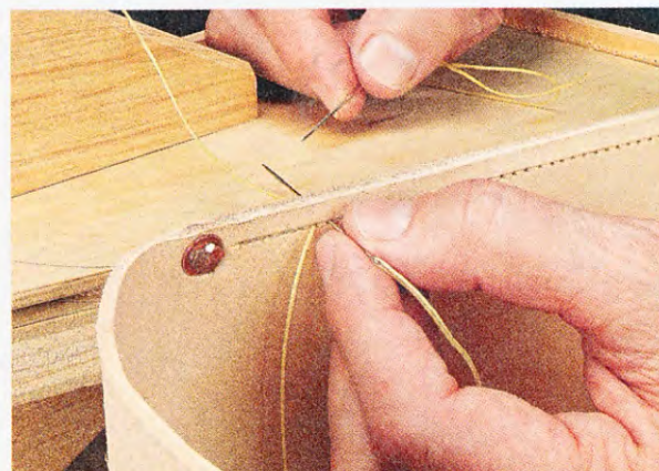
▲ Double Stitching. Saddle stitching is a strong and easy way to secure leather. Simply pass each end of the thread through each hole.
