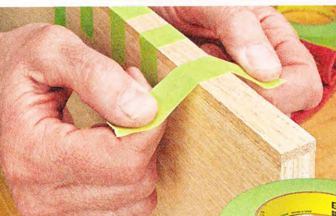
▲ Scotch 233+. This stretchy masking tape is great for tasks like gluing on edging.
