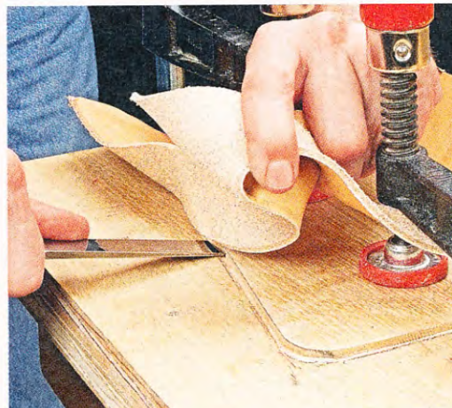
▲ Trim to Shape. After tracing the outline of the arc on the leather, trim the excess with a sharp chisel, bevel side down.
