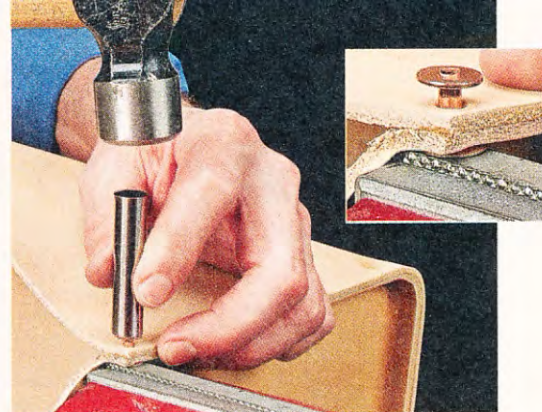
▲ Installing Rivets. Use a rivet-setting tool to set the burr on the rivet before peening the rivet shaft over the burr.
