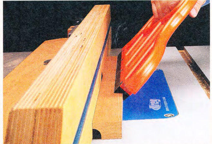
▲ Push Stick. The angled shoe on this push stick lets you apply pressure down and in on a narrow workpiece. A heel at the back pushes the workpiece past the bit.
