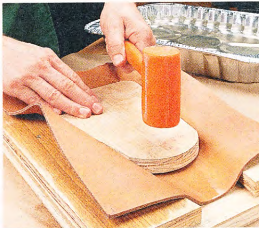
▲ Press Block. Seat the press block firmly by tapping it in place with a mallet, making sure the rounded edge is face down.
