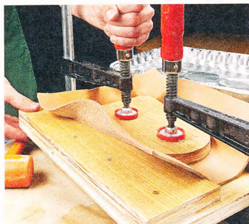
▲ Clamp & Dry. Clamp the press block securely and allow to dry for two or three days before removing the clamps.
