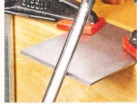
▲ Roll a Hook. The real cutting edge of the blade is the hook. Use a burnisher at the tip of the blade (see detail below).
