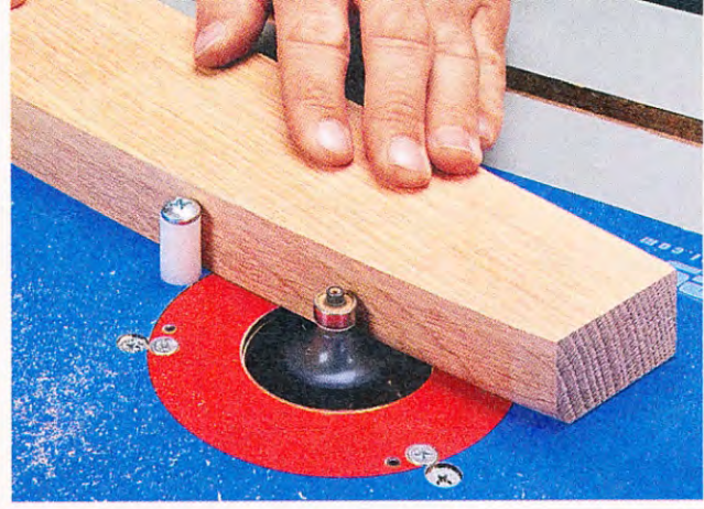
▲ Starting Pin. Use the starting pin as a pivot point to increase your control of a workpiece when routing curved parts on the router table.
