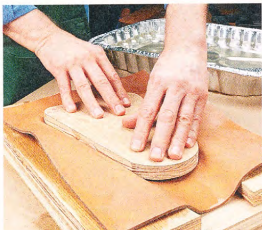
▲ Forming the Ends. After soaking the leather in room-temperature water, place it in the form, rough side down.
