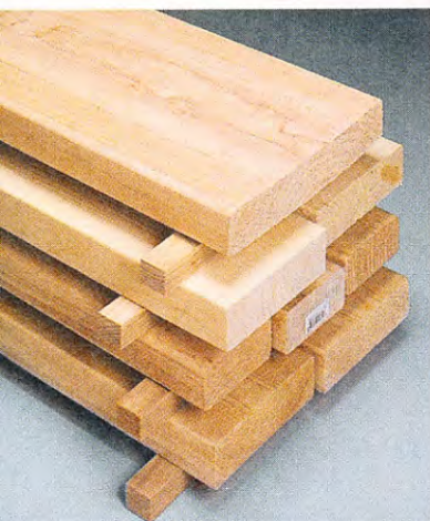
▲ Dry & Stable. Construction lumber needs to dry before you can use it in a bench.
