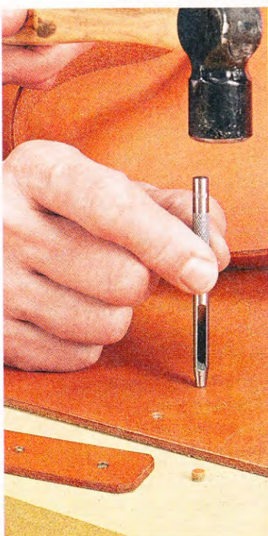
▼ Punch. Use an \frac{1}{8} " hollow punch to make holes for installing the handle and buckle straps.
