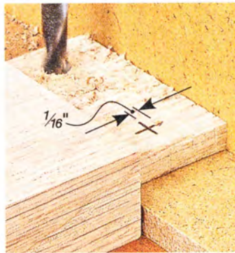
▲ Tenon Holes. Drill holes in the tenon approximately \frac{1}{16} " closer to tenon shoulder.
