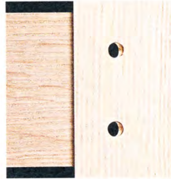
▲ Offset Holes. The offset holes are visible when viewed through the mortise holes.
