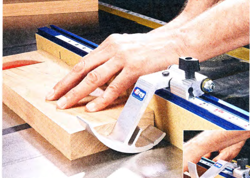
▲ Kreg Swing Stop. The sturdy stop flips up out of the way or, more conveniently, slides out of the way when making initial rough cuts (right).
