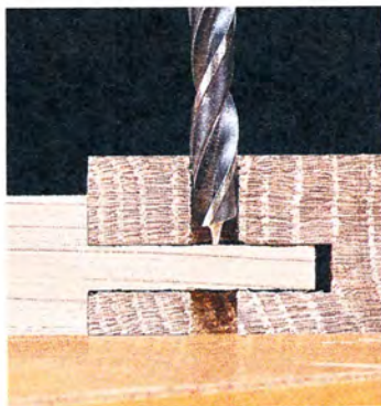
▲ Mark Tenon. Locate the centerpoint of the mortise holes on the tenon.
