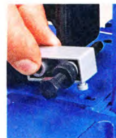
▲ Adjustable Stop. The workpiece stop snaps into keyhole slots in the jig's base.
