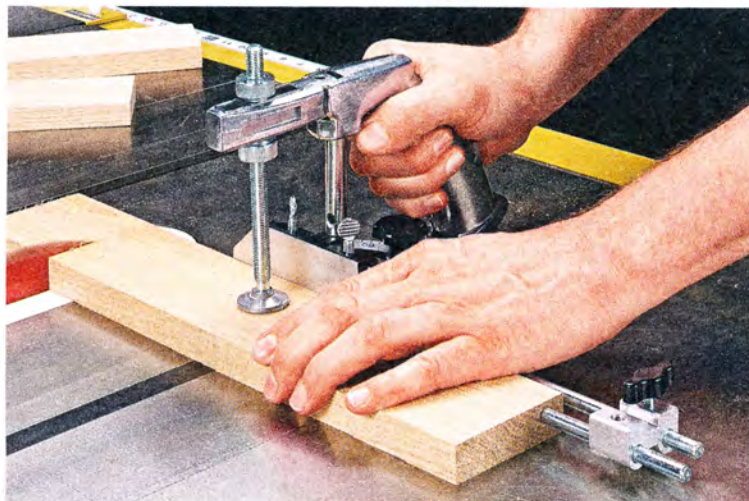
▲ Squeeze Action. This aftermarket miter gauge includes a hold-down and adjustable stop. Squeeze the handle to firmly clamp the workpiece during the cut.
