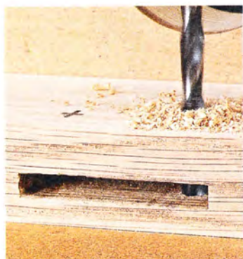
▲ Mortise Holes. Remove the tenon and drill holes through the mortise.
