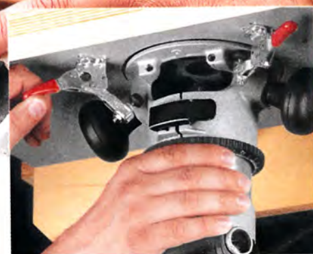
▲ Toggle Clamps. Release the clamps to switch to use the router hand-held routing tasks.
