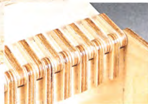
▲ Routing Hinge Recesses. A CNC router is perfect for tedious tasks like routing all of the recesses for the hinge knuckles to attach the lid, as shown in the inset photo.
