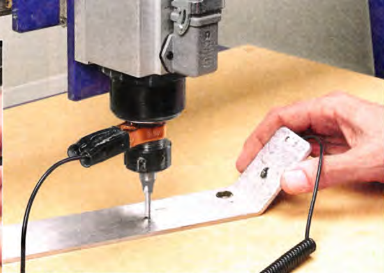
▲ Zero the Z-Axis. After installing a bit in the spindle (left), use the touch plate (above) to tell the machine where the zero point of the Z-axis is located.
