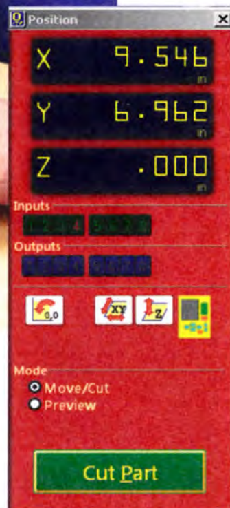
▲ Status. This window tells you the status and location of the end of the router bit.
