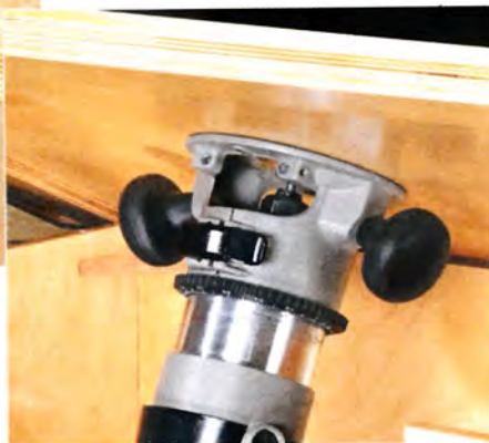
▲ Direct Approach. Long screws thread through the table into the router base. A hinged top makes access easier (right).
