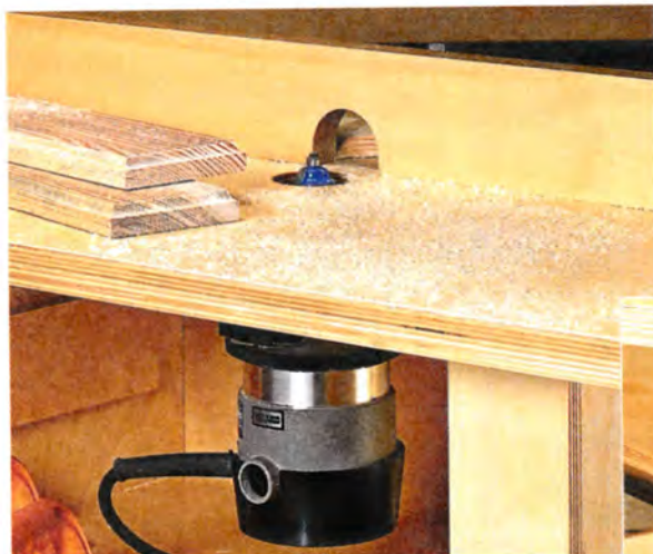
▲ Direct Approach. Long screws thread through the table into the router base. A hinged top makes access easier (right).
