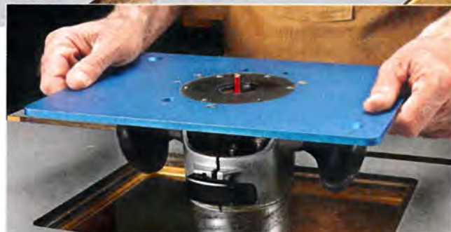
▲ Insert Plate. Bolting the router to an insert plate provides ready access (right).
