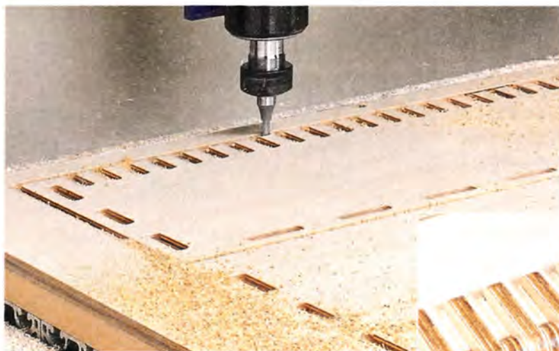
▲ Routing Hinge Recesses. A CNC router is perfect for tedious tasks like routing all of the recesses for the hinge knuckles to attach the lid, as shown in the inset photo.
