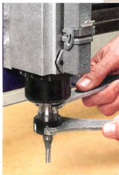
▲ Zero the Z-Axis. After installing a bit in the spindle (left), use the touch plate (above) to tell the machine where the zero point of the Z-axis is located.
