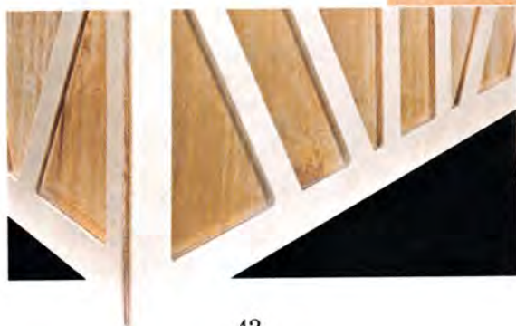
▲ Pocket Cuts. The decorative pocket cuts in the toolbox (left) are cut in two shallow passes (above).
