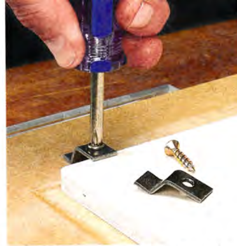
▲ Attaching a Workpiece. One of the keys to success is making sure the workpieces are secure. Here, Z-clip fasteners do the trick.
