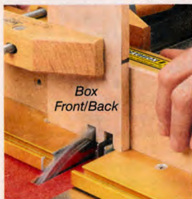
▲ Front/Back. Make the first cut with the piece against the pin, then cut the remaining notches.
