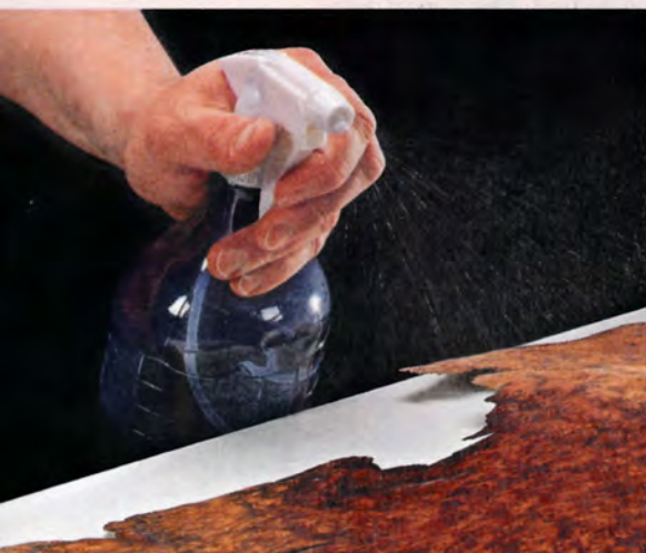
▲ Spray with Warm Water. Water mixed with glycerin quickly softens the fibers of thin, brittle veneer so it can be flattened.
