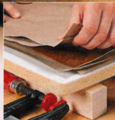
▲ Veneer Press. Moisten the veneer before sandwiching it between paper to press it flat.
