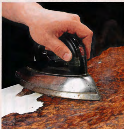
▲ Iron It Flat. A clothes iron set on medium can be used to quickly press the waves out of a piece of veneer.
