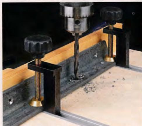
▲ Heavy-Duty Hold-Downs. For drilling in metals, I like to use heavy-duty hold-downs in case the bit catches.
