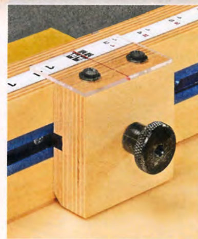
▲ Stop Block. Align the cursor with the tape for repeatable and accurate cuts every time.
