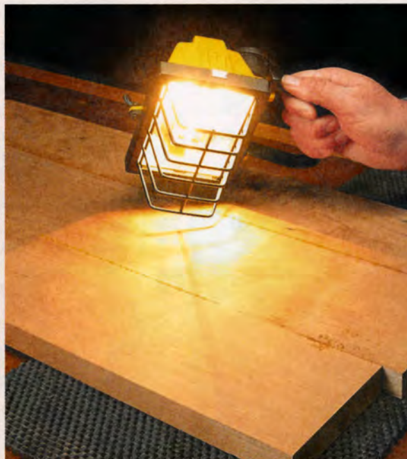
▲ Raking Light. When sanding or applying a finish, shine a light at a low angle across a workpiece to highlight surface flaws.
