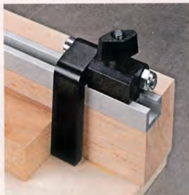
▲ Flip-Stop. For cutting several workpieces to identical length, a stop is the answer.
