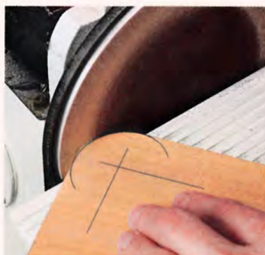
▲ Final Smoothing. Use a disk sander to carefully smooth the arc to the layout line.
