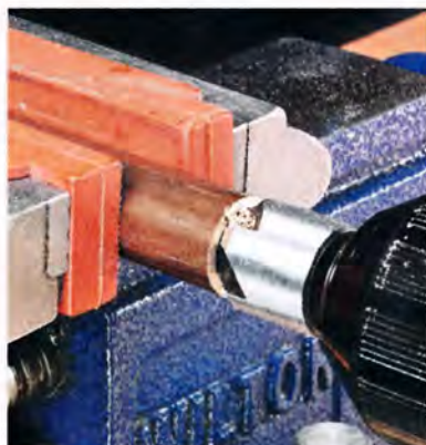
▲ Chamfering. A countersink bit makes quick work of forming a small chamfer.
