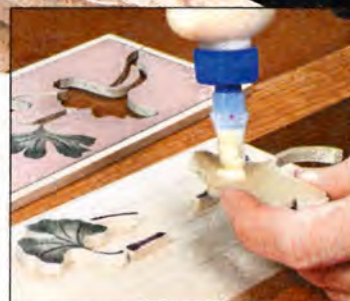
▲ An Original. Scroll-sawn pieces glued to a blank create an original pattern to be carved.
