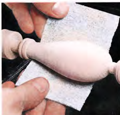
▲ Sanding. Remount the blank on its true centers to sand the handle smooth at low speed.
