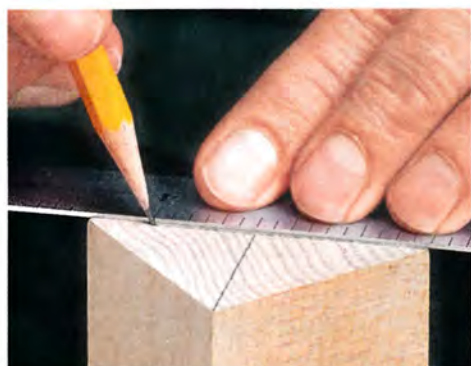
▲ Mark the Centers. Start by marking diagonals across each end of the blank to find the true center.
