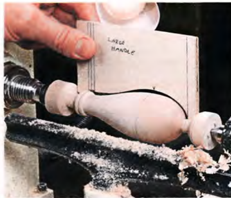
▲ Shaping. Check the size and shape of the teardrop handle shape by using the pattern as a visual guide.
