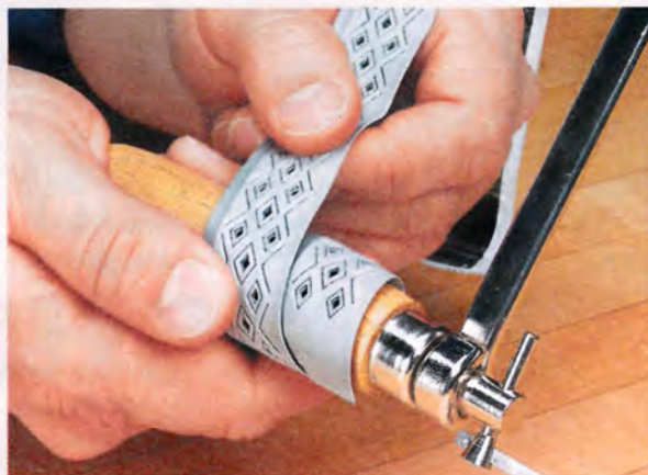
▲ A Better Grip. Instead of reshaping the handle, you can add athletic grip tape to create a cushioned handle that's easier to grasp.
