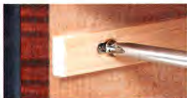
▲ Drawer Guide. A slot in the drawer guide creates a secure connection to the side panel.
