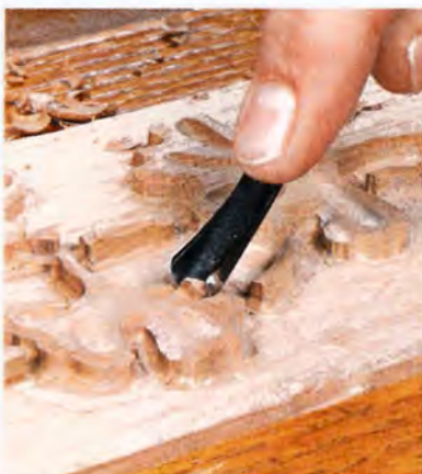
▲ Hand Work. You can use carving tools to add detail and create crisp edges.
