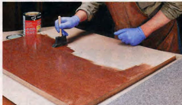
▲ Spreading the Adhesive. You don't need to be fast but you need to be thorough. It's a good idea to double-coat porous materials like MDF.
