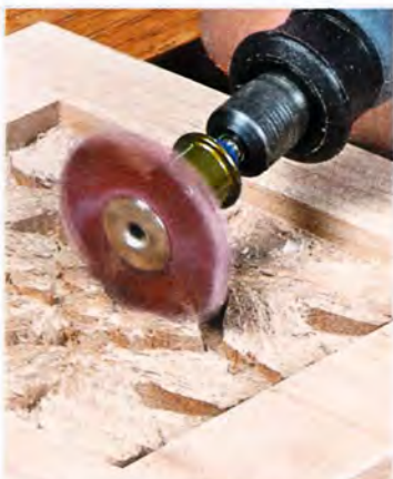
▲ Sanding. A detail sander on a rotary tool removes any remaining fuzz.
