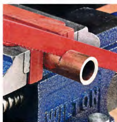
▲ Cut to Length. Cut the ferrule to length and then press it onto the tool handle (photos below).
