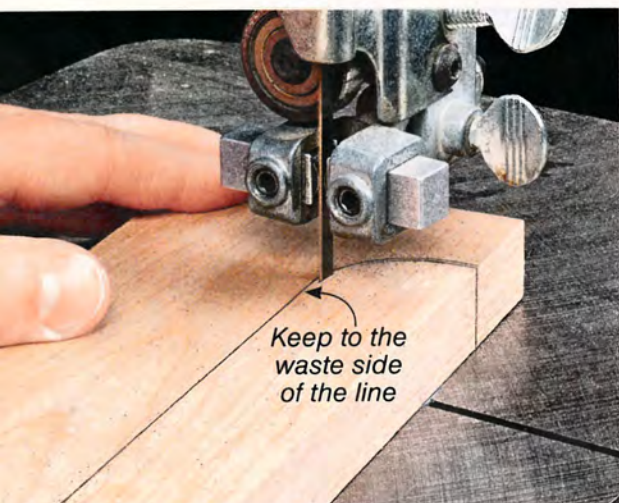
▲ Cut It Close. To save time and effort while smoothing, cut as close as possible to the layout line. Aim for \frac{1}{32} " to \frac{1}{16} " of waste.
