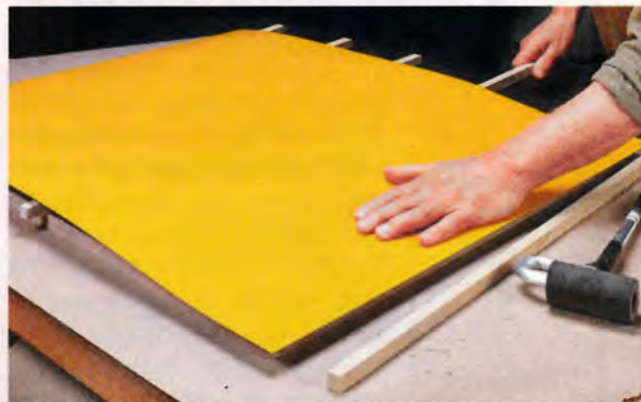
▲ Press in Place. With the laminate aligned over the substrate, start at one end and remove the strips in order, pressing it down with your hand.
