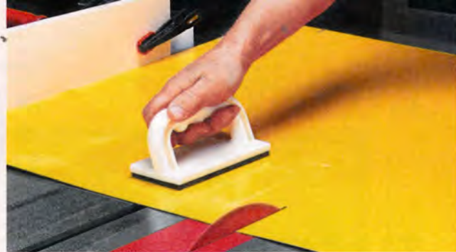
▲ Cut to Size. With an auxiliary rip fence fit tight to the saw's table, use a push pad to help feed the thin laminate and keep it flat.
