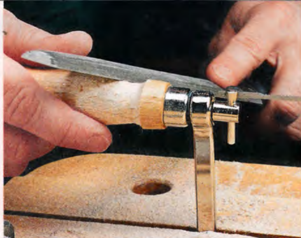
▲ Create a Comfortable Shape. Use files and sandpaper to reshape the handle so that it's more comfortable and less likely to slip.
