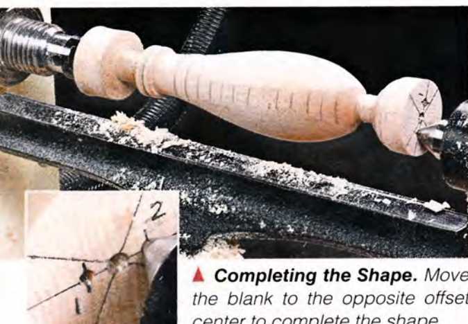
▲ Offset Turning. Switching to an offset center allows you to start forming the oval shape.
