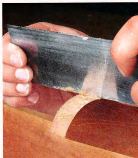
▲ Use a Card Scraper. The sharp hook on a card scraper quickly removes blade marks from curves.
