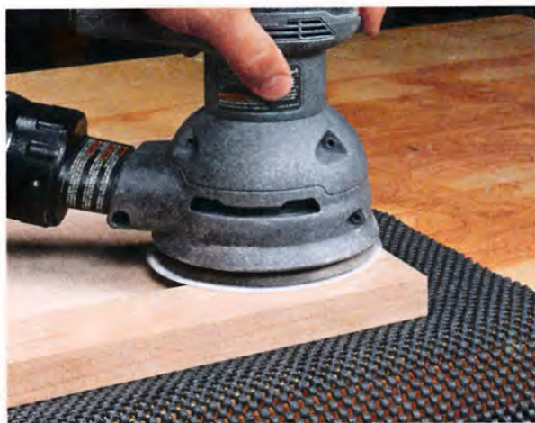
▲ Rubber Sanding Mat. The textured rubber mat creates enough friction to keep workpieces and assemblies in place for sanding or routing.
