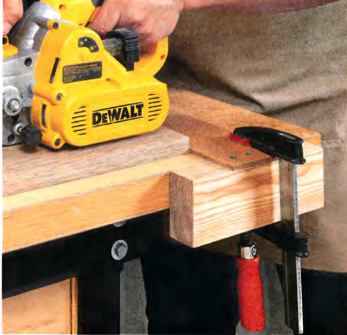
▲ Bench Stop. A thin hardboard strip creates a low-clearance stop that won't get in the way of tools. Use it to keep parts from sliding off the worksurface.
