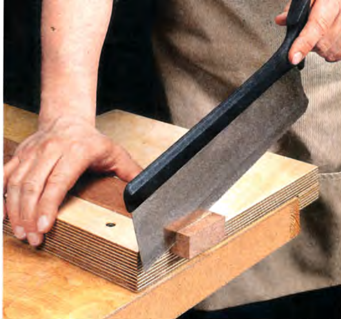
▲ Bench Hook. Brace a workpiece against the fence to cut parts to size or plane a chamfer. The platform can serve as a backer for drilling holes, too.
