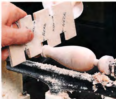
▲ Gauge. Monitor your progress by checking the diameter of the tenon, neck, and beads with the gauge.
