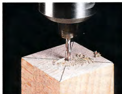
▲ Pilot Hole. On the opposite end of the blank, drill an \frac{1}{8} "-dia. pilot hole for the shaft of the tool.
