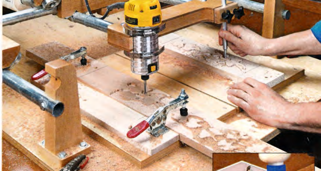
▲ Repeating Patterns. By installing a fence with hold-down clamps, you can create repeating patterns on a long workpiece. Use index marks to locate each section.
