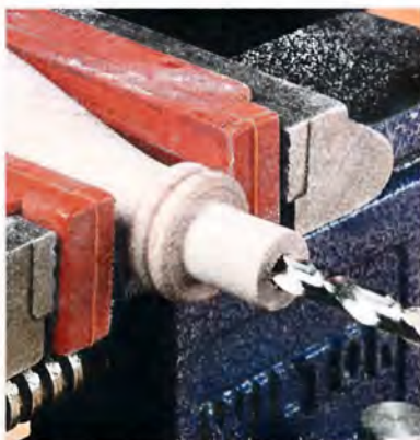
▲ Drill Shank Hole. Enlarge the pilot hole you drilled earlier to match the shank of the tool.
