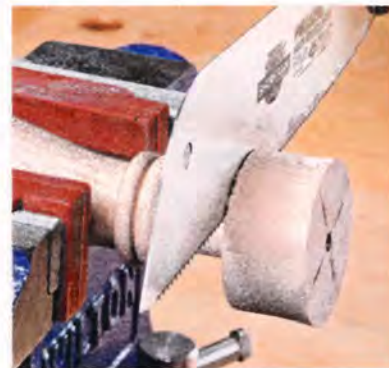
▲ Cutting Off the Waste. Use a hand saw to remove the waste at each end of the turning.
