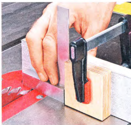
▲ Square the Block. The last thing to do before making cuts is to make sure the stop block is square to the table.
