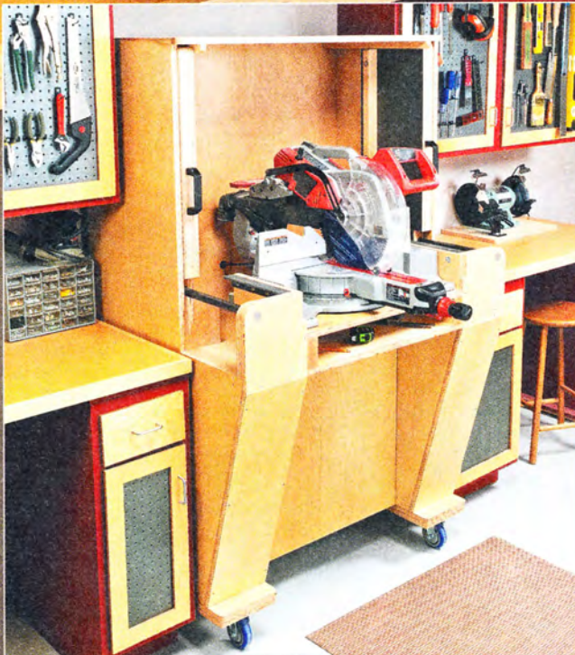
▲ Folded Up. When not in use, you can fold up the wings and slide them inside the cabinet.
