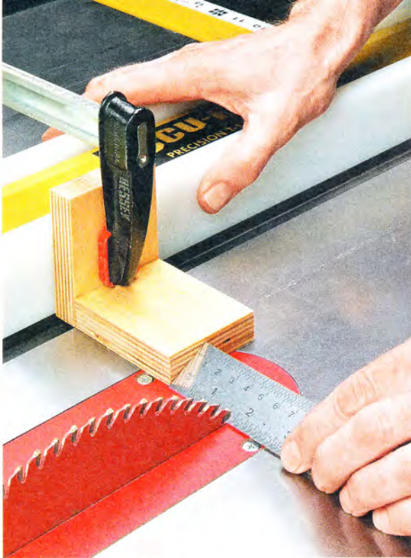
▲ Positioning. After aligning the stop block with the blade and clamping it in place, adjust the rip fence to set the distance from the blade.
