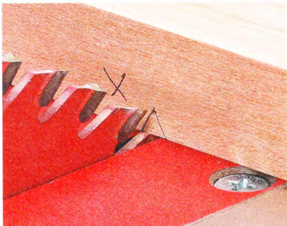
▲ Aligning the Workpiece. Take the time to position the workpiece by aligning your mark with the teeth of the saw blade.
