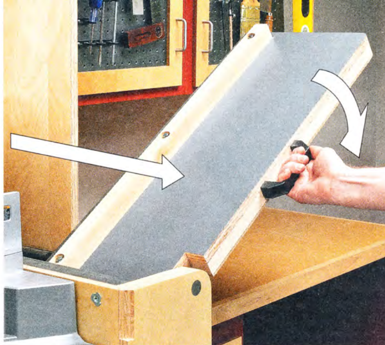
▲ Folding Wings. The wings are stored in the cabinet but slide out on the steel rod and fold down to support long workpieces.
