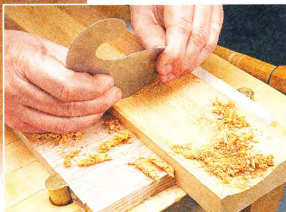
▲ Flat or Curved. Profiled scrapers allow you to smooth and refine convex and concave shapes.
