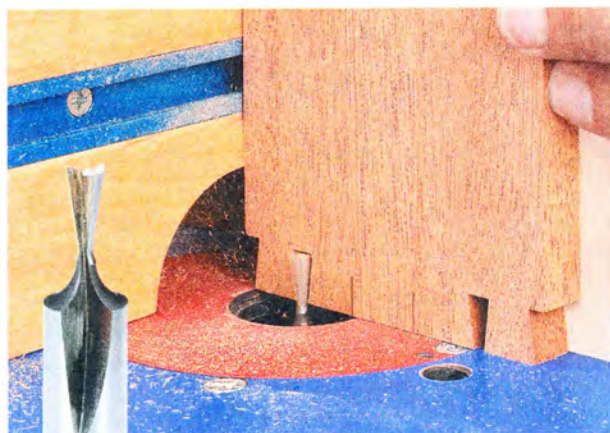
▲ Small Dovetail Bit. In the router table, this bit makes quick work of cutting tails with a handmade look.
