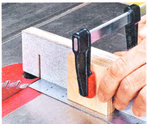
▲ Measure. Use a steel rule to position the stop block. Measure from the edge of one of the teeth on the blade.
