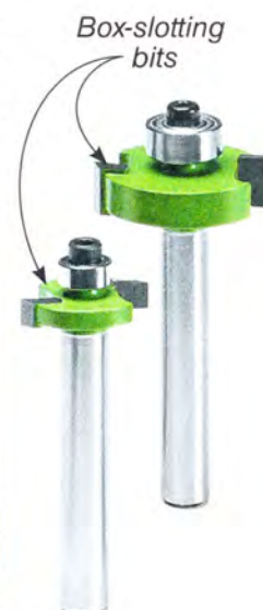
◀ Box-Slotting Bit. Dry clamp the box parts together to rout a bottom groove that won't be visible from the outside.
