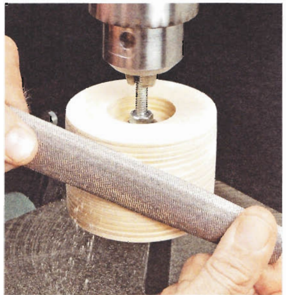
▲ Final Shaping. Use files and sandpaper to create a smooth surface. A slight camber helps the abrasive belt track properly on the rollers.
