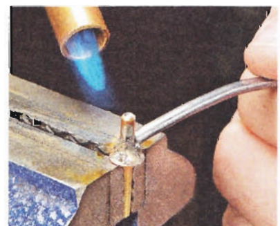
▲ Soldering. A quick soldering job creates a power button for the tablet case (below).
