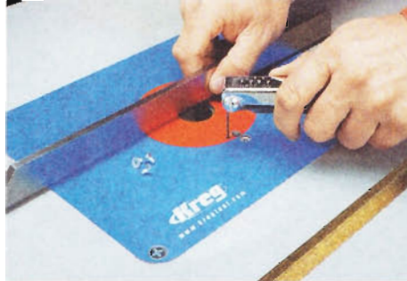
▲ Level Plates. Making sure the insert plate is level results in more accurate cuts and prevents a piece from catching.
