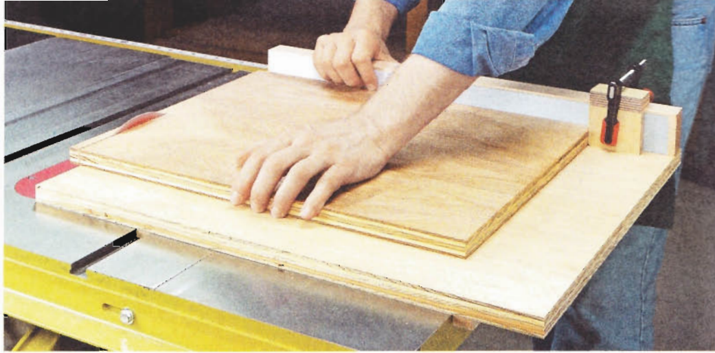
► Crosscut Sled. Make your table saw more versatile and more accurate at the same time with a crosscut sled. Whether you're cutting a small workpiece to final length or squaring up the end of a large panel, you can be certain it will be perfectly square.
