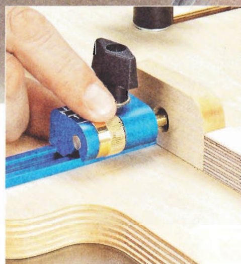
▲ Dial It In. A micro-adjuster lets you tweak the setup in precise amounts to create a good fit.
