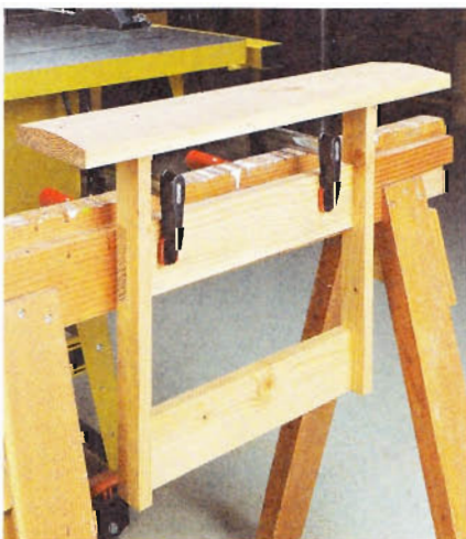
▲ Outfeed Support. Supporting the workpiece can be as easy as using this handy shop-made support.
