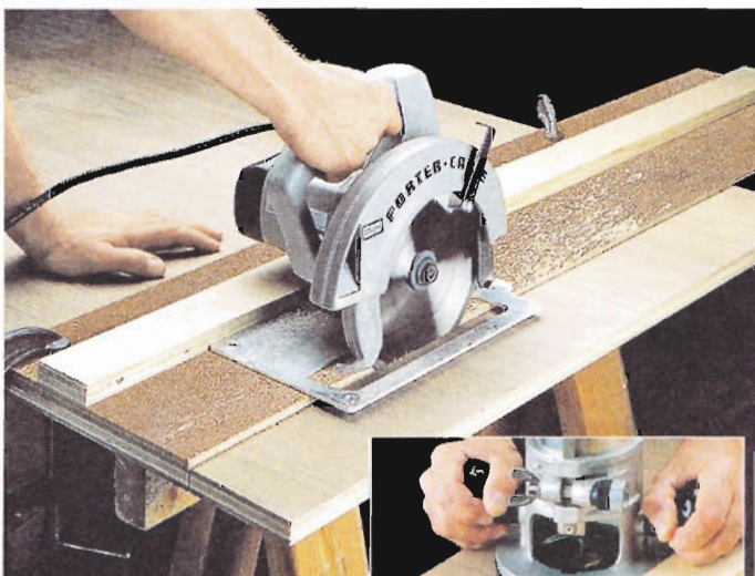
▲ Plywood Edge Guide. A shop-made edge guide makes using a circular saw more accurate. The opposite edge of the jig doubles as a router guide.
