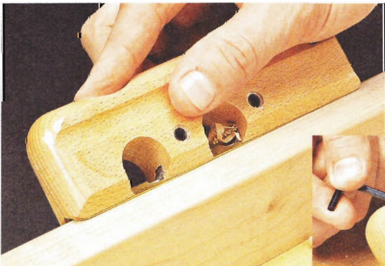
▲ Two Blades. The front blade makes a lighter cut while the rear blade creates the final profile (photo above). Adjust and replace blades using the included Allen key (photo at right).
