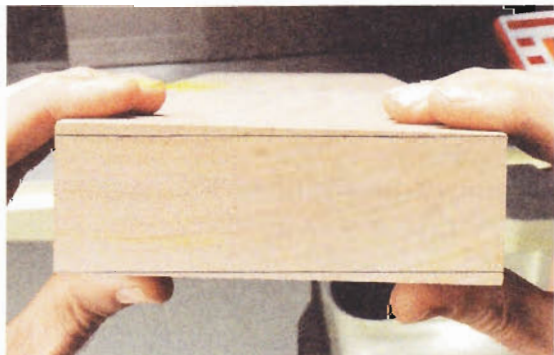
▲ Twisted Lumber. A few passes on the jointer will remove the "proud" corners of a twisted board and leave a flat face ready for planing.
