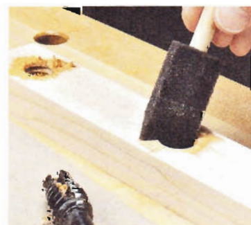
▲ Lubricate. Apply a little oil to the pilot hole to reduce friction while tapping threads.
