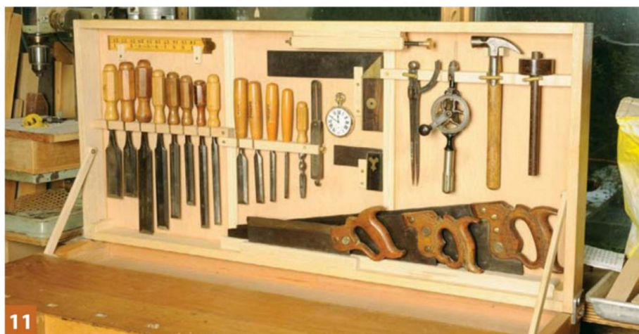
11 The inside of the lid shows the sectioned construction and the way all these lovely tools have fitted into it. Also note the spring catch at the top for locking the lid down on the completed workbench
