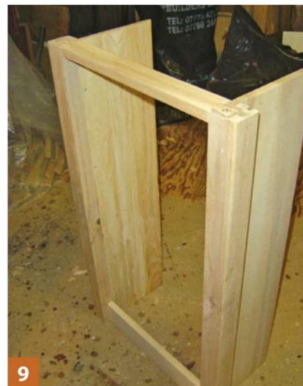
9 One of the assembled carcasses ready to fit together with the linking rails in-between
