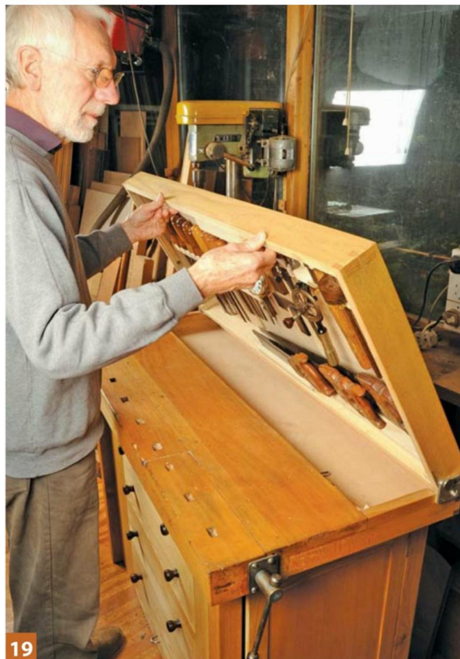
19 Demonstrating how the lid raises and lowers without any tools falling out!
