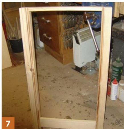
7 The rebate for the ash panels is visible in this view
