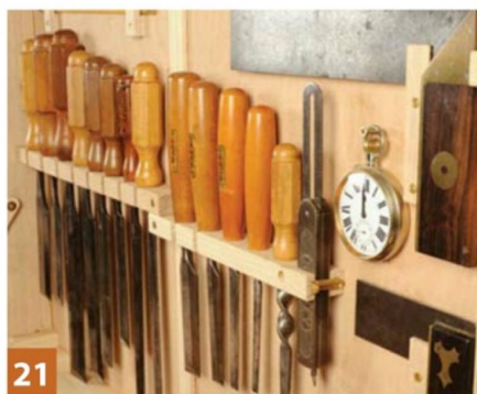
21 The holding method for the chisels is conventional, it just requires care in slotting the rail so the chisels cannot come loose
