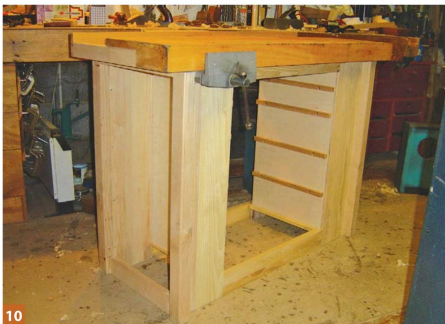
10 The carcasses now in place showing the as yet unfitted left-hand one and simple drawer runners installed in the middle to take the wide tool drawers
