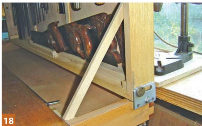
18 The unusual custom-made sliding hinge arrangement that allows the lid to move from closed to upright position and is held open by two simple stays
