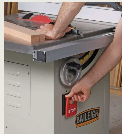
Long reach for the power switch. Located beneath the height adjustment wheel, the switch requires you to lean over too far.
