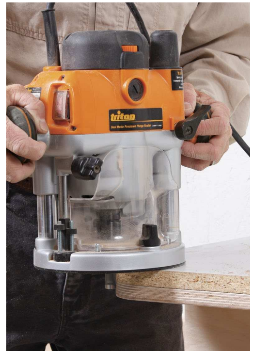
Add the countertop. After roughing out the corner radius of the countertop, screw it to the subtop from below, then rout the chipboard top flush to the subtop.
