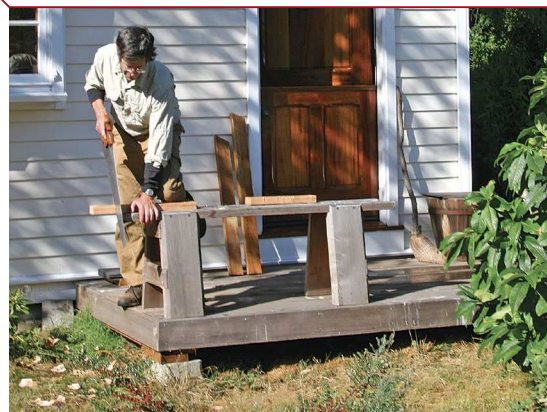
Outdoor sawing. A saw bench on the porch is where Tolpin cuts raw stock to rough size before taking it into the shop. The bench is also useful for roughing stock with a hatchet.
