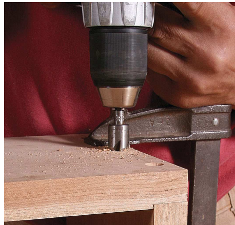
Countersink last. For flathead screws, use a countersink bit to cut a conical recess for the screw head.
