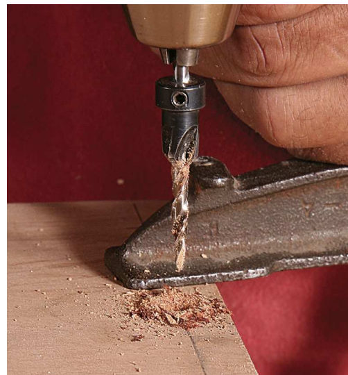
Countersink last. For flathead screws, use a countersink bit to cut a conical recess for the screw head.
