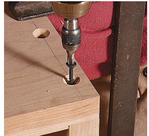
Then drive the screw. Accurate, tight, split-free screw joints result from proper predrilling.
