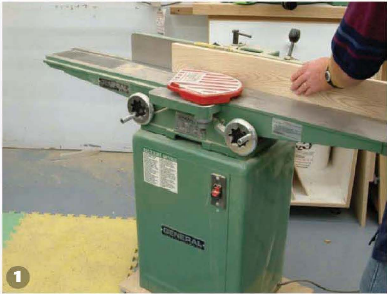
STEP ONE Cut a length of solid wood \frac{3}{4} " x 3\frac{1}{2} " x 48" (19mm x 89mm x 1219mm). This guide board must have parallel edges, so if you don't have a jointer ask your lumberyard to joint the edges for you.
