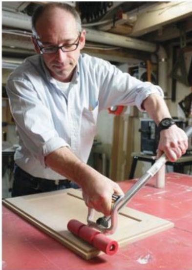
TO GET a solid glue bond, use a J-roller or, if you're in a bind, a kitchen rolling pin
