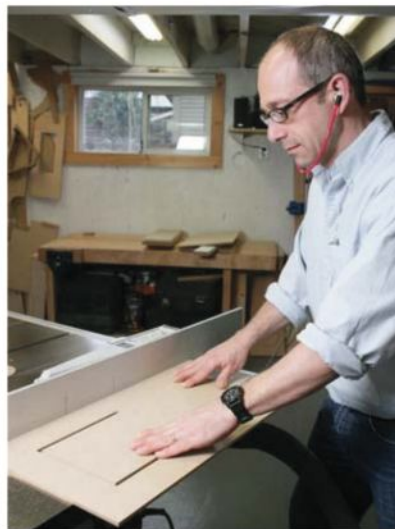
THE BEST way to cut through MDF is to take several passes rather than one single, long cut
