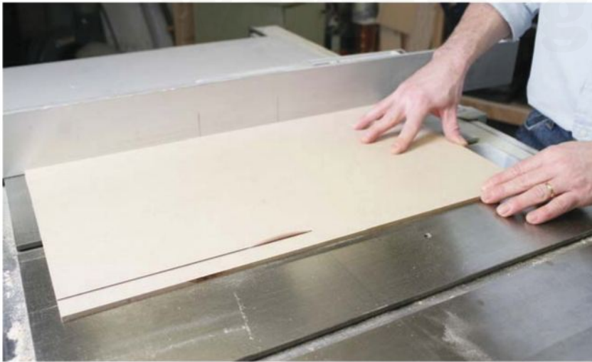
CUTTING ACCURATELY sized cabinets demands slow but deliberate work at the tablesaw. Go slow and make sure everything's aligned; otherwise, it won't fit properly
