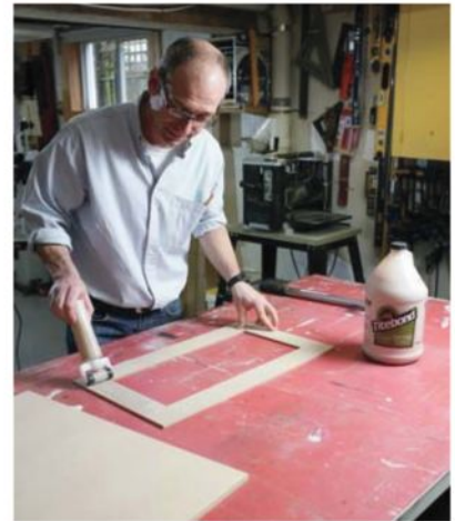
WHEN APPLYING glue, use cold-press laminating adhesive applied with a small roller
