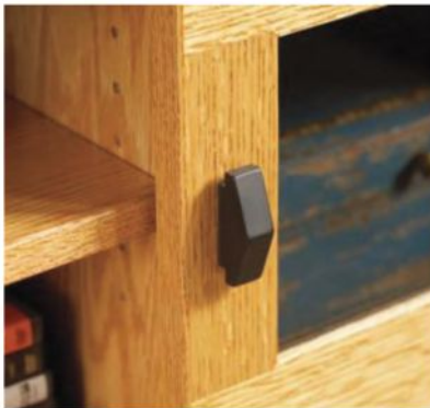
BLACK PAINT makes these simple, shop-built door pulls stand out as important design elements
