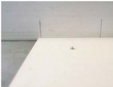
MAKE SURE you have your fence lined up properly, with the starting and stopping points marked clearly on the MDF
