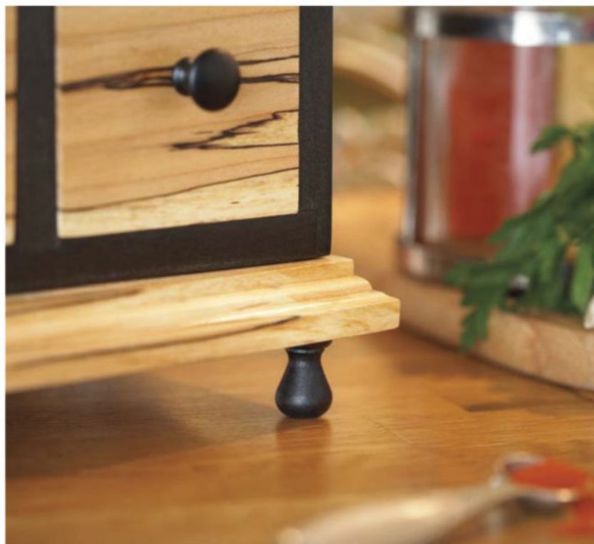
FOOT PEGS give this project a lighter overall look, while also offering a more stable stance than a flat base. The pegs were cut down from longer, factory-turned ones
