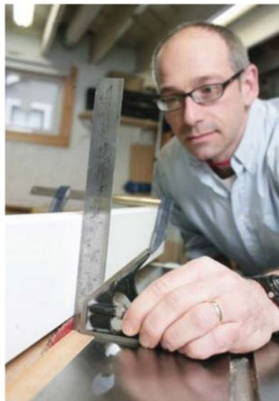
BY CLAMPING a spacer onto your tablesaw fence, you're ensuring a perfect cut every time for each door
