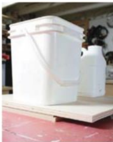
BASIC BUCKETS filled with water provide the best clamping pressure for projects such as these
