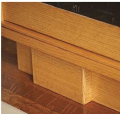
JUST FOR looks , both base blocks are made from veneered ply and solid edging to create a 1"-thick design element
