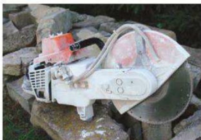
A MASONRY saw with a diamond blade is ideal for cutting stones to length
