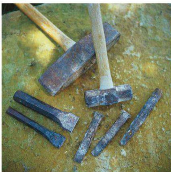
A 14-LBS. SLEDGE (top), pitching tools (left), a 4-lbs. mallet (middle), wedges and a point (bottom)
