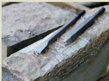
A COMB chisel and point (above) were used to create this classic stone finish. The 7-hp stationary compressor (right) in Steve's shop keeps his air hammers going
