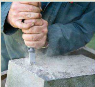
HERE STEVE works the surface of the stone more finely using a four-point toothed chisel
