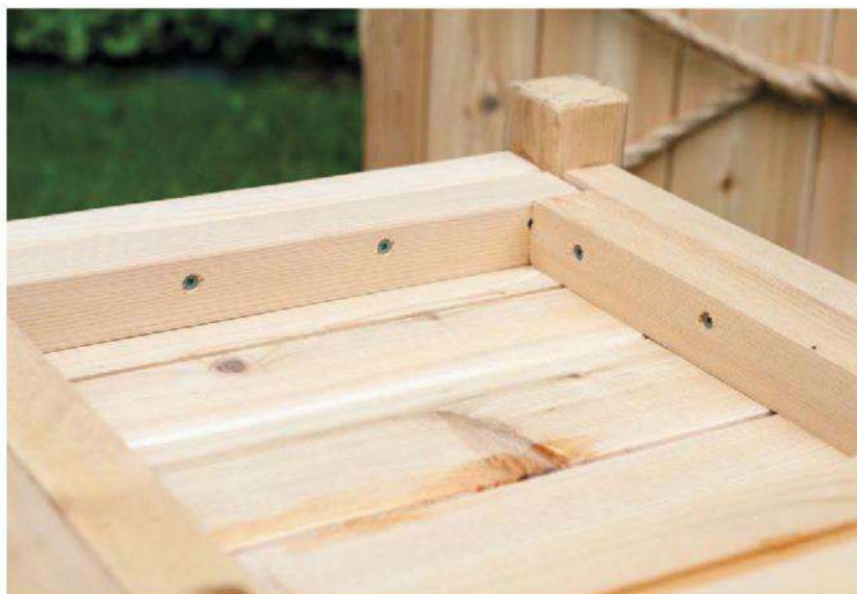
THE UNDERSIDE of the planter, showing the cleats that support the bottom boards
