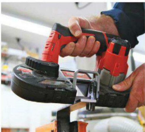
PRECISION AND speed are the biggest advantages of this cordless electric hacksaw
