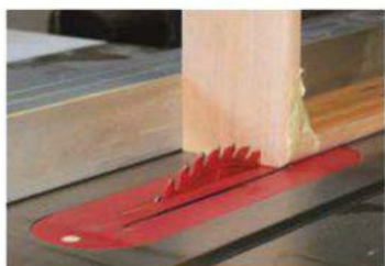
POSITION THE fence to make the first pass along one side of the box
