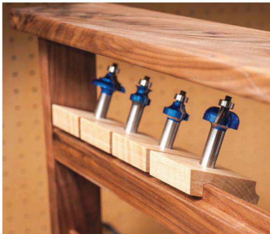
THE BIT holders fit on the frame in the same way they do on the standalone rail. Adjust the size of the frame to suit your needs
