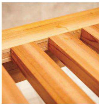
THE BENCHTOP slats come together with mortise-and-tenon joinery with spaces between the slats
