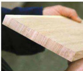
THIS PERFECTLY flat vertical-grained board started as a slab from a 126-year-old ash tree cleaved with a wood splitter
