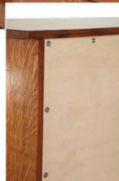
USE FULL-EXTENSION slides for the drawers (top) and screws for the back panel (left)
