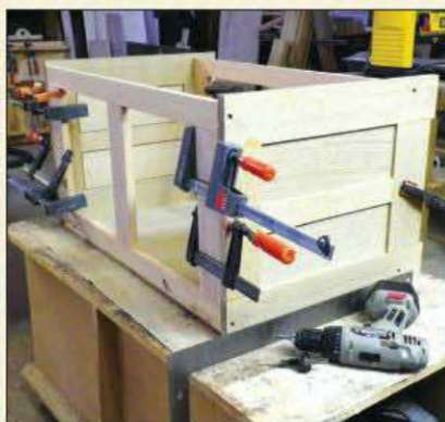
THE CARCASS of the cabinet is held together with F-clamps as the glue dries
