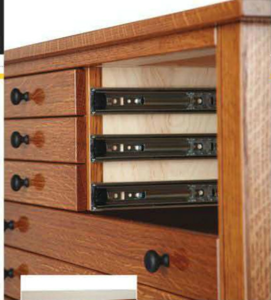
USE FULL-EXTENSION slides for the drawers (top) and screws for the back panel (left)
