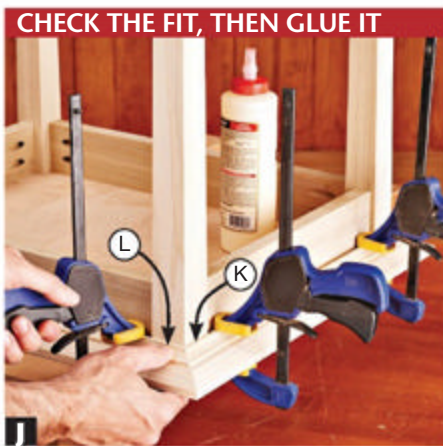
J Miter-cut the cove molding (K, L) to length, testing the fit of all four pieces around the table before gluing it in place.
