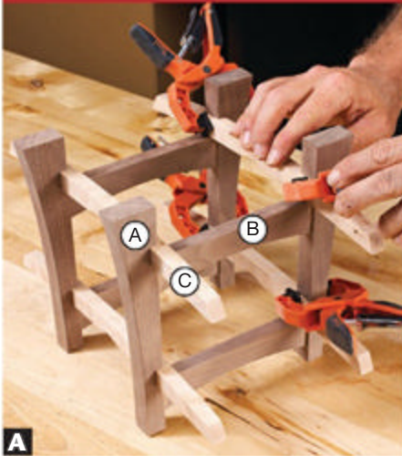
A Stand the frames (A/B) upside down to make it easier to position the rests (C) against the bottom of the rails (B).
