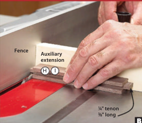
Using an auxiliary extension on your miter gauge for backup and your rip fence as a stop, form \frac{3}{8} "-long tenons on the rails (H, I).
