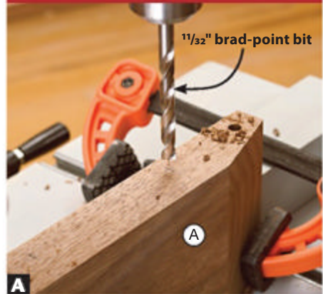
Lay out the axle-hole centers on the chassis (A). Clamp the chassis to the drill-press fence at each location, and drill 1\frac{1}{2} "-deep holes.
