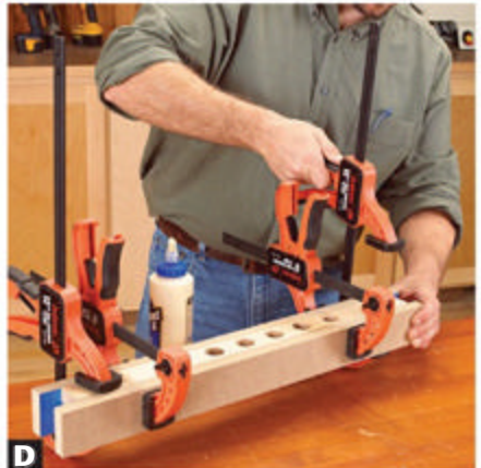
Clamp the parts between the cauls, and then clamp vertically. Keep the mast sides (B) and lower mast spacer (C) flush at the bottom.
