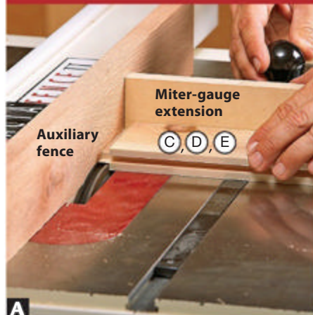
A Using a miter-gauge extension for backup, form a \frac{1}{4} " tenon \frac{3}{8} " long on each end of the rails (C, D) and center stiles (E).
