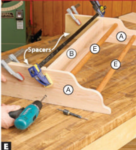
E Spacers clamped to the sides (A) keep the shelf (B) from slipping out of alignment as you drill and drive screws.
