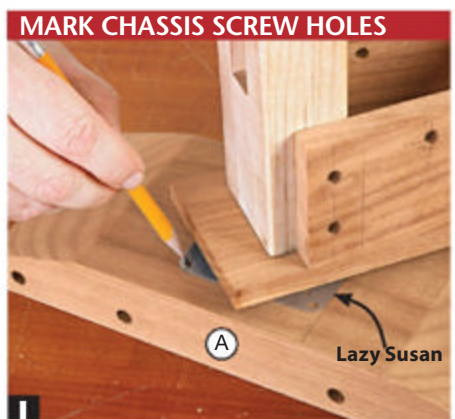
1 Center the lazy Susan on the chassis (A), rotate the mast/hoist assembly to uncover the mounting holes, and mark the locations.
