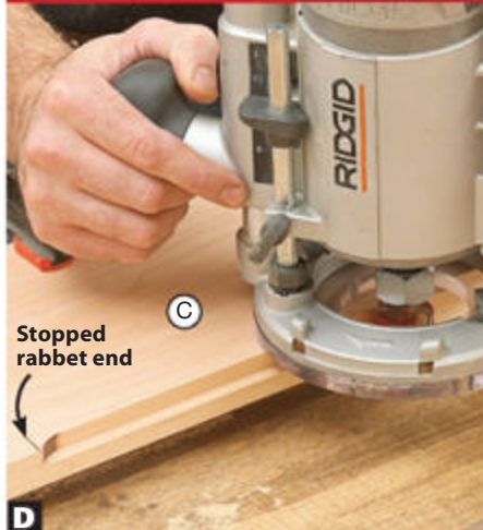
D Begin a stopped rabbet on the top (C) at the first mark and continue until you reach the mark on the opposite end.
