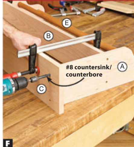
F A combination counterbore/pilot drilling accessory makes quick work of boring screw holes in the top (C).
