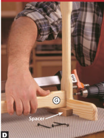
D With the stretcher (G) supported on the spacers and clamped between the support assemblies, drill pilot holes into the stretchers, and drive in the screws.
