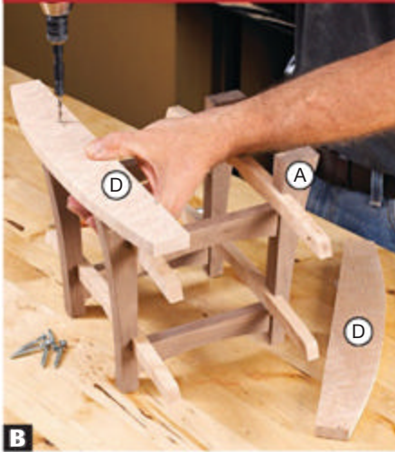
B Drill screw holes through the base (D) into the legs (A) with a countersink bit and portable drill.
