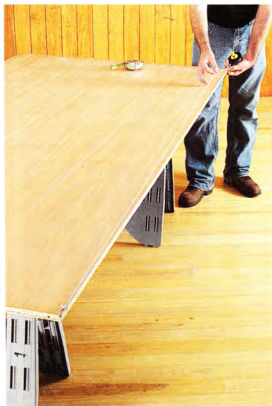
A string or chalk line makes a ready reference for checking the straightness of a sheet of plywood.
