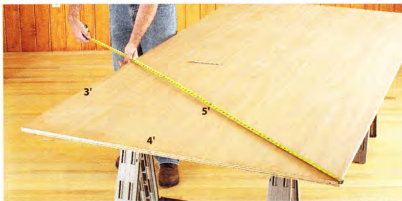
If the diagonal measures 5' at the 3' mark of a 4' wide sheet of plywood, then the corner is square. Just remember: Not all plywood is exactly 4' wide.
