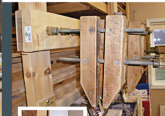
Dan stores all of his handscrew clamps on the wall behind this bench, inserting the handles into 1"- to 1½"-diameter holes, spaced 4" apart on a 2×6. "Instead of adjusting the clamp to squeeze a 1×6, I just push a handle into a hole," Dan says.
