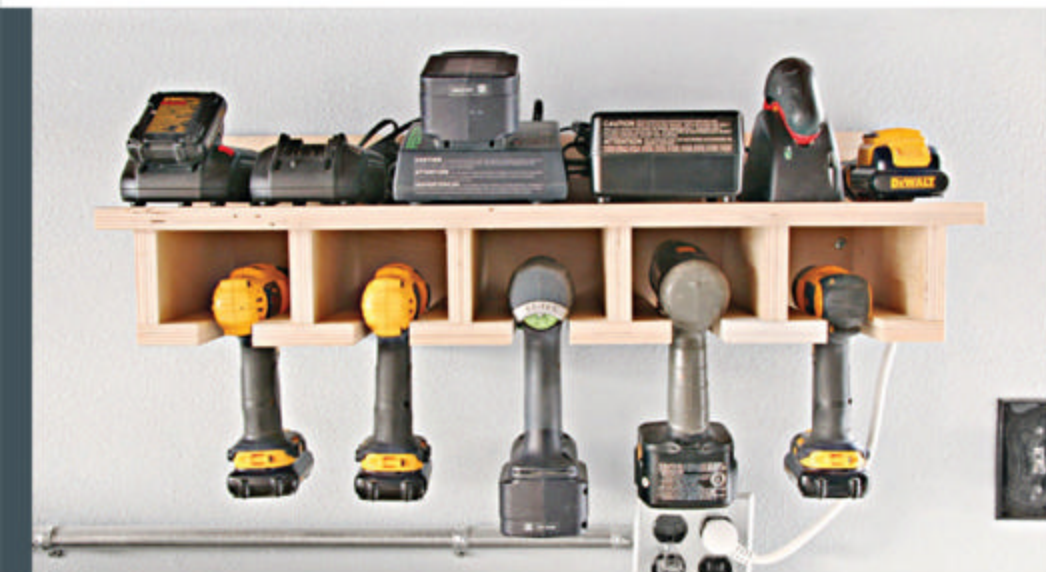
Bobbi adapted a wall-mounted garage for drill/drivers and chargers from a plan available at woodmagazine.com/drillstation . Her version is 10x27½x7¼".
