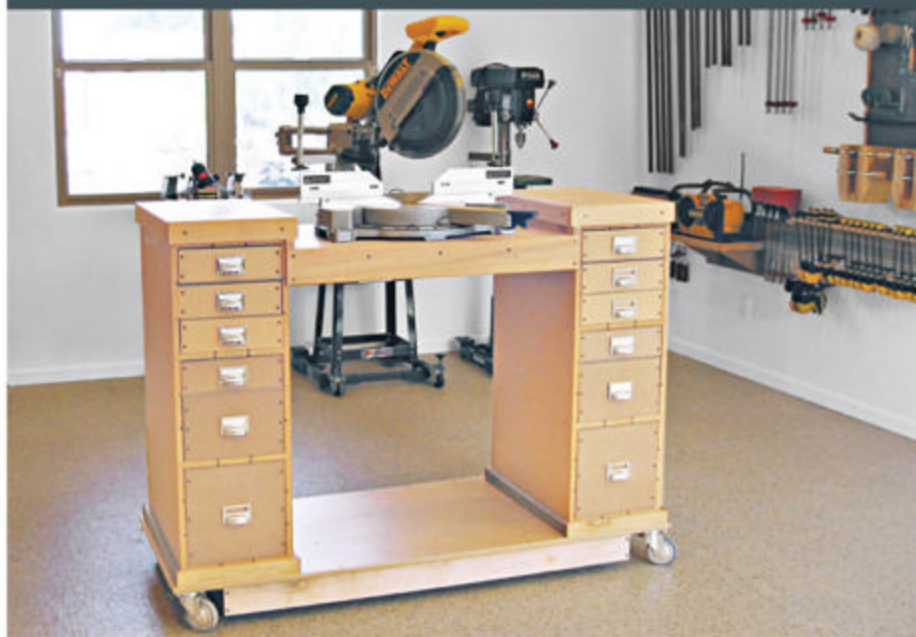
Chris's 25x64x48" mitersaw station stores mitersaw accessories, tablesaw accessories, and an orbital sander with accessories. The station rolls about the shop on 4" locking casters.
