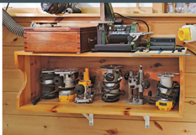
Two open shelves provide a home for a combo sander on top, and routers and other portable power tools below. Bill organizes his router bits in the 4x13 \frac{1}{4} x13 \frac{1}{4} " lidded box (above and right) lined with 1 \frac{1}{4} "-thick foam.
