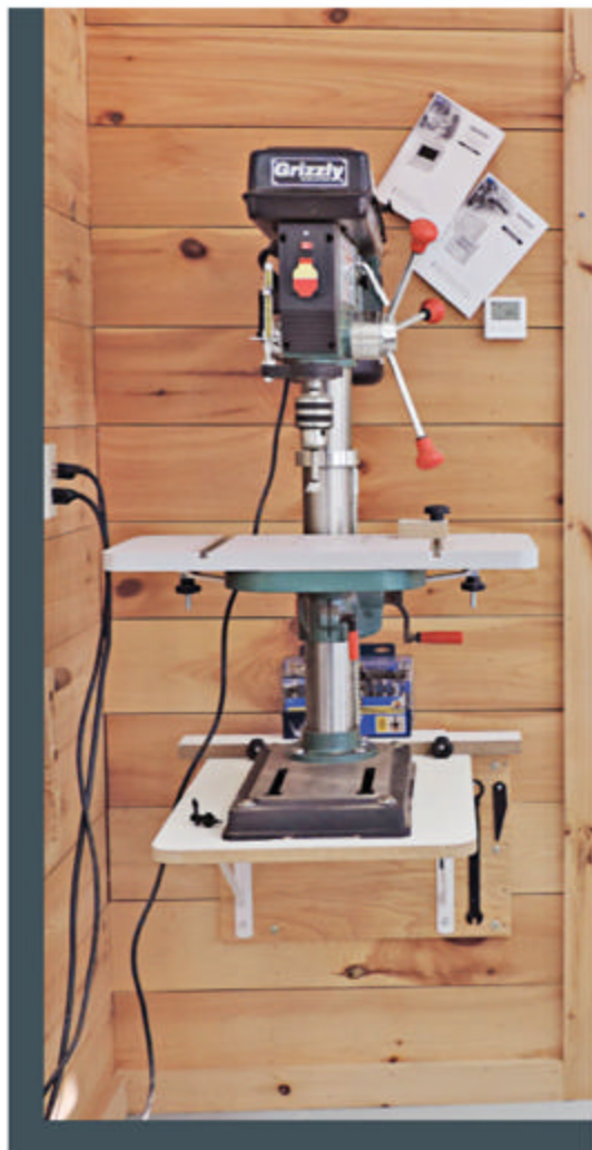
Bill's benchtop drill press sits on a \frac{3}{4} ×18×24" melamine base. He fastened a \frac{3}{4} ×13 \frac{3}{8} ×21" mounting plate to the wall before securing the shelf brackets with lag bolts.
