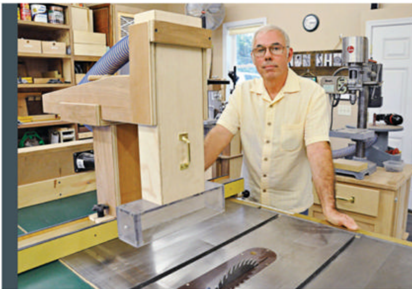
Dan Martin stands behind a multipurpose tablesaw guard that acts as a see-through blade guard, holds down stock, and collects dust. The guard clamps to customized fittings on his tablesaw rip fence. Using the gate handle, Dan raises the guard to fit over stock.
