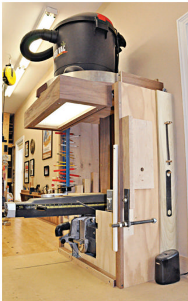
This 34½×46" lumber rack rests on a heavy-duty tablesaw mobile base for good reason: It must roll out of the way temporarily when it's time to service the propane heater (not shown) above it.
