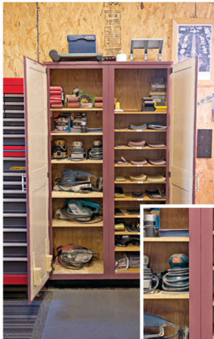
A 12x36x66" cabinet (repurposed from Bill's kitchen remodel) stores sanding equipment and supplies. "I use a flat-blade paper trimmer to cut each sheet to one-half or one-quarter size or sized for my hand-sanding block," Bill says. "It works great." Bill stores the paper trimmer, purchased at an office supply store, above the cabinet.
