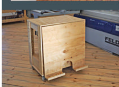
To lift 4x8' sheet goods onto the saw table, Bill loads the material on the side of this mobile bench, raises the hinged side, and then slides the sheet across the bench and onto the saw.
