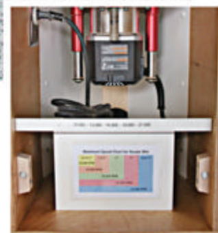
A speed chart beneath Bobbi's router shows the proper rpm for each bit diameter. A JessEm lift raises and lowers the router.
