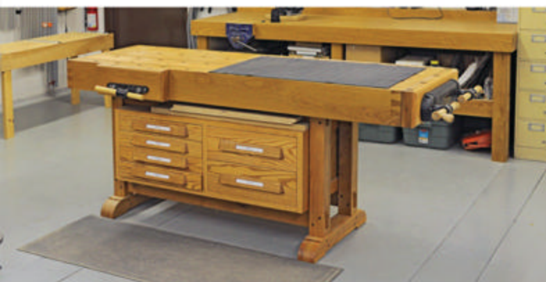
Steve built this 27½x76" workbench from white oak felled on the lot where his house and garage now stand. A nearby sawyer kiln-dried all the lumber, including the 2¾"-thick oak for the laminated benchtop. Steve added no-slip pads (designed for washing machines) to the feet.
