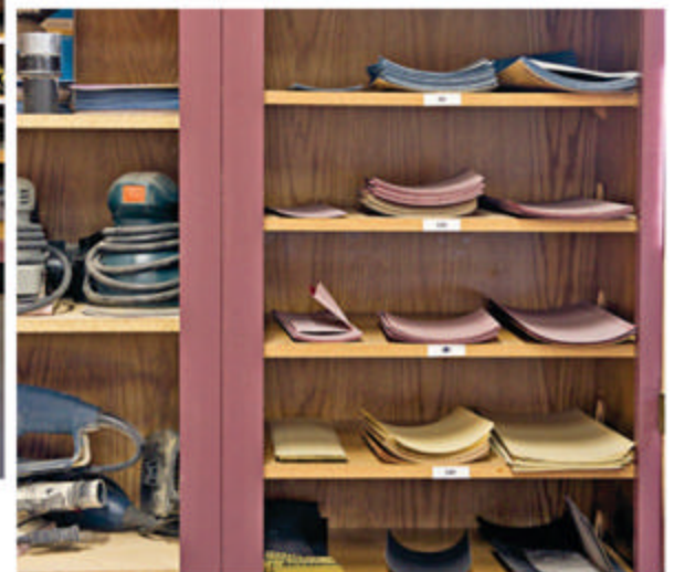
A 12x36x66" cabinet (repurposed from Bill's kitchen remodel) stores sanding equipment and supplies. "I use a flat-blade paper trimmer to cut each sheet to one-half or one-quarter size or sized for my hand-sanding block," Bill says. "It works great." Bill stores the paper trimmer, purchased at an office supply store, above the cabinet.
