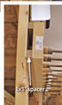
Dan stores all of his handscrew clamps on the wall behind this bench, inserting the handles into 1"- to 1½"-diameter holes, spaced 4" apart on a 2×6. "Instead of adjusting the clamp to squeeze a 1×6, I just push a handle into a hole," Dan says.
