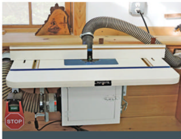
Above: Two 19 \frac{3}{4} "-long metal shelf brackets support Bill's wall-mounted router table. The 24×31 \frac{3}{4} " Rockler top includes a fence with a 2 \frac{1}{2} " dust port.
