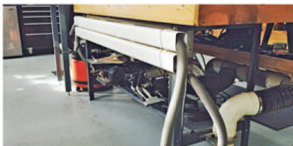
A network of ducts beneath the workbench feeds a 24"-long floor sweep (above and right), a downdraft cutout in the bench, and the tablesaw. If Bill upgrades his tablesaw, he can easily convert the in-floor 110-volt outlets to 220-volt.
