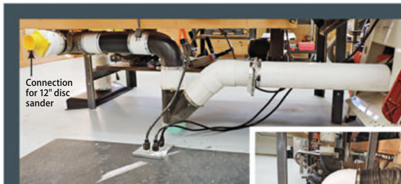
A network of ducts beneath the workbench feeds a 24"-long floor sweep (above and right), a downdraft cutout in the bench, and the tablesaw. If Bill upgrades his tablesaw, he can easily convert the in-floor 110-volt outlets to 220-volt.
