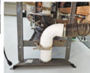
To corral 15' of flexible hose on his Fein dust extractor, Bill runs the hose through 60"-long sections of plastic downspout.
