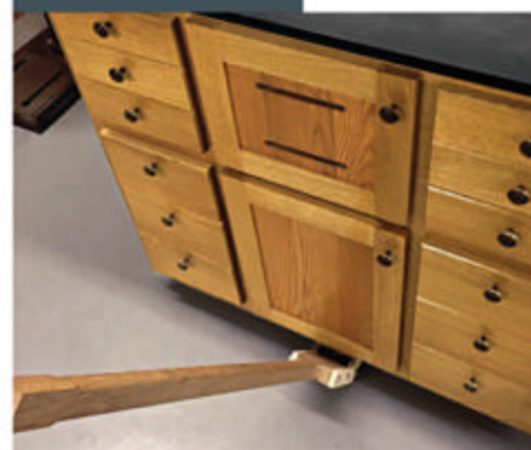
A wheeled handle—"a stick with two wheels"—elevates the front of the router table off nonslip pads. The wheeled handle and two wheels at the back of the table allow Steve to reposition the base.
