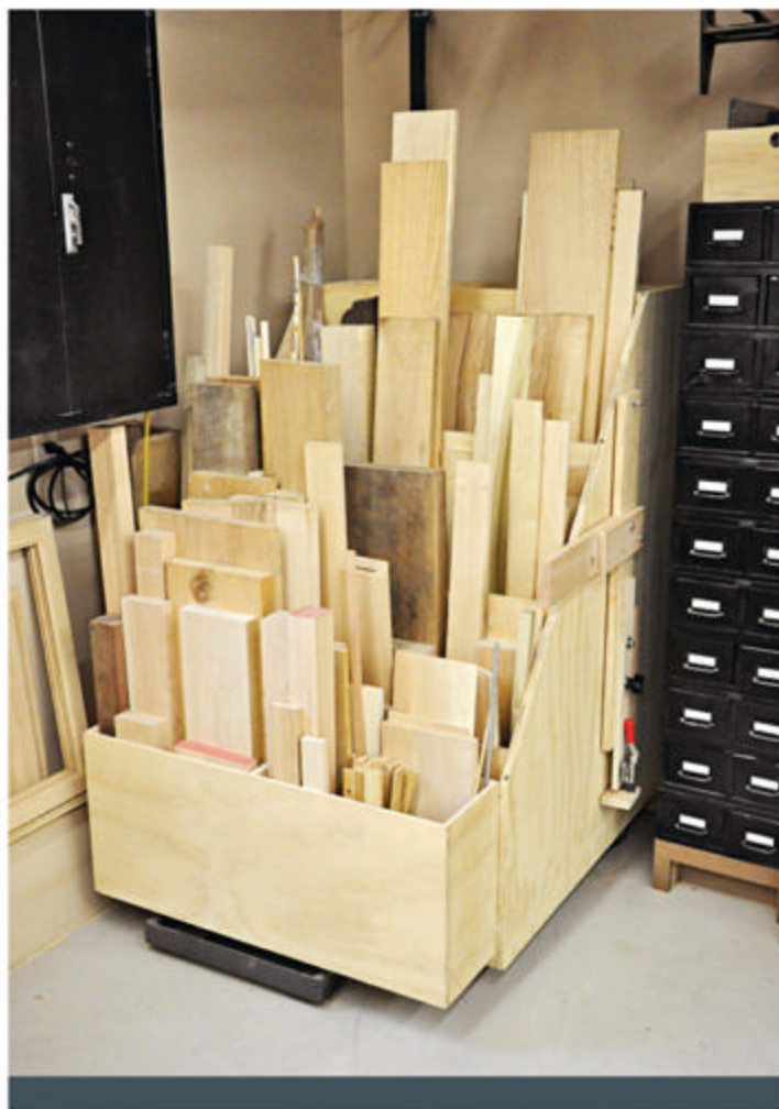
This 34½×46" lumber rack rests on a heavy-duty tablesaw mobile base for good reason: It must roll out of the way temporarily when it's time to service the propane heater (not shown) above it.
