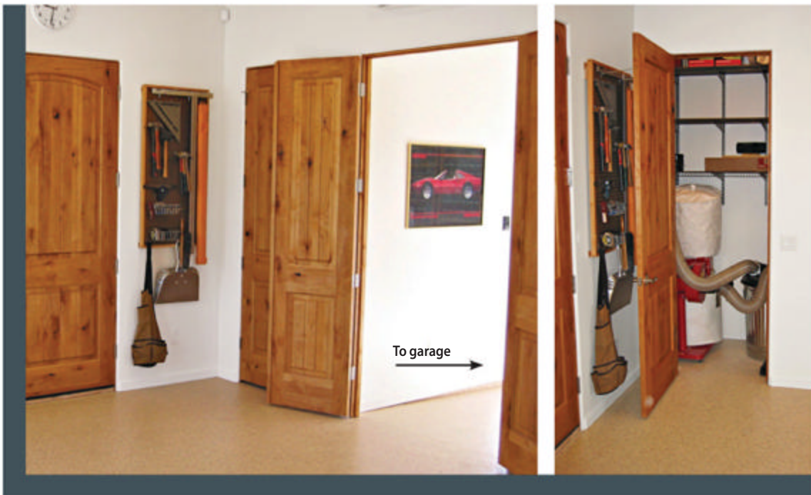
Far left: The hallway between the garage and the shop has a ramp required by building code. The ramp also allows Chris to easily bring materials from his truck into the shop. Near left: A closet reduces the noise from Chris's dust collector. All the ductwork runs above the ceiling.
