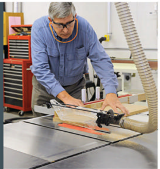
Steve modified his table saw's blade guard to accept a 2" dust hose.
