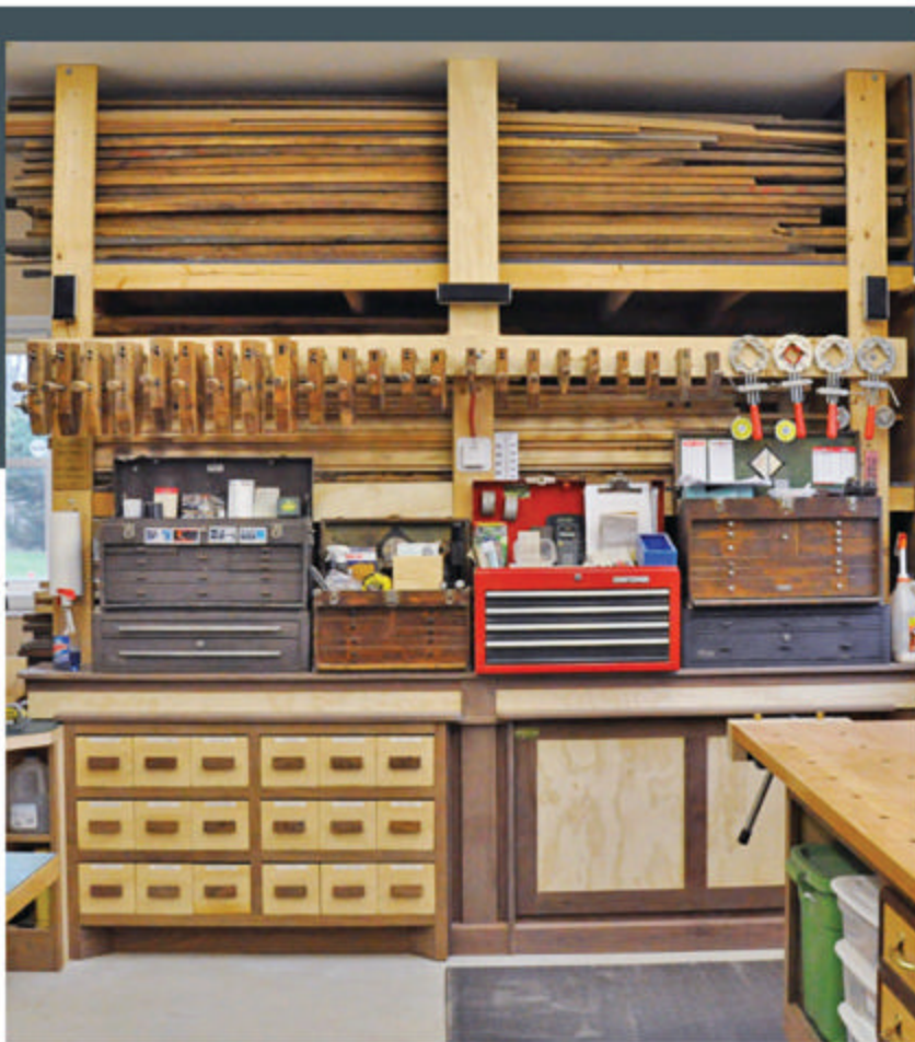
Four tool chests consume just about all of the horizontal space on this 10'-long bench. Dan has organized calipers, hand tools, and gauges in the toolbox drawers; the drawers below the bench hold more tools and miscellaneous hardware.
