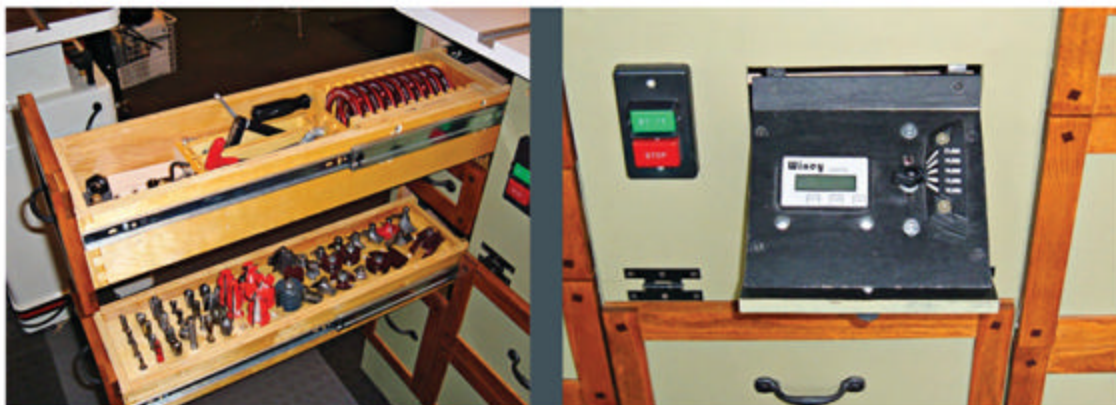
Ted outfitted his 33x54" router-table top with an Incra fence. A 3¼-hp variable-speed Porter-Cable router sits below a Woodpecker plate insert and lift.
