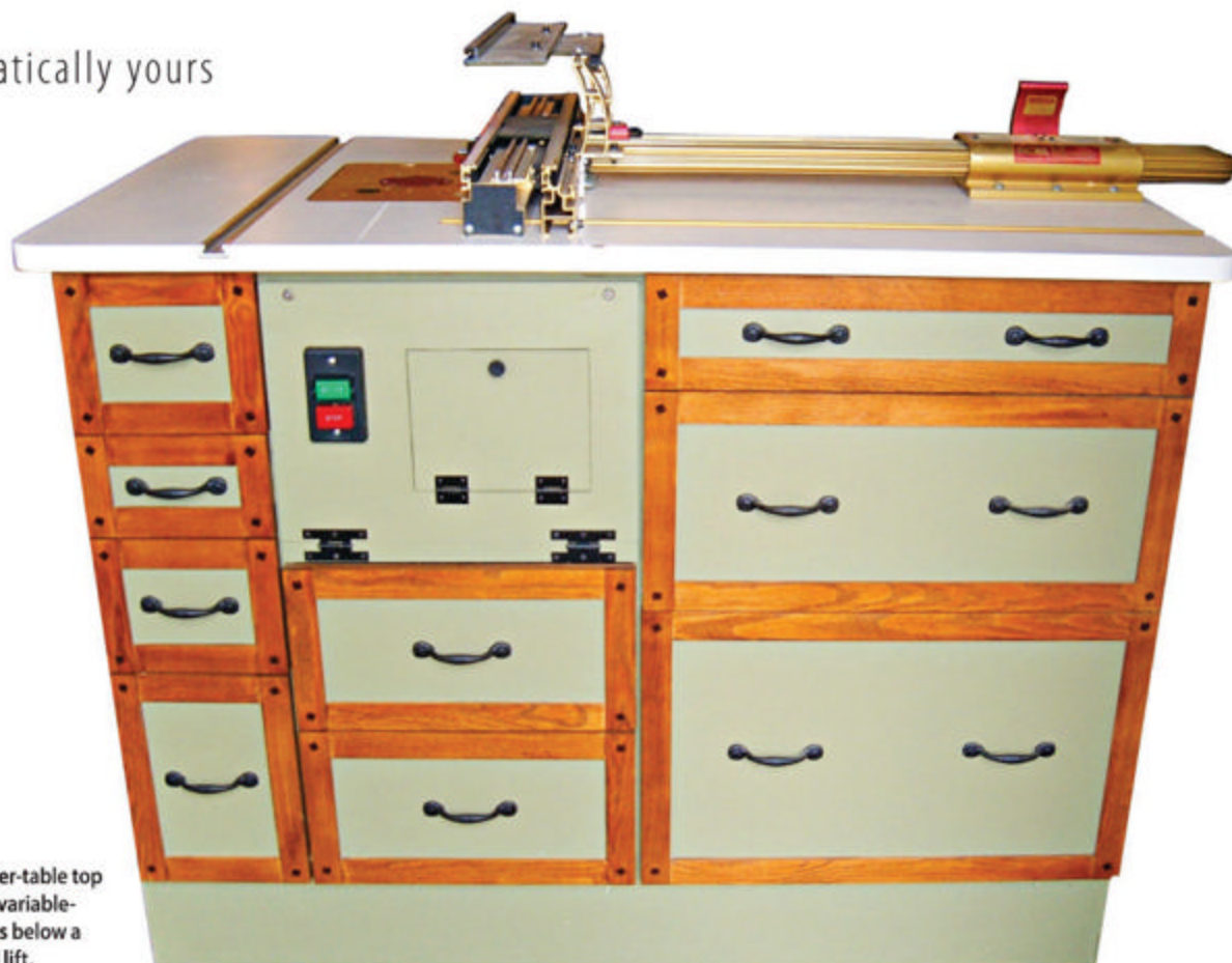
Ted fine-tunes his router performance with a drop-down Wixey digital depth-control indicator and speed control (left) hinged to the front of his router table.
