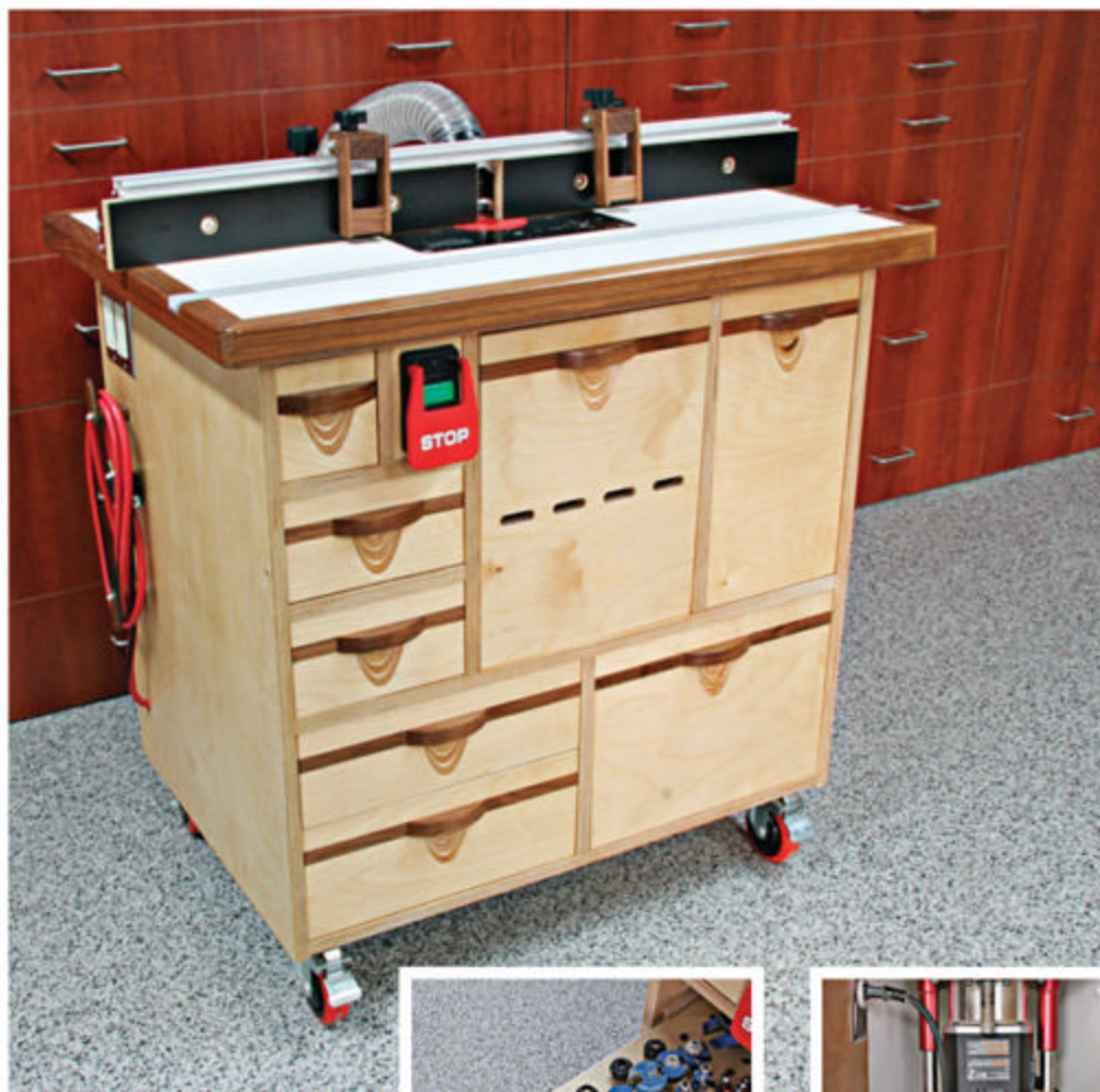
Above: Bobbi made this 26x36x36" router table on 4" casters as part of a class project. She added shop-made stops to the Woodpecker fence. Right: A top drawer organizer provides space for a full complement of router bits.
