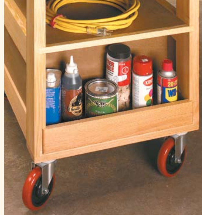
▲ Storage Cubby. Adding a false front to the opening at the back of the cart creates a handy storage area for often-used items.
