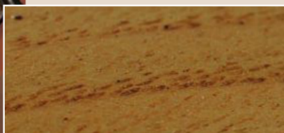
ABOVE: Macro shot showing dust stuck in the applied finish. This compromises the visual appeal of the piece and you can also feel the dust on the surface
