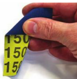
1 First fold the sandpaper over at a 90° angle...
