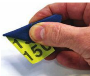
3 ... fold the sandpaper up over the 45° angle...
