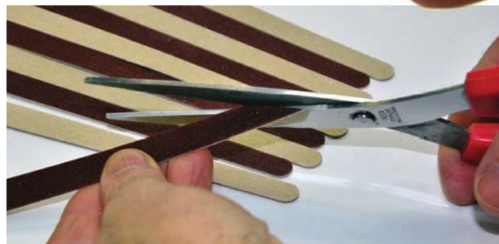
▲ Manicure emery boards can be trimmed to shape for access to awkward areas
