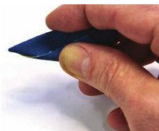
4 ... and fold the sandpaper back down and around the lower 90° angle
