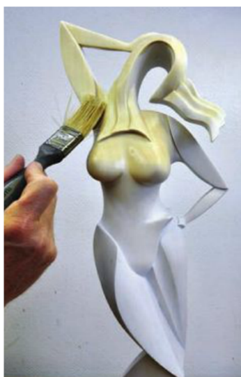
▲ Brushing on hot water raises the fibres of the wood, allowing the following grit to be worked more easily and effectively
