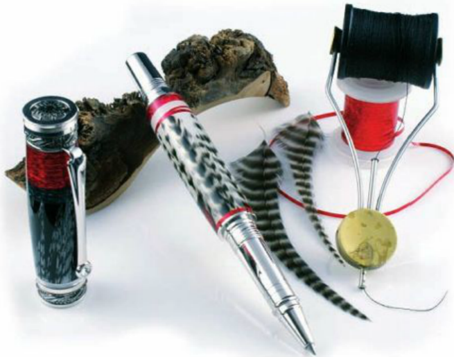
'Apache's Arrow' pen turned on a Jnr Majestic rhodium roller ball kit. Made from the following feathers and materials: Grizzly saddle, (lower barrel); dyed red Amherst pheasant tail (lower barrel); a clipping of natural (black and white) Amherst pheasant tail (clip end barrel); red flat tinsel and some black flat tinsel, with the tubes being air brushed with a water based acrylic paint. By Mervyn Cadman
