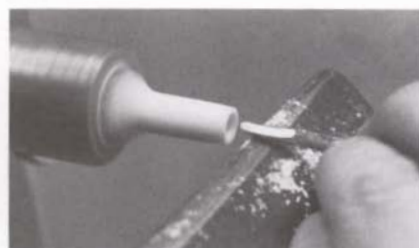
Internal shaping requires special little scrapers, which you can easily make from concrete nails or the tang of an old tool.
