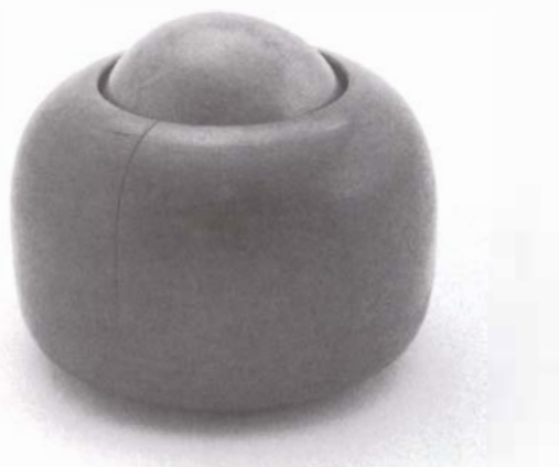
Massage ball, probably Chinese. The ball is turned from very dry material, the holder from a green limb. The ball is forced through a hole just large enough to take it. As it dries, the holder shrinks around the ball.
