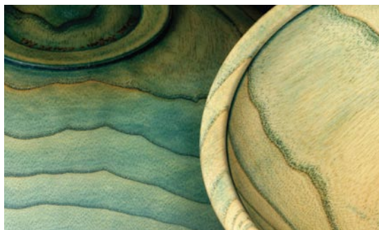
▲ These ash bowls were stained an intense blue then sanded back to reveal the wood and highlight the grain.
