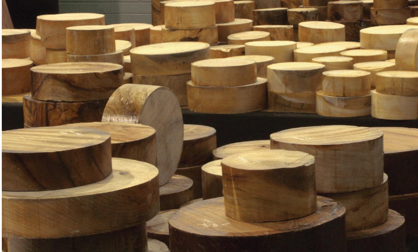
▲ Turning blanks cut round on a bandsaw.
