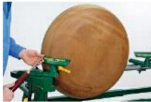
Photo 12. The headstock may have the facility to swing round through 90^\circ
