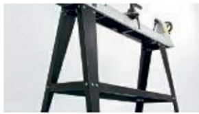
Photo 5. Some more rigid leg-stands include provision for a tool shelf
