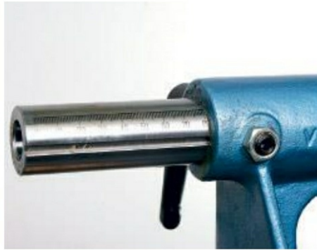
Photo 24. The tailstock barrel needs plenty of travel for drilling work...
