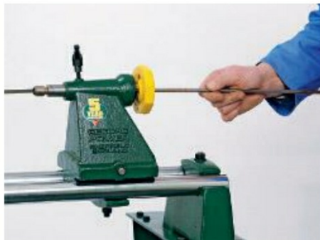
Photo 25. ...and should be drilled through to allow for long hole boring
