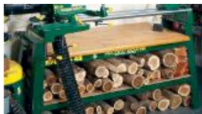
Photo 6. Under-bench storage helps to give a stand useful extra mass
