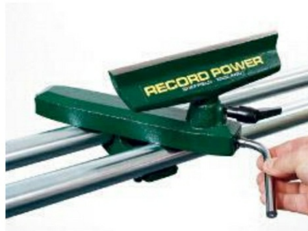
Photo 26. A cam lock on the tool rest is easily accessible from the front
