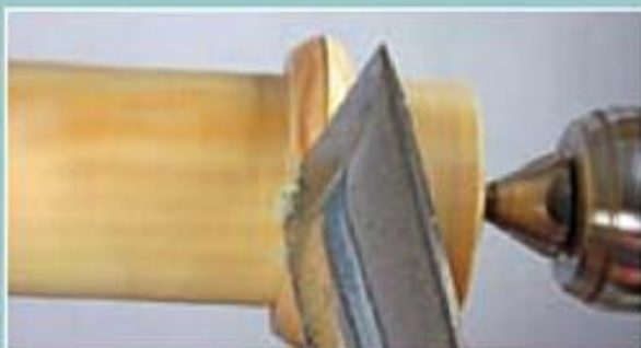
Rounding the corners on a proud bead.
