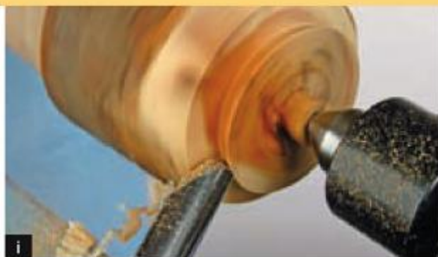
Cut 6 Roughing the stem – DFG.
