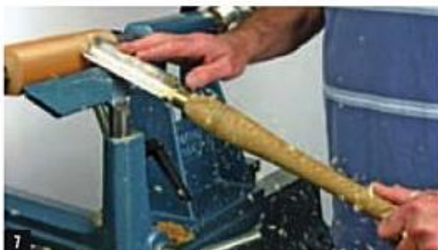
7 Roughing left-handed; power grip for control hand, fingers grip for support hand.
