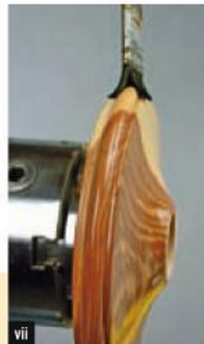
Applying finish with brush – lathe running very slow.
