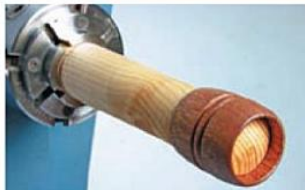
Above Tapered mandrill for holding napkins.
