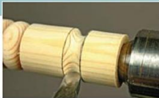
Cutting a cove with a cove form tool.
