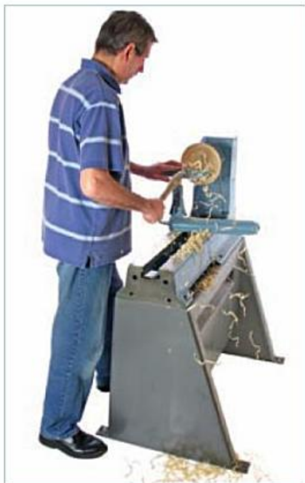
Above Turning inside a bowl right-handed.
