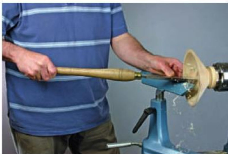
Fingers behind supporting the wood, thumb on the tool.
