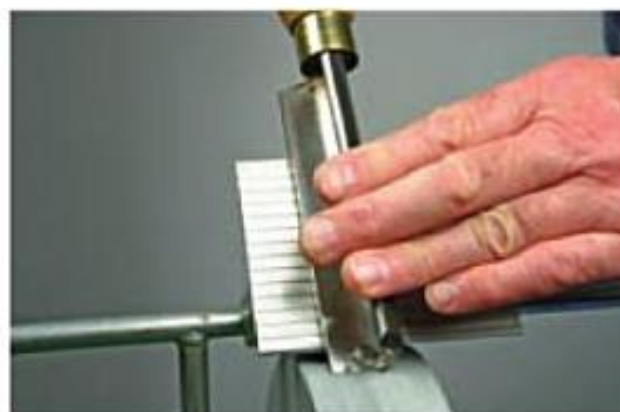
Above Sharpening the SRG on the Tormek platform in the end position; wheel running towards the tool.
