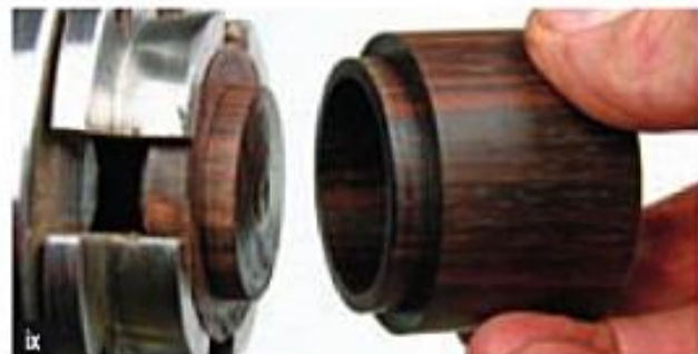
ix Jam fitting base on spigot turned on waste.
