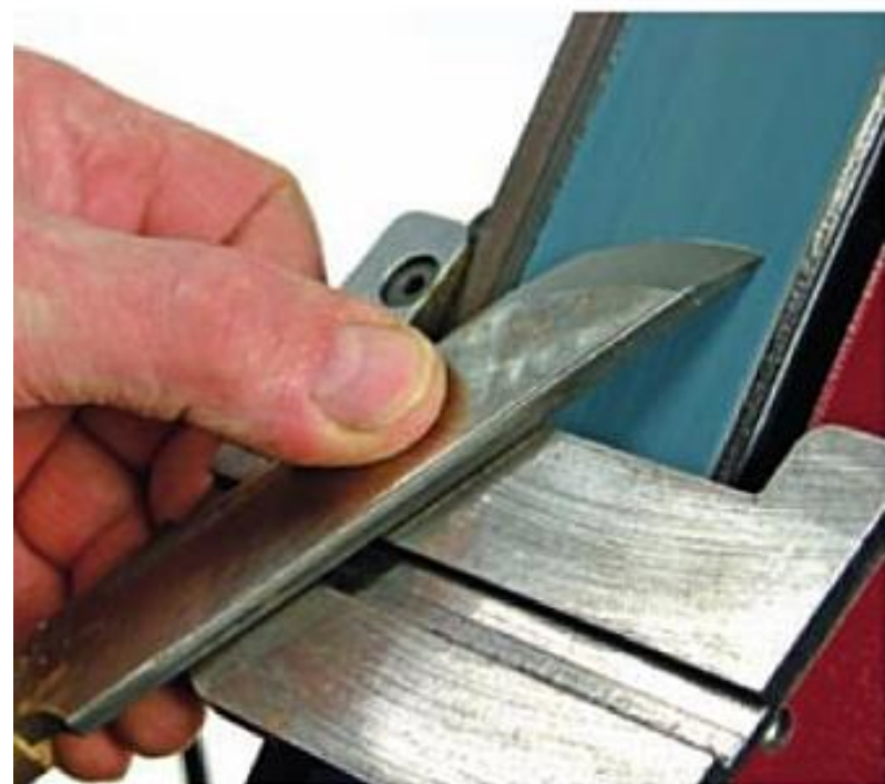
Left Curved skew held with thumb.
