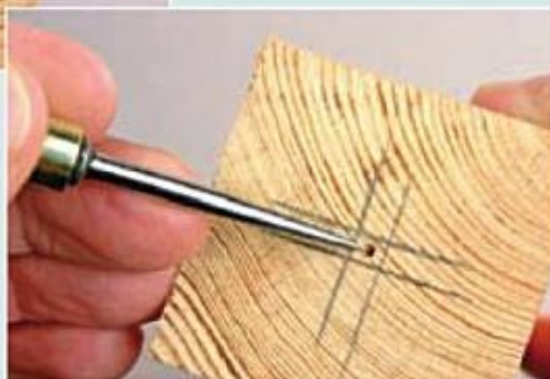
Right Marking the centre with a fine-pointed bradawl.
