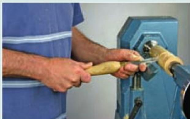
Holding the parting tool, power grip and back grip.
