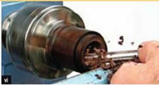
vi Cut 17 Hollowing the base with SFG.
