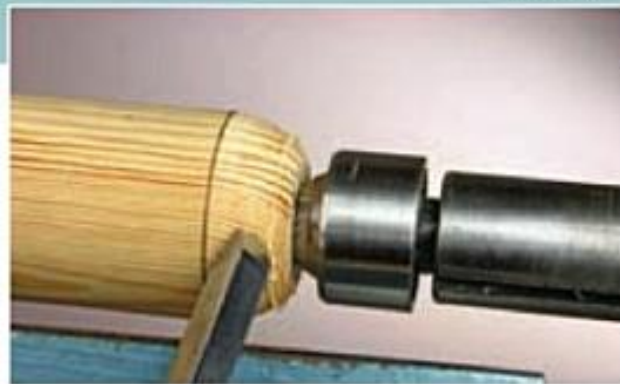
Rounding the end with the beading tool.
