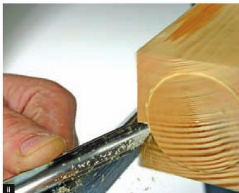
Squaring the end of a spindle.
