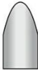
Fingernail grind on the shallow-fluted gouge (SFG)
