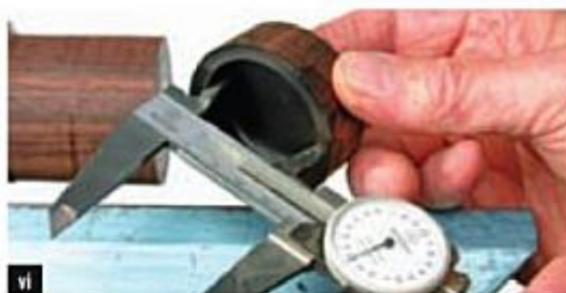
Measuring joint face diameter in lid.
