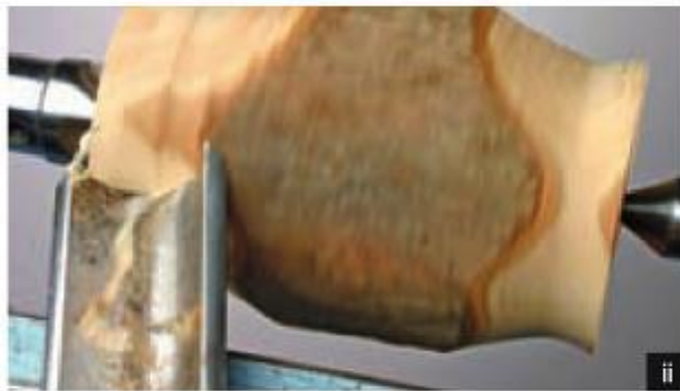
Cuts 1 and 2 Clearing bark at both ends with SFG.
