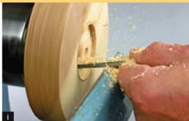
i Cut 3 Making recess for expanding chuck.
