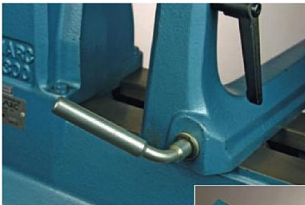
Above Cam-lock on the Vicmarc lathe saddle.
