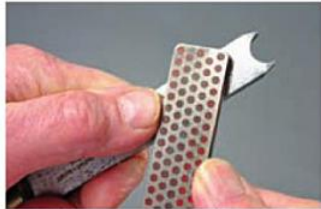
Above Sharpening form tool with a diamond file.
