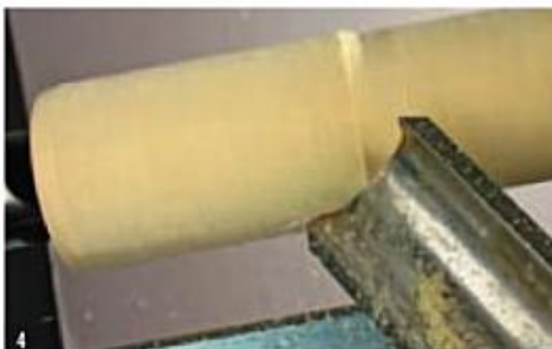
4 SRG presented for a finishing cut, working from tailstock.
