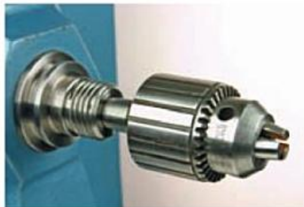
Above Jacobs chuck; no. 1 morse taper with 2-1 sleeve.
