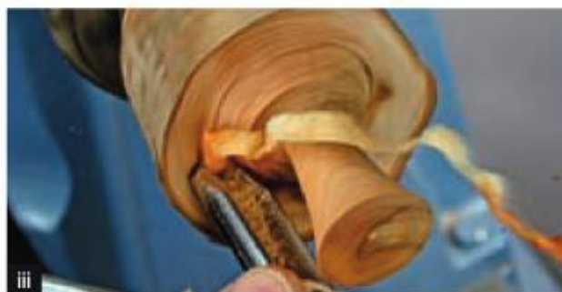
Cut 8 Undercutting the rim – DFG.
