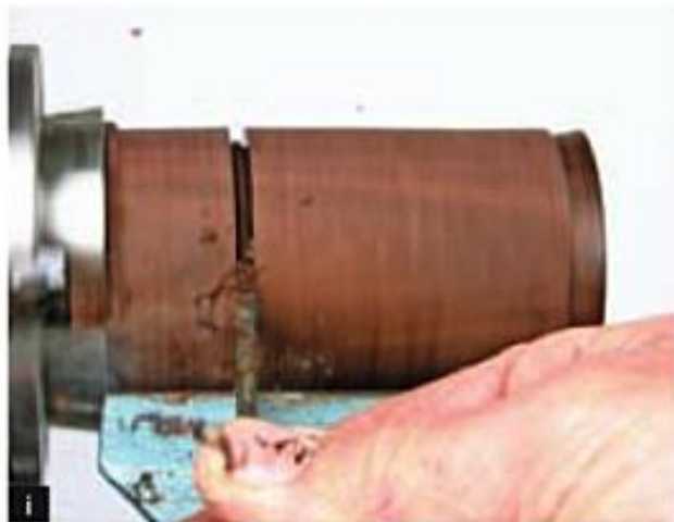
Cut 6 Blank held in chuck – parting.
