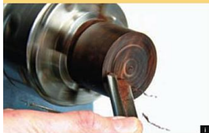
Cut 20 Clean under the base – DFG.
