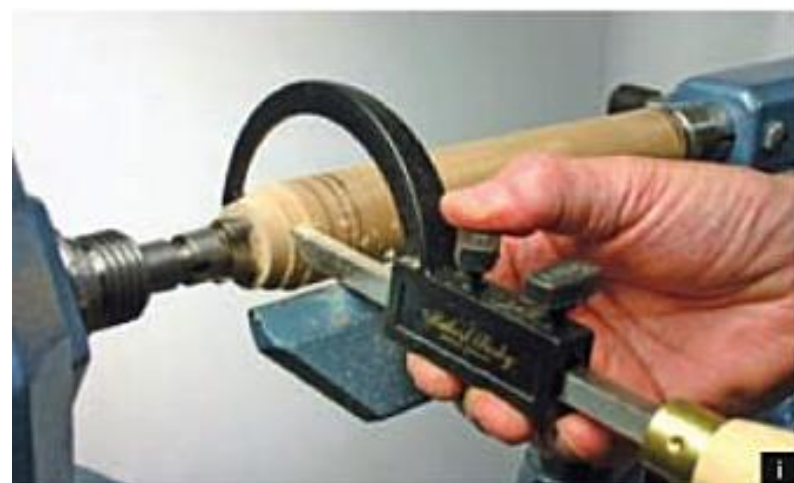
Cut 14 Shaping the stem.
