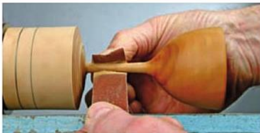
Above The edge of the abrasive being worked around the detail.
