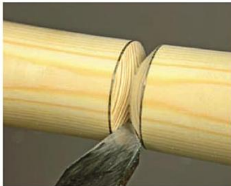
Cutting a vee with a vee-form tool.
