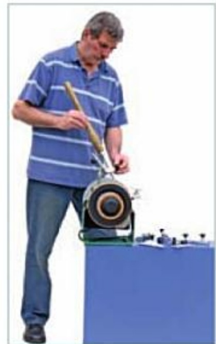
Above Comfortable height and stance for tool sharpening on the top of the Tormek wetstone grinder.
