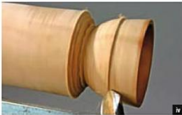
Cut 10 Shaping the outside of the bowl.
