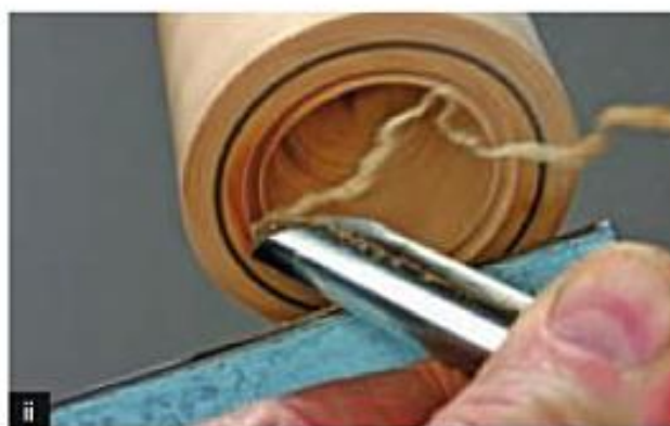
Cut 8b. Hollowing from rim to base with DFG.
