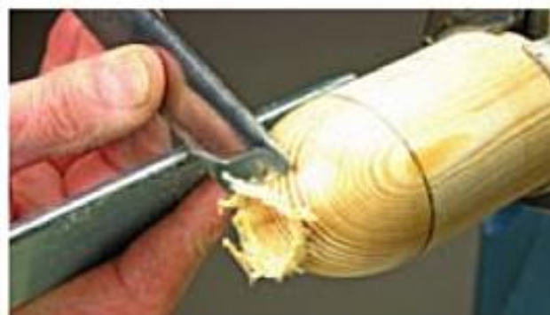
Hook grip while making a curve on the end of a spindle.
