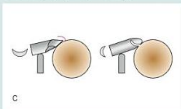
C. Shallow-fluted gouge being rolled on the bevel until the edge makes contact.
