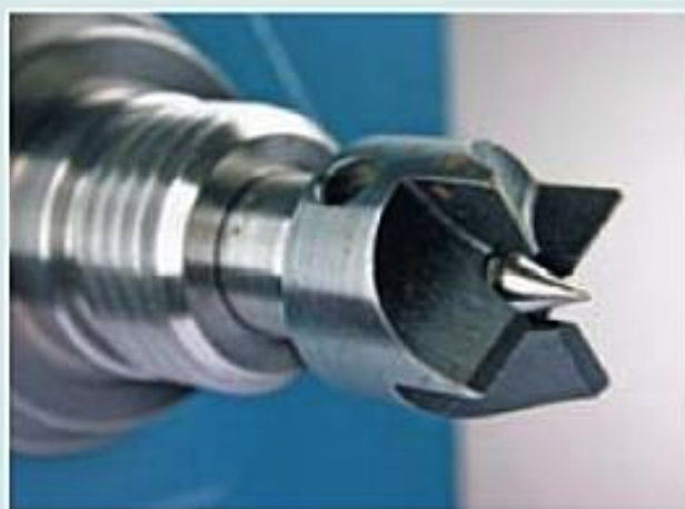
Above Two-prong centre; no. 1 morse taper and 2-1 sleeve.
