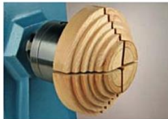
Above Expanding wooden jaws on Axminster chuck.
