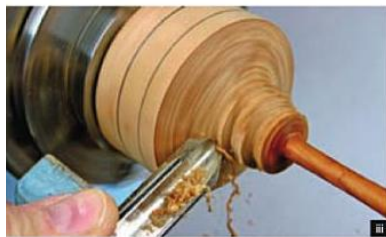
Cut 15 Shaping around the curve.
