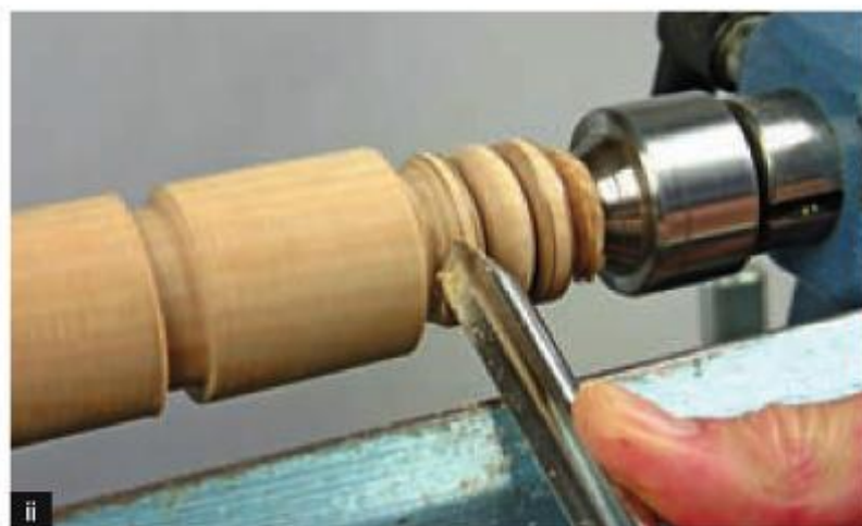
Cut 9 Turning the detail at the top with the spindle roughing gouge.
