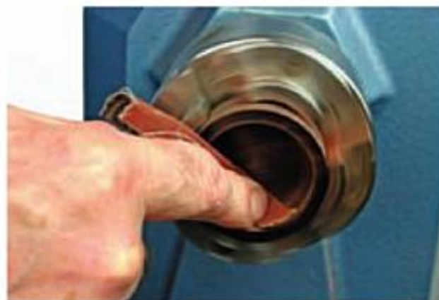
Above The edge of the abrasive being worked around the detail.
