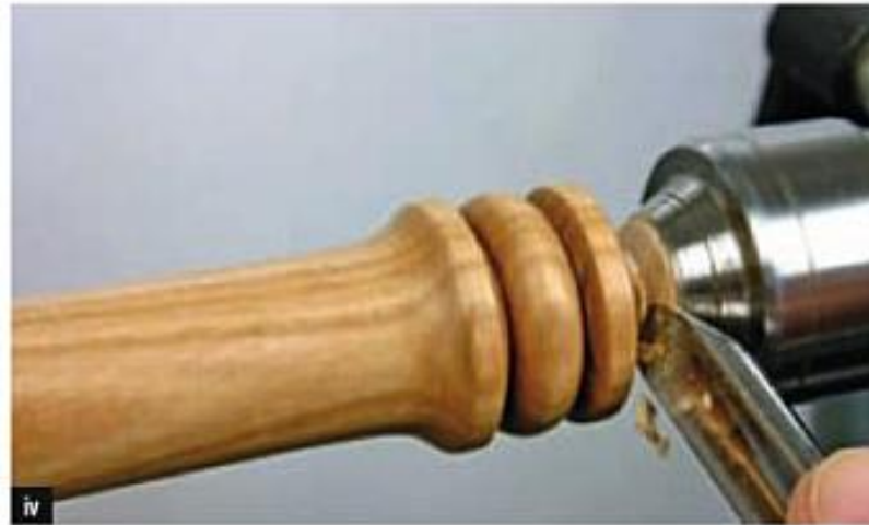
Cut 9 Turning the detail at the top with SFG.
