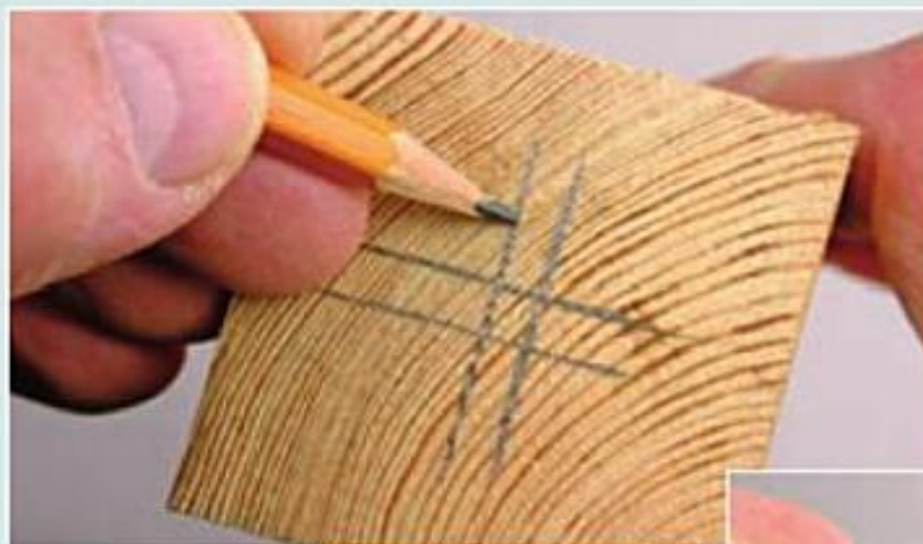
Above Using fingers as a gauge to find the centre of a square.
