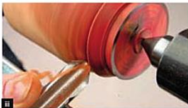
Cut 5 Shape the bottom of the apple.
