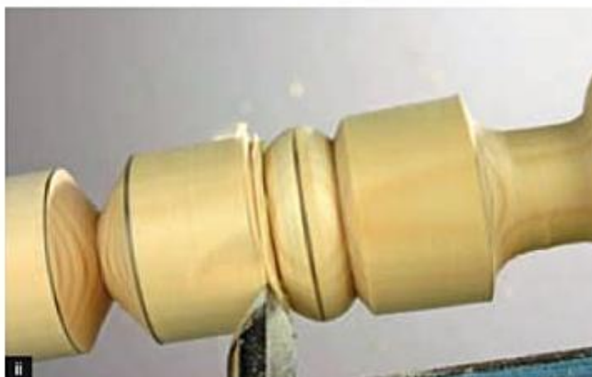
Turning an inset bead.
