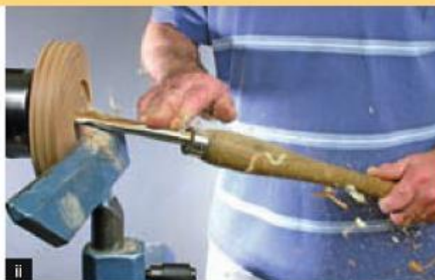
ii Cut 4 Shaping top of base with DFG from centre to rim.
