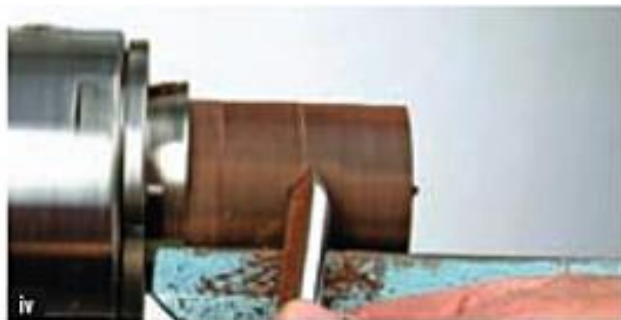
iv Surfacing lid and base together with SFG.
