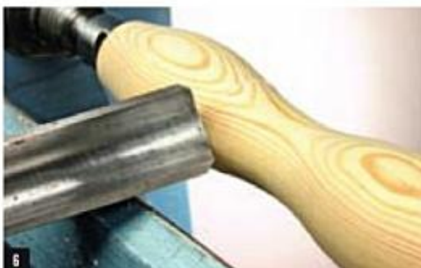
6 Making simple curve shapes, leaving a good finish.
