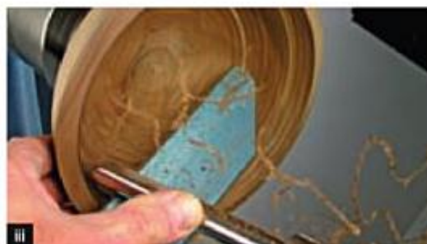
iii Cut 10 Last cuts inside with fingers supporting the wood
