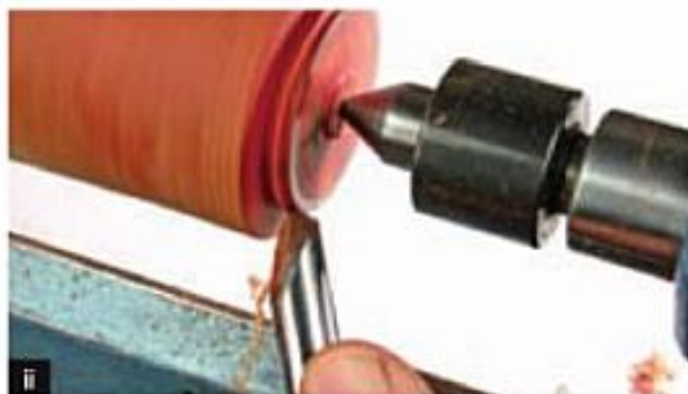
Cut 4 Turning the spigot.
