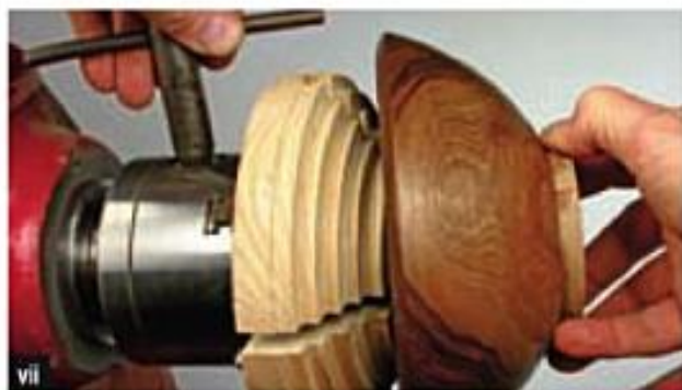
Reverse mounting on wood jaws.
