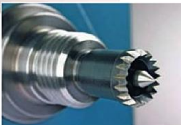
Above Counter bore; no. 1 morse taper with 2-1 sleeve.
