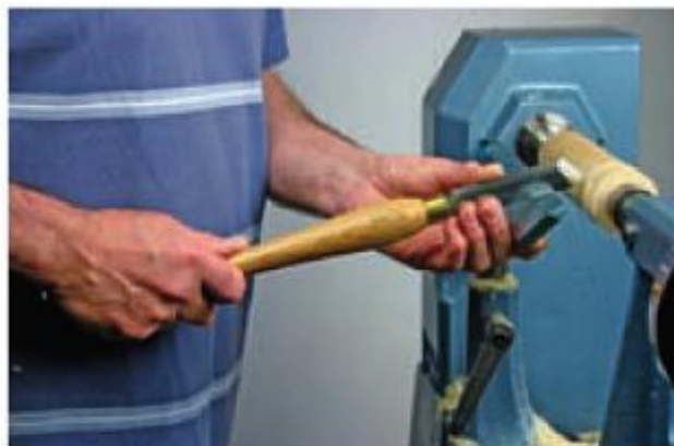
Power and hook grips while turning a vee.
