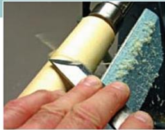
Smoothing cut along a spindle.
