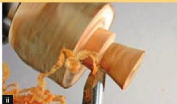
Cut 7 Shaping the stem – DFG.
