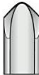
Swept back grind on the deep-fluted gouge (DFG)
