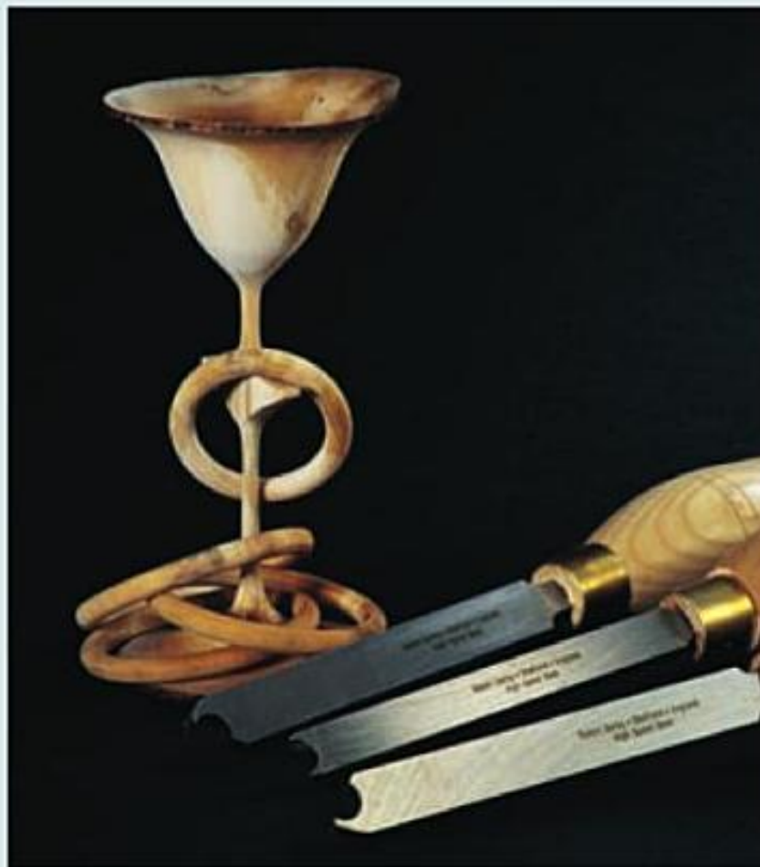
Left Form tools for captive ring cutting.
