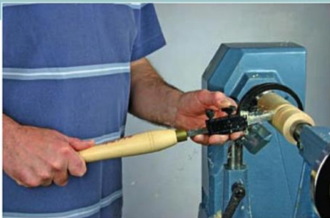
Sizing with the bedan and sizing attachment.
