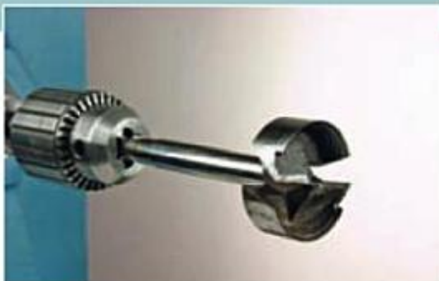
Above Forstner bit, used for pin chuck.
