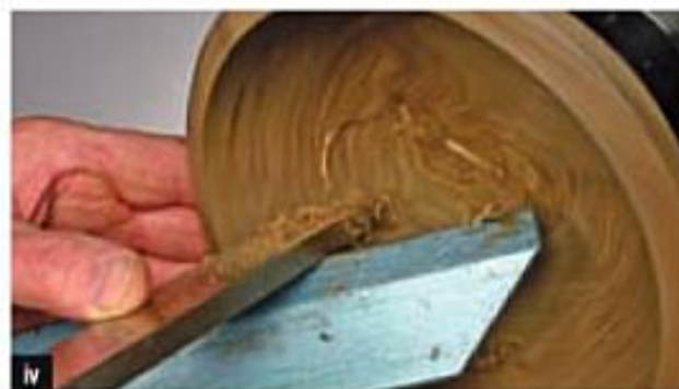
iv Cut 11 Refine the inside with scraper, fingers supporting the wood.
