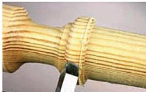
Rolling a bead with the point of the beading tool.
