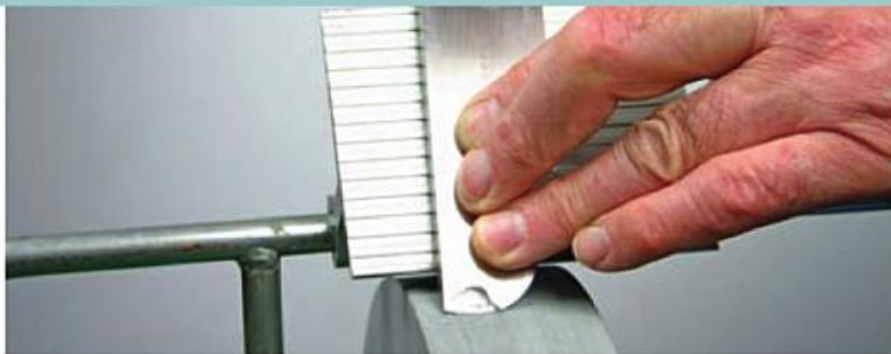
Above Swinging scraper on Tormek wetstone.
