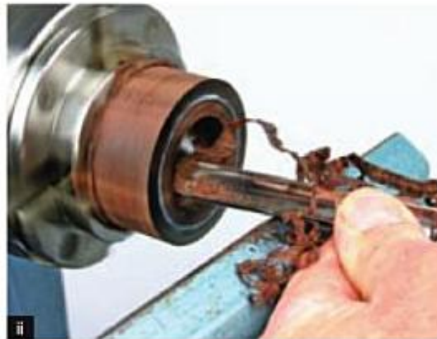
Cut 8 Hollowing lid from centre with SFG.
