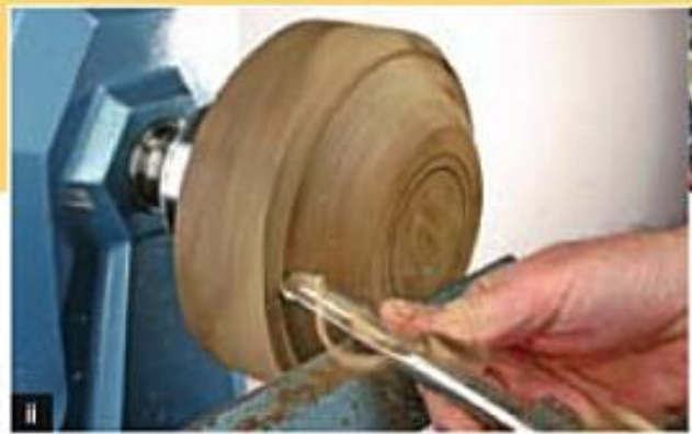
Cut 1 Shaping the outside – DFG.
