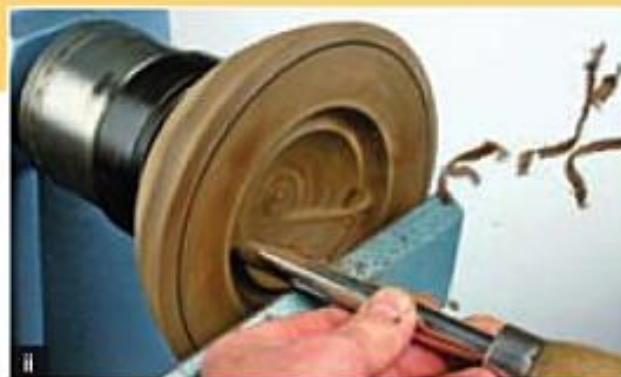
ii Cut 10 Hollow inside,
