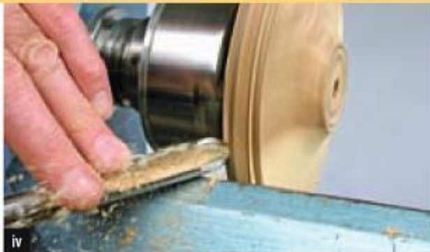
Cut 7 Clearing around the bead with DFG.
