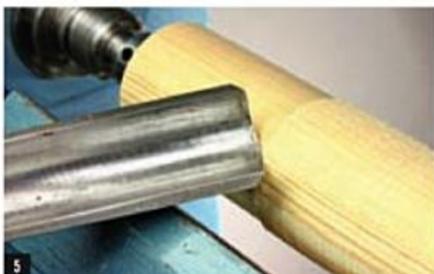
5 Bevel contact behind cutting edge, working from headstock. Leaves the perfect finish.
