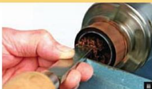
Cut 9 Refining inside lid shape and joint face shape with scraper.
