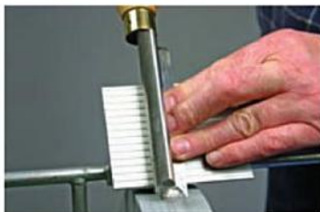
Above Sharpening the SRG on the Tormek platform in the start position; wheel running towards the tool.
