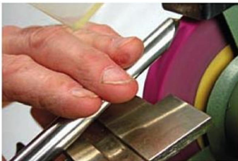
Above Manoeuvring the DFG in mid-position to achieve the swept-back grind.
