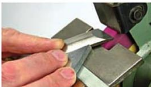
Above A skew chisel using a guide located in the platform.
