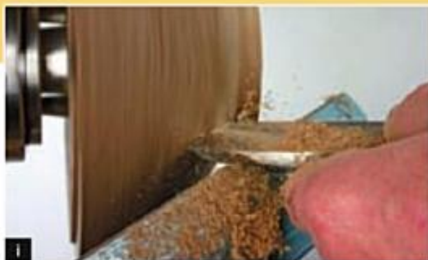
i Cut 7 Refine shape with scraper.
