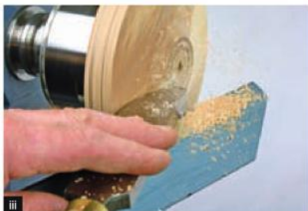
iii Cut 5 Refining top shape with large curved scraper.
