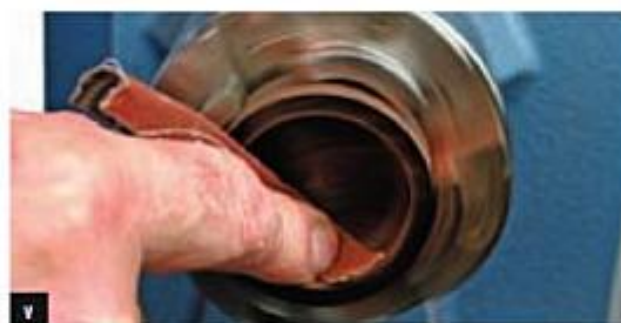
Sanding – inside the lid.
