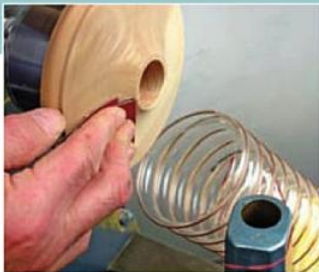
Above Using the cut edge of the abrasive to sand a bead detail.
