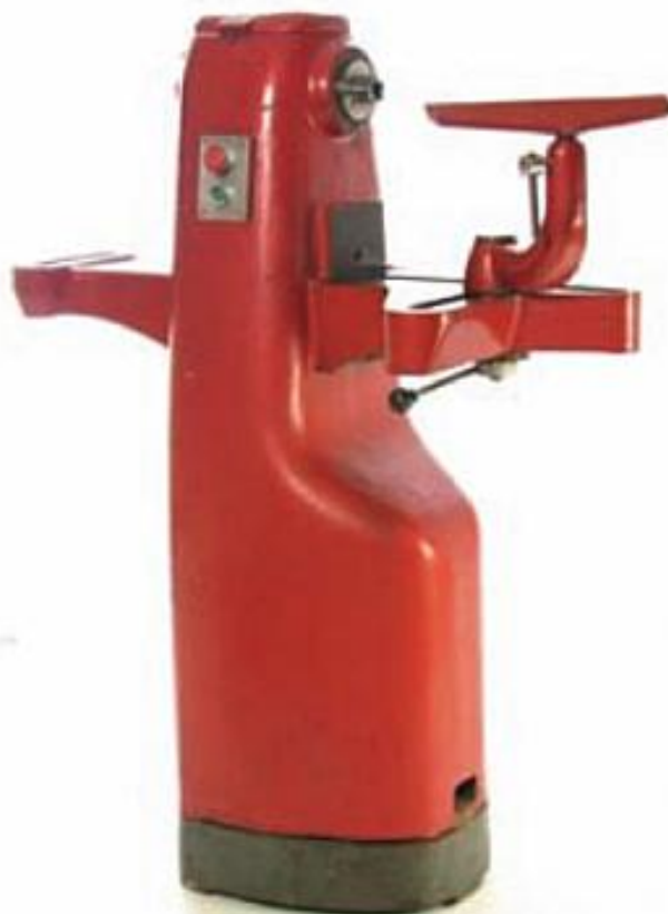
Above The Harrison Graduate shortbed four-speed lathe.
