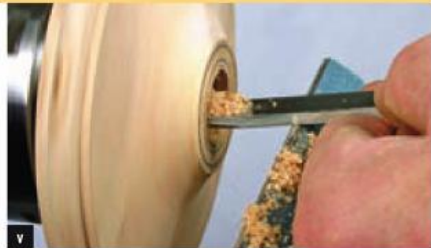
Cut 9 Boring for the lamp stem with square scraper.
