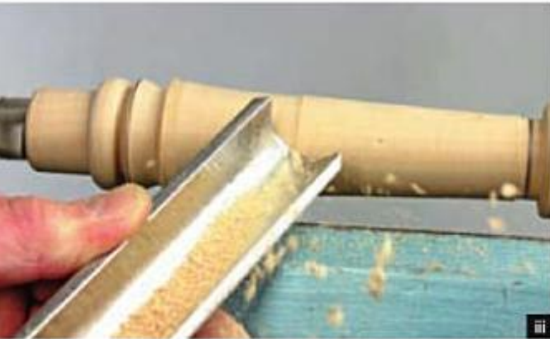
Cut 11 Shaping centre section between end detail with the spindle roughing gouge.
