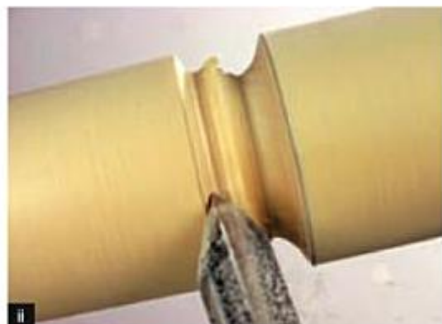
Turning a cove in three cuts.
