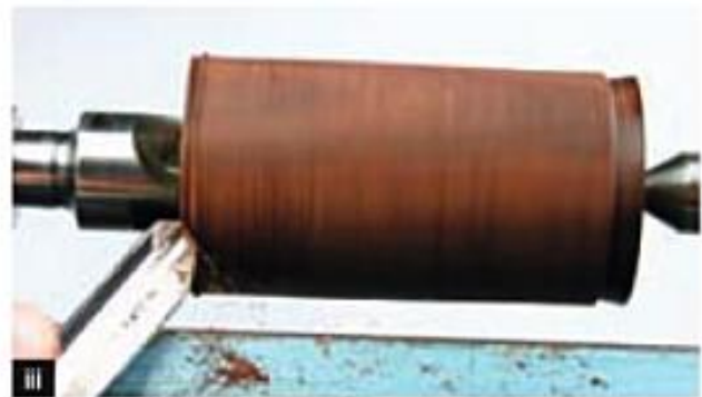
Cut 5 Turning spigot on headstock end with DFG.
