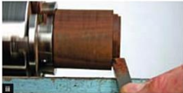
iii Making joint spigot full length.
