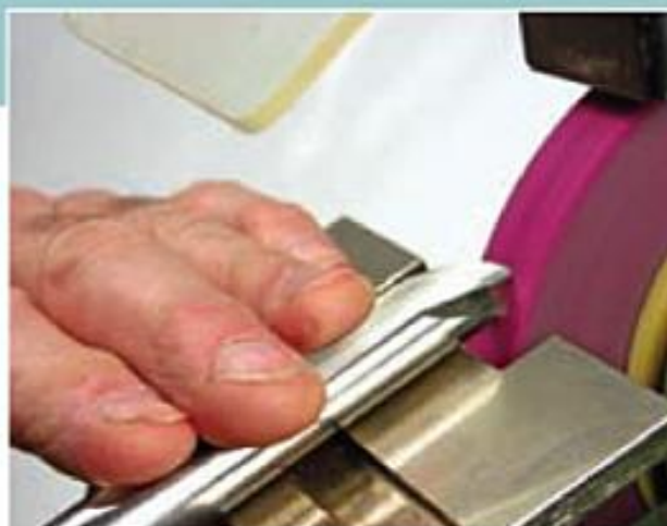
Above Manoeuvring the DFG in start position to achieve the swept-back grind.
