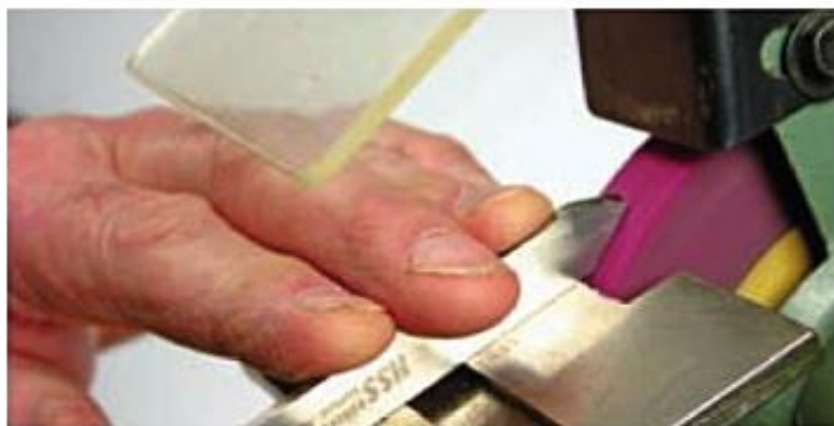
Above Sharpening parting tool on lower bevel.
