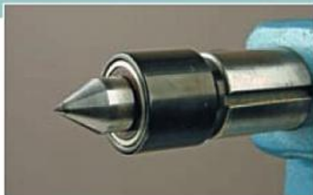
Above Revolving cone centre suitable for hardwoods; no. 2 morse taper.
