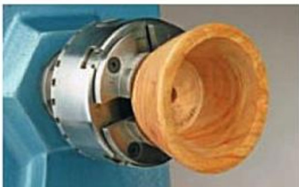
Above Jam chuck held in Vicmarc chuck.
