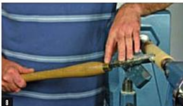
8 Right-handed smoothing cut, arm over headstock. Power grip for control hand, fingers grip for support hand.
