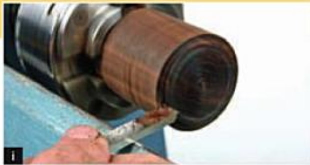
i Cut 12 Turning short joint spigot on base with scraper.
