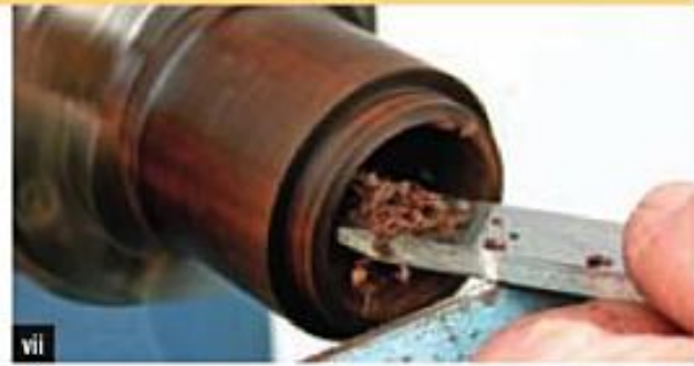
vii Cut 18 Refining shape with scraper.
