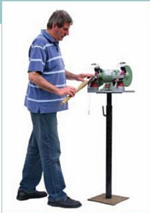
Above A dynamic stance for tool sharpening, standing to the side of the high-speed grinder.
