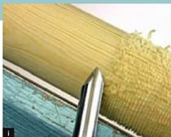
Making a smoothing cut.
