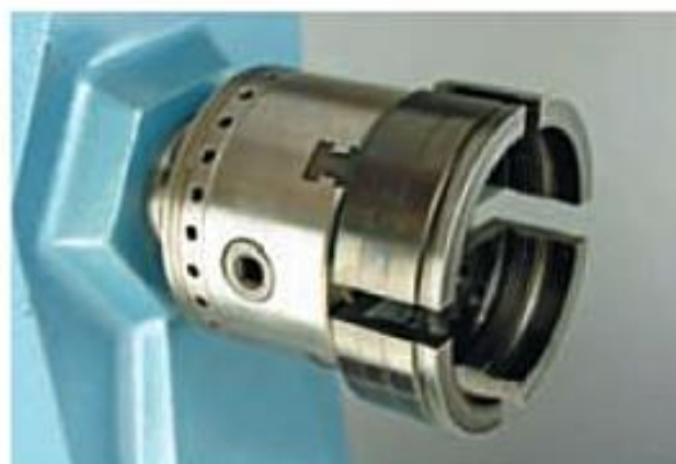
Above Vicmarc VM120 chuck with long nose jaws.
