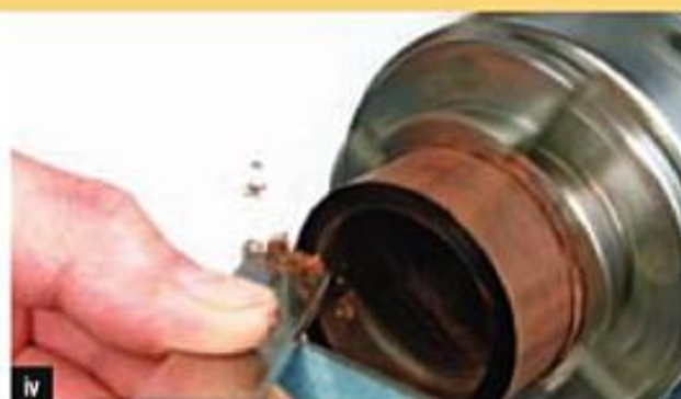
Refining top face with scraper.
