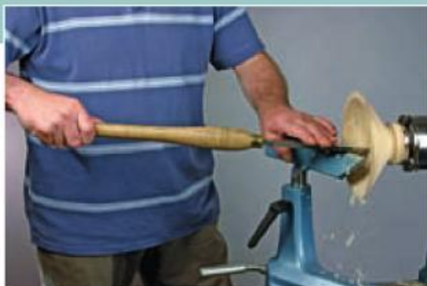
Power grip on the handle and fingers on the stock.
