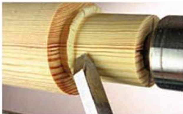
Rolling a bead with the point of the beading tool.
