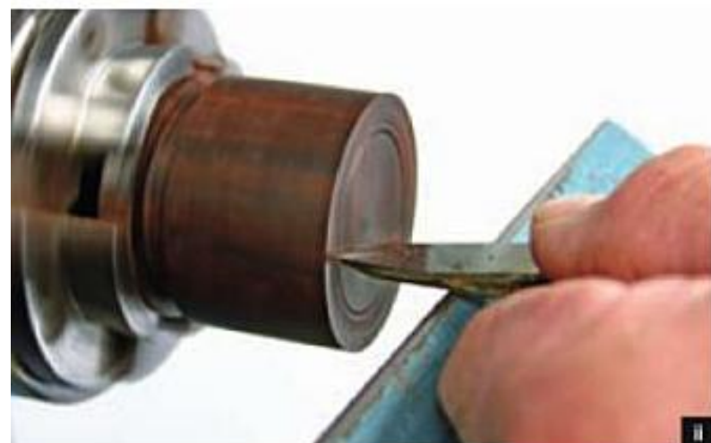
Cut 21 Put detail marks under base with pointed scraper
