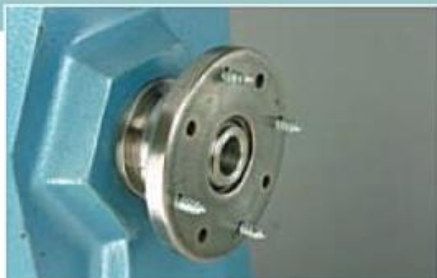
Above 4in-faceplate (multi-screw chuck); four straight holes and four countersunk holes.
