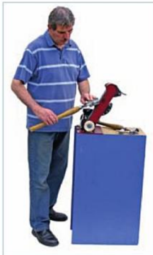
Above Comfortable height and stance for tool sharpening on the top of the Tormek wetstone grinder.
