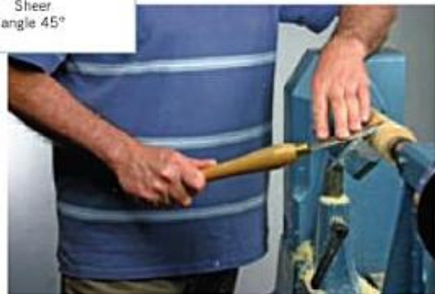
Power grip and fingers with arm over headstock.
