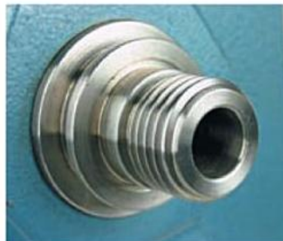
Above M33 threads and large registers on the Vicmarc spindle.
