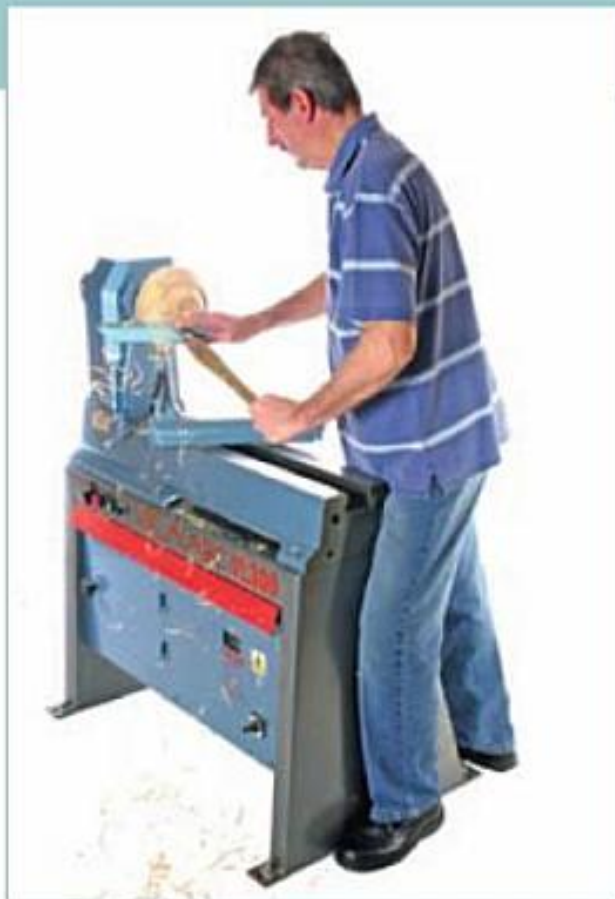
Above Turning the outside of a cross-grain bowl left-handed.
