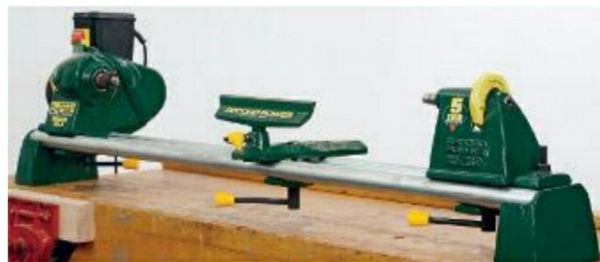
Photo 4. A bench-mounted model like this will suit most woodturning beginners
