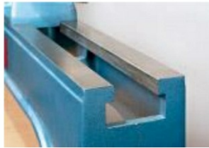
Photo 8. More expensive beds are solid castings that are almost a work of art
