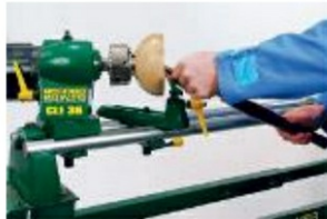
Photo 13. Swinging the head off-centre keeps tool handles clear of the bed
