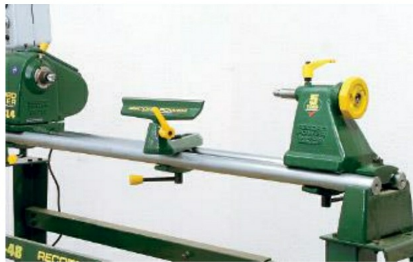
Photo 7. The lathe bed is made from heavy metal bars or tubes
