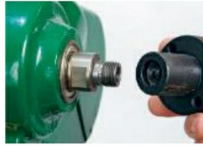
Photo 16. A spindle thread size of \frac{3}{4} in x 16 tpi is the industry standard
