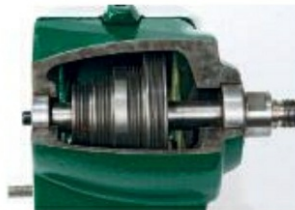
Photo 10. The bearings should be good quality heavy-duty ball races
