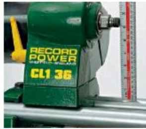
Photo 3. ...and a swing of at least 9in between spindle and bed
