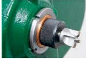
Photo 18. A solid spindle needs a centre ejector screwed onto the spindle nose
