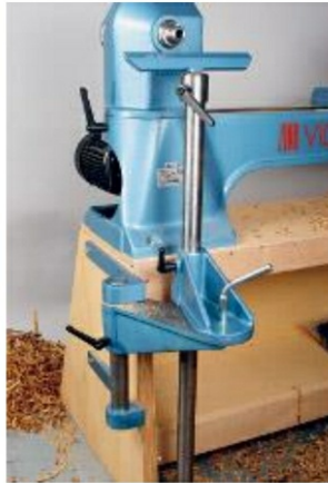
Photo 14. You need an additional tool rest for turning big-diameter bowls
