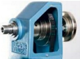
Photo 19. A three-or four-step pulley gives a speed range of 400-2000rpm
