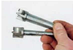
Photo 17. Morse tapers are a universal means of installing centres
