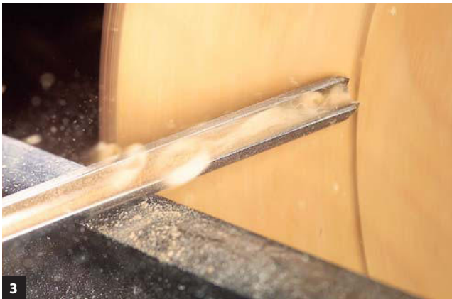
3 A 1/4" bowl gouge was traditionally used for finishing the inside or outside of a bowl. I prefer to make a light finishing cut with a 1/2" gouge that has a finger-nail profile (see "Edge Profiles:" page 9).
