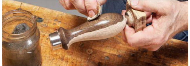
1 Wiping a solution created by immersing steel wool in household vinegar onto woods that contain high amounts of tannic acid causes a chemical reaction that turns the wood black.
