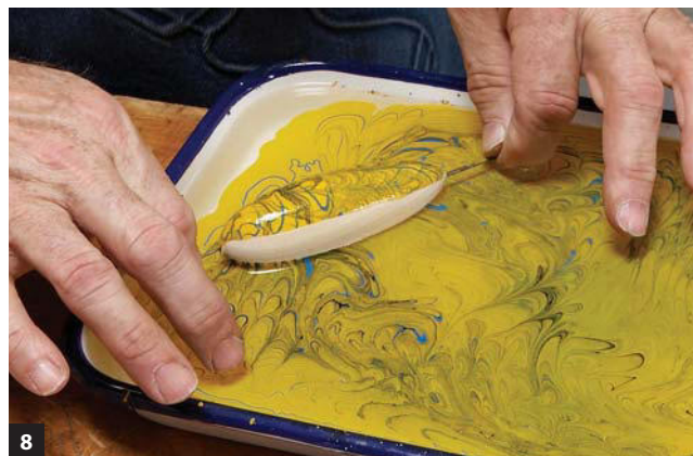
8 Gently dip the workpiece onto the paint and roll it across the pattern.
