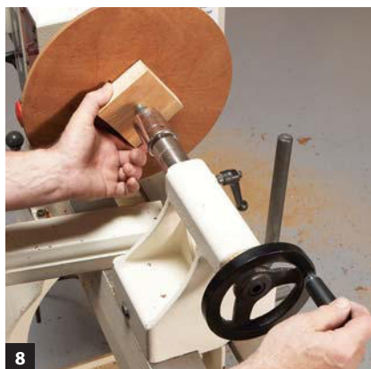
Remount the blank. Then use the tailstock and a block to clamp the taped joint. The block isn't glued; it's used to distribute the clamping pressure. Allow one hour for the tape's bond to fully strengthen.
