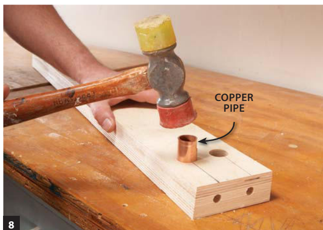
8 Tap copper tubes, made from copper pipe, into the holes. Drill through the ends of the rails and through the tubes to finish the joint.
