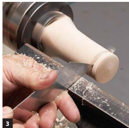
3 Cut in with the narrow parting tool to establish the disc.
