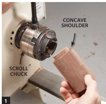
1 Mount the blank in a scroll chuck after turning a tenon on one end. The tenon's shoulder must be slightly concave.
