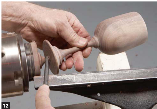
12 Part the goblet from the waste material after cutting into the underside of the base at a slight angle to create a concave bottom surface, so the goblet will sit flat.
