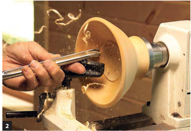
2 A 3/8" bowl gouge is a better choice if you own a mini-lathe. This gouge is large enough to turn a bowl as big as the machine can handle, but it's not so aggressive that it will bog down a mini-lathe's smaller motor.
