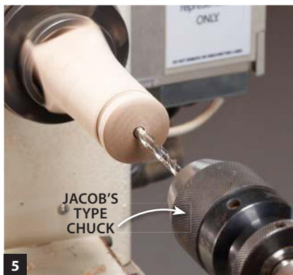
5 Use the recess and a Jacobs-type chuck mounted in the tailstock to drill a hole through the disc. This hole must be precisely centered for the top to spin without wobbling.
