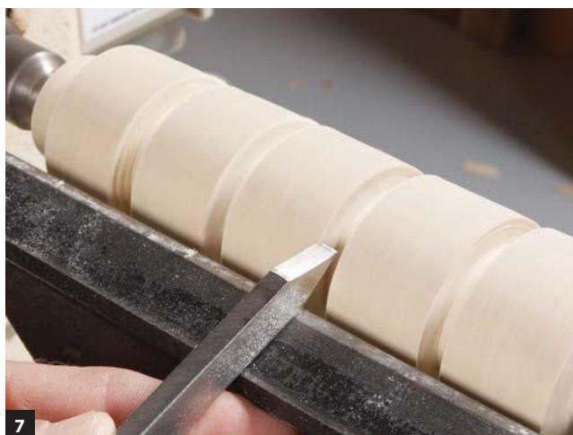
7 Time to use the rolling cut to make beads. Lay out a series of 1" to 1-1/4" wide beads with the parting tool. Cut down on each side of the bead about one-third the diameter of the cylinder.
