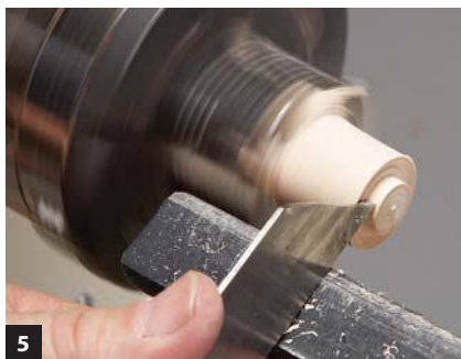
5 Mount a short, square blank for the top. As before, work from the tailstock end of the blank towards the chuck. On a short cap like this one, the tenon can go on either end.
