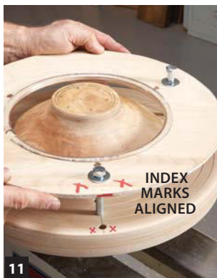
11 Install the ring and use it to clamp the bowl to the plywood base using bolts, washers and wing nuts.
