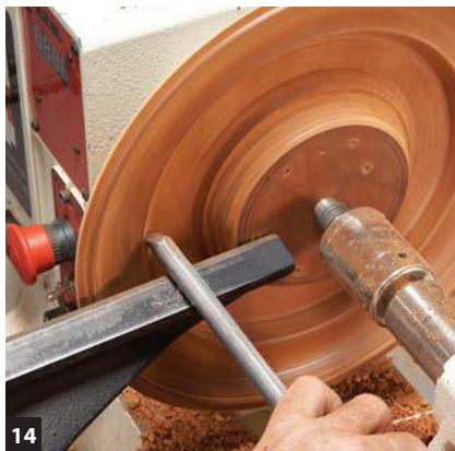
14 Establish the plate's depth. Cut in decisively from the edge of the rim, plunging down and towards the center.
