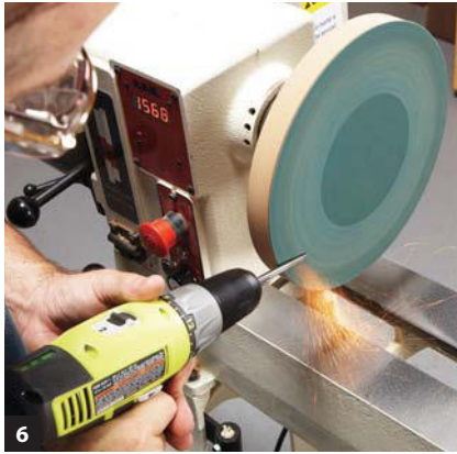
6 Shape a tapered point on the shaft using a drill and a lathe mounted abrasive disc. With the drill running, grind the point on the near lower quadrant of the spinning disc. Wear eye protection!
