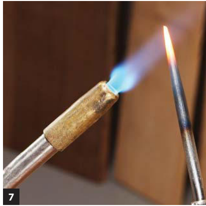
7 Harden the shaft by heating the pointed half to an even cherry red color. Hold the shaft in a pair of locking pliers.
