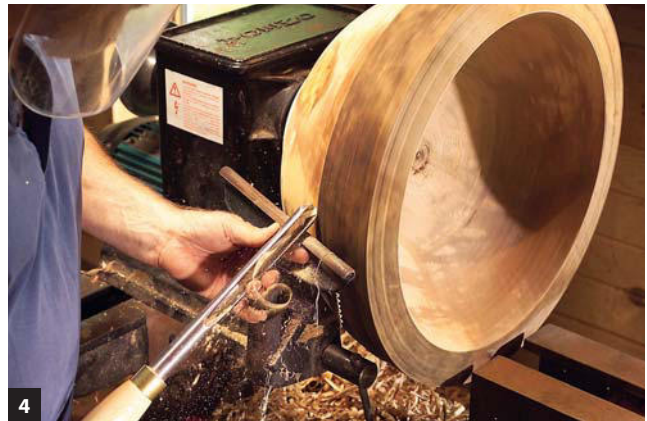
4 A 5/8" or 3/4" bowl gouge is useful for making heavy, aggressive cuts on bowls larger than 14" in diameter. Turning a monster bowl usually requires a heavy-duty, large-capacity lathe with a 2-hp or larger motor.
