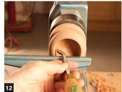
12 Switch to a bent round-nose scraper to create a concave area under the base's rim. When you're done with all turning and sanding, part off the base.
