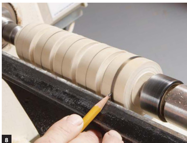
8 Draw a broad pencil line at the center of the bead. The skew should never cut in this region. When you sand the bead, the marked area will blend nicely into the rounded sides.
