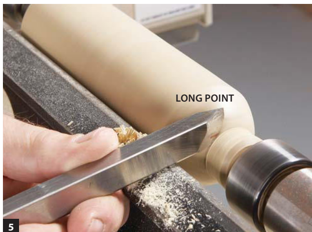
5 Complete the cut with the bevel of the skew vertical to the axis of the lathe. The tool will stop cutting at this point. Pull the tool straight back to avoid catching the wood with the long point.
