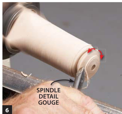
6 Shape the body as you would roll a bead. Start at the edge and cut toward the center, rotating the gouge as you go. When shaping the back, don't cut all the way to the center hole.
