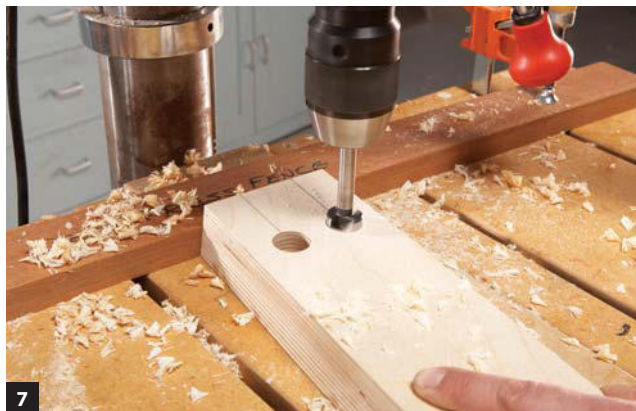
7 Drill holes for the copper tubes using a \frac{7}{8} " Forstner bit. Precision is important for a strong joint and easy assembly.
