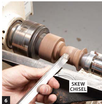
6 Refine the bowl's shape and add decorative elements such as tiny beads with the gouge and the skew chisel.
