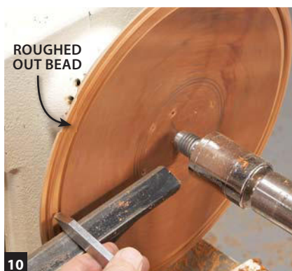
Always work from the outside edge towards the middle when shaping the open side of the blank. Start by creating the rim. It can be flat, curved or detailed. Here, cutting in with a parting tool roughs out a bead.
