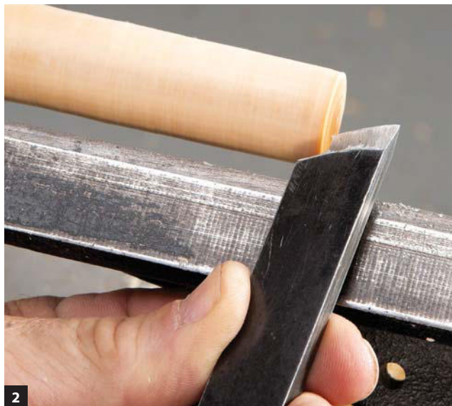
2 Use the modified skew to practice rolling shavings on a scrap block of green wood turned to a cylinder. Start by positioning the point of the hook at a low entry level.
