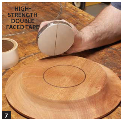
Remount the faceplate on the outside of the blank, using the centered circle and high-strength double faced tape. Trim the tape to match the faceplate.
