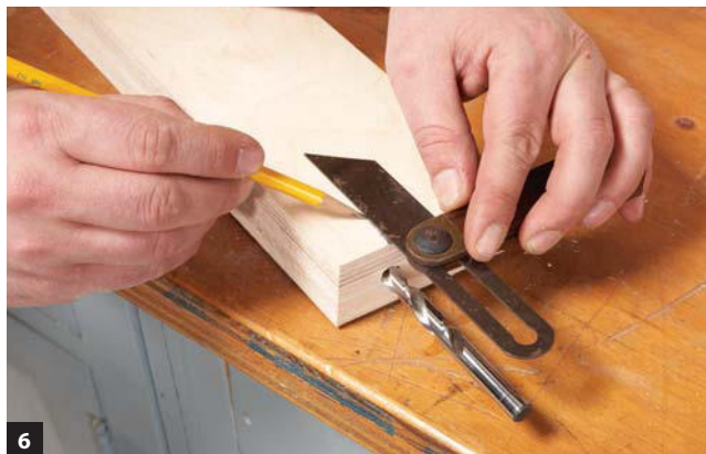
6 Insert the same drill bit into the rails. Using a sliding bevel, transfer the bit's angle to the rail's face. This enables you to find the exact center of the holes for the copper tubes that will hold the nuts.
