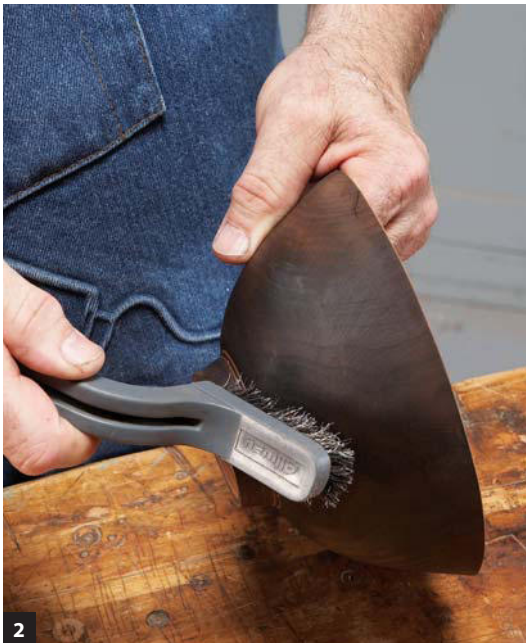
2 Brush off the loose debris with a soft bristle brush. Repeat the process, if necessary, to create a consistent black color. Then apply an oil finish to intensify the black.
