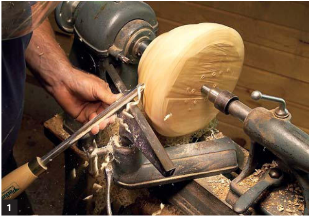
1 A 1/2" bowl gouge is a nicely balanced size for most bowl turning on a standard-size lathe (see Sources, page 9). With this workhorse tool, you can turn 5" to 24" diameter bowls.
