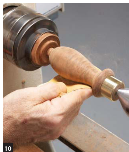
10 Finish-sand the handle. Start with #120-grit; if turning marks remain, drop back to #100-grit. Sand to #220-grit, or further if you still see sanding scratches. Sand the brass ferrule to the same grit.
