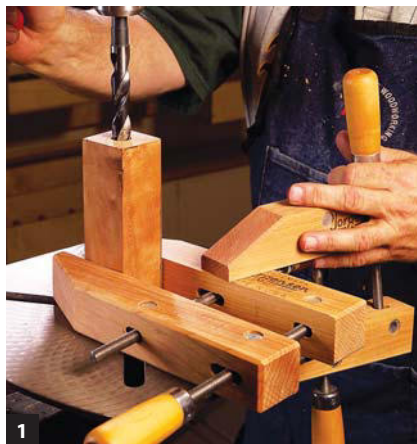
1 Drill a 5/8"-dia. starter hole in a square blank. Make the hole 1 in. deep.
