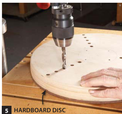
5 Drill through the hardboard disc at every hole in the plywood base to create a template for drilling the chuck's rings.
