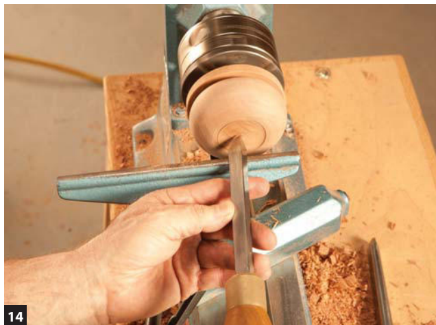
14 Complete the underside of the base using the half-round scraper. Raise the scraper on edge, as shown here, to make the final finishing cuts.
