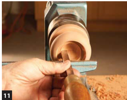
11 Use a half-round scraper to hollow most of the base's interior.
