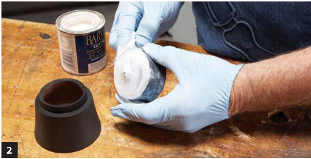
2 Wipe on white gel stain to fill the pores. Continue wiping until the stain is completely removed from the surface.
