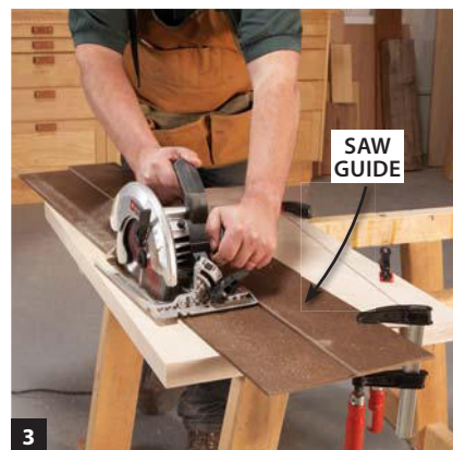
3 Use a saw guide and a circular saw to taper the legs.
