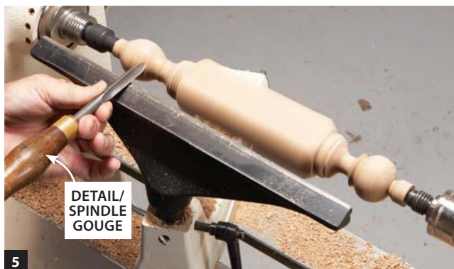
5 Shape the knobs with the detail/spindle gouge and the skew. The knobs don't have to match, because you're creating two separate doorstops. Ball or bulb shapes are easiest to grip.
