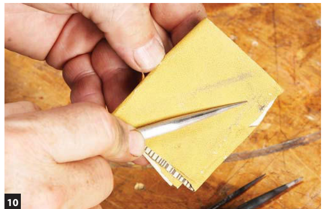
10 Sand the steel to a bright, clean surface with #220-grit paper. Wash it with soap and water to remove oil residue first.
