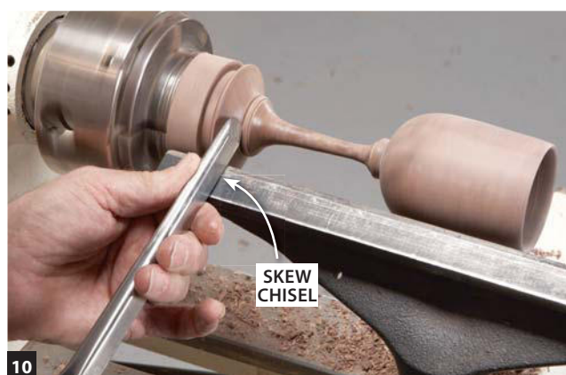
10 Complete the base and add details, using the detail/spindle gouge and the skew chisel.
