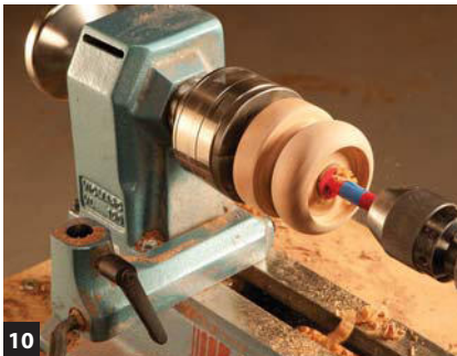
10 Remove the lid, then drill the base to roughly establish the depth of its interior. This step also simplifies hollowing the base.
