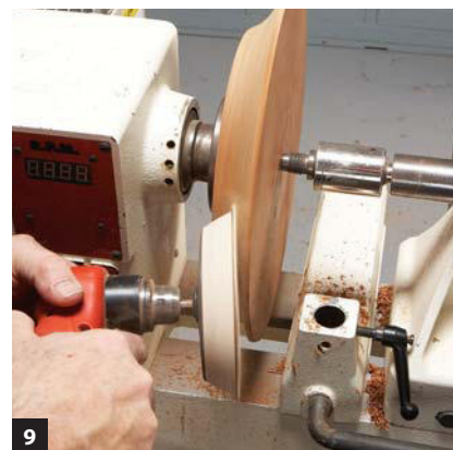
Sand the back of the rim using a cushioned disc and a drill set to rotate clockwise. Before sanding, remove the clamp block and reposition the tailstock so it continues to support the plate.
