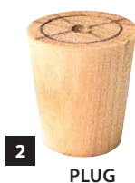
2 Turn a tapered plug to fit in the hole. Put the plug in the hole and mount the blank on your lathe. The plug's center bears against the point of the live center in the tailstock. You may use a metal cone-type center as well.
