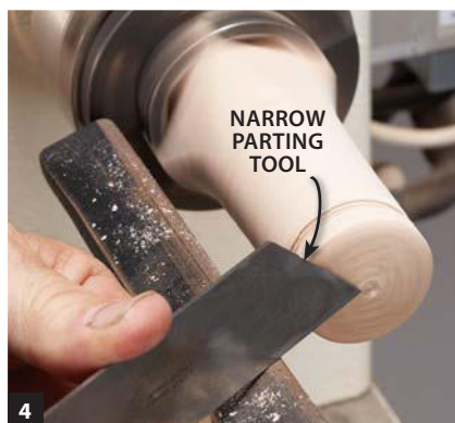
4 Exactly center a tiny recess in the disc's face.
