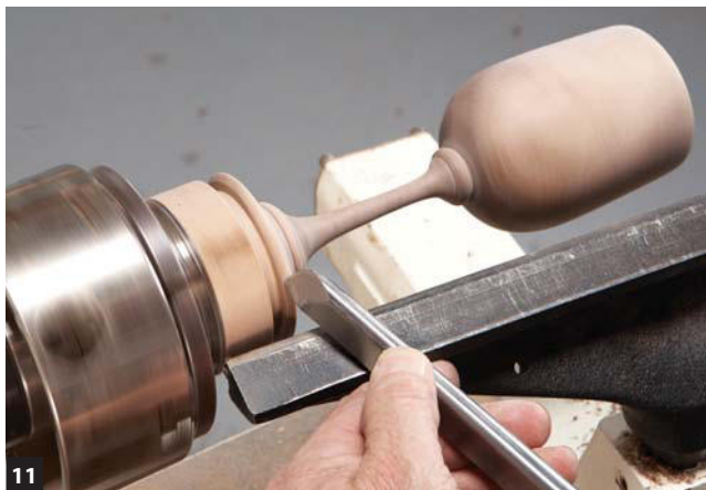
11 Refine the rim of the base by making an angled cut on the bottom edge, using the long point of the skew chisel.
