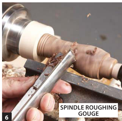
Complete the barrel by connecting the two ends. If you decide not to add a ferrule, leave extra thickness at the joint to keep the wood from splitting.
