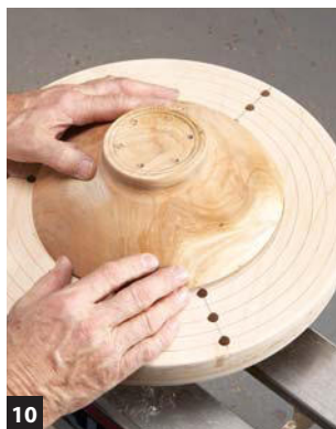
10 To use the chuck, start by roughly centering a bowl on the appropriate groove cut in the base.
