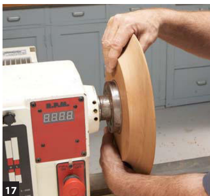
17 Remove the plate from the faceplate with a slow, steady pull. Remove any tape or residue that remains with mineral spirits. Finish-sand the back side of the plate by hand.
