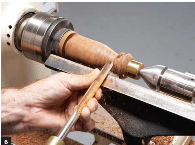
6 Reduce the diameter behind the flange to create the neck. From this point on, remove the handle often to check how it feels in your hand.
