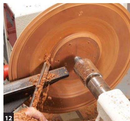
Remove waste beyond the rim, using the bowl gouge. Plunge down and toward the center, using the bowl gouge. This step provides clearance, so you can complete the rim.
