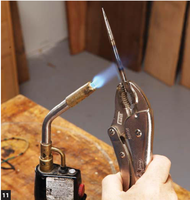
11 Temper the shaft with a torch held just below the heat-treated area. Keep the flame there and rotate the shaft until the hardened area is a uniform dark gold or bronze color. Then, quickly quench it in water.
