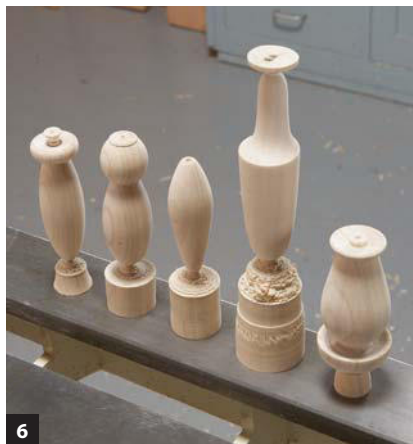
Most lures take ten minutes or less to turn, so it makes sense to turn multiples, whether they’re unique or all the same. Leave the waste attached for now—it makes painting much easier.
