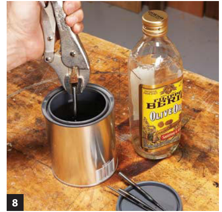
8 When the steel is evenly bright red from the point to the middle, quickly quench and stir it in a can of olive oil.
