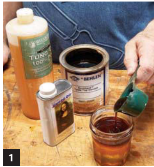
Mix equal parts pure tung oil, boiled linseed oil and gloss varnish. Premium ingredients are the key to this finish.
