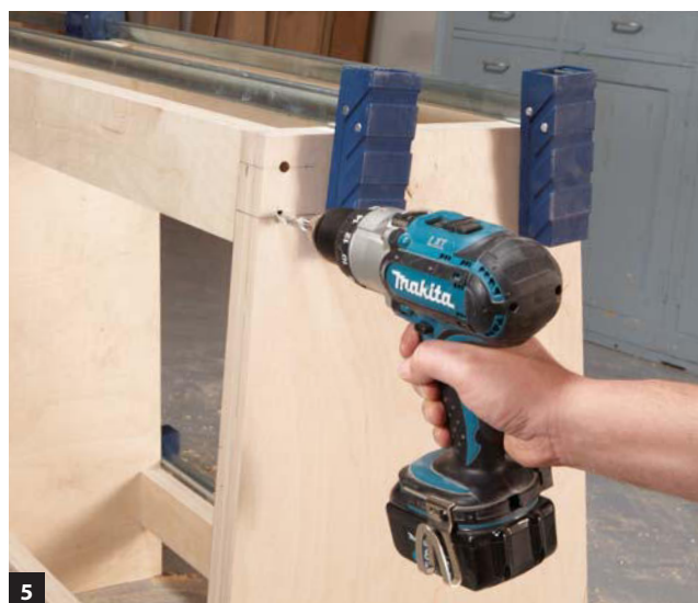
5 Drill into the rails through the holes in the legs. Disassemble the base.
