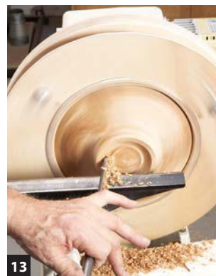
13 Use this chuck to create a hollow base with a rim, add lines or beads, remove screw holes and chuck marks or fully round the bottom.
