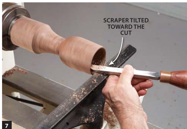
7 Finish hollowing the cup by making light passes from the bottom to the top edge with the scraper tilted toward the cut. Then sand the inside of the cup and the upper part of the outside.
