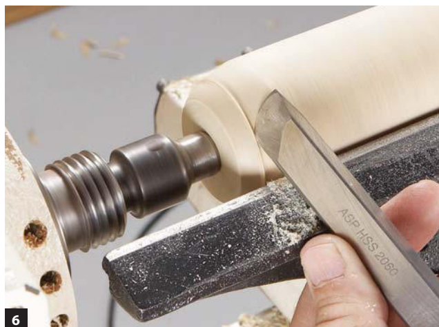
6 Practice on the other end of the cylinder. You find one side is easier than the other. Practice extensively on the weak side until you're comfortable with the rolling cut in either direction.
