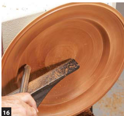
16 Make a light, cleaning cut with the bowl gouge to blend the transition between the previous two cuts. Switch to a square ended scraper to level the surface. Then finish-sand this side of the plate.
