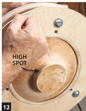
12 Center the bowl with the chuck mounted. Mark the high spot. Gently tap it as necessary and then tighten the wing nuts.
