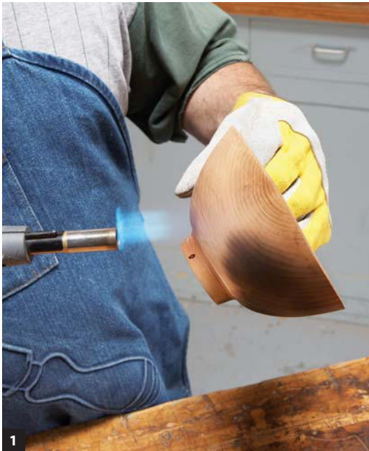
1 Lightly scorch the wood with a torch. Move the flame continuously and quickly so the wood doesn't overheat.
