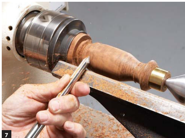
7 Start to shape the end of the handle. Be sure to leave sufficient waste, so you don't whack into the chuck.
