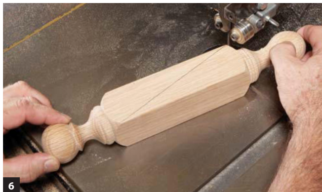
6 Cut diagonally across the pommel to create two wedge-shaped doorstops. The sawn edges are the bottoms. Flatten them by sanding.
