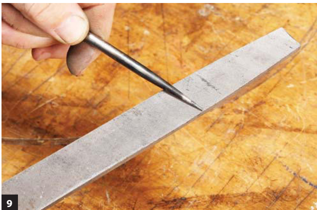
9 Test the hardness of the shaft by running it along a file. The hardened part should skate off the file, not bite in.
