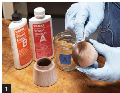
1 Remove the wood's natural color with two-part wood bleach. Several applications may be necessary.
