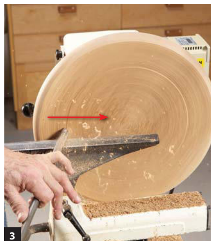
3 Hollow the seat using the bowl gouge, working from large to small diameter.
