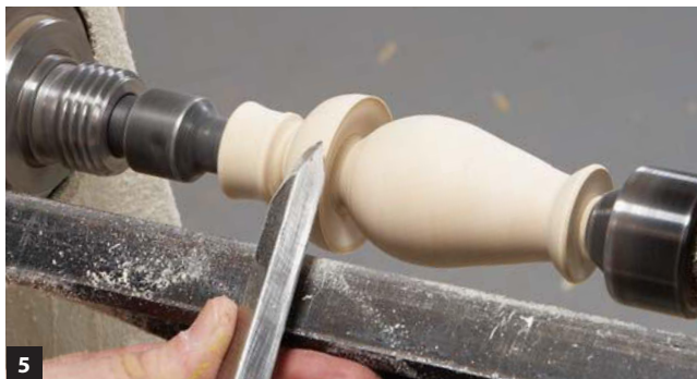
5 Create your own designs. I call this one the “Leapin’ Lacer.” The turning is just a squat-shaped ellipse with hollowed collars at both ends. But to a largemouth bass, the completed lure will look like a tasty frog (Photo 10).
