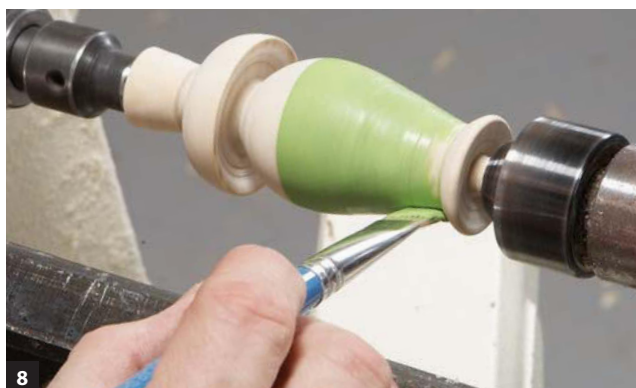
8 Here’s the lazy man’s painting method—just hold the brush and let the lathe do all the work. Run the lathe very slowly and thin the paint so that it flows evenly onto the lure.
