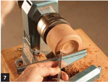
7 Gradually increase the mortise's diameter using a small parting tool—make diagonal cuts until the tenon barely fits, then finish with a straight cut.
