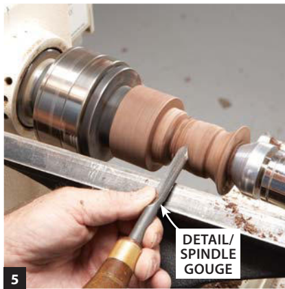
5 Use a detail/spindle gouge to roughly shape the outside of the cup, including the flared rim.
