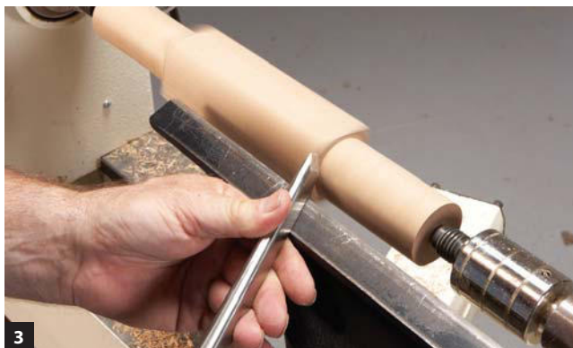
3 Square each pommel shoulder after rounding the ends, by cutting in at the layout line, using the skew with its long point down.
