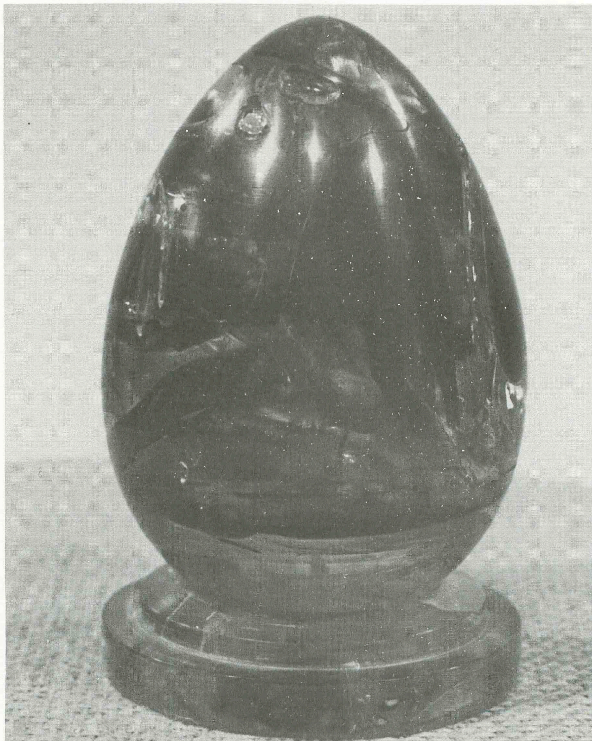
Fig. 5-22. Dyed and pigmented resin turned to egg shape.
