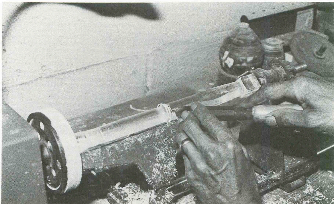
Fig. 2-11. Turning acrylic with specially ground tool. Waste comes off acrylic in long spirals.
