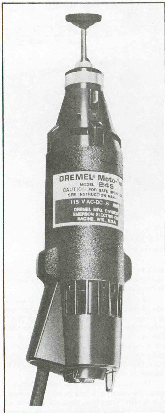
Fig. 1-9. This tool was often used by hobbyists as the nucleus for a little lathe.
