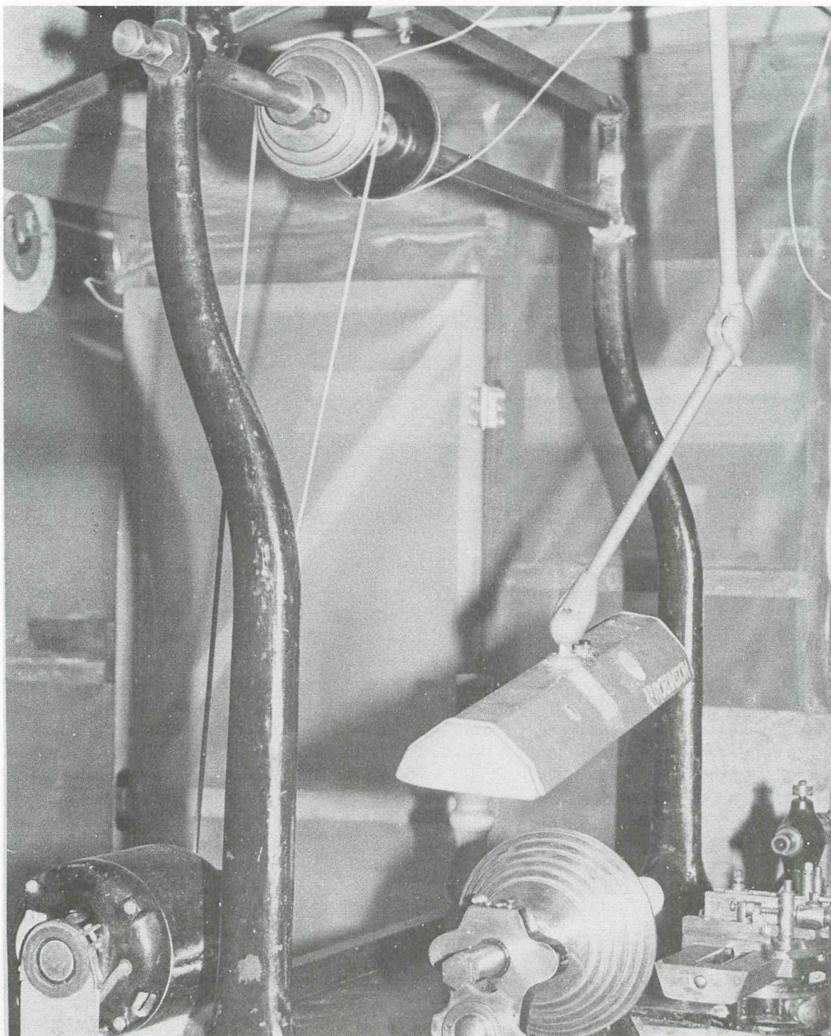
Fig. 14-15. Supports for overhead assembly before refinishing.
