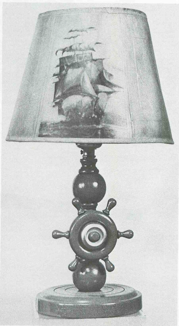
Fig. 5-32. Lamp made up of individual beads, collars, discs, and pegs, all lathe turned. They are held erect by a metal pipe up the middle.
