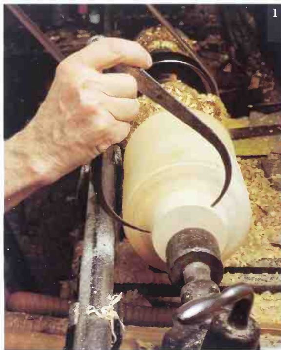
1. The diameter of the spigot must fit into the cup chuck.
