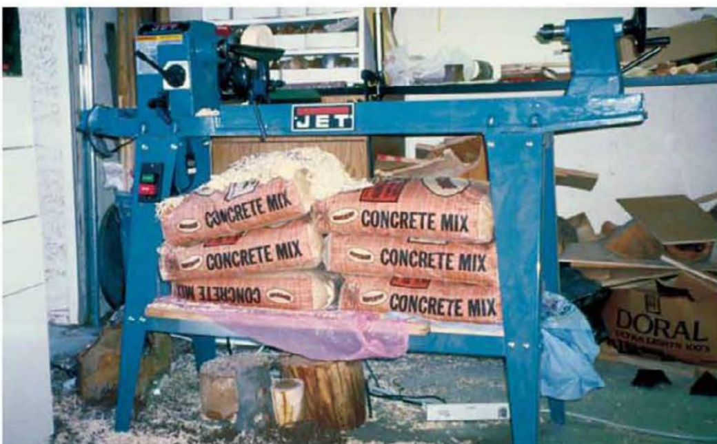
When turning off-balance work on a small lathe, it's a good idea to stabilize the machine. Bags of concrete mix work well.
