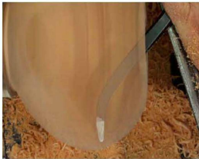
Three Kelton Hollowers are employed on different portions of the curve as it is refined.
