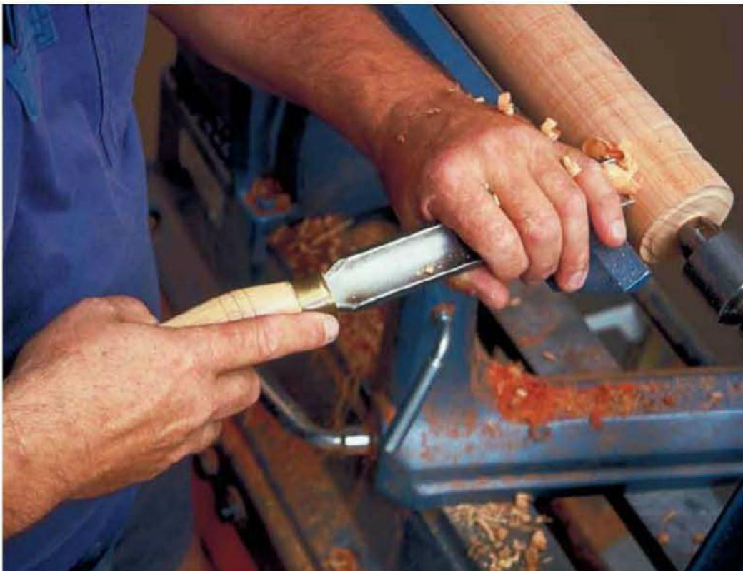
A hand-over grip is ideal for roughing a spindle blank when the tool is moved flowingly from one end of the rest to the other.
