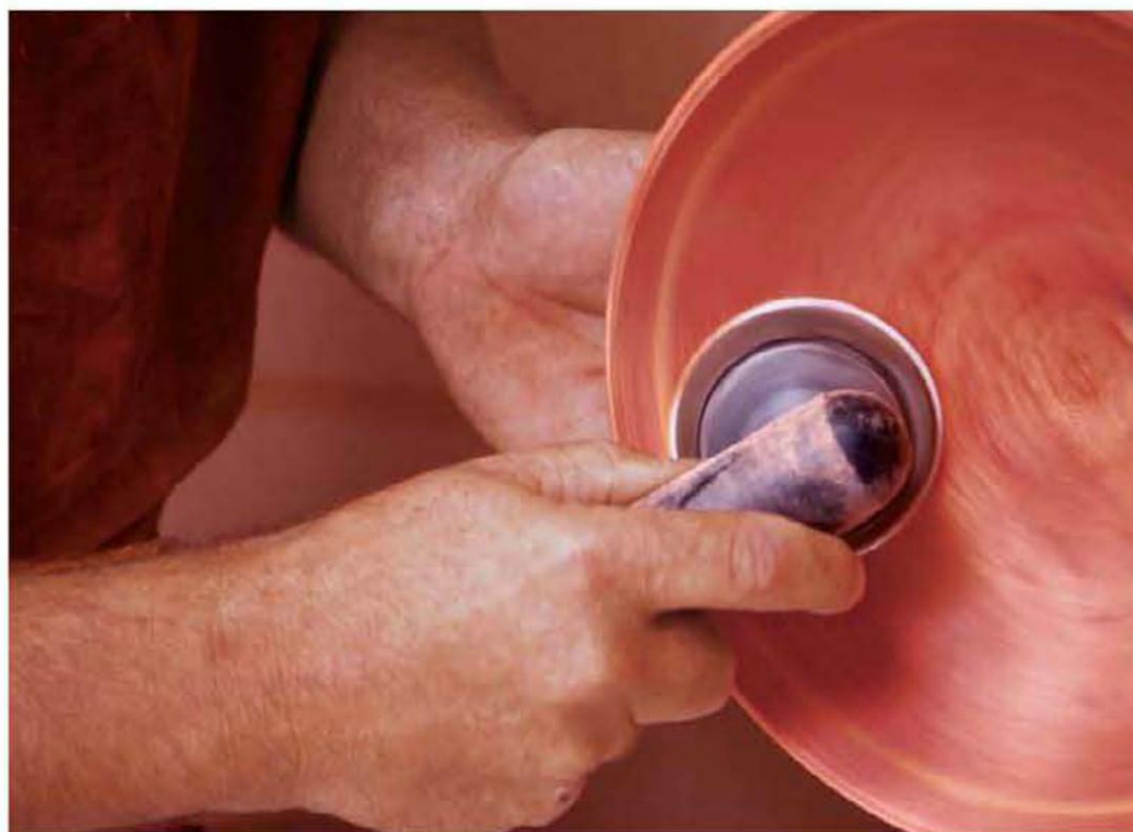
The Rotary Sander is similar to an angle drill. Powered by the rotating wood, the tool produces the finest sanded surface.
