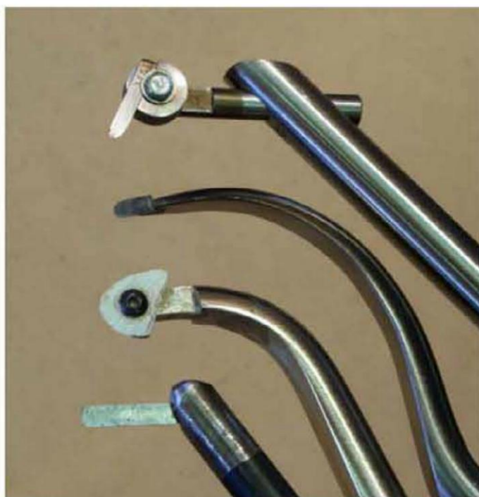
The first hollowers, similar to the lowest, were homemade, tricky to use freehand, and ever likely to catch; then the Stewart swan-neck hollowers, center, made freehand hollowing much easier. The Jamieson cutter, top, is used in a hollowing rig that prevents the tool catching as it reaches into corners traditional turning tools cannot.
