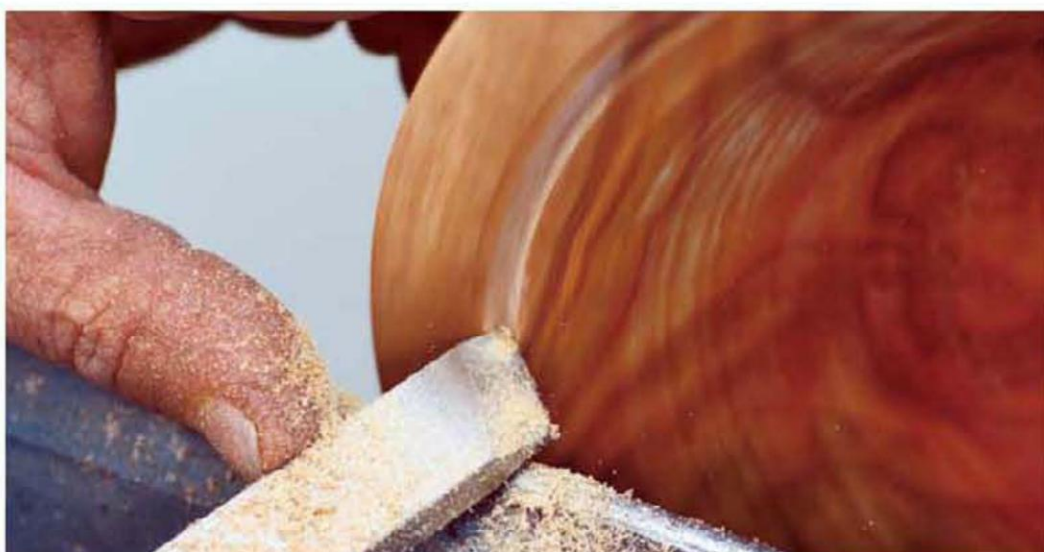
If you have trouble with the tool kicking back while making an entry cut, use a skew chisel flat on the rest to cut a small shoulder against which to rub the gouge bevel.
