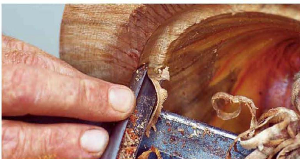
(TOP) For the entry cut, have the tool on its side with the bevel aligned in the direction you want to cut. (BOTTOM) Then roll the tool slightly counterclockwise to pick up a better shaving.
