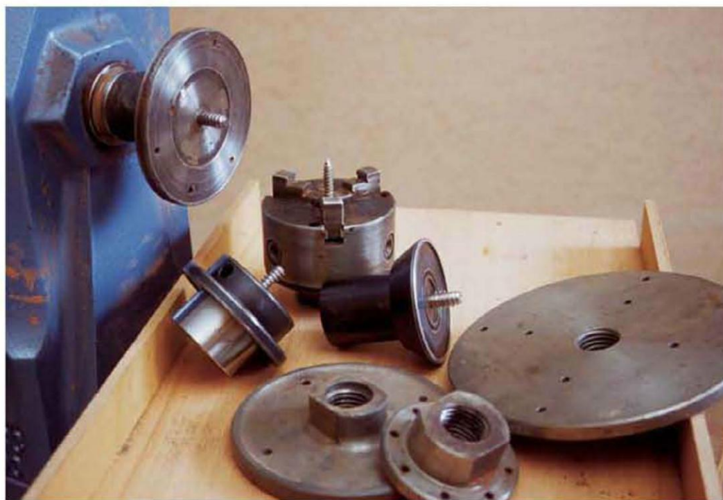
The faceplates in the foreground came standard with my lathes. The screw centers to the rear and on the lathe are easier to use.
