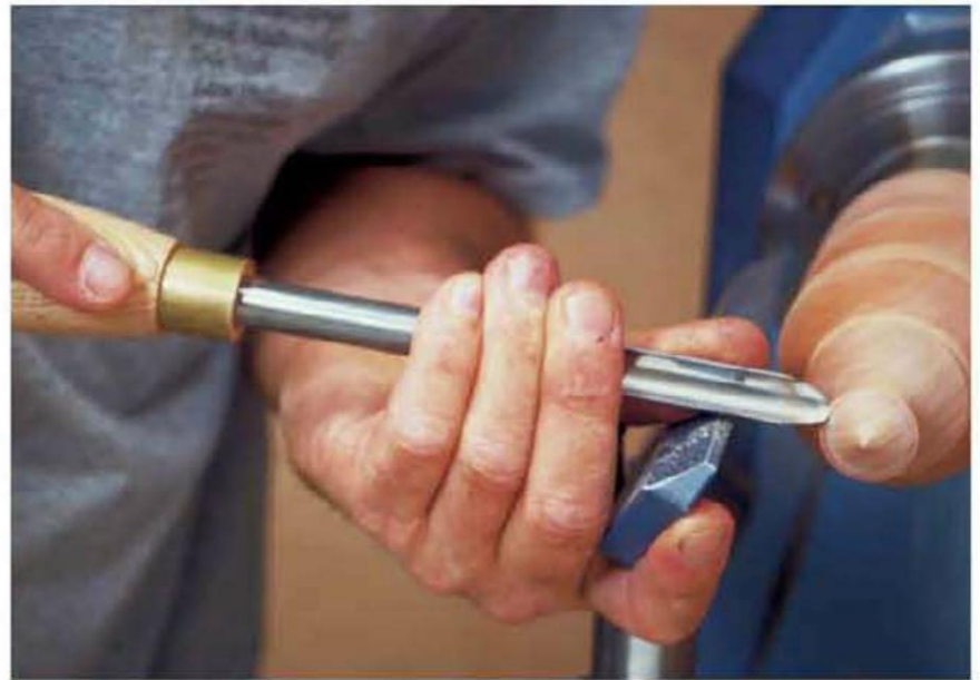
This secure hand-under grip gives very precise control of the edge for precision detailing.
