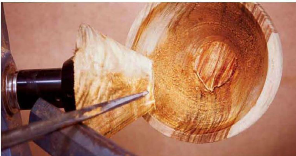
A Stewart System Slicer is used to save the inside of a bowl.
