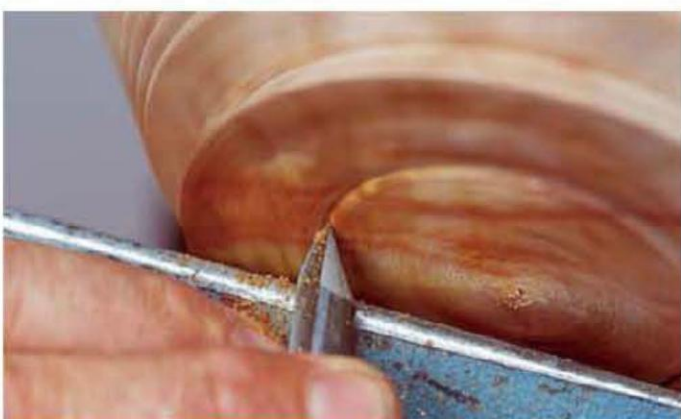
(TOP) To cut a groove into a face, start the tool on its side, then pivot it into the wood. (BOTTOM) Pivot the edge in from the right to clean up the right shoulder.
