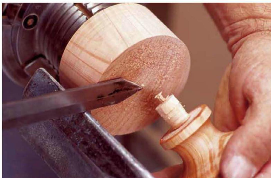
When parting-off, be sure to catch the work so it is cut, rather than pulled, off the lathe.
