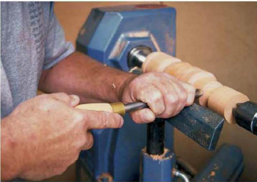
In this very controlled hand-over grip, my hand is planted firmly on the rest to prevent lateral movement along the rest. This grip is useful when cutting beads or grooves.
