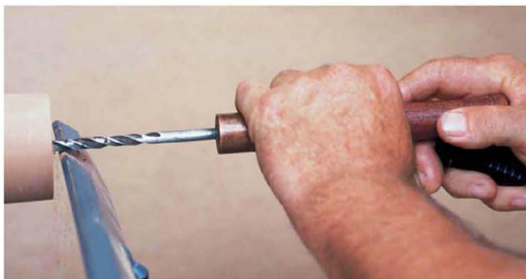
(TOP) To drill a depth hole, first cut a small V to get the drill started. (CENTER) Then rest the drill bevel on the V cut. (BOTTOM) Bring the drill parallel to the lathe axis and push into the wood.
