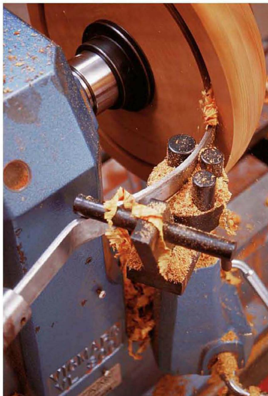
The McNaughton System uses a vertical gate and antikick-back arm to counteract the leverage exerted against the curved blades.
