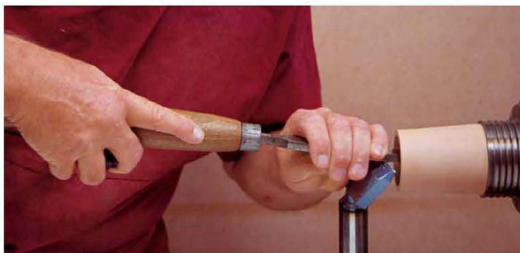
Using scrapers on end grain, raise the tool rest so that as you start a cut at center, the tool tilts down a few degrees. For a flowing internal curve, ease your elbow down on the handle and don't move the tool forward on the rest.
