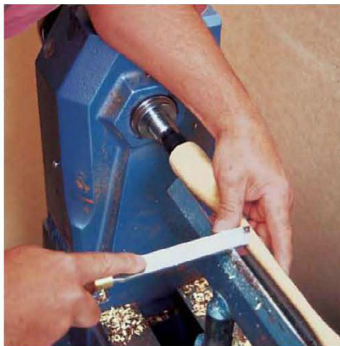
Extra support from the lathe, here from leaning on the headstock, always makes the job easier.
