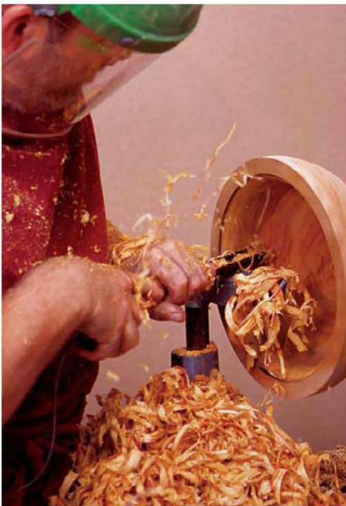
When roughing a bowl using a deep-fluted gouge, these are the shavings you're after.
