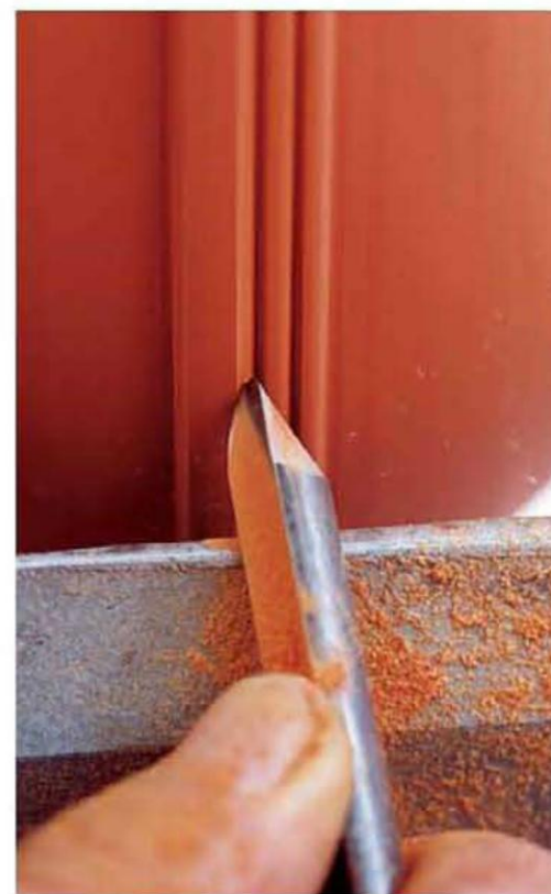
(LEFT) Beads sitting on a curve are blocked out, (RIGHT) then cut using a \frac{3}{8} -in. (9mm) shallow gouge.
