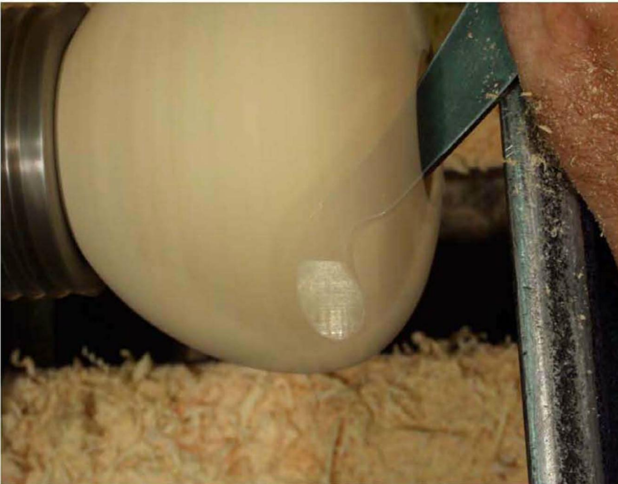
The round Kelton Undercutter was all I needed to hollow this 4¼ in. (110mm) diameter vessel. The opening is 1⅜ in. diameter.
