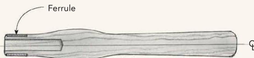
Fig. 2: For square-section tangs, drill the first hole 1 1/2 in. (38mm) deep. Use a bit the same diameter as the shaft, about 3 1/4 in. (80mm) from the end.
