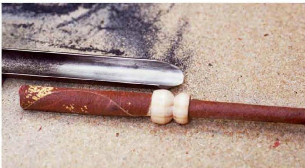
A used 120-grit sanding disc wrapped around doweling honed this flute smooth in preparation for grinding.
