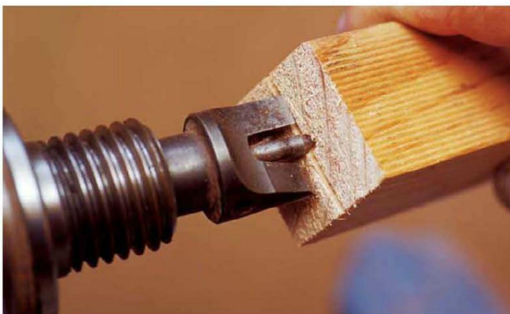
A bandsawn \frac{1}{16} -in.- (2mm) deep slot improves the grip while keeping the spur drive from boring into the end grain.
