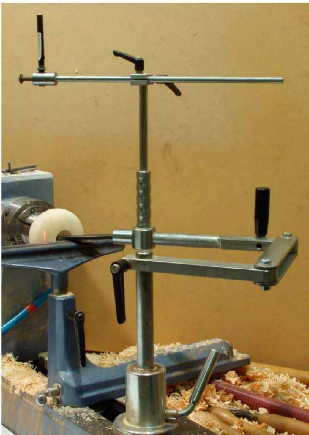
The Vicmarc Tool Support accepts a range of standard cutters and hollowers and is very easy to set up.
