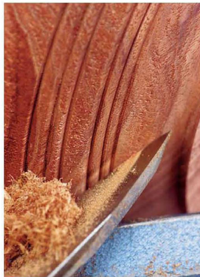
Shear-scraping with a spear-point scraper.
