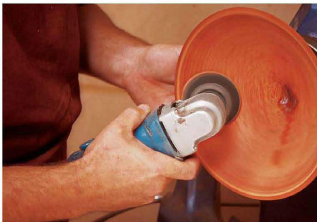
An angle drill is easier to handle than a conventional drill and you can use it one-handed. Use the trailing edge of the sanding disc to avoid a catch.
