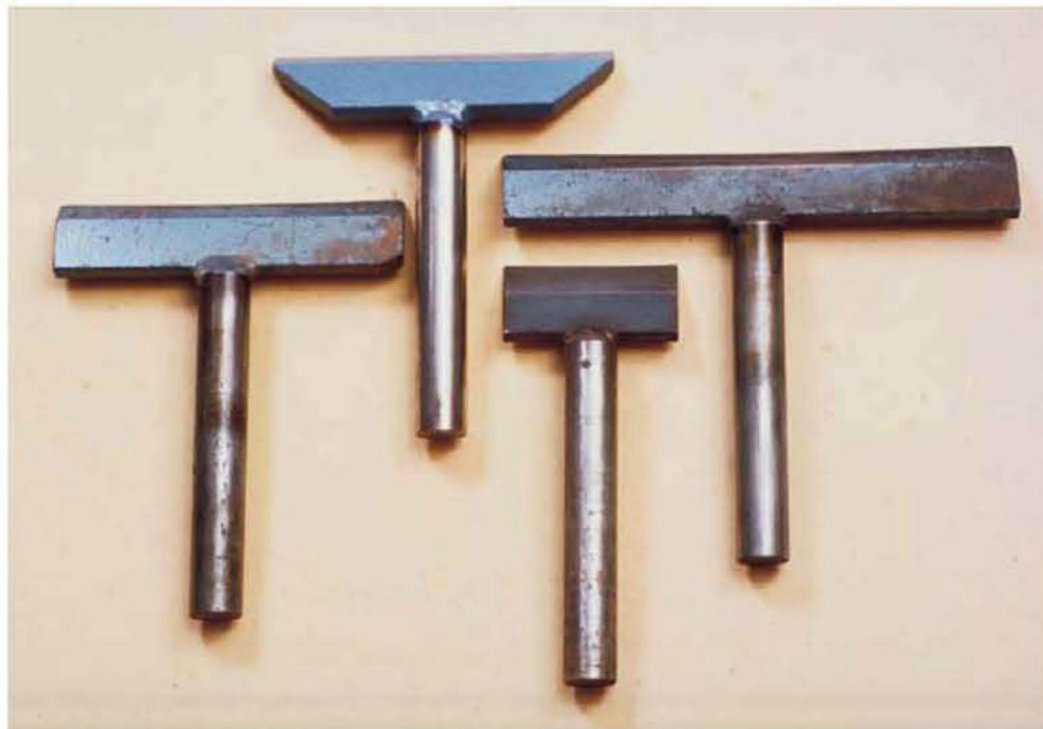
A range of tee rests makes life at the lathe easier. Never use a longer rest than you need.
