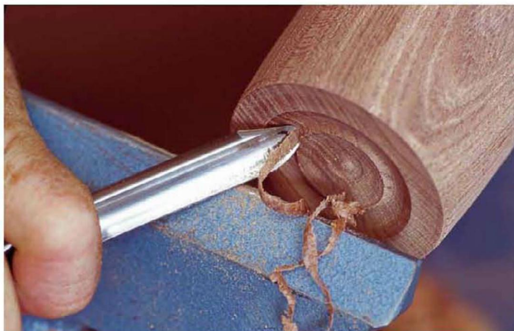
Hollowing end grain from the rim.
