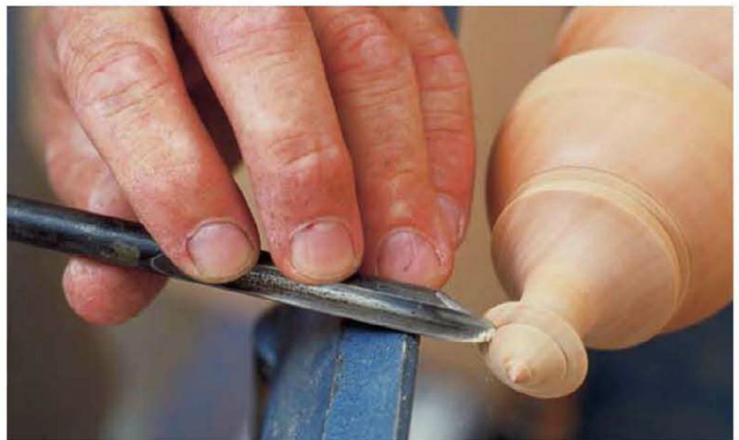
When the tool can kick back in only one direction, as when truing end grain, a stop grip is sufficient. The lower hand keeps the tool pressured against the top hand's fingers, which ease the blade into the cut.
