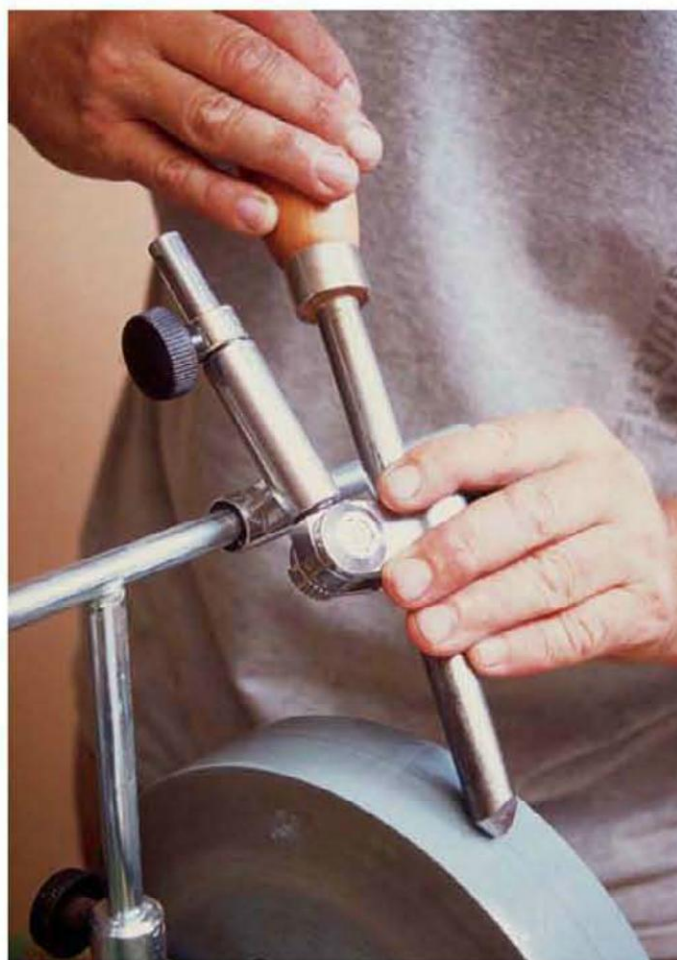
Grinding jigs ensure a perfect edge every time, here on a shallow gouge.
