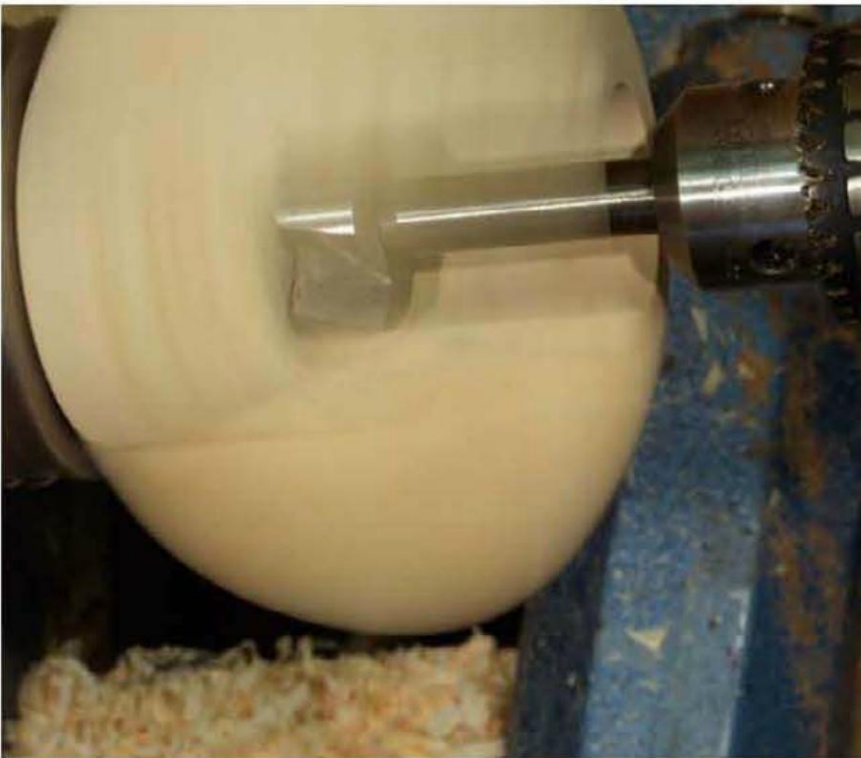
Drill the central depth hole.
