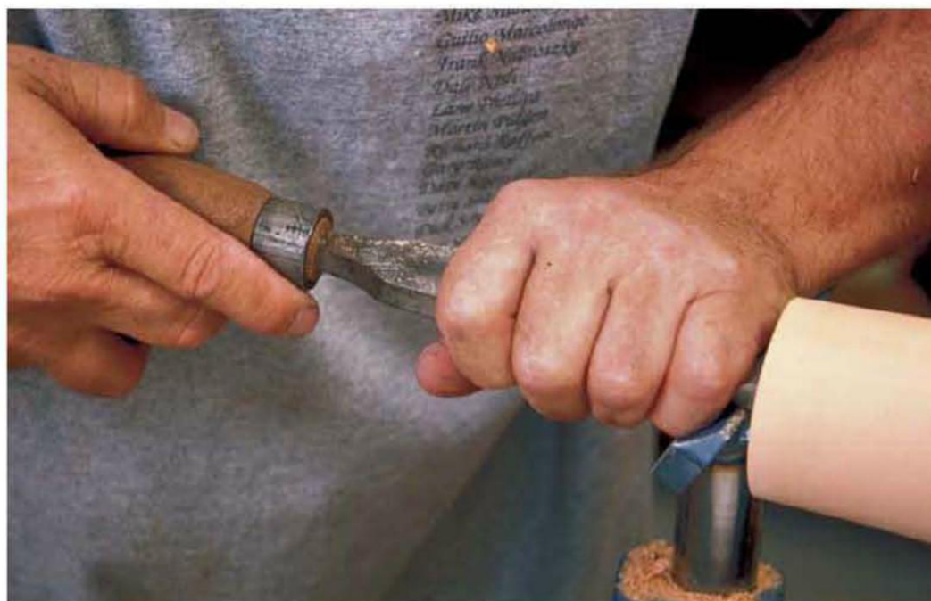
A squeeze grip gives you very fine control over the forward movement of the edge.
