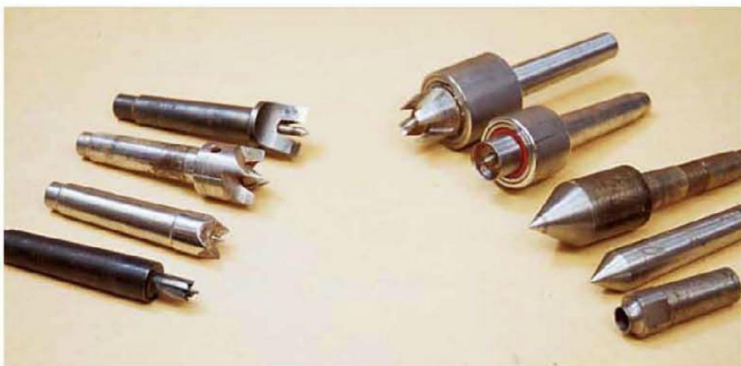
At left are typical spur drives. Those in front are for spindles smaller in diameter than the standard upper drives. At right are four types of tail centers. From the top right: two live cup centers, a live center, a dead center, and a hollow center for use with an auger or drill.
