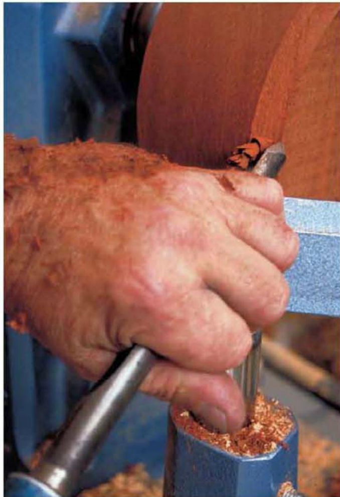
This is a normal hand-over grip cutting left.
