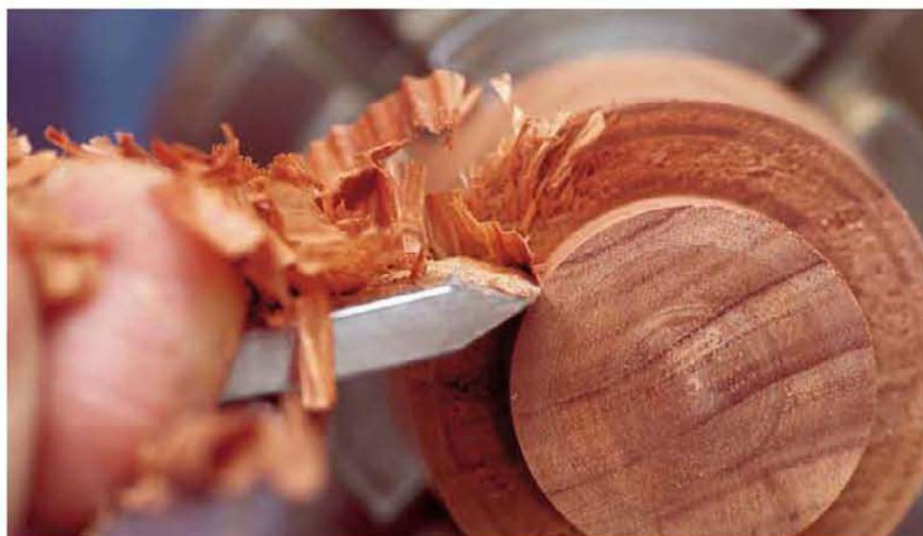
(TOP) You can reduce a cylinder rapidly by using a rotary-peeling action. Keep the cutting edge just below the surface of the wood. (BOTTOM) As the edge peels, raise the handle while pushing the edge forward to maintain the relationship of the cutting edge to the wood.
