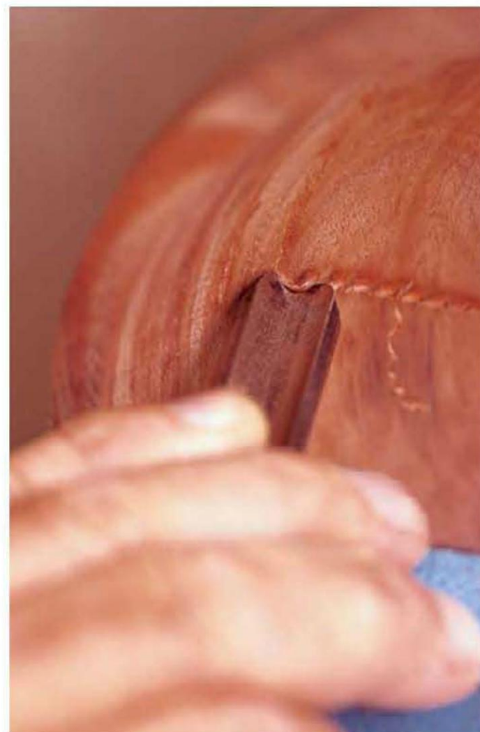
A deep-fluted gouge is used flute up for a back-cut—the finest finishing cut. Note how the rounded wing of the tool keeps clear of the wood and the possibility of a catch.
