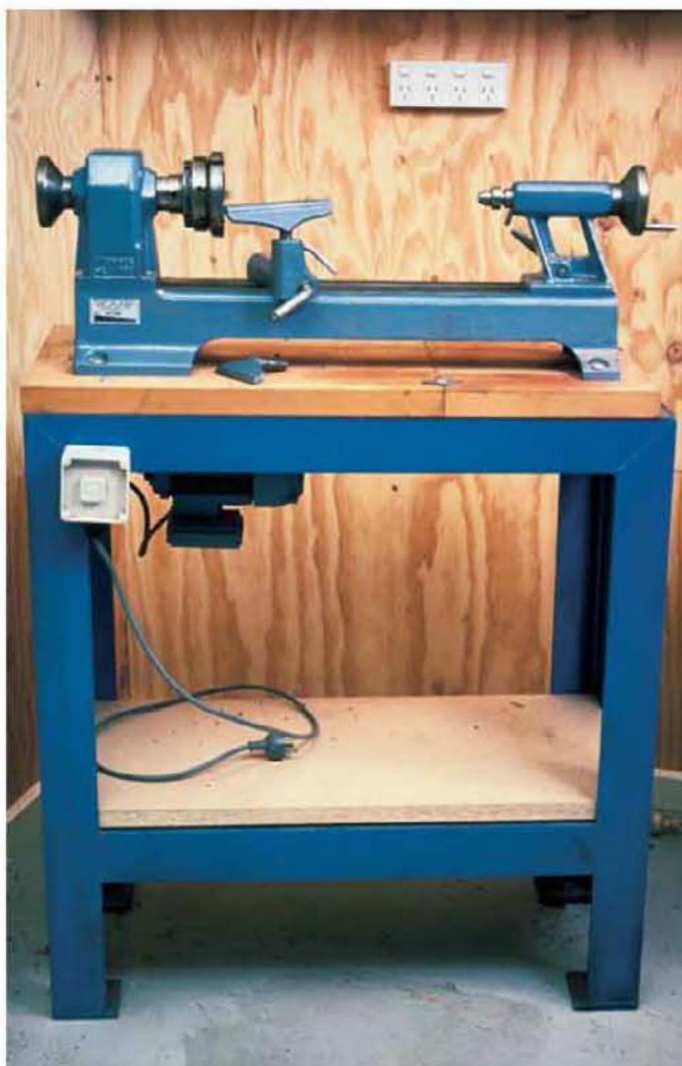
Mounted on a custom stand made of 3-in. (75mm) angle iron, this mini lathe will swing 9 in. (230mm) and accept 13¼ in. (350mm) between centers.
