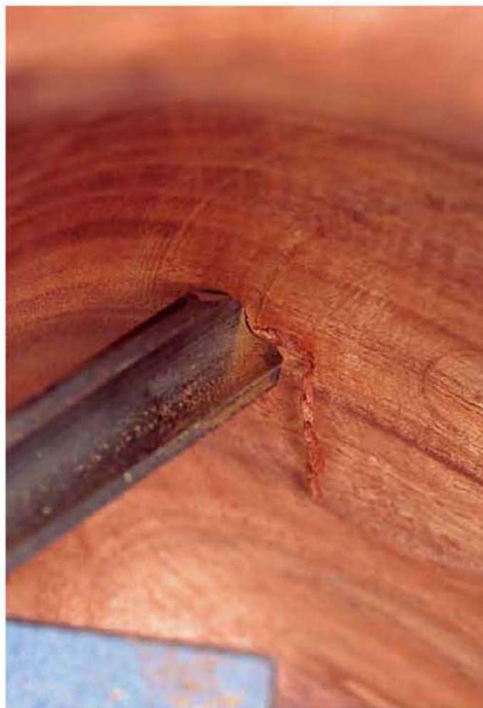
To shear-cut across the bottom of a deep form, you need a steep bevel on the nose and right wing of your gouge.
