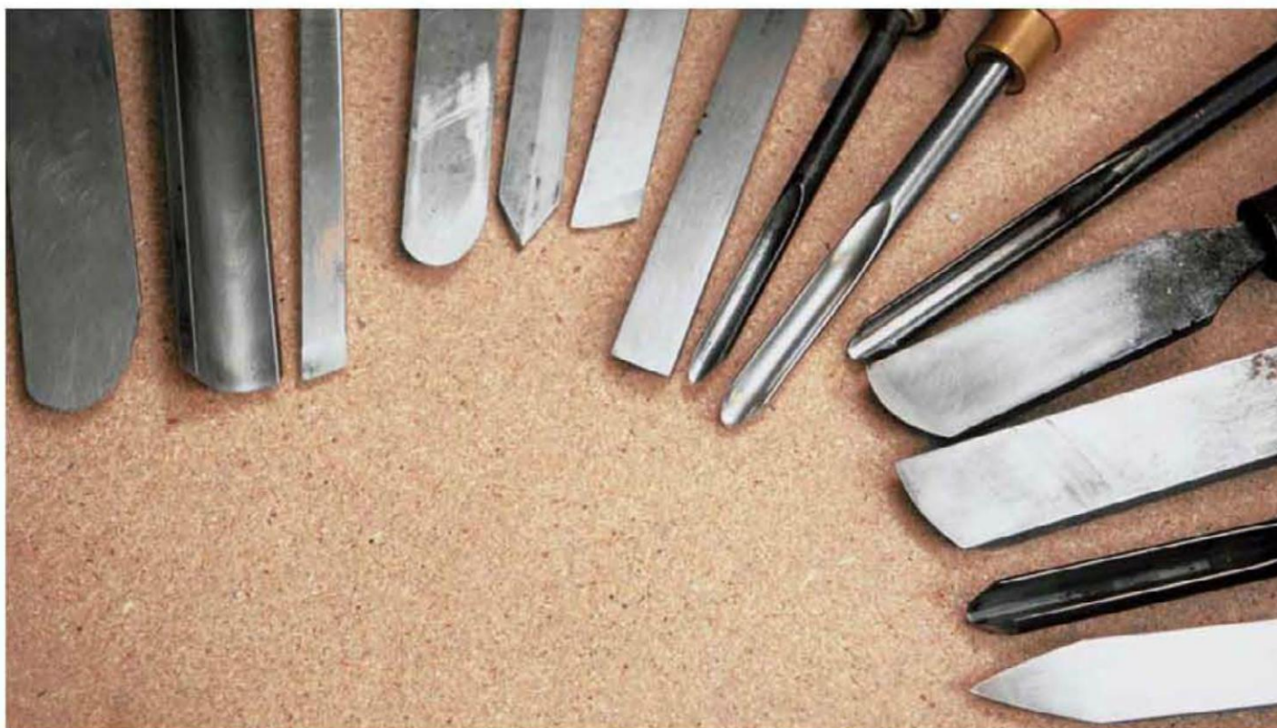
Basic tools, clockwise from left: 1½-in. (32mm) long-and-strong round-nose scraper; 1-in. (25mm) shallow spindle roughing gouge; ½-in. (13mm) skew chisel; 1-in. (25mm) round-nose scraper; parting tool; ¾-in. (19mm) standard skew chisel; ¾-in. (19mm) square-edge scraper; ¾-in. (9mm) shallow gouge; ½-in. (13mm) shallow gouge; ¾-in. (9mm) deep-fluted bowl gouge; 1½-in. (32mm) long-and-strong bowl scraper; 1½-in. (32mm) long-and-strong bowl scraper; ½-in. (13mm) deep-fluted bowl gouge; and 1-in. (25mm) spear-point scraper.
