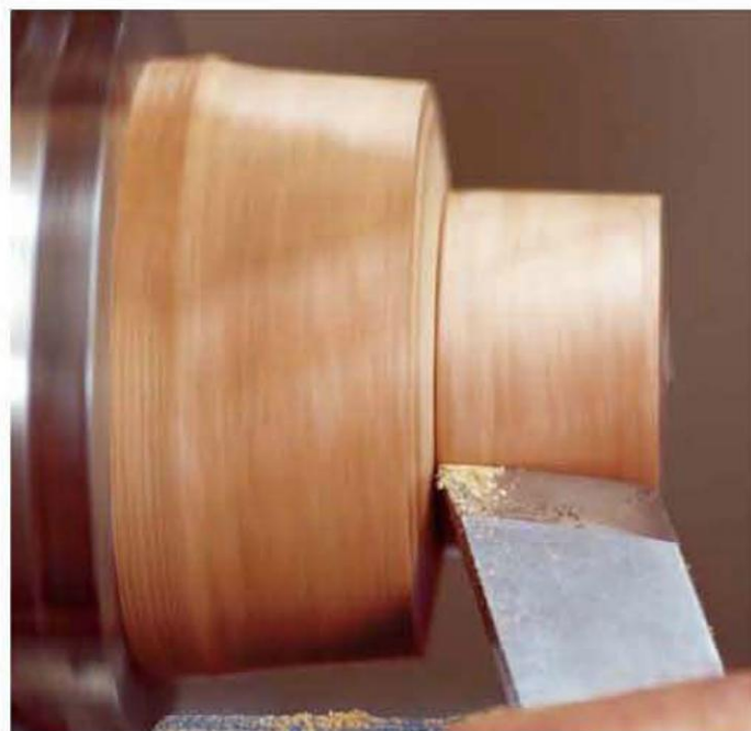
A curved edge skew is particularly useful for delicate low-peeling cuts. Here the long point reaches into the corner without touching the rest of the surface.
