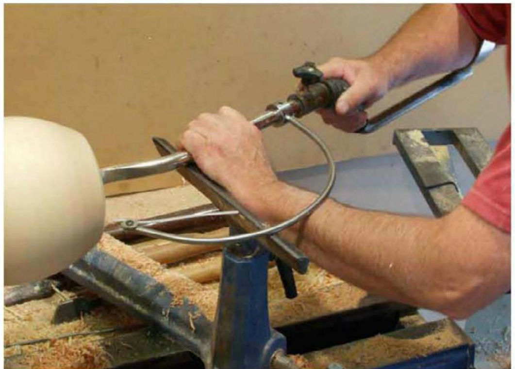
Since the mid 1980s the Stewart System has been the hollower of choice for many vessel turners.
