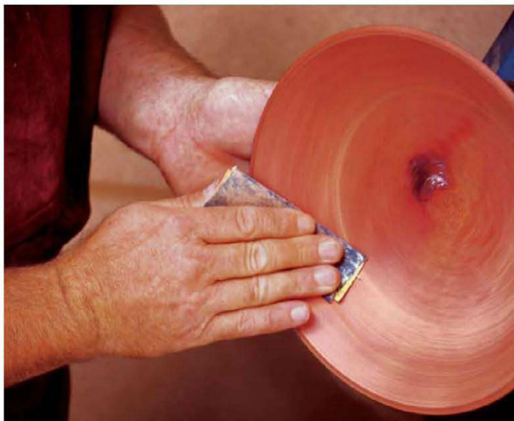
When sanding a fragile bowl, don't wrap abrasives around your fingers. Support the work with your free hand to equalize the pressure of the sanding.
