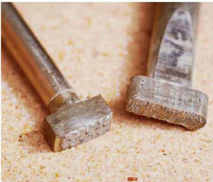
Diamond-wheel dressers are by far the best tools to keep your grinding wheels clean and running true.
