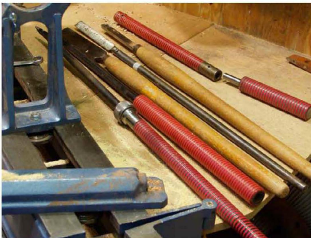
For deep hollowing, a handle should be about four to five times longer than the distance between the cutting edge and the rest.
