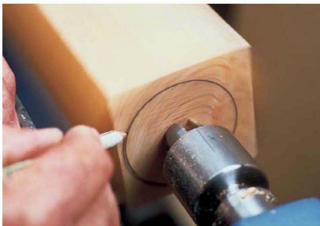
A circle marked on end grain shows how far off-center a blank is mounted.
