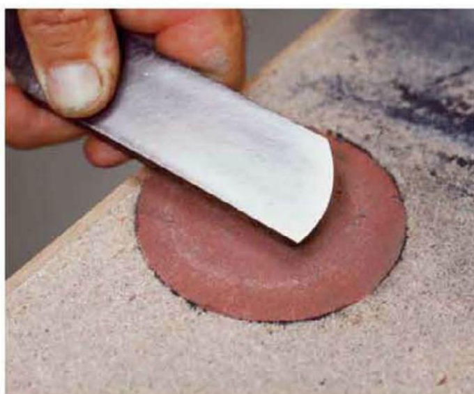
To prepare scrapers for grinding, I rub them on a used 100-grit sanding disc stuck on the bench close to the grinder.
