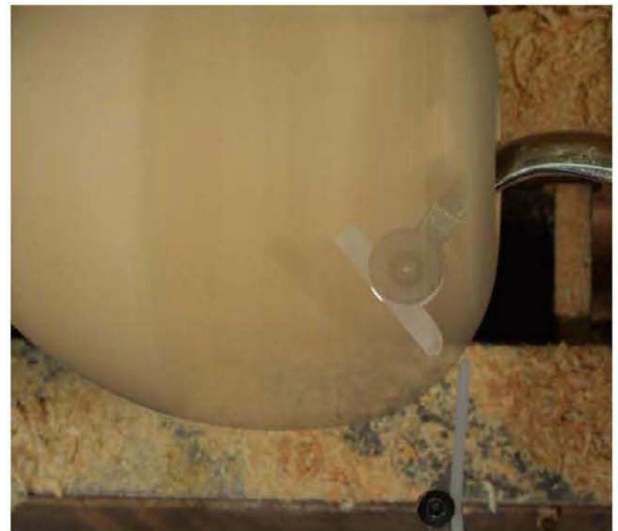
A swan-neck cutter refines an undercut with the aid of a hoop calliper.
