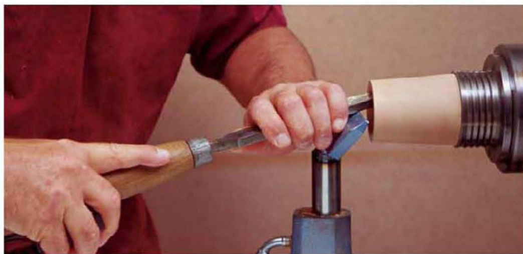
The large round-nose scraper is tilted upwards to shear-cut as I begin smoothing an internal curve.
