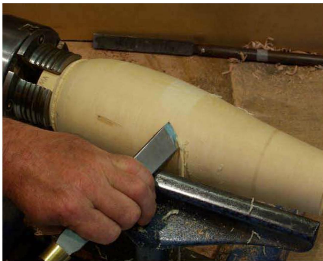
Once a form is roughly hollowed, the profile of the vessel should be completed to the initial sanding stage. Use the standard techniques for face work (TOP), and center work (BOTTOM).
