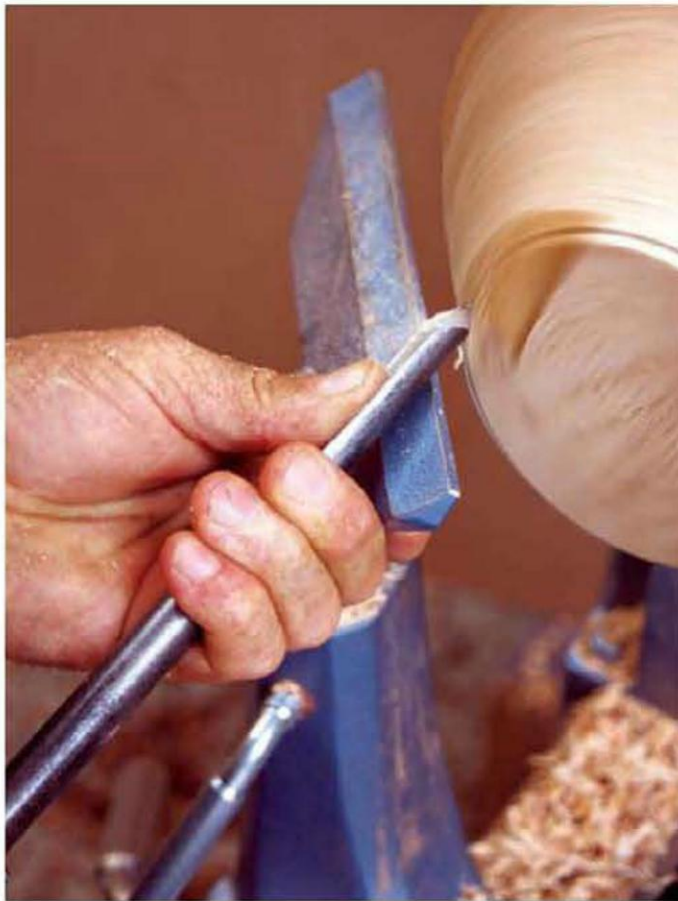
The tool is easier to steer when it's pointing in the direction you're cutting. Note that this shallow gouge is rolled over about 45°.
