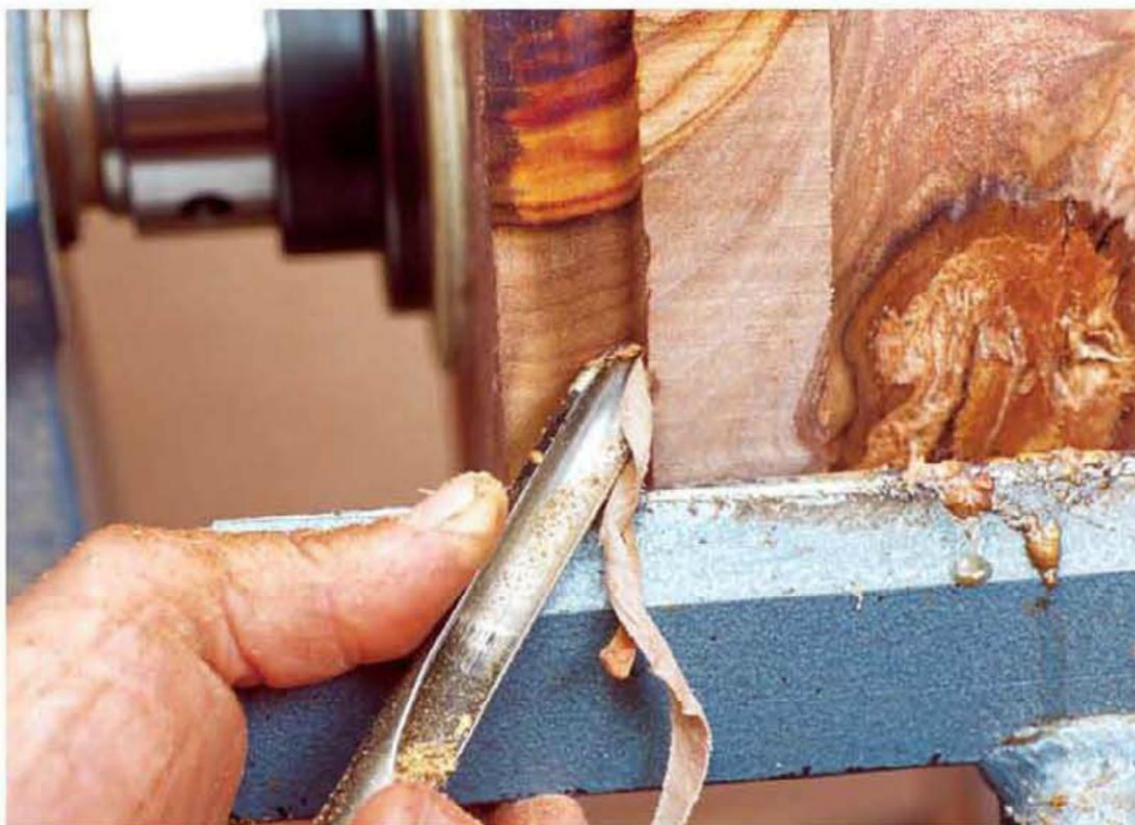
Always cut in from a face to prevent the corners from splintering.
