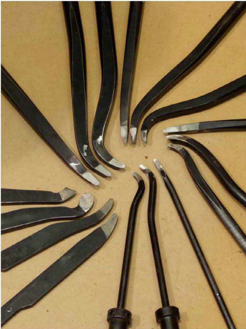
With sets of bent scrapers like these Kelton Hollowers you can hollow vessels as small as 2 in. (50mm) diameter with \frac{5}{8} in. (16mm) openings; and at the other end of the scale are tools with a reach of about 18 in. (460mm). They can be used freehand or in hollowing rigs.
