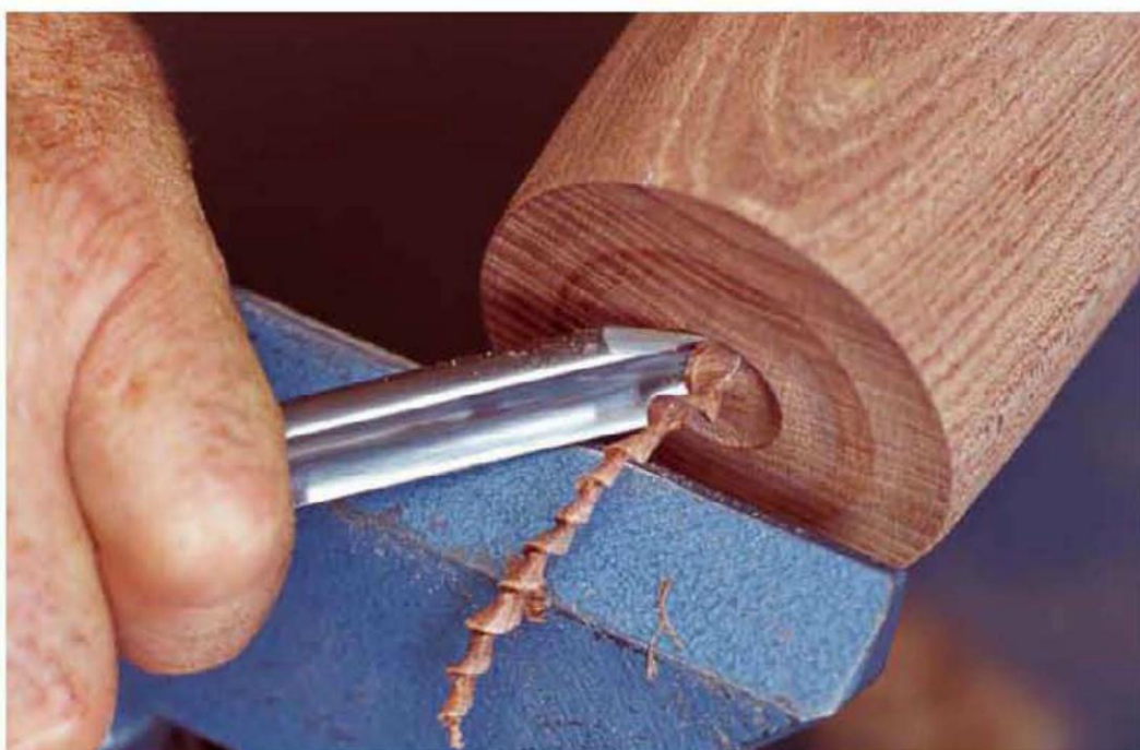
Start the back-hollowing near center to create a small opening.
