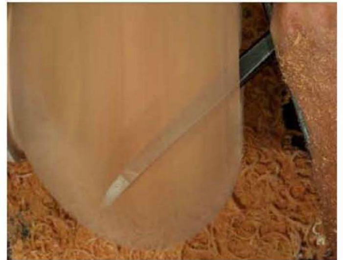
Three Kelton Hollowers are employed on different portions of the curve as it is refined.
