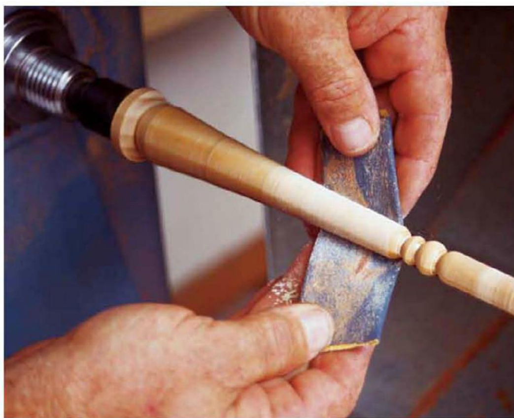
Hold both ends of the abrasive when sanding a spindle. By working from below, you can see what you're doing.
