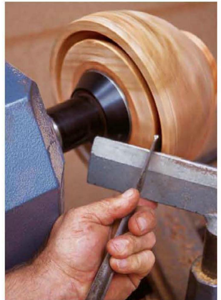
A Stewart System Slicer is used to save the inside of a bowl.
