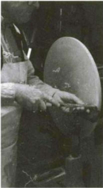
An outboard tool base on some lathes allows turning of large faceplate work off the back end of the spindle, with the rigidity of inboard turning.
