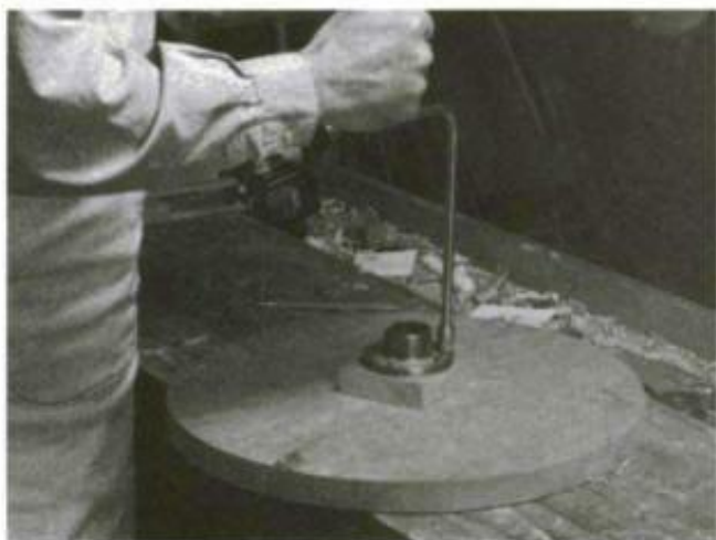
1. Cut a glue block of sufficient size, attach it to a faceplate and scrape the block flat. Then glue and screw the assembly to the blank.
