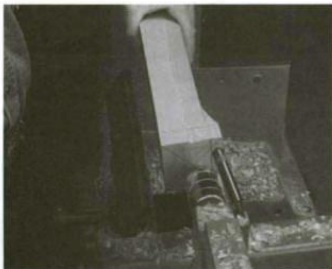
1. Mount the trimmed billet on the second axis and rotate it by hand to be sure it does not hit the tool rest.
