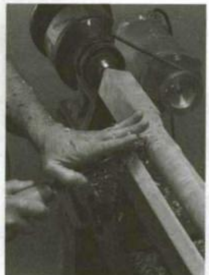
3. Use a roughing-out gouge to bring the billet round.
