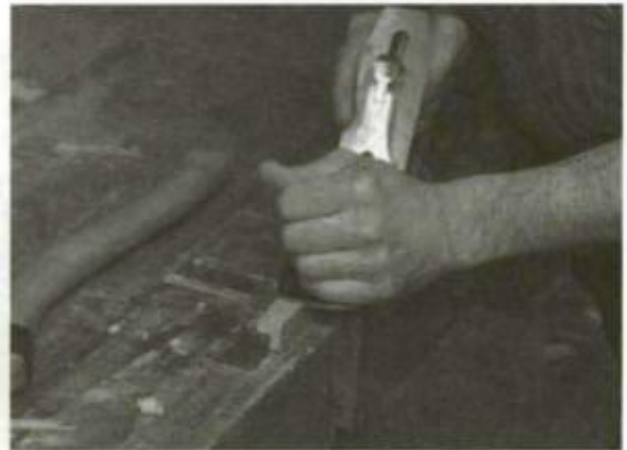
2. True up the sides with a hand plane.
