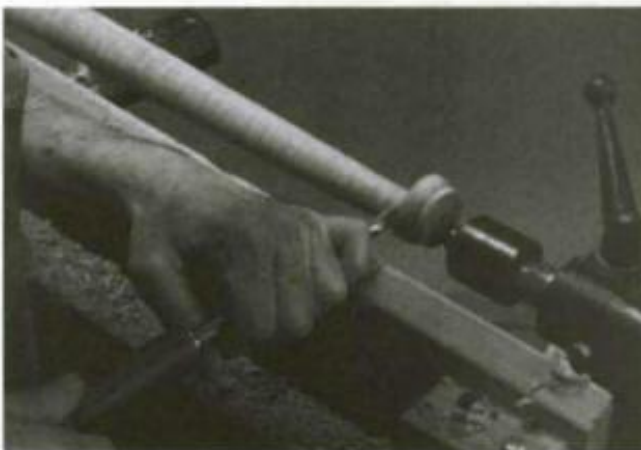
5. Finish turning the top of the foot with a 1/2-in. spindle gouge. Place the gouge high and raise the handle until it cuts, then cut a cove to form the top of the foot.
