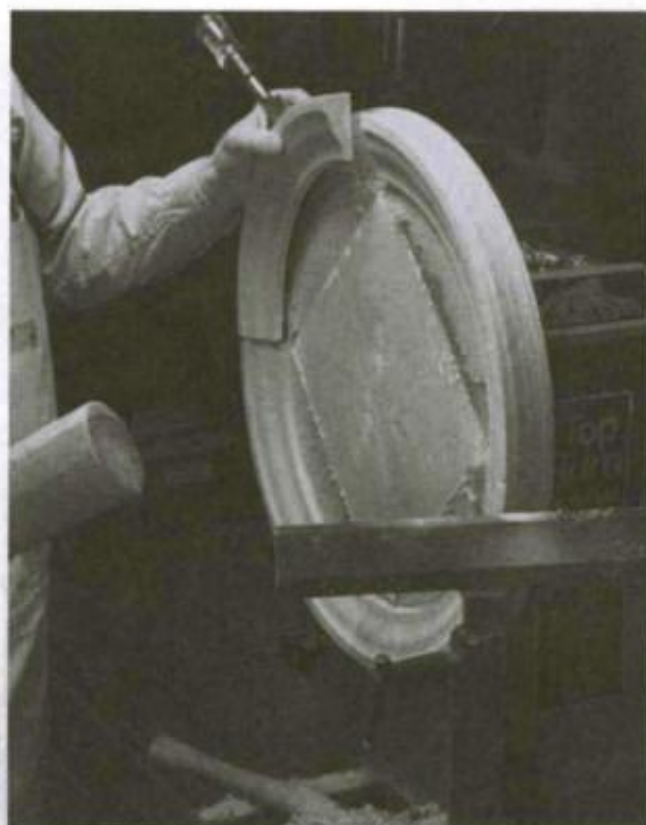
4. Insert a chisel between the molding and the faceplate and give it a sharp rap with a mallet to remove a finished section.
