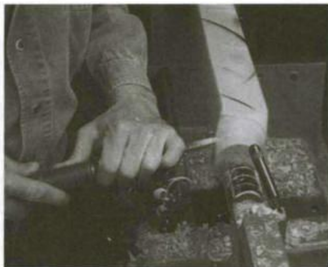
2. Turn the foot. Make it slightly longer than necessary at this point (it will be corrected when the ankle is turned).
