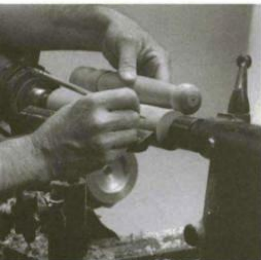
A master part provides a tangible reference for adjusting calipers and dividers, and it serves as the visual informant for turning further parts.
