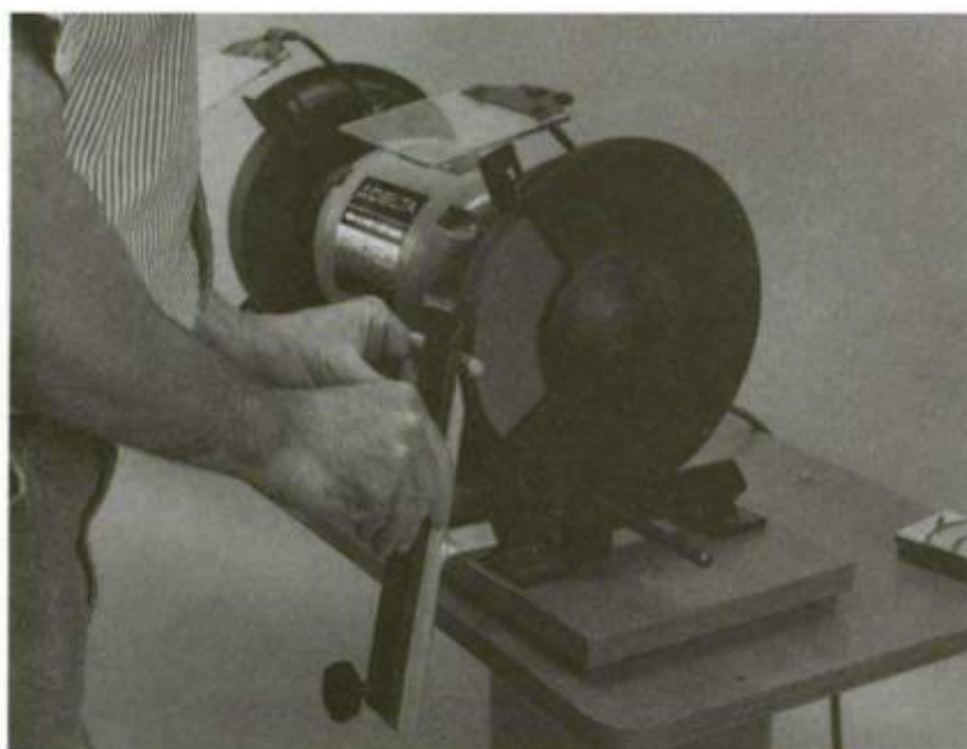
The Oneway dressing jig presents the diamond dresser to the wheel at the correct 5° negative (downhill) angle and ensures that the wheel is dressed true to its axis.
