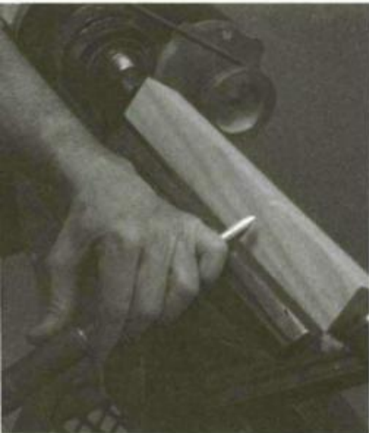
All lathes come with one or two tool rests, usually 6 in. and 12 in. long. The 6 in. rest is reserved for small work, like knobs and finials, and the 12-in. rest is used most of the time.
