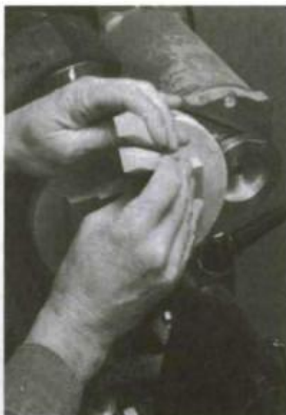
2. Rip the last cleat in half at an angle to make it easy to take blanks in and out of the chuck.
