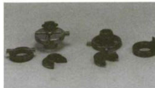
The scroll of each chuck engages the rack on the bottom of the base jaw, moving it in or out, depending on what direction the scroll is turned. (The scroll for the Nova is on the right; the Oneway is on the left.)
