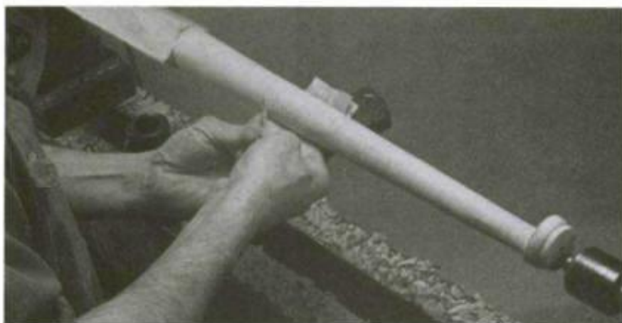
7. Sand the shaft and the top of the foot while offset, then remount the leg on the true centers to sand the bottom of the foot and the pad.
