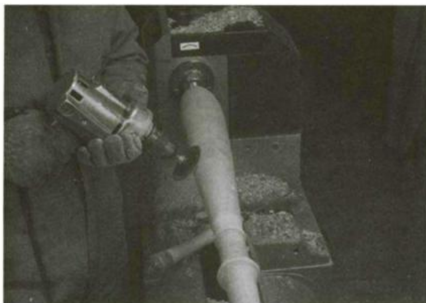
A rubber sanding pad mounted in a high-speed electric drill is perfect for cleaning up cylinders and tapers, quickly removing tool marks and slight imperfections.
