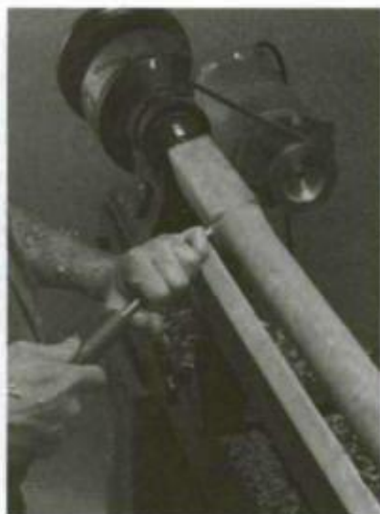
4. Turn details in the post using a spindle gouge.
