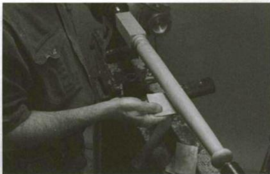
5. Sand and finish the completed post.
