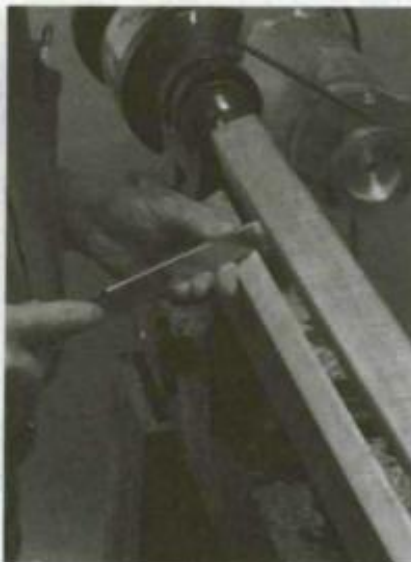
2. Use the toe of a skew to cut a shoulder at the bottom of the pommel.
