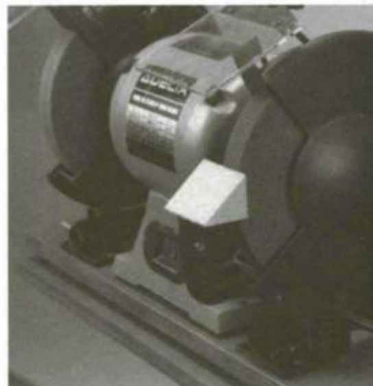
A one-piece cast rest is easily modified so that it can be used with turning tools. Simply attach a wedge of wood to the rest with double-sided tape or sheet-metal screws.
