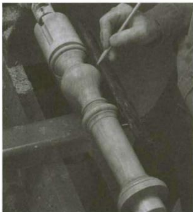
1. In conjunction with an indexing mechanism, use the tool rest to lay out the flute or reed pattern.
