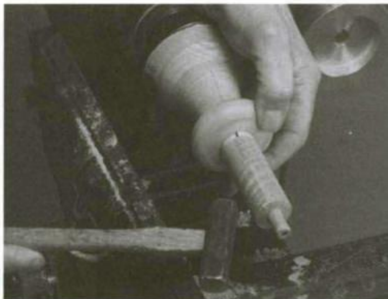
2. Tap the ring with a mallet to tighten the jaws.
