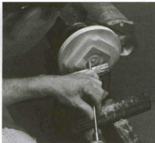
5. As long as all the blanks are the same size, the nest chuck will hold them tightly.
