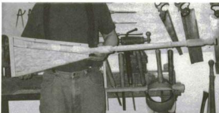
This chuck allows the turning of bent spindles. It has a notch in it to accept the bent portion of the spindle, and it can be counterbalanced with sand or weights to eliminate vibration. In use, the "broom" end is driven by the headstock, and the handle spins balanced on the tailstock.
