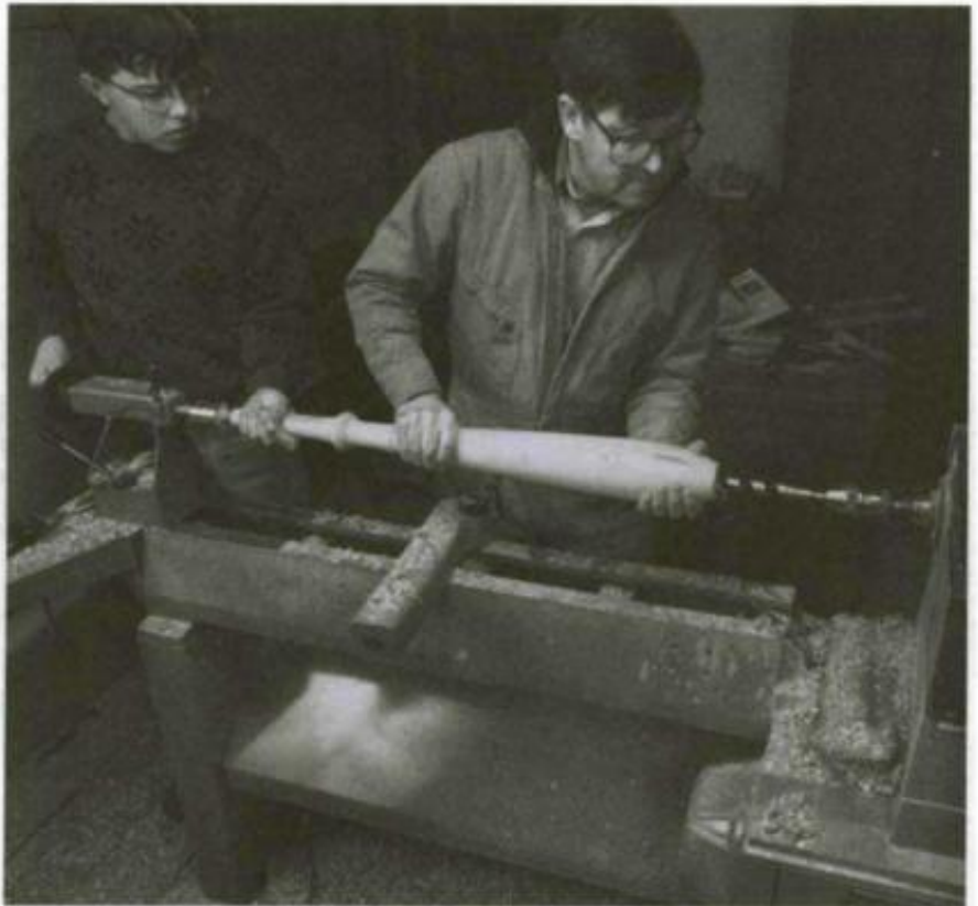
If your lathe is big enough to accept both the post and the drill bit, you can drill the mortise on the lathe.
