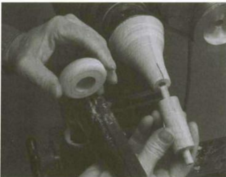
1. Mount the billet in the chuck.
