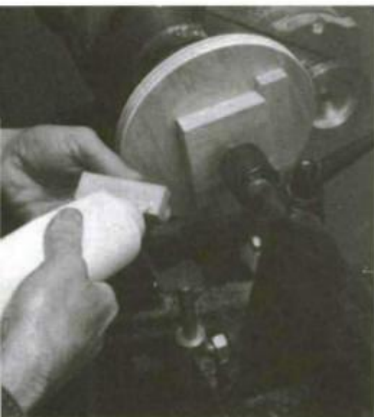
1. Fasten a piece of plywood to the faceplate, then glue and nail three cleats to the plywood to form a U.
