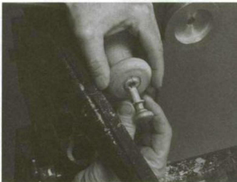
4. When you're finished with the first pull, remove it and mount the second. To loosen the ring, you may need to give it a few sharp raps with a mallet.
