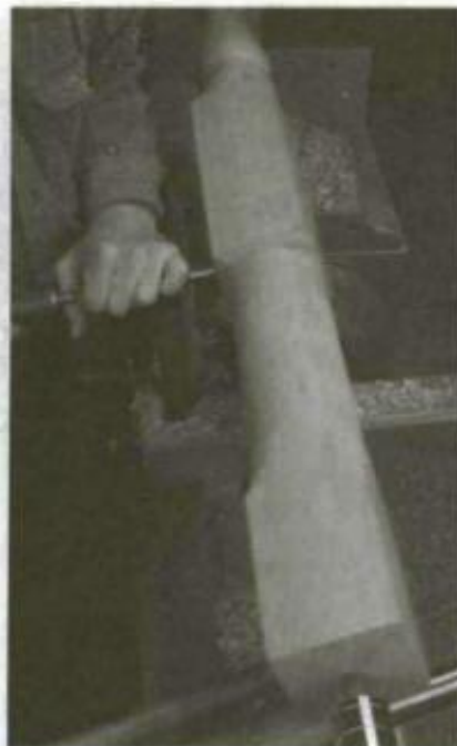
2. Use the spindle gouge to shape the shoulders.
