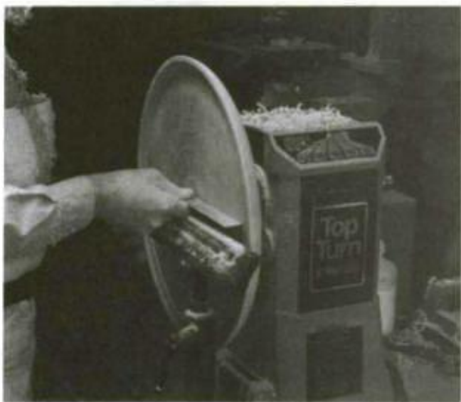
4. Use a straightedge to check the surface for flat.
