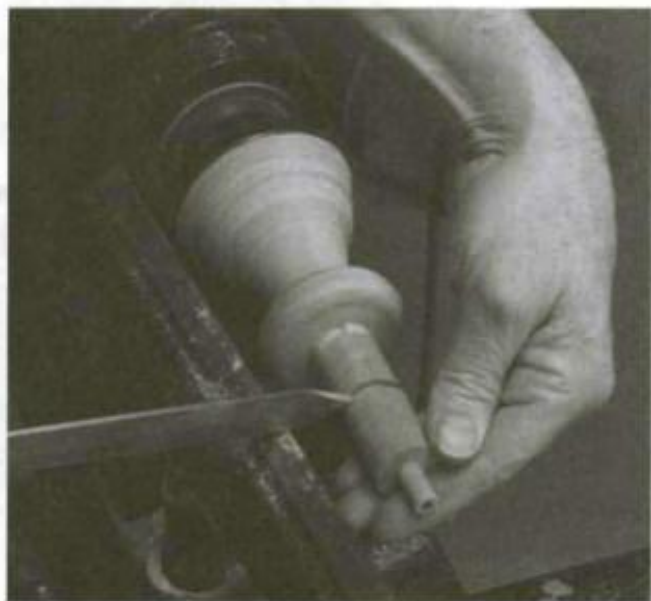
3. Use a cutoff tool to part the billet in the center and then turn the first pull. Be sure and turn the chuck down to match the base diameter of the pull so that you match subsequent pulls without using calipers.
