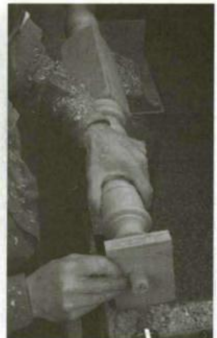
3. Turn a generous tenon, in this case 1-in. diameter by 4-in. long, at the top of the section. Check the size of the tenon with a test block drilled the same size as the mortise.
