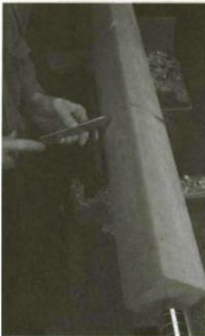
1. From 3¼-in. stock, use the toe of the skew to cut the transitions from square to round on the bottom section of the post.
