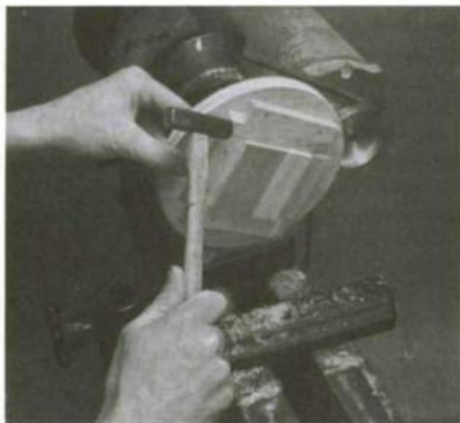
4. The other half of the cleat serves as a wedge to capture the blank in the chuck.
