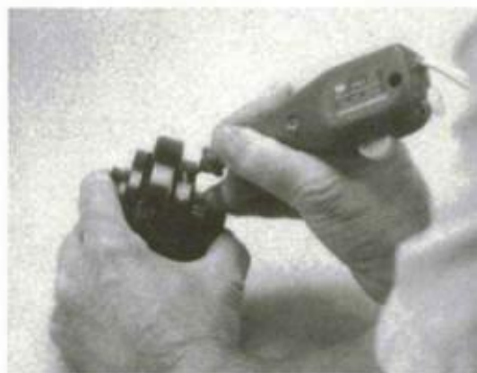
Engraving an arrow on the scroll chuck will help you remember which way to turn the lever to tighten or loosen.
