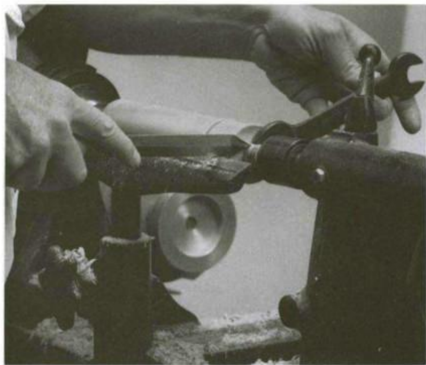
An open-end wrench is a tool that makes it easy to size tenons.
