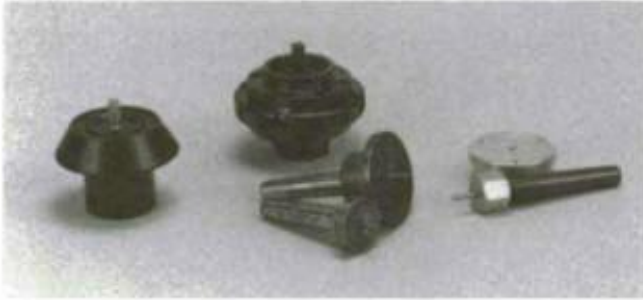
The Glaser screw chuck (left) and the Nova scroll chuck with screw-chuck accessory (middle, back) can hold fairly large work. Traditional screw chucks built on Morse tapers (front middle and right) are for small work.
