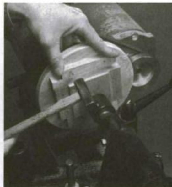
3. Nail one half of the cleat to the chuck.
