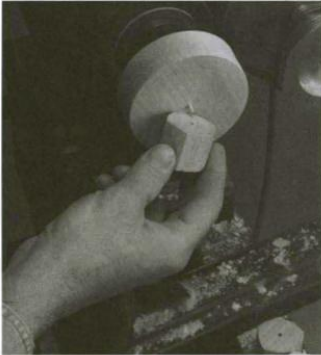
Thread a blank onto the homemade screw chuck, then turn it round using a \frac{1}{4} -in. bowl gouge.
