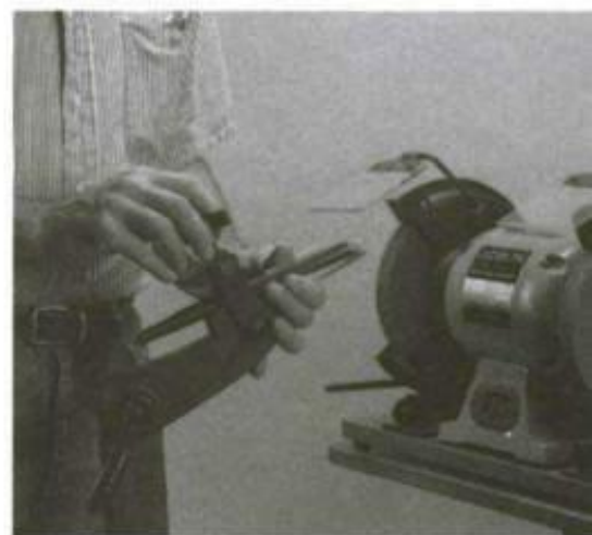
A plastic tube supplied with the Glaser Jig helps get the tool adjusted in the jig. Simply slide the tool forward until the tip is even with the end of the tube.
