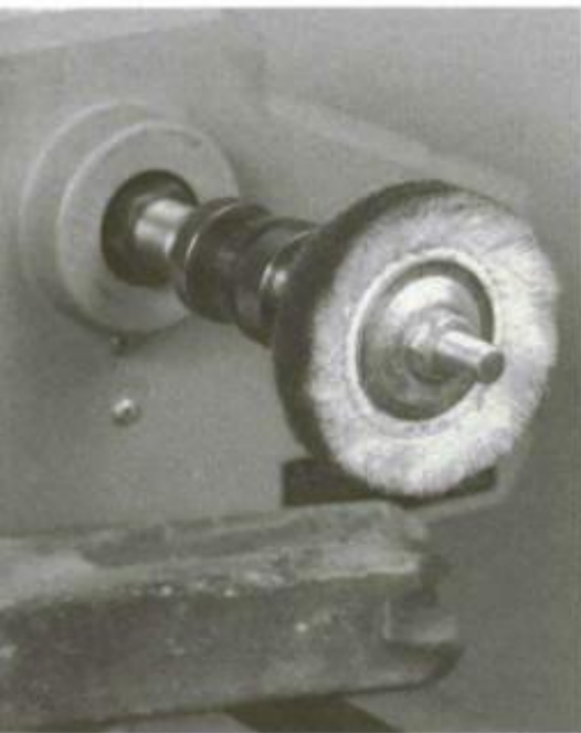
Mounting a buffing arbor in the lathe makes an inexpensive buffer.
