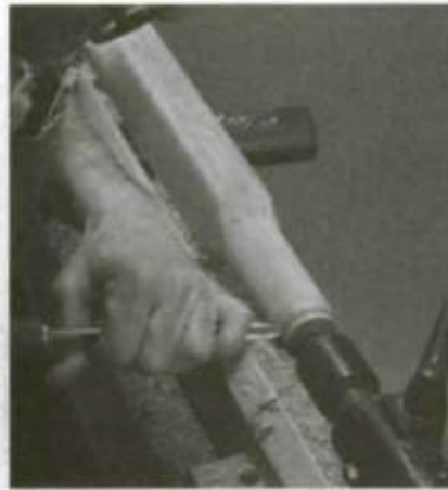
2. Mount the billet on the true center points, turn the bottom of the pommel and then the foot and pad.
