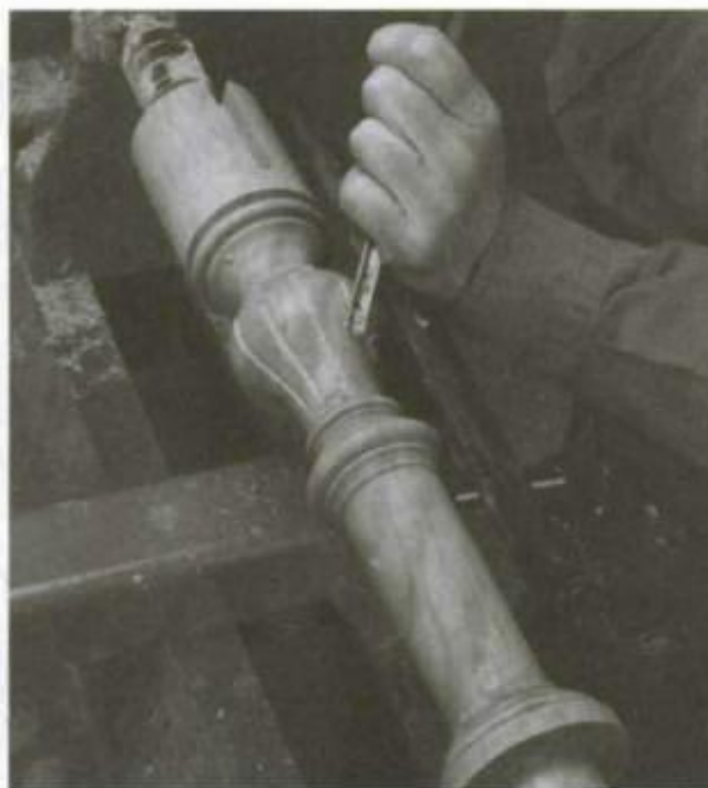
2. Following the pencil layout, use the tool rest to guide your chisel in cutting the flutes or reeds. Light blows with a carver's mallet work much better than trying to push the gouge by hand.
