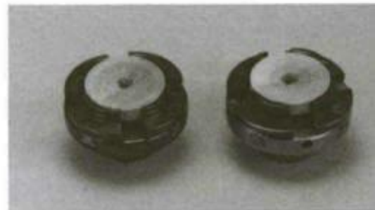
The Nova (left) and Oneway (right) scroll chucks are nearly identical, right down to their diameters and jaw sizes. These commercial chucks are made specifically for wood turning.
