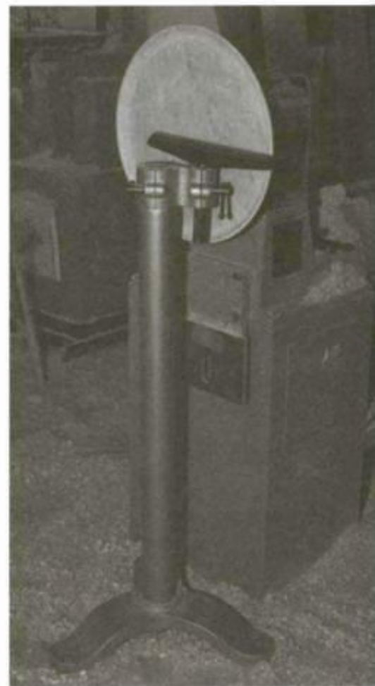
Because a floor-stand rest does not have the rigidity of a normal tool base, it should be used only with light scraping cuts.
