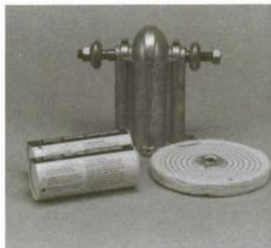
An inexpensive jack shaft mounted to a motor makes a simple buffer.
