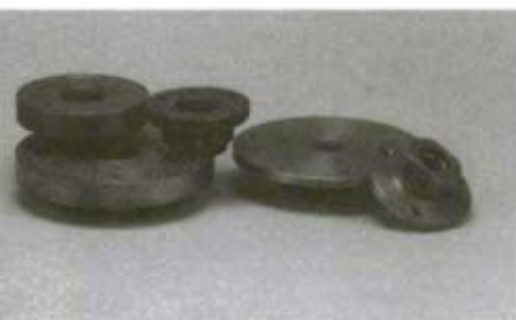
Faceplates are used to mount flat work on the headstock spindle.
