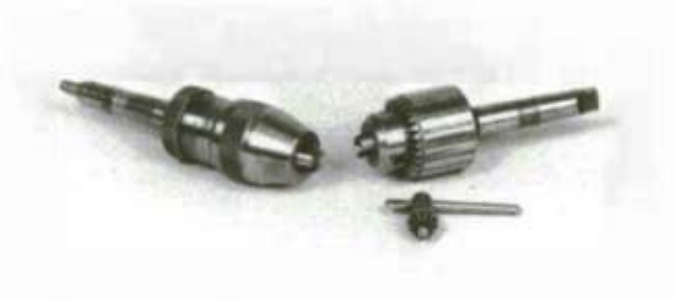
Drill chucks (also known as Jacobs chucks) are great for mounting drill bits and other accessories in either the tailstock or headstock spindle.
