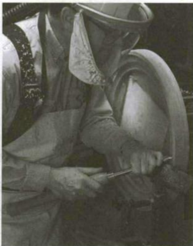
3. Turn the molding. This can be done inboard or outboard, depending on the size of the molding and your lathe.
