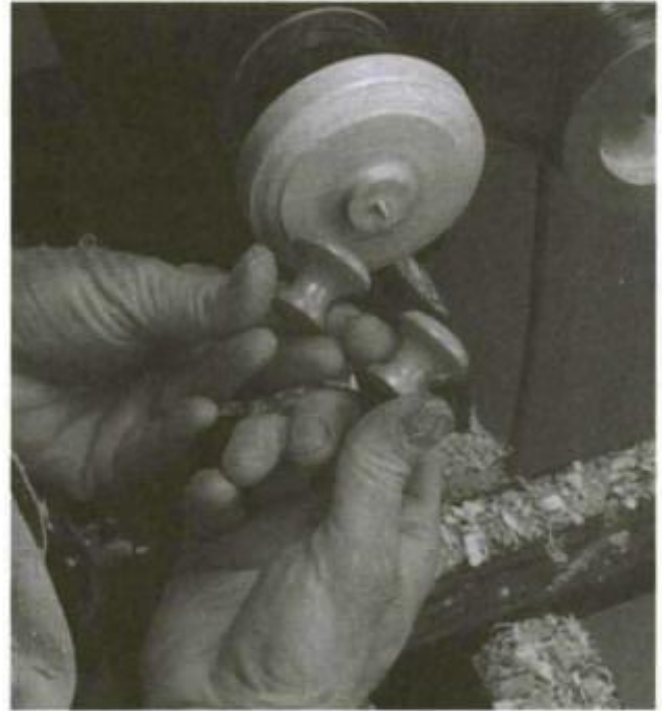
To make duplication easier, trim the screw chuck to match the base diameter of the knob. You won't have to use calipers to size the base—the screw chuck will be the guide.
