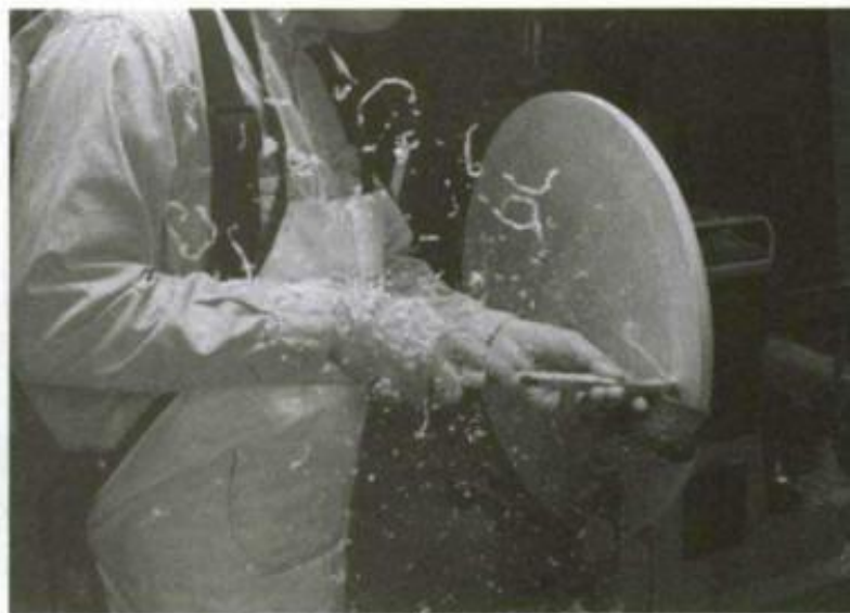
2. Make the initial cuts with a scraper to flatten the top.
