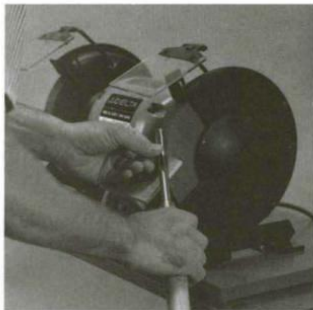
As you swing the tool, simultaneously tip its handle upward and rotate the handle slightly. The rotation is clockwise if swinging to the right and counterclockwise if swinging to the left. Repeat in mirror image for the other half of the tool.
