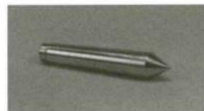
A dead center consists of a simple pivot on which the work spins. Many lathes include such a center in the standard accessory kit. Dead centers must be lubricated to reduce friction and burning.
