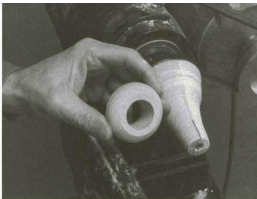
This chuck is a simple shop-built collet. The hole in the center matches the diameter of the tenon on the pull to be turned. The ring is forced down over the tapered end and closes the "jaws" around the tenon.
