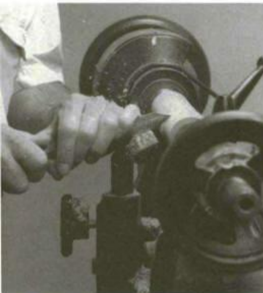
When shear cutting with the cutoff tool, place the edge of the tool on the rest and present it at too high an angle to cut. Then slowly raise the handle until the tool begins the cut.
