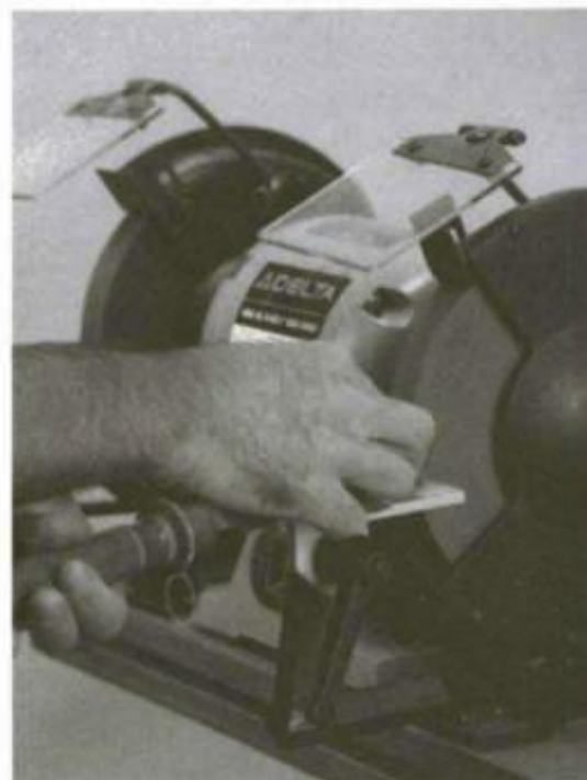
When grinding a flat bevel for a skew on the side of the wheel, the top half of the tool tends to be ground more than the bottom. To compensate, put additional pressure on the bottom half with your thumb.
