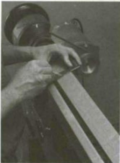
1. Lay out the pommel with a pencil, a square and a ruler. You need only mark a square line on one side of the billet.
