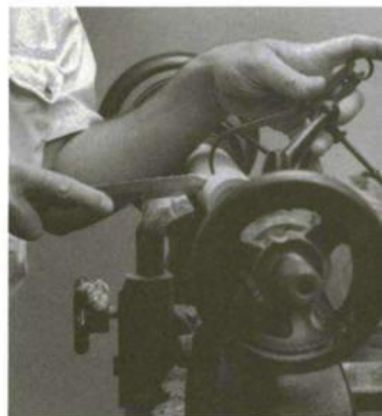
Calipers can help you determine an exact diameter easily.
