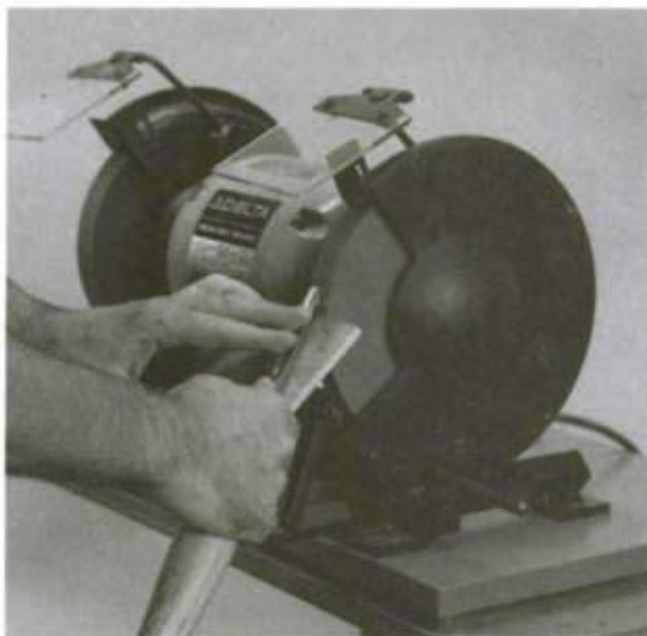
When sharpening a spindle gouge freehand, touch the nose of the tool to the wheel (with the table set to 30°) and immediately start swinging the tool either to the right or the left. In this case the author is swinging to the right.
