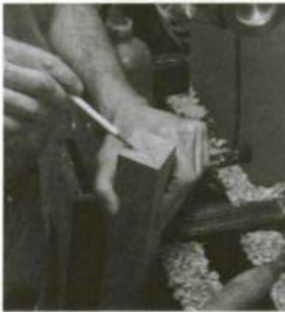
1. Lay out the true and offset center points. Then punch them to make mounting easier and more accurate.
