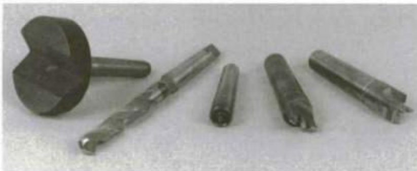
Accessories with Morse tapers expand the capabilities of your lathe. Shown here (from left) are a crotch center, a drill bit, a cup center and two drive centers.
