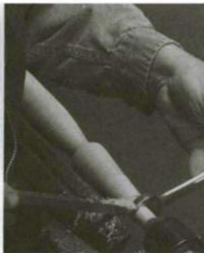
2. Turn the right half of the stretcher first (or left half if you are left-handed). Here the author is sizing the tenon using a bedan and an open-end wrench.
